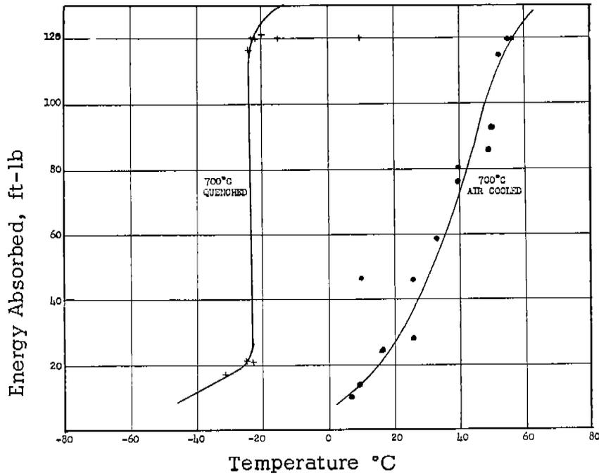
Fig. 11. Standard Charpy V-Notch Impact Tests of Alloy with 0.018% C Showing Effect of Precipitated Carbides.
