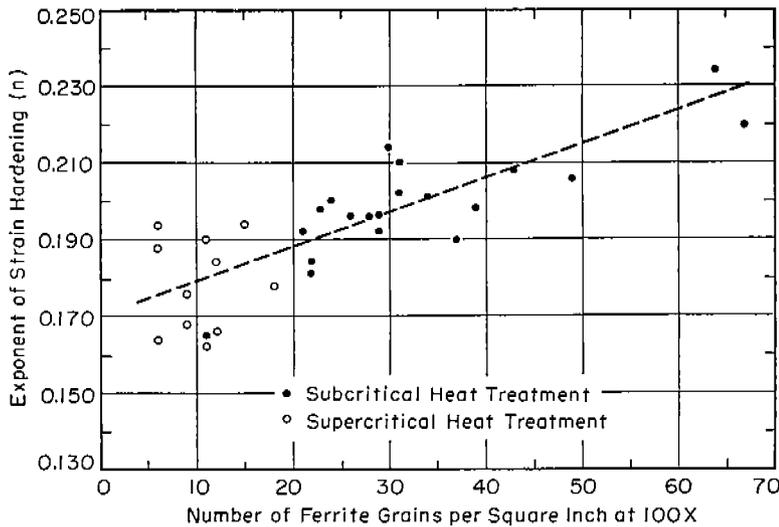
Fig. 8. Effect of Ferrite Grain Size on the Strain Hardening Exponent of an 0.02% Carbon Alloy Tested at Liquid Air Temperature.
