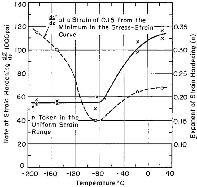
Fig. 6. Effect of Temperature on Strain Hardening. (0.02% carbon alloy heat treated subcritically.)
