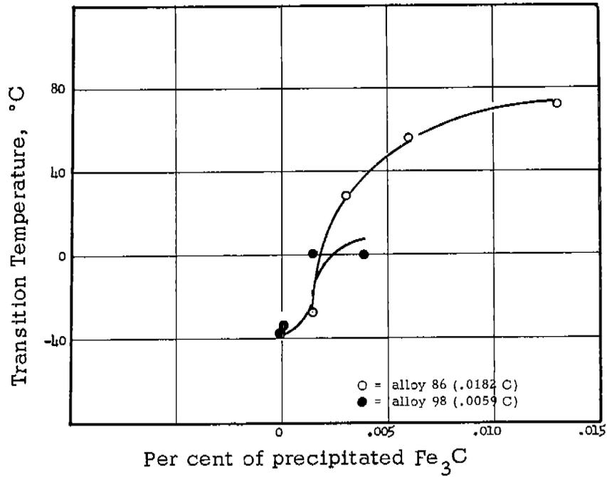
Fig. 10. Increase in Charpy V-Notch Transition Temperature with Increase in Amount of Precipitated Fe<sub>3</sub>C.
