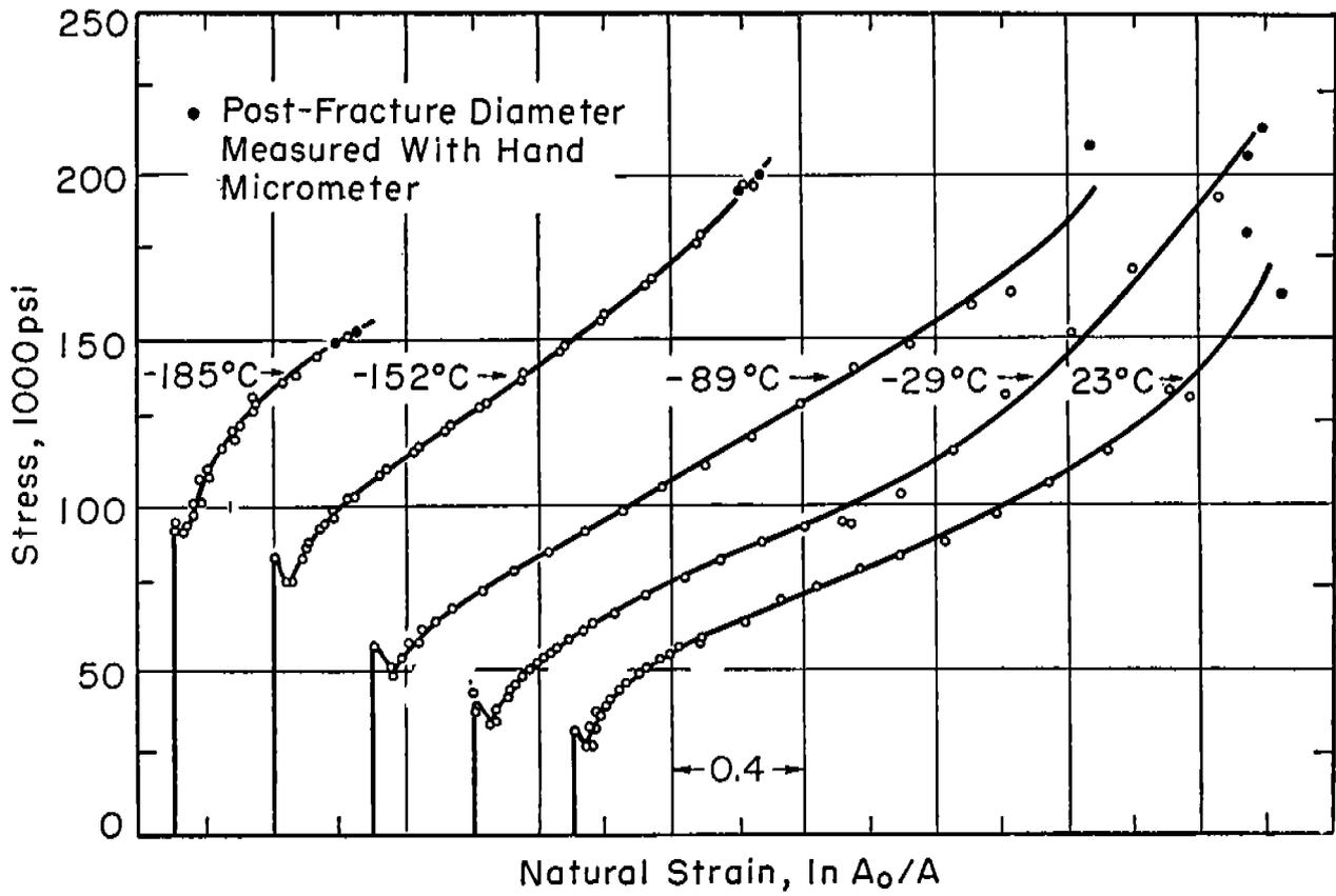
Fig. 1. Natural Stress-Strain Curves for Iron-Carbon Alloy Containing 0.02% Carbon.
