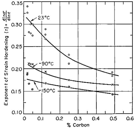
Fig. 7. The Effect of Carbon on the Exponent of Strain Hardening. All heat treatments are supercritical except for the 0.02% carbon alloy.
