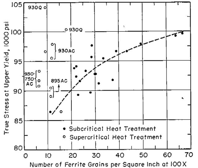
Fig. 9. Effect of Ferrite Grain Size on the Upper Yield Point at Liquid Air Temperature. (0.02% carbon alloy.)
