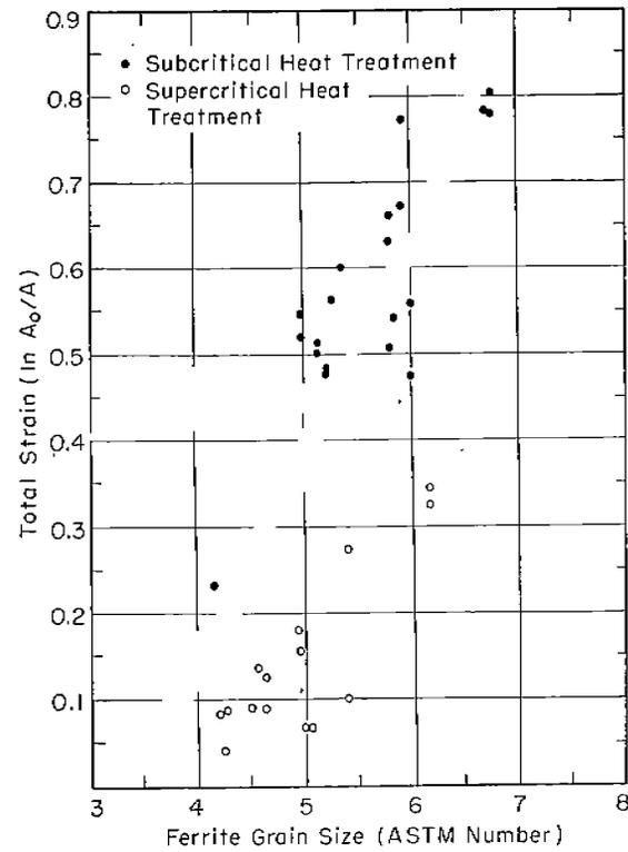
Fig. 5. Effect of Ferrite Grain Size on Total Strain at Liquid Air Temperature (0.04% carbon alloy.) (-185 C)
