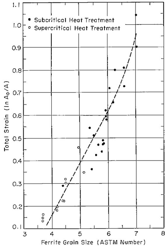
Fig. 4. Effect of Ferrite Grain Size on Total Strain at Liquid Air Temperature. (0.02% carbon alloy.) (-185 C)
