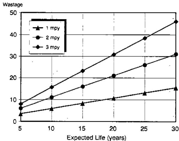
Figure 6. Mean Value of  $W_a$  as a Function of  $T$  and  $R_m$
