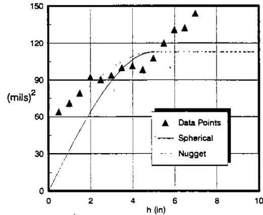
Figure 3. Fitted Semivariogram Models for Plate A
