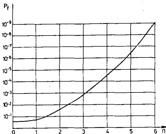
Fig. 2: Relation between reliability index and probability of failure.
