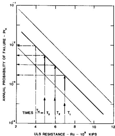
Fig. 15 Effect of Time (Fatigue Damage) on Platform Risk
