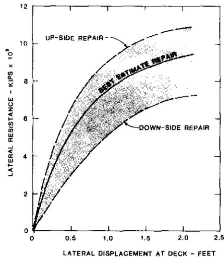
Fig. 11 Effect of Repairs on Platform Capacity
