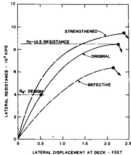
Fig. 10 Capacities of Original, Defective and Strengthened Platform
