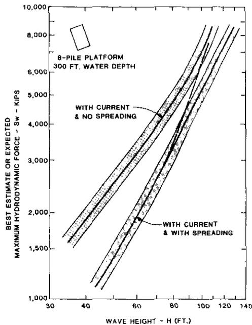
Fig. 7 Influence of Current and Wave Spreading on Hydrodynamic Forces
