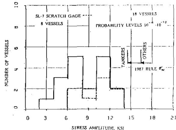
Figure 3 A Comparison of Deck Stress Measurements in Ships, with Wave Load Criteria Nominally used in their Design Assessment.
