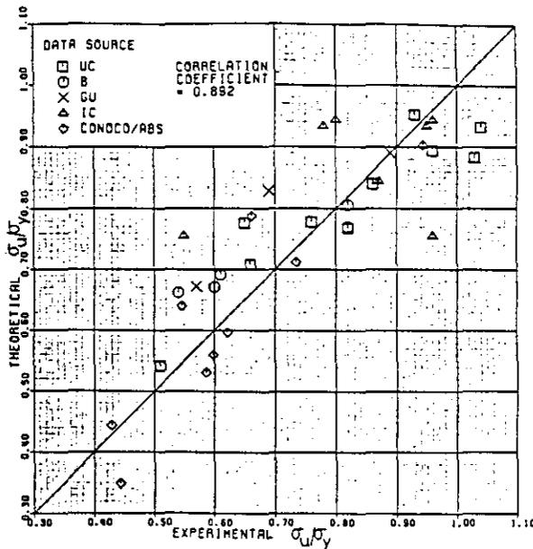
Figure 9 Comparison of Theoretical Strength of Orthogonally Stiffened Cylinders under Axial Compression with Test Data.
