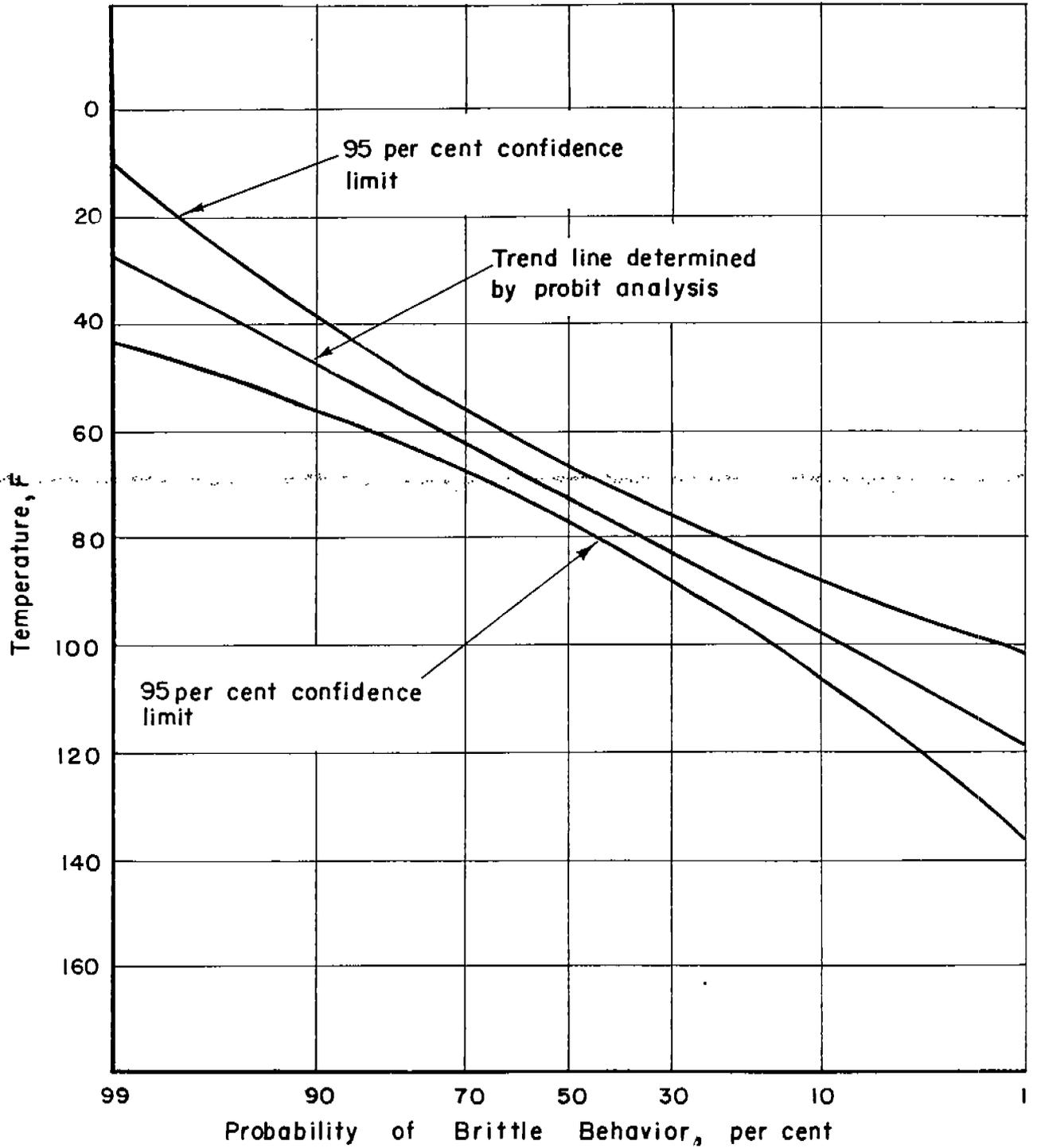
FIGURE 10. PROBABILITY OF BRITTLE BEHAVIOR IN NAVY TEAR TESTS ON TYPE A STEELS AT VARIOUS TEMPERATURES
