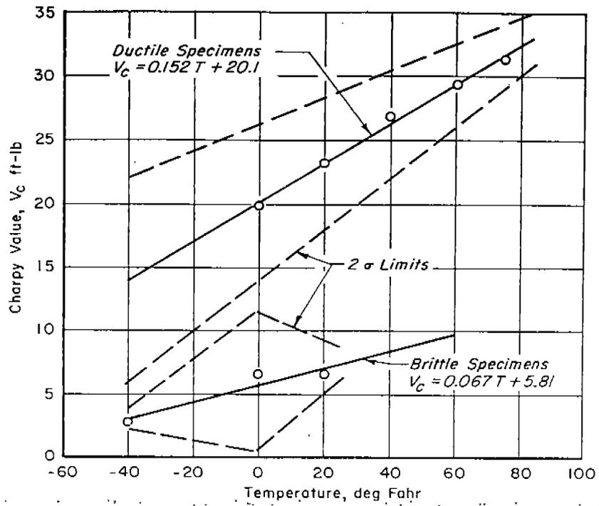
FIG. 5.—Keyhole Charpy Test Characteristics of Type A Steels.
