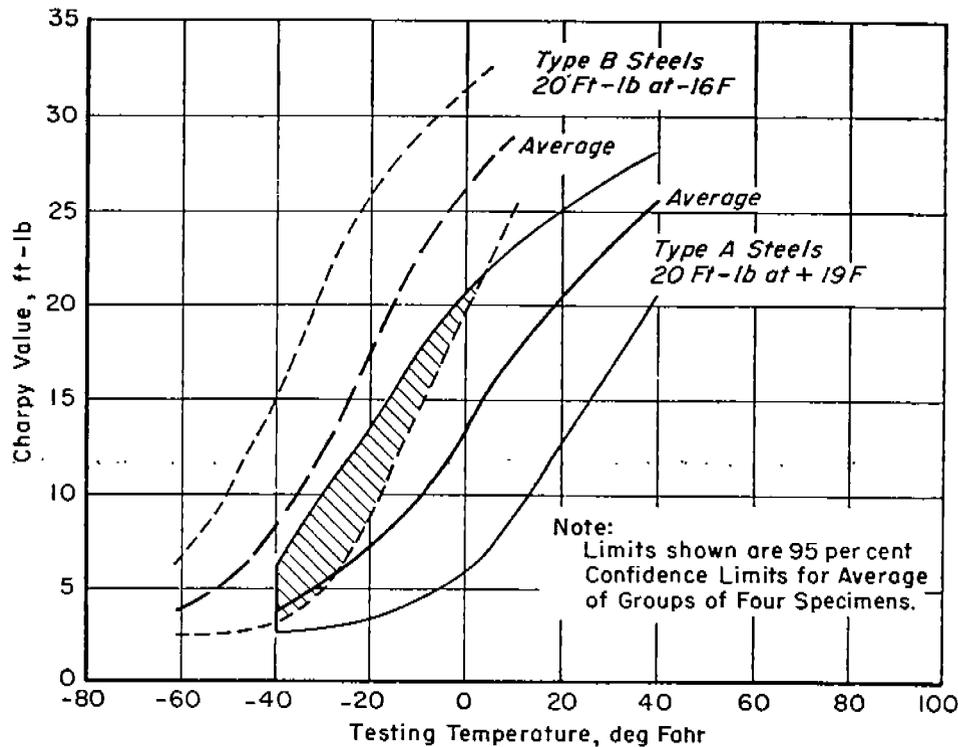
FIG. 7.—Charpy Transition Curves and Their Confidence Limits Calculated by Methods Described in the Appendix.
