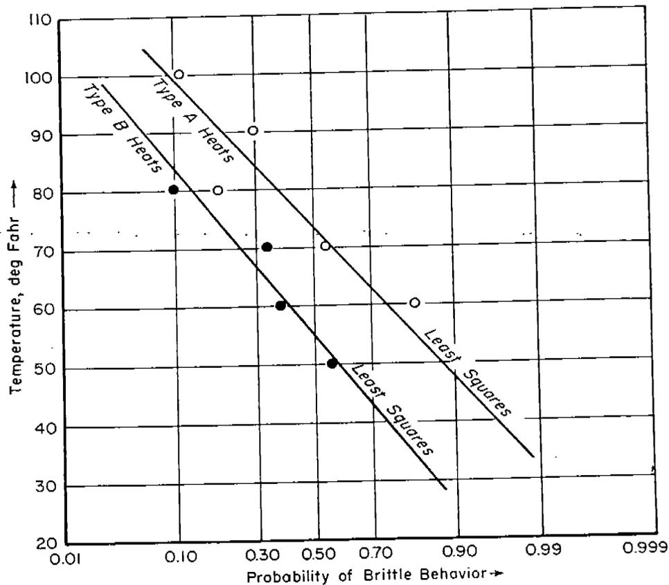
FIG. 8.—Frequencies of Brittle Tear-Test Specimens at Various Testing Temperatures.
