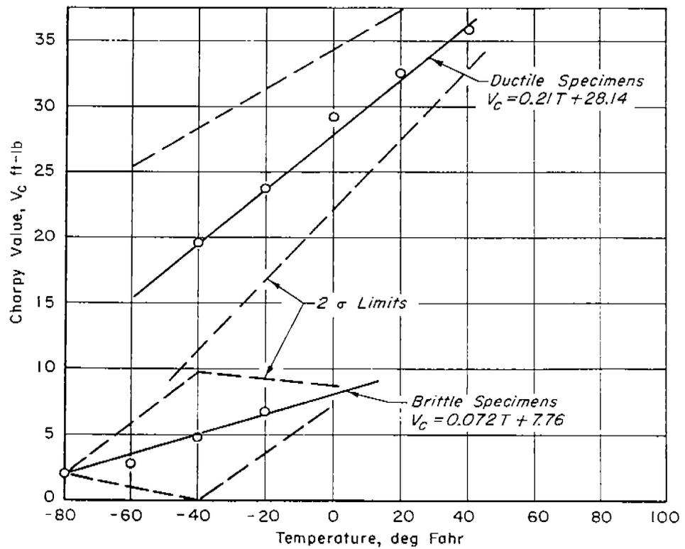
FIG. 6.—Keyhole Charpy Test Characteristics of Type B Steels.
