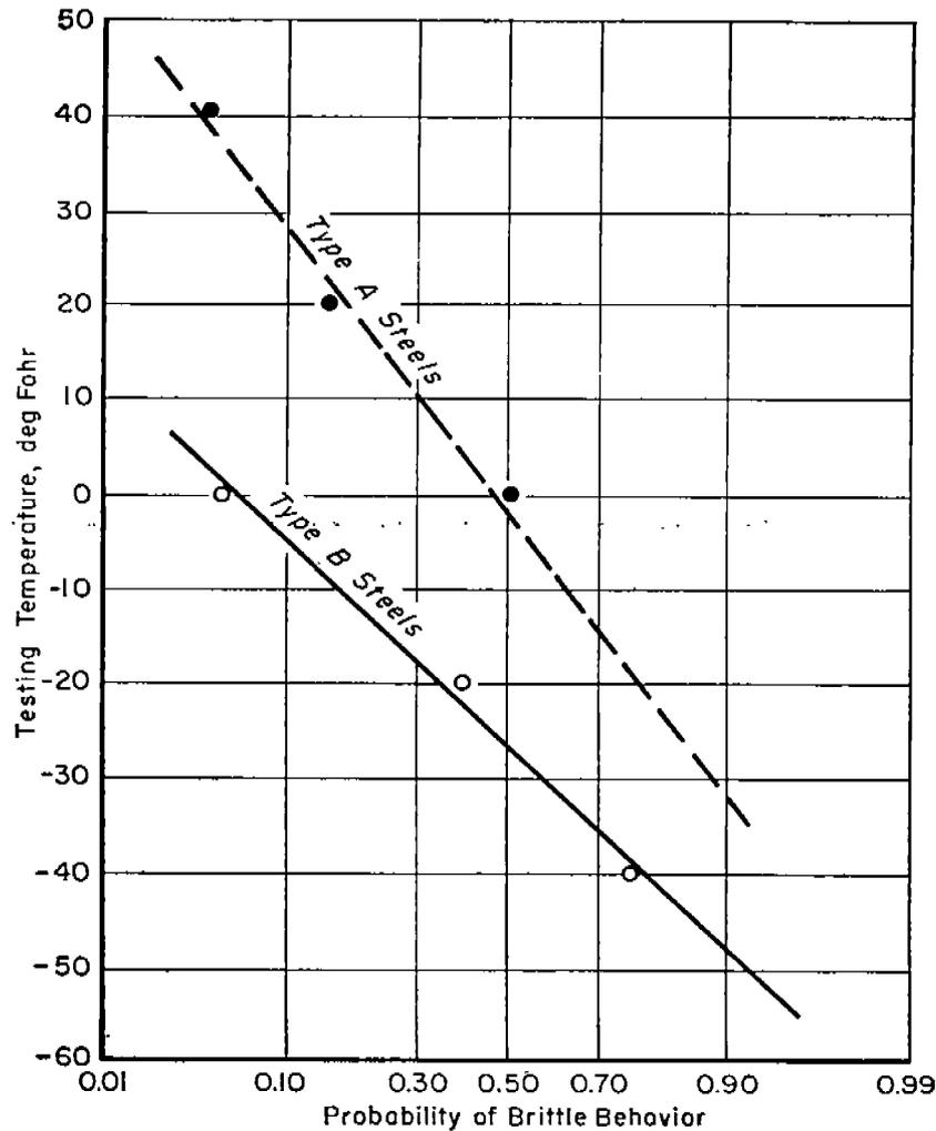
FIG. 4.—Frequencies of Brittle Charpy Specimens at Various Testing Temperatures.
