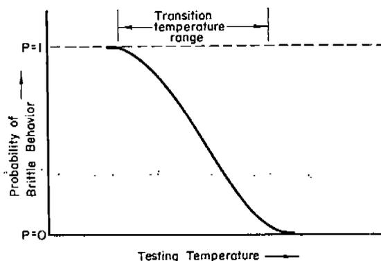
FIG. 2.—Schematic Diagram Illustrating the Probability Nature of the Transition from Ductile to Brittle Behavior in Steels.
