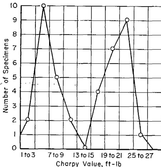
FIG. 3.—Frequency of Energy Values for a Group of Forty Specimens of Type A Steel Tested at 0 F.
