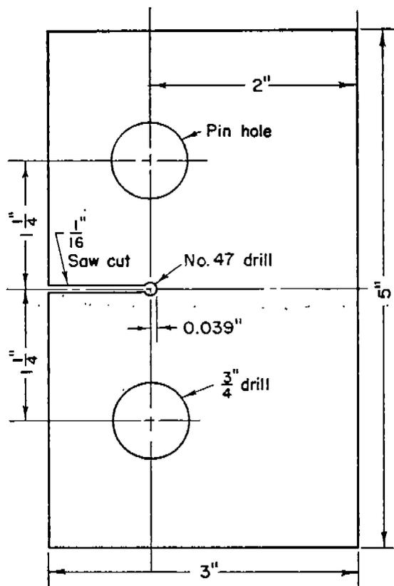
FIG. 1.—Navy Tear-Test Specimen Utilizing Full Plate Thickness.
