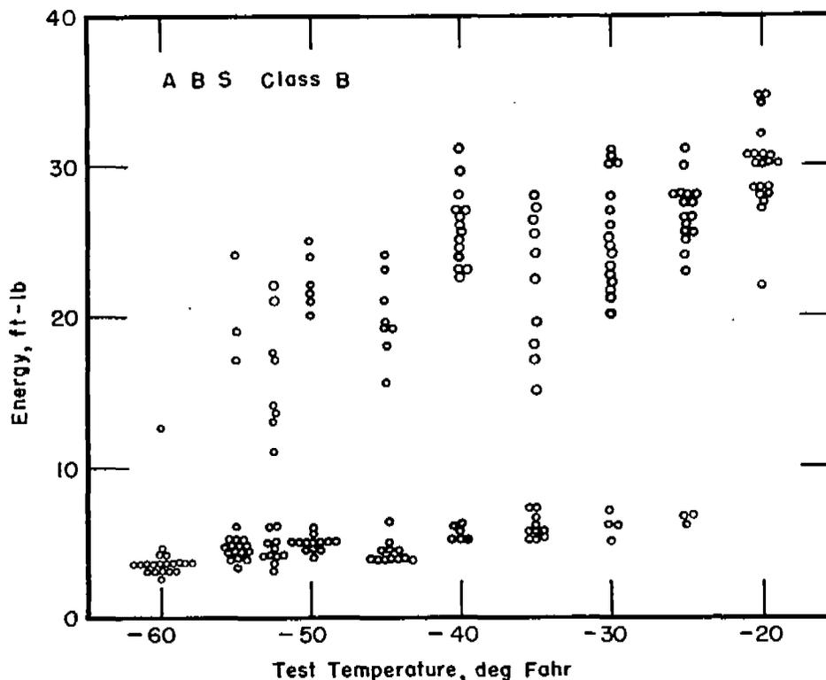
FIG. 10.—Keyhole Charpy Impact Test Results on ABS Type B Hull Steel.
