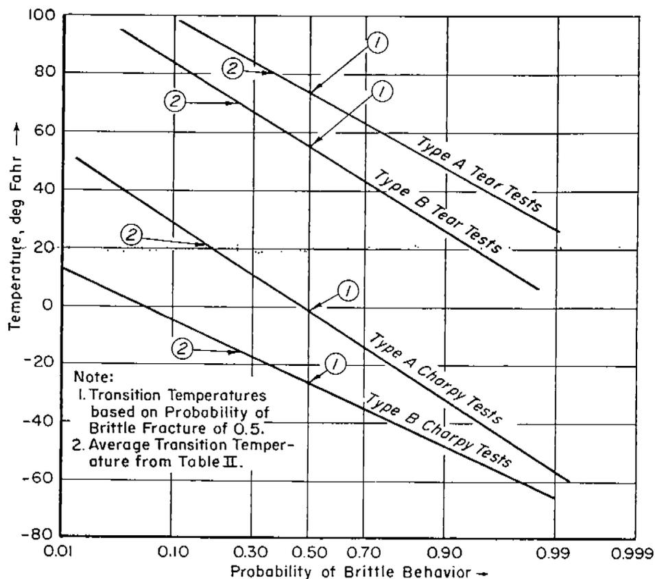
FIG. 9.—Probability of Brittle Behavior in Notched-Bar Tests at Various Temperatures.
