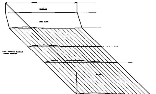
Fig. 4 Sketch of bottom primary membrane deformation in tank number 2
