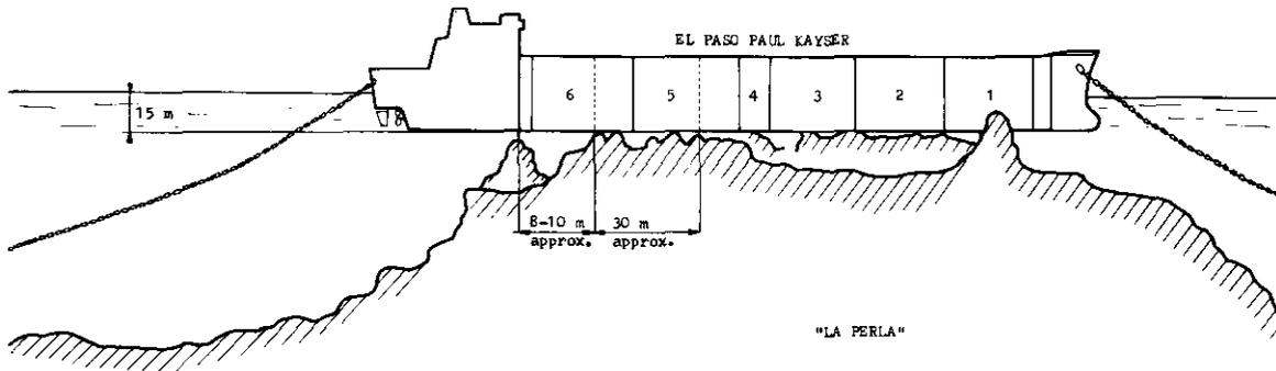
Fig. 2. View of the "Paul Kayser" ship and "La Perla" rock after the grounding
