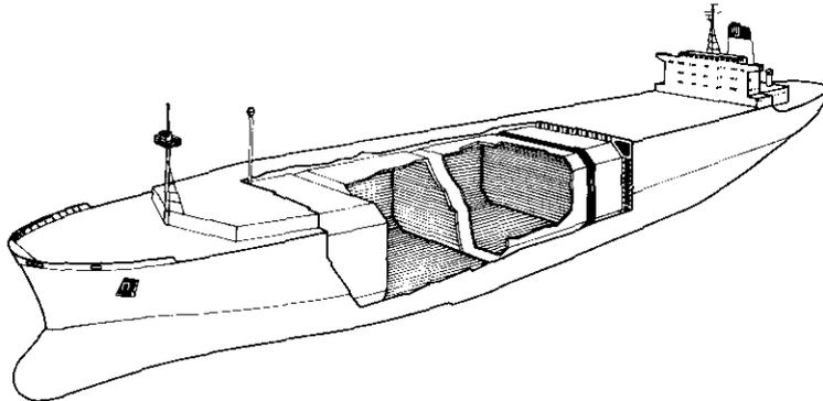
Fig. 1. General view of a membrane LNG carrier
