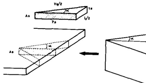
Fig. 10. Basic definition of the parameters used by the Vaughan method.
