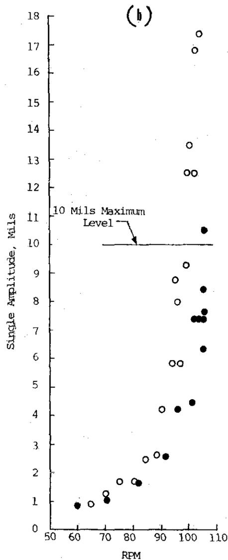
Longitudinal Vibration of Forward End of Bull Gear Shaft
