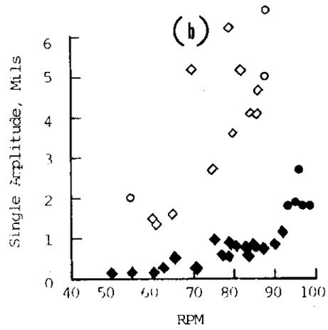
Longitudinal Vibration of High Pressure Turbine
