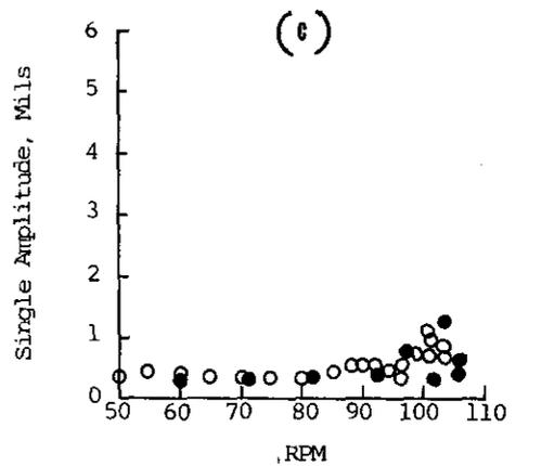
Vertical Vibration of Thrust Bearing
