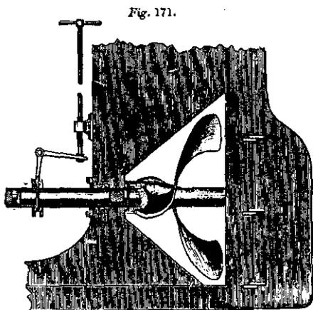
Figure A2 - Beadon's Screw Propeller
