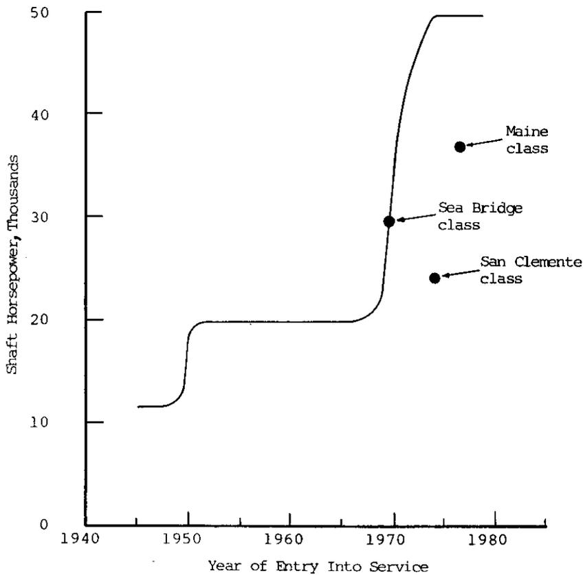
Figure 4 - Maximum Shaft Horsepower Single Screw Merchant Ships
