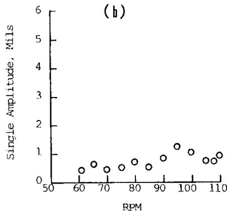
Athwartship Vibration of Elevator Casing at Cabin Deck
