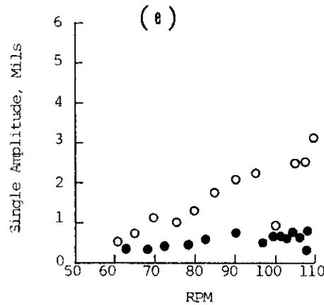
Longitudinal Vibration of Thrust Bearing
