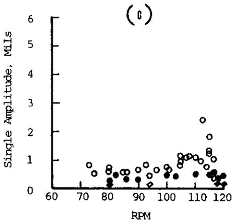
Longitudinal Vibration of Thrust Bearing
