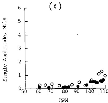
Vertical Vibration of Thrust Bearing
