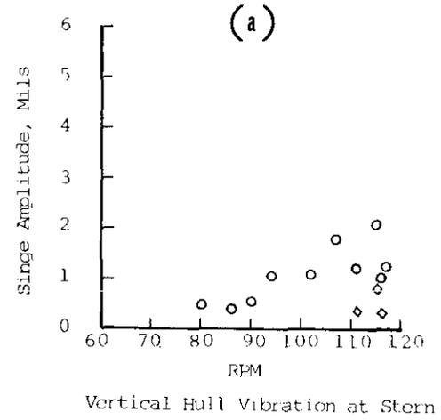
Vertical Hull Vibration at Stern
