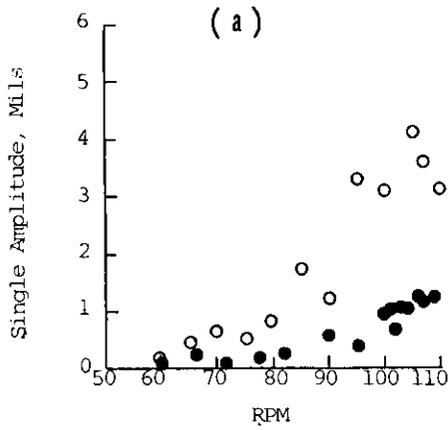
Vertical Hull Vibration at Stern
