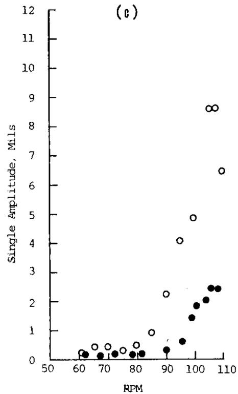
Vertical Vibration of Elevator Casing at Cabin Deck
