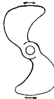
Figure A3 - Hirsch's Screw Propeller
