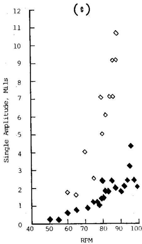
Longitudinal Vibration of Low Pressure Turbine
