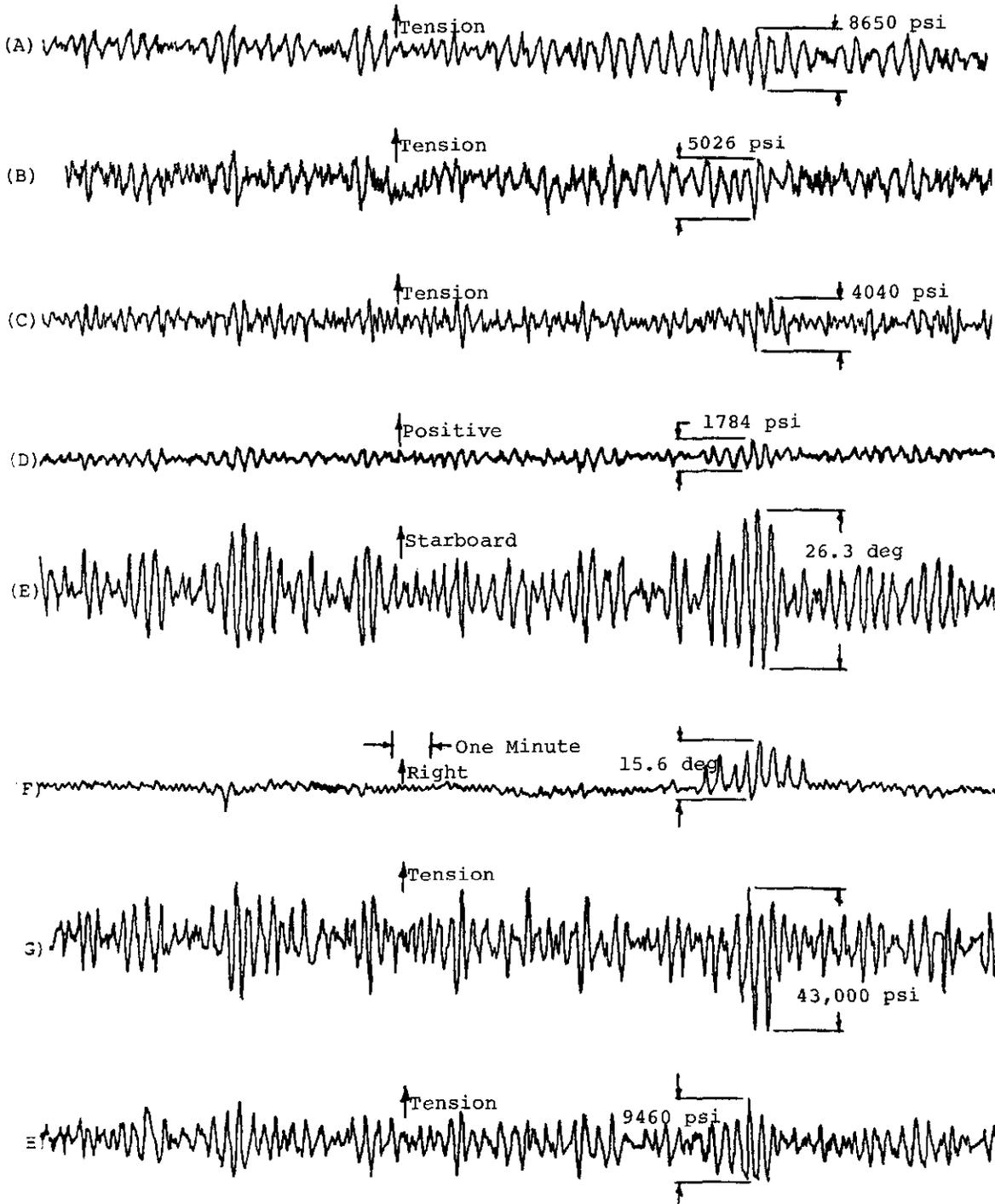
Key: (A) Midship Longitudinal Vertical Bending Stress (E) Roll Angle
