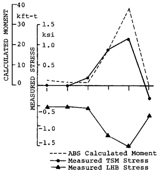
Fig. 10 Measured Torsional Shear Midships (TSM), Longitudinal Horizontal Bending (LHB) and Calculated Torsional Moment vs. Load Condition
