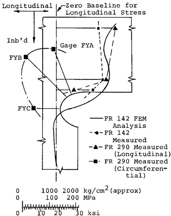
Fig. 3 A Sample Comparison Between FEM Stress Prediction and Measured Stresses for Two Hatch Corners
