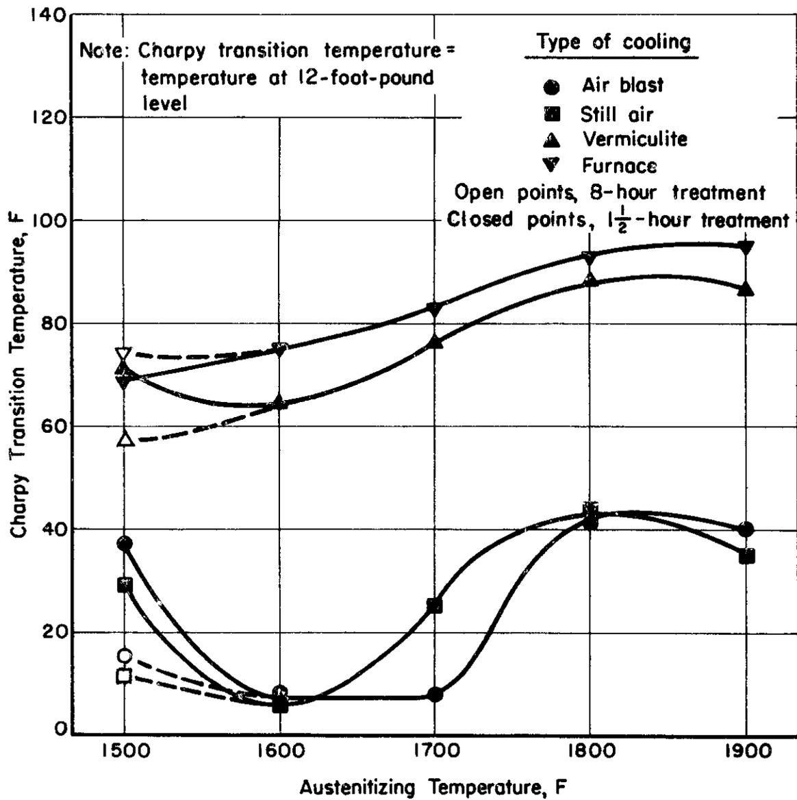
FIGURE II. EFFECT OF AUSTENITIZING TEMPERATURE AND COOLING RATE ON CHARPY TRANSITION TEMPERATURE OF STEELS COOLED BY VARIOUS METHODS
