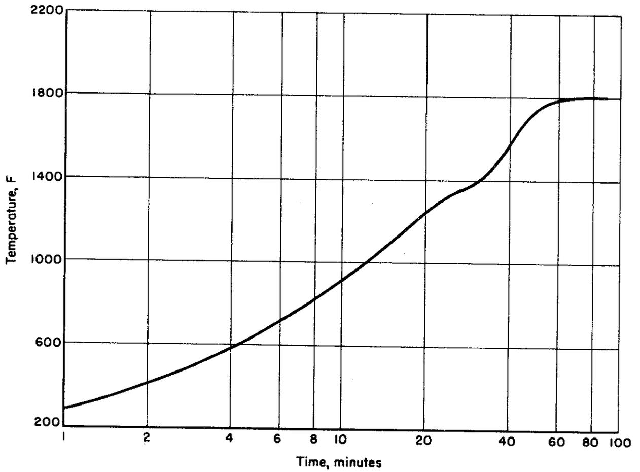
FIGURE 3. HEATING RATE FOR CENTER OF  $\frac{3}{4}$ -INCH PLATE;
