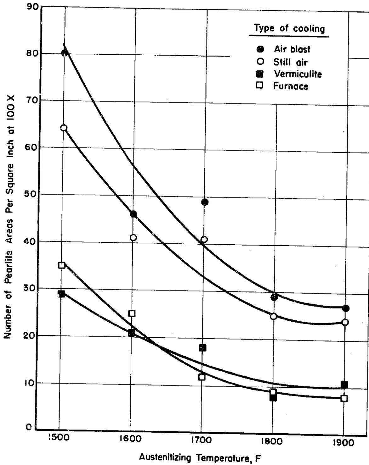
FIGURE 8. EFFECT OF AUSTENITIZING TEMPERATURE AND COOLING RATE ON DISTRIBUTION OF PEARLITIC AREAS
