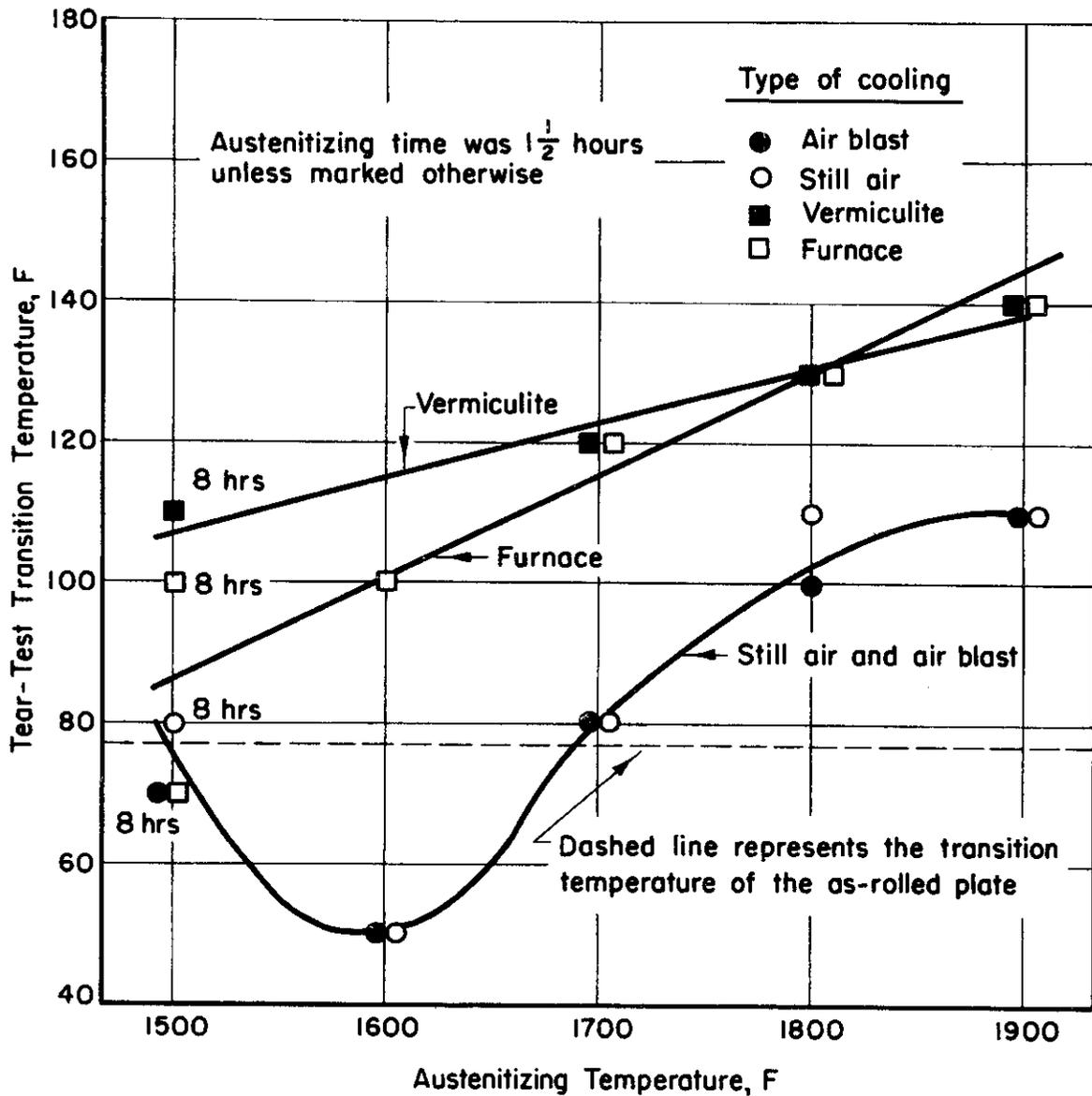
FIGURE 9. EFFECT OF AUSTENITIZING TEMPERATURE AND COOLING RATE ON TEAR TEST TRANSITION TEMPERATURE OF PROJECT STEEL "A"
