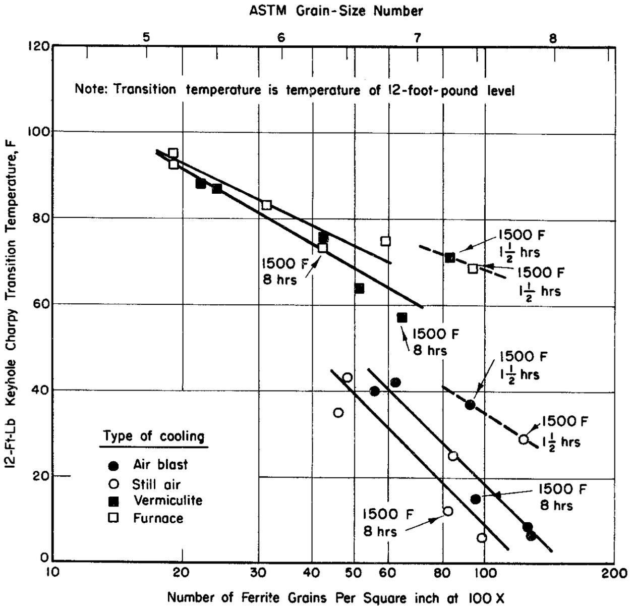
FIGURE 12. EFFECT OF FERRITE GRAIN SIZE ON KEYHOLE CHARPY TRANSITION TEMPERATURE OF PROJECT STEEL "A" COOLED AT DIFFERENT RATES. The variation in grain size was obtained by using different austenitizing temperatures and cooling rates.
