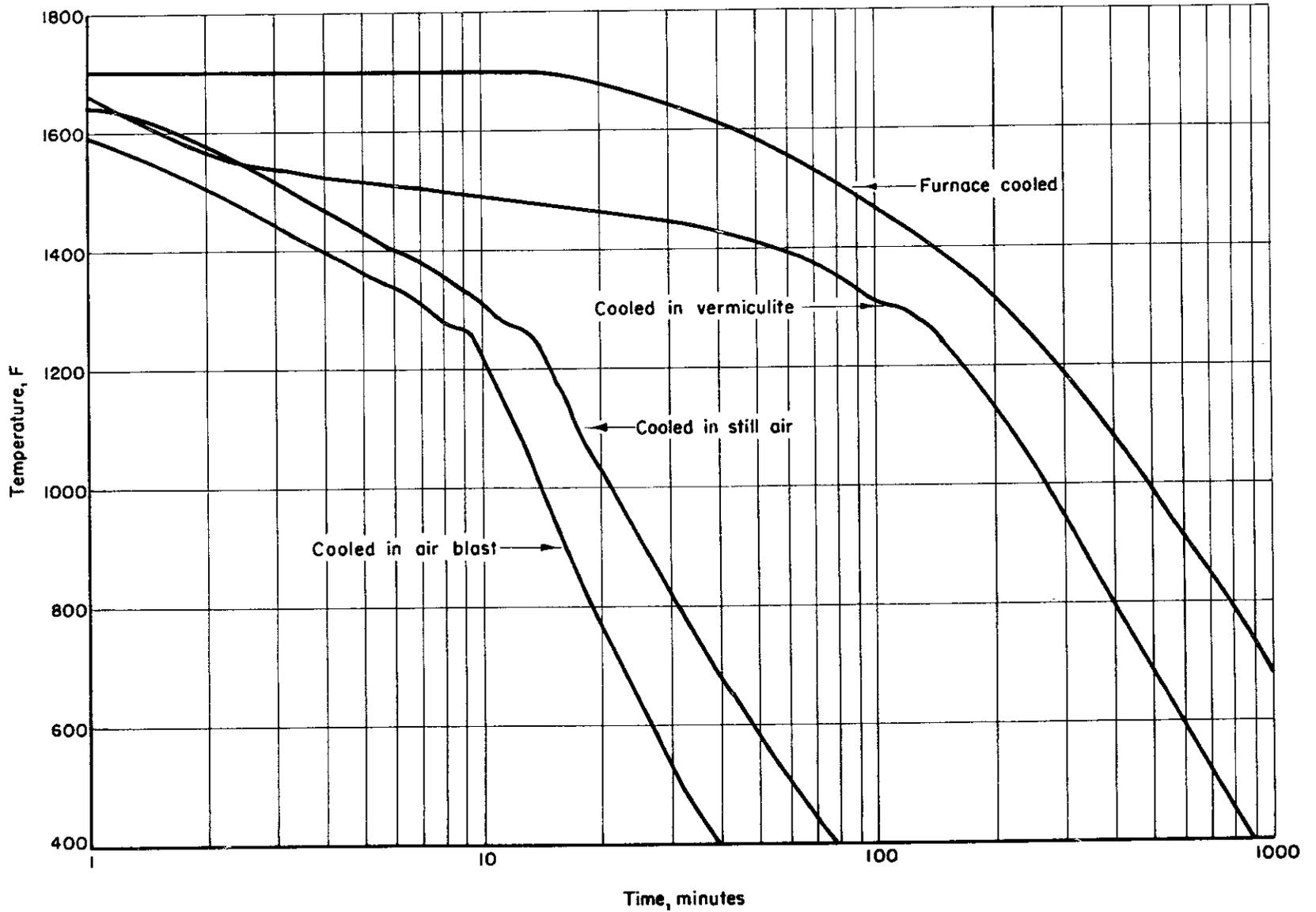
FIGURE 5. COOLING CURVES OF PLATE AUSTENITIZED AT 1700 F
