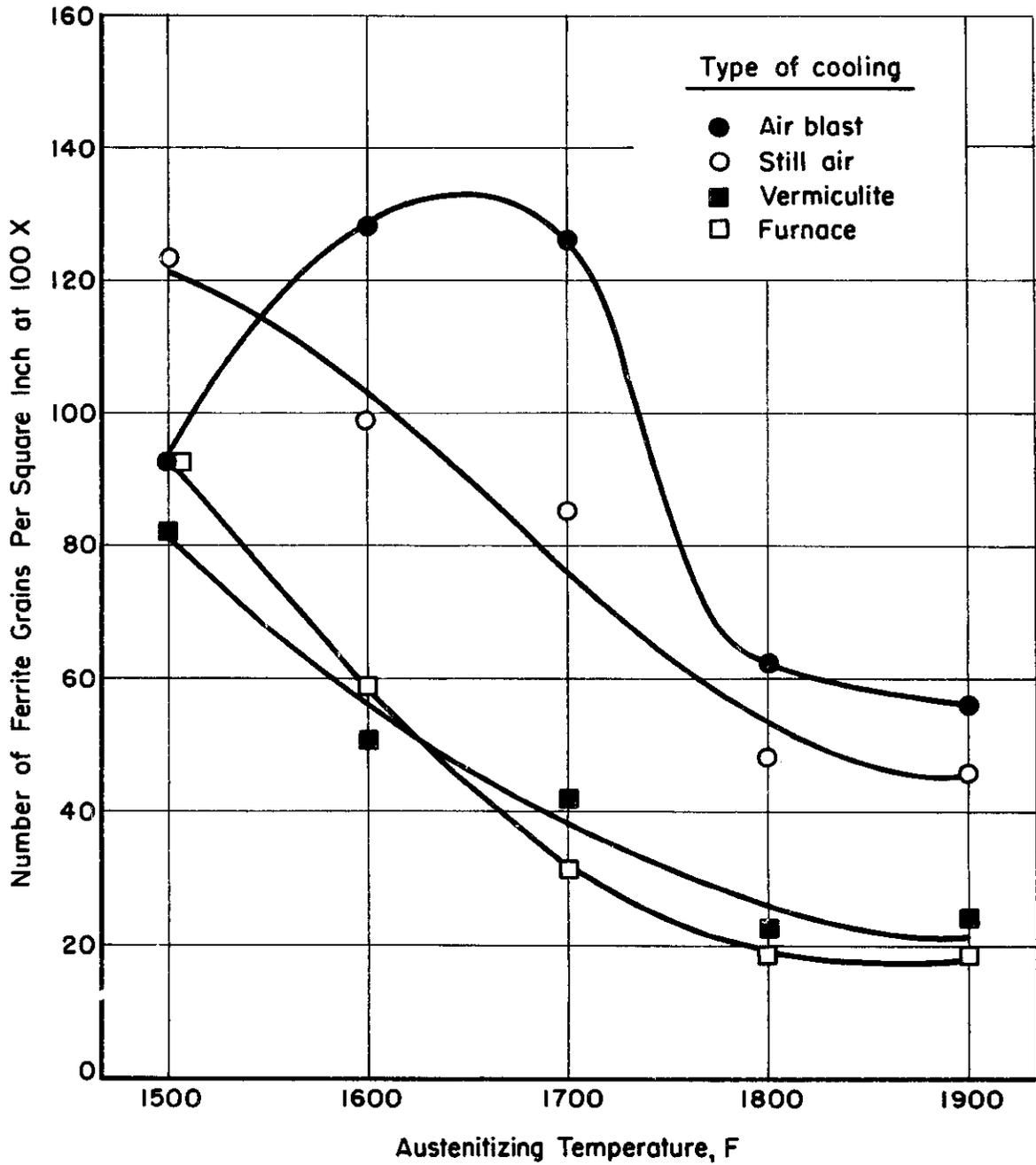
FIGURE 7. EFFECT OF AUSTENITIZING TEMPERATURE AND COOLING RATE ON FERRITE GRAIN SIZE
