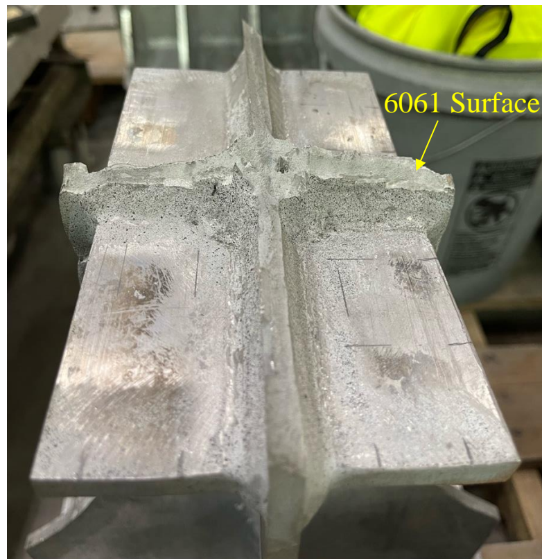
Figure 4.27 Lower failure surface of Specimen LT2 with focus are covering: (a) the AA5083 failure surface and (b) the AA8061 surface
