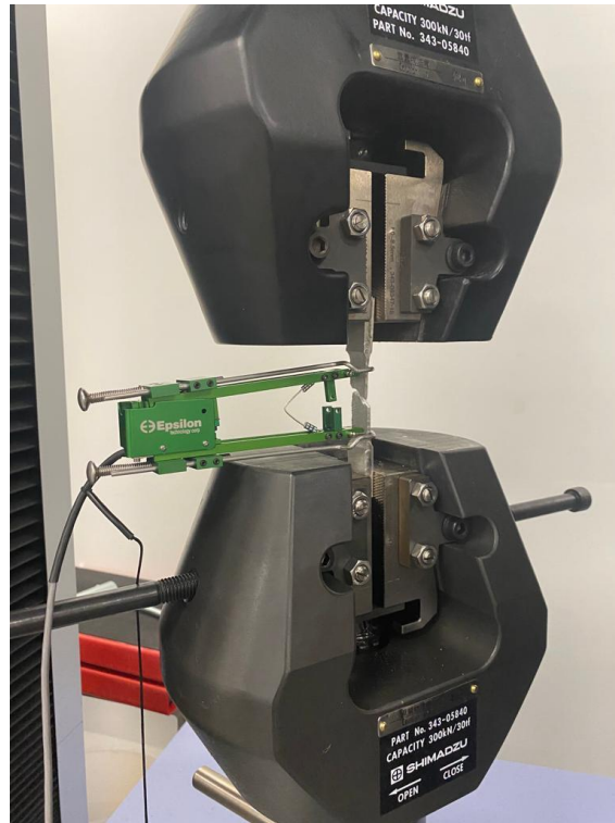
Figure 4.2: Close-up view for one of the AA5083-H116 HAZ coupons after the test was completed.
