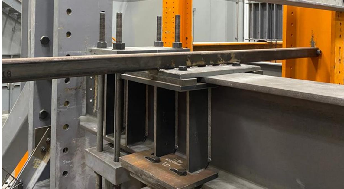
Figure 3.16: View of the lateral support system attached to the loading beam.
