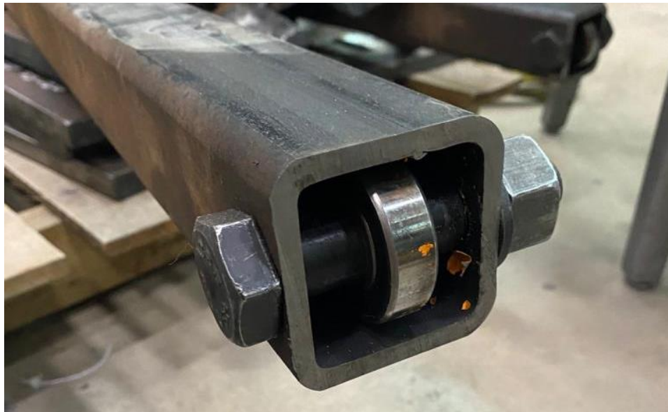
Figure 3.17: Closeup view on the roller bearing that accommodates the in-plane movement.
