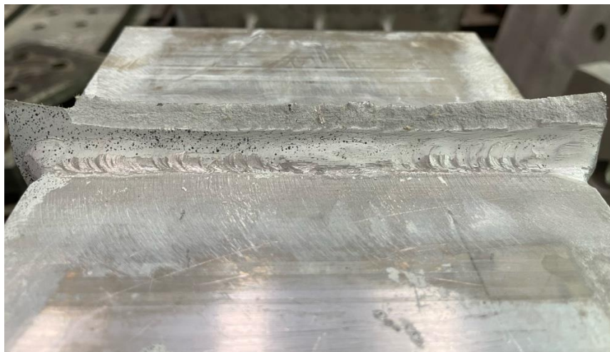
Figure 4.15: Failure of the T specimens: (a) general location of failure, (b) upper fracture surface of Specimen T2, and (c) lower fracture surface of T2.
