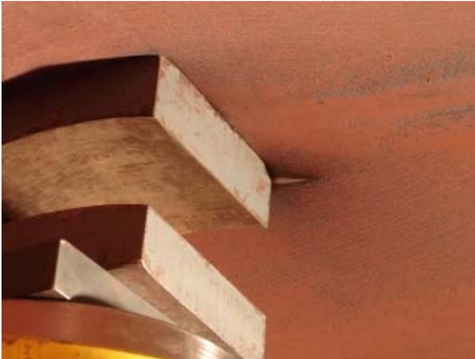
**Figure 29: LG1\_2: ram after test (note imbedded platen and small tear)**
