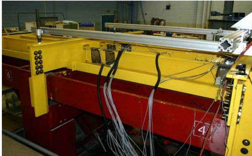
**Figure 15: Large Grillage Test Arrangement**
