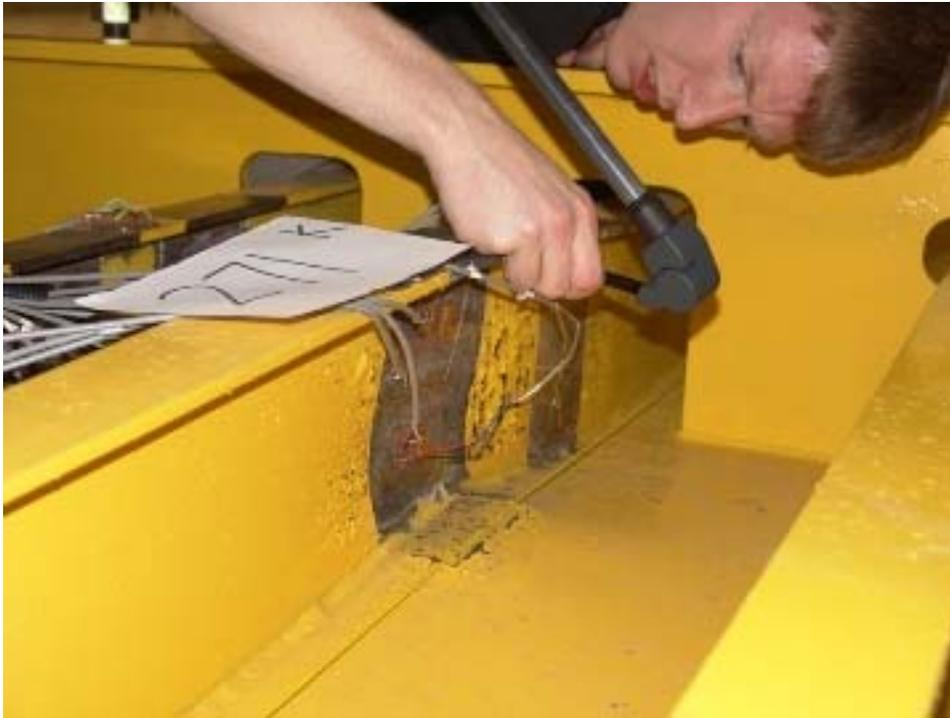
**Figure 21: LG1\_1 test: MicroScribe measurements at 271kips (1205kN)**
