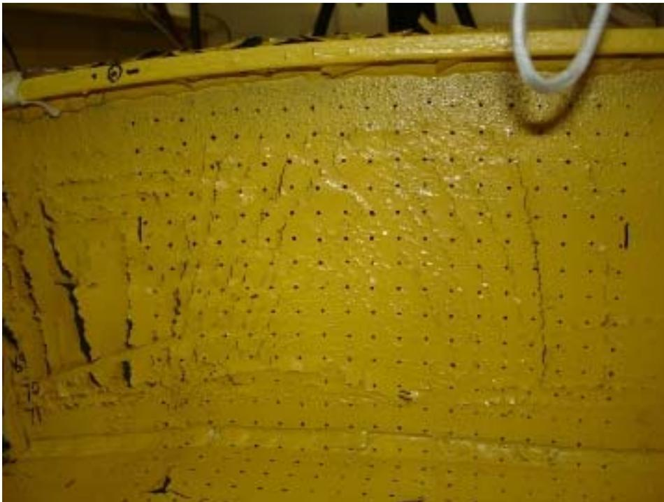
**Figure 30: LG1\_2 test, web distortion**
