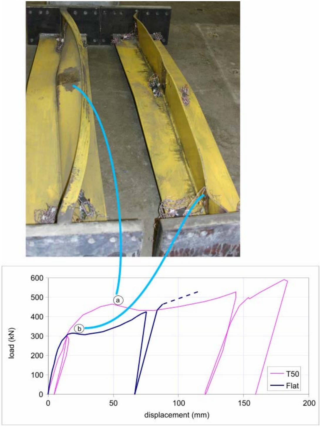
Figure 11: Comparison of T50c and Fc tests.
