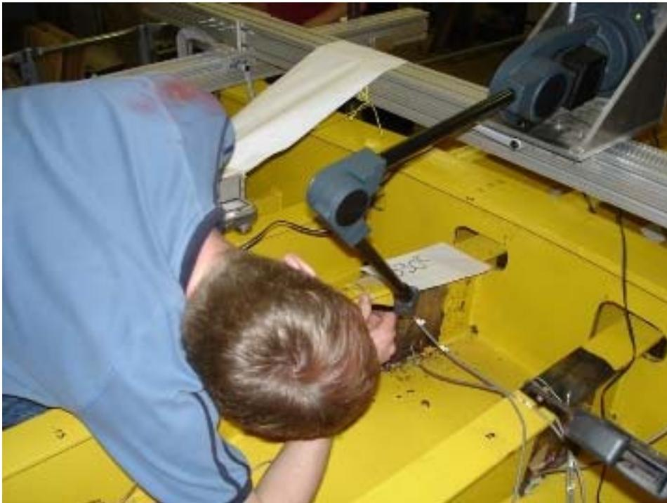
**Figure 26: LG1\_2 test: MicroScribe measurements at 330 kips (1468 kN)**
