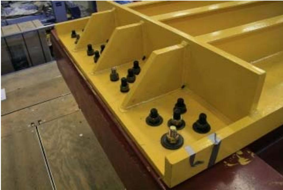
**Figure 35: Large Grillage end clamp arrangement.**
