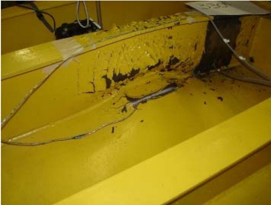
**Figure 27: LG1\_2 test: web deformation at 330kips (1468 kN)**
