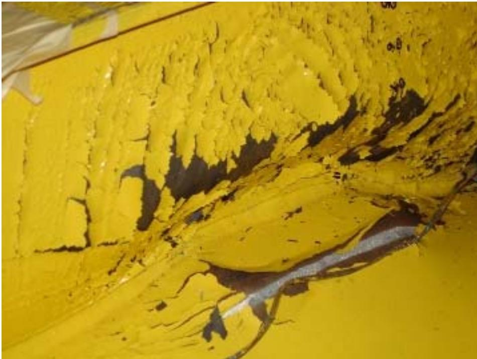
**Figure 28: LG1\_2 test: close-up of web deformation at 330kips (1468 kN)**
