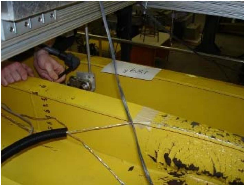
**Figure 31: LG1\_3 at 198 kips (note: load is at center, with prior shear damage at end)**
