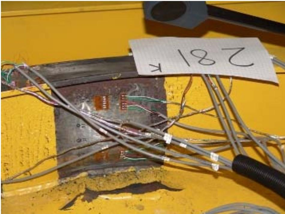
**Figure 22: LG1\_1 test: web deformation at 281kips (1250 kN)**
