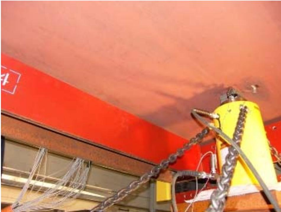
**Figure 25: LG1\_1 view of ram after test (note imprint)**
