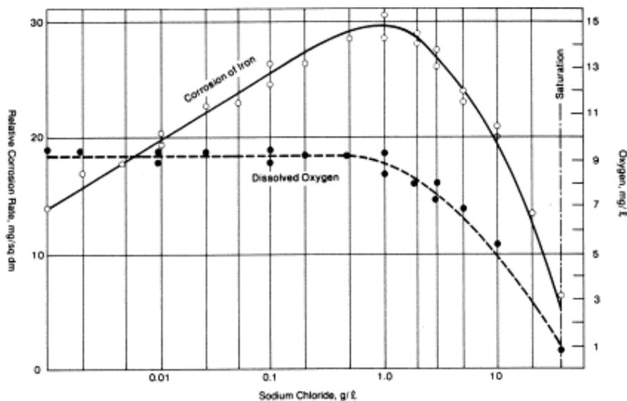
**Figure 2.5: Variation in Corrosion of Iron as a Function of Salinity and Dissolved Oxygen**
