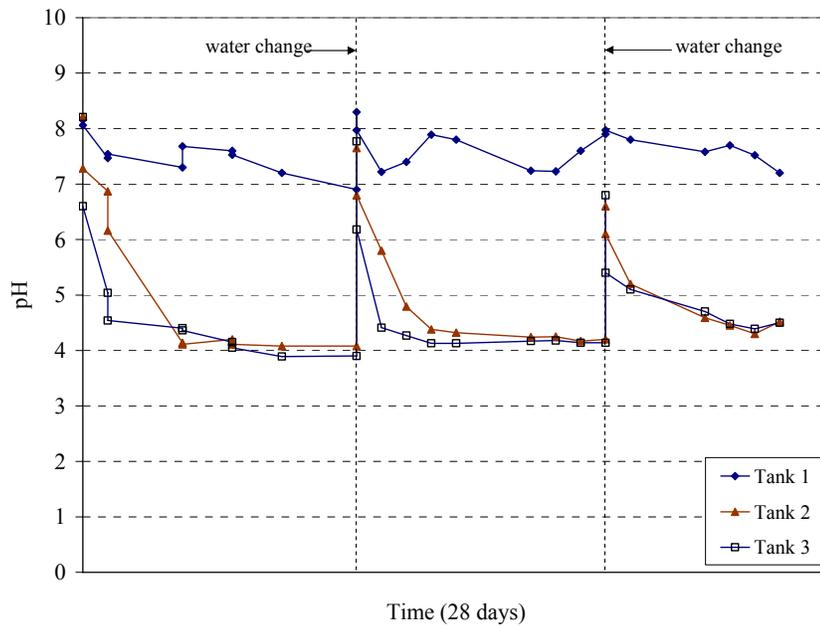
**Figure 4.25(a): Bulk Solution pH Measurements Carried out During 15 ppt Salt Water Tests Treated with PERACLEAN® OCEAN**
