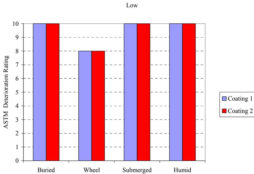
Figure F10: Tank 5 (35 ppt) - Deterioration Rating vs. Location (SeaKleen™)
