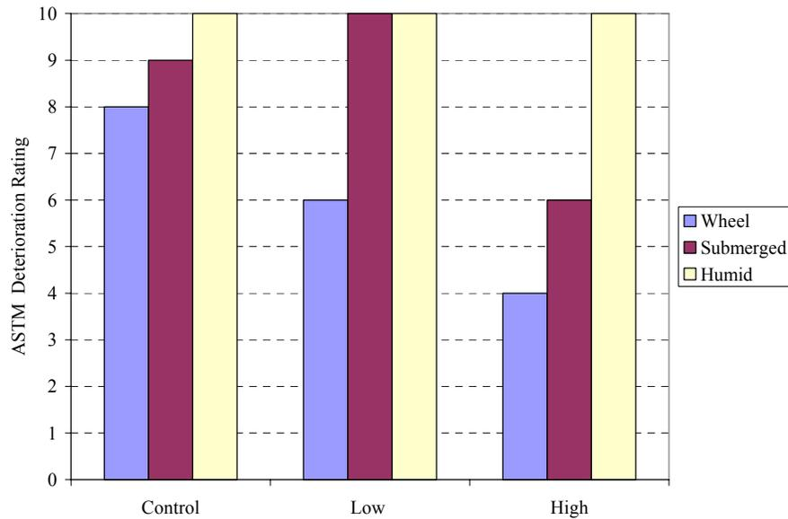
Figure H4: Coating 1(Fresh Water) - Deterioration Rating vs. Concentration (PERACLEAN® OCEAN)
