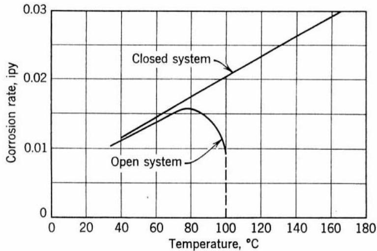
**Figure 2.4: Effect of Temperature on Corrosion of Iron in Water Containing Dissolved Oxygen**
