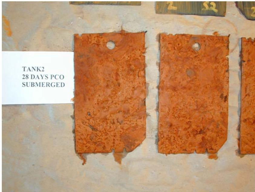
Figure G8: Corroded Plates Exposed to Submerged Environment in 15 ppt Salt Water, Tank 2, (Low Dosage, PERACLEAN® OCEAN)
