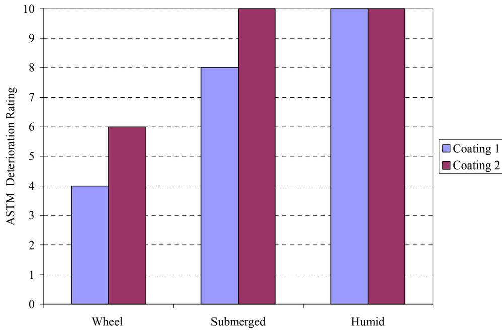
Figure F2: Tank 2 (Fresh Water) - Deterioration Rating vs. Location (SeaKleen™)
