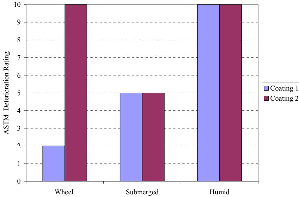
Figure F3: Tank 3 (Fresh Water) - Deterioration Rating vs. Location (SeaKleen™)
