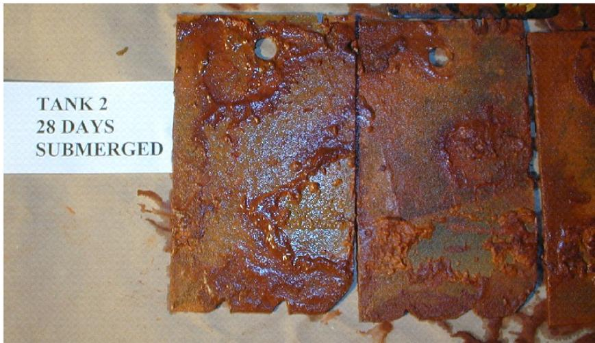
Figure E8: Corroded Plates Exposed to Submerged Environment in 15 ppt Salt Water, Tank 2, (Low Dosage, SeaKleen™)
