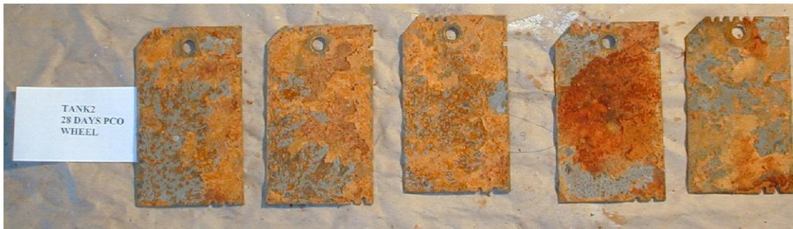
Figure G2: Corroded Plates Exposed to Splash Zone Environment in 15 ppt Salt Water, Tank 2, (Low Dosage, PERACLEAN® OCEAN)
