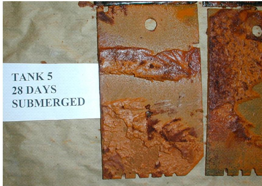
Figure E11: Corroded Plates Exposed to Submerged Environment in 35 ppt Salt Water, Tank 5, (Low Dosage, SeaKleen™)
