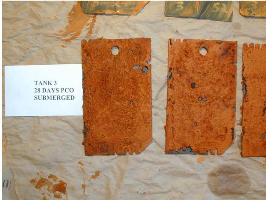
Figure G9: Corroded Plates Exposed to Submerged Environment in 15 ppt Salt Water, Tank 3, (High Dosage, PERACLEAN® OCEAN)
