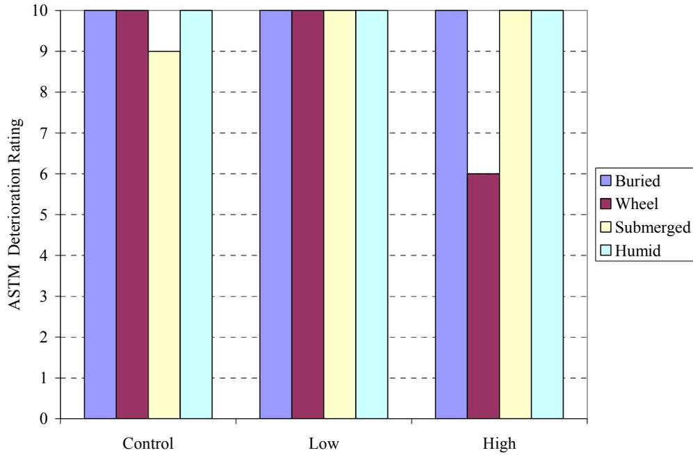
Figure H13: Coating 2 (15 ppt) - Deterioration Rating vs. Concentration (PERACLEAN® OCEAN)
