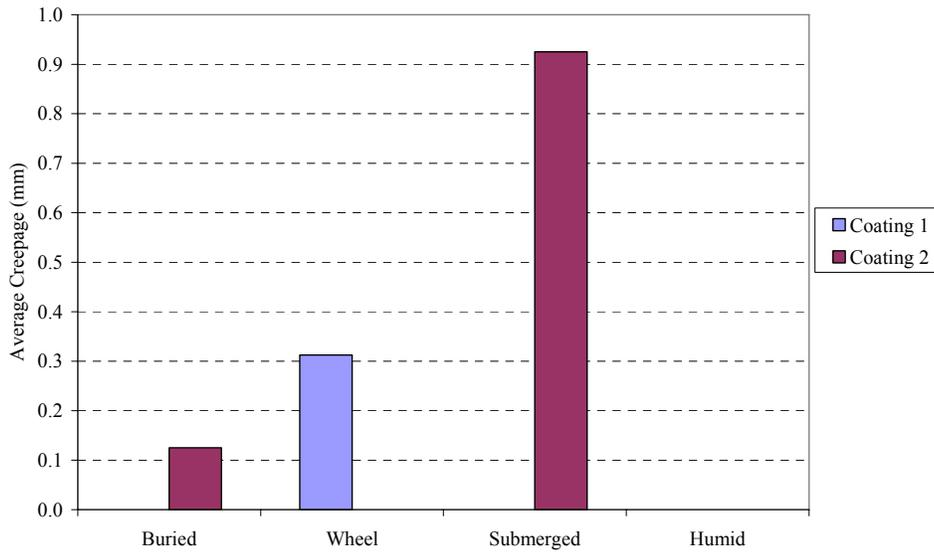
**Figure 4.17(c): Average Creepage vs. Location in Tank, 15 ppt Salt Water**
