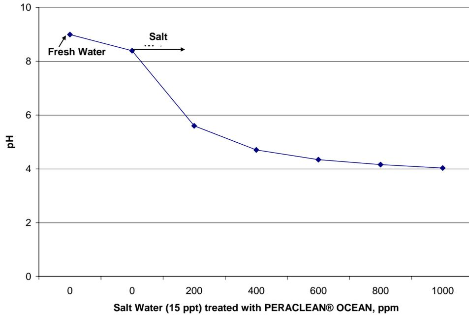
**Figure 4.19(b): Effect of PERACLEAN® OCEAN Concentration on pH of Salt Water (15 ppt Salinity)**
