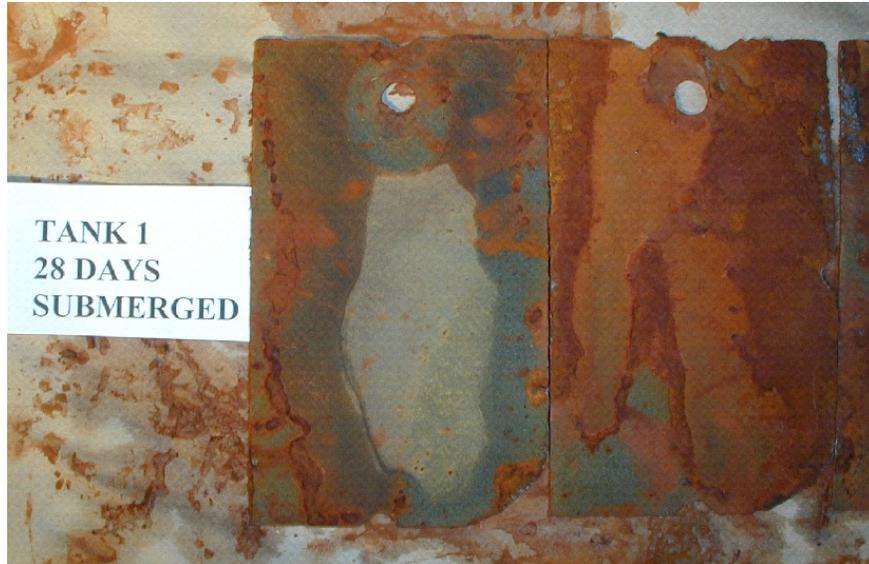
Figure E7: Corroded Plates Exposed to Submerged Environment in 15 ppt Salt Water, Tank 1, (Control Tank)
