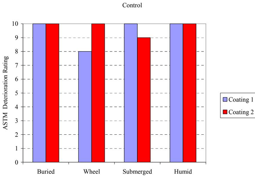
Figure H6: Tank 1 (15 ppt) - Deterioration Rating vs. Location (PERACLEAN® OCEAN)
