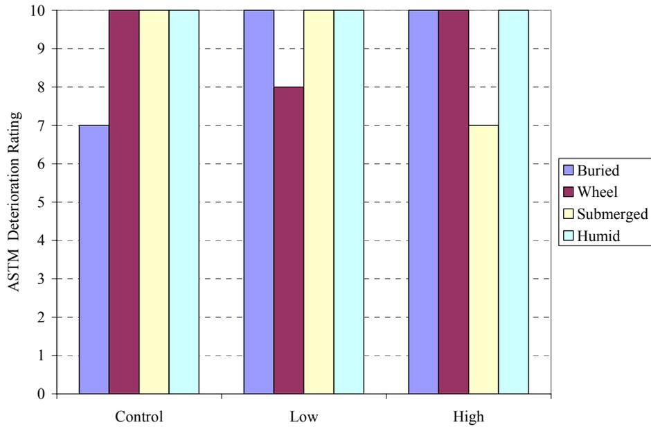
Figure F15: Coating 2 (35 ppt) - Deterioration Rating vs. Concentration (SeaKleen™)
