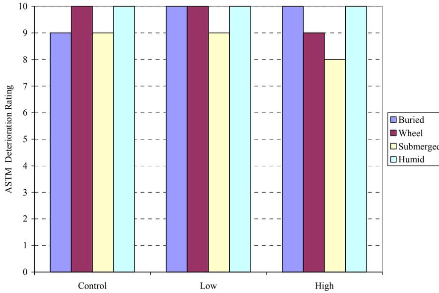
**Figure 4.17(b): ASTM Score vs. Exposure (Average across all Coatings), 15 ppt Salt Water**
