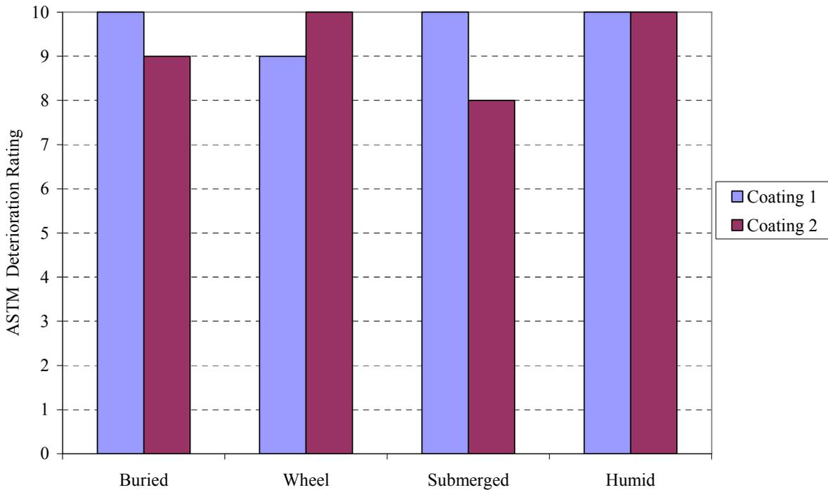
**Figure 4.17(a): ASTM Score vs. Location in Tanks, 15 ppt Salt Water (Average across Control and SeaKleen™ Treated Tanks)**
