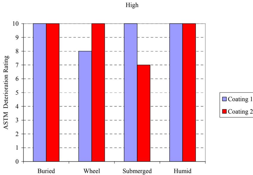
Figure F8: Tank 3 (15 ppt) - Deterioration Rating vs. Location (SeaKleen™)
