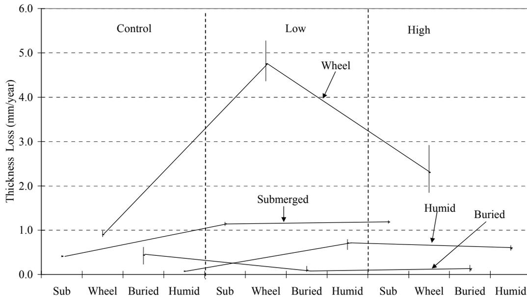
**Figure 4.30: Loss of Thickness in Corrosion Tank, 35 ppt Salt Water Tests**
