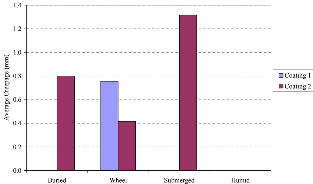
**Figure 4.18(c): Average Creepage vs. Location in Tank, 35 ppt Salt Water**
