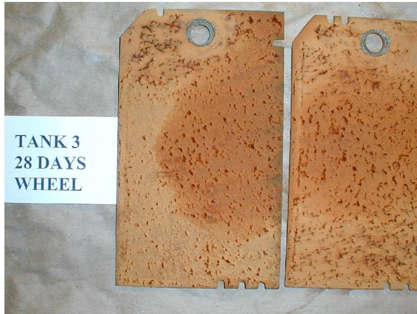
Figure E3: Corroded Plates Exposed to Splash Zone Environment in 15 ppt Salt Water, Tank 3, (High Dosage, SeaKleen™)
