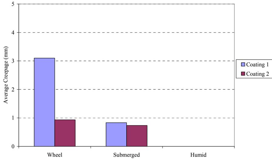
**Figure 4.32(c): Average Creepage vs. Location in Tank, Fresh Water**
