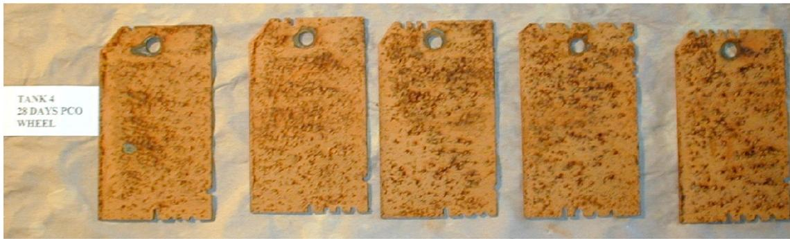
Figure G4: Corroded Plates Exposed to Splash Zone Environment in 35 ppt Salt Water, Tank 4, (Control Tank)
