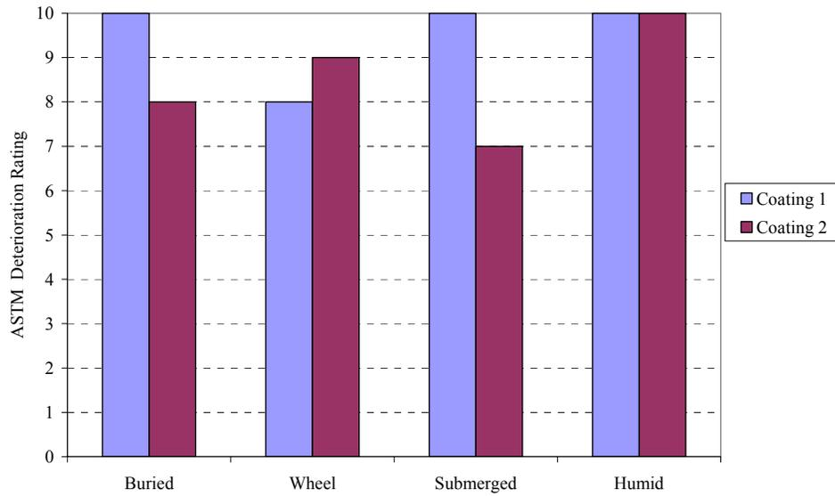
**Figure 4.18(a): ASTM Score vs. Location in Tanks, 35 ppt Salt Water (Average across Control and SeaKleen™ Treated Tanks)**
