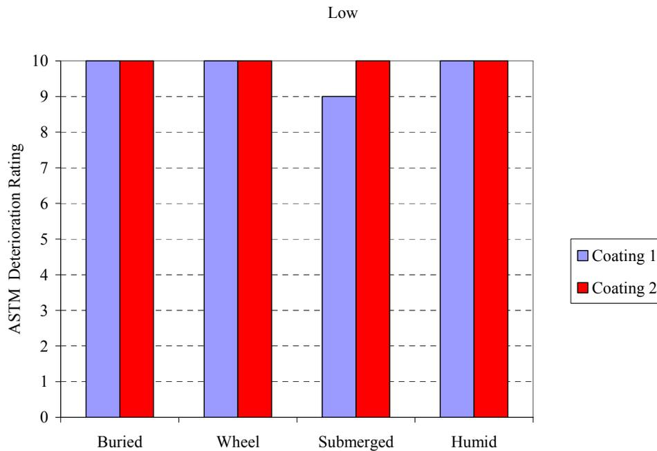
Figure H10: Tank 5 (35 ppt) - Deterioration Rating vs. Location (PERACLEAN® OCEAN)
