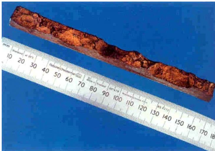
**Figure 2.7: Cross-section of the Hull Plate, Showing the Reduction in Normal Thickness (12mm) [5]**
