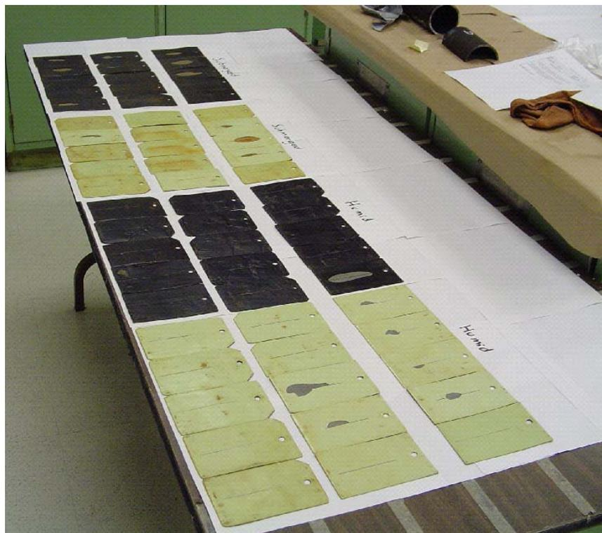
**Figure 4.7(a): Post Experiment Cleaned Coated Steel Plates**
