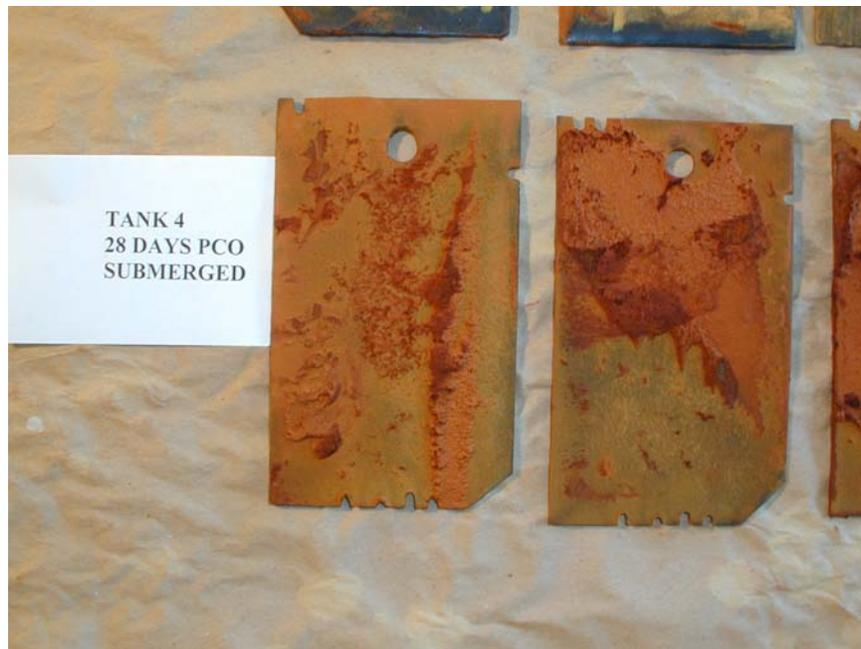
Figure G10: Corroded Plates Exposed to Submerged Environment in 35 ppt Salt Water, Tank 4, (Control Tank)
