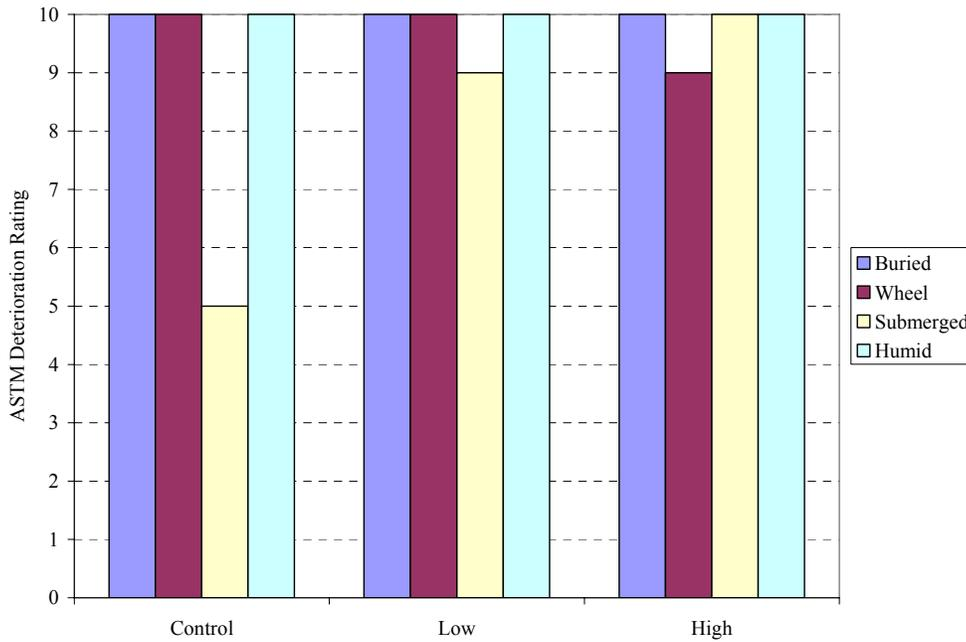
**Figure 4.34(b): ASTM Score vs. Exposure (Average across all Coatings), 35 ppt Salt Water**
