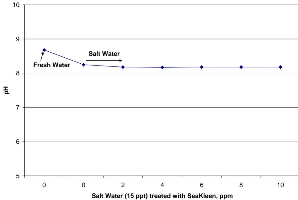
**Figure 4.8(b): Effect of SeaKleen™ Concentration on pH of Salt Water (15ppt salinity)**
