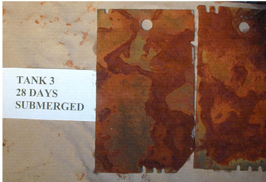
Figure E9: Corroded Plates Exposed to Submerged Environment in 15 ppt Salt Water, Tank 3, (High Dosage, SeaKleen™)
