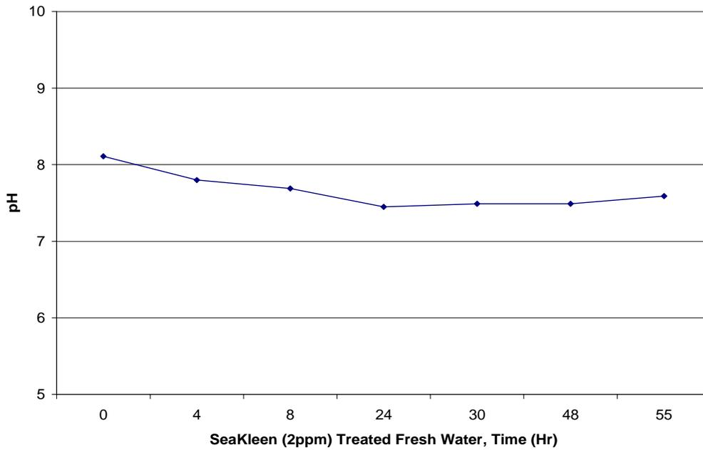
**Figure 4.9(a): pH vs. Time for SeaKleen™ (2ppm) Treated Fresh Water**
