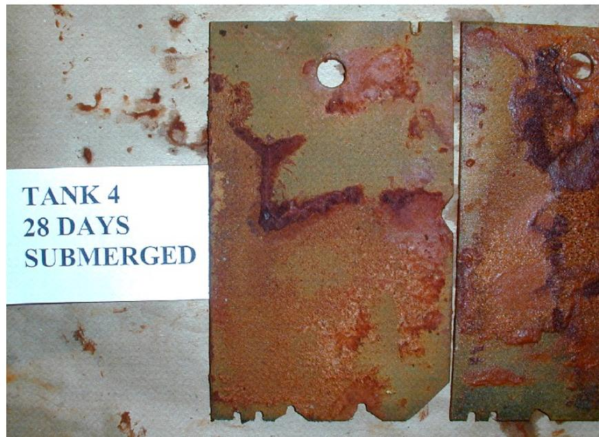
Figure E10: Corroded Plates Exposed to Submerged Environment in 35 ppt Salt Water, Tank 4, (Control Tank)
