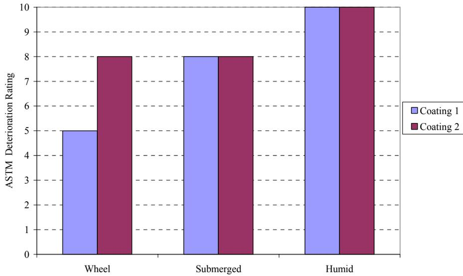
**Figure 4.32(a): ASTM Score vs. Location in Tanks, Fresh Water (Average across Control and PERACLEAN® OCEAN Treated Tanks)**
