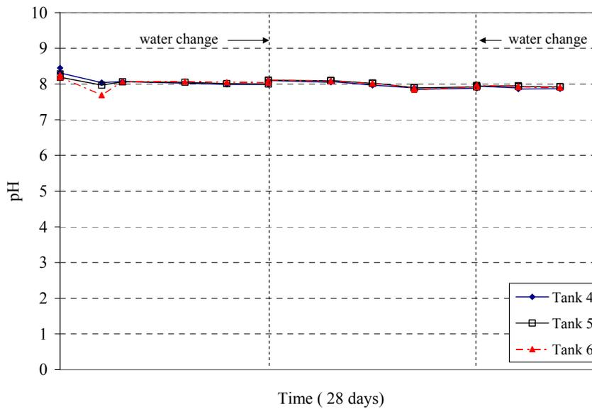
**Figure 4.11(b): Bulk Solution pH Measurements for Tanks 4, 5 and 6 for the Duration of the Salt Water Corrosion Test**
