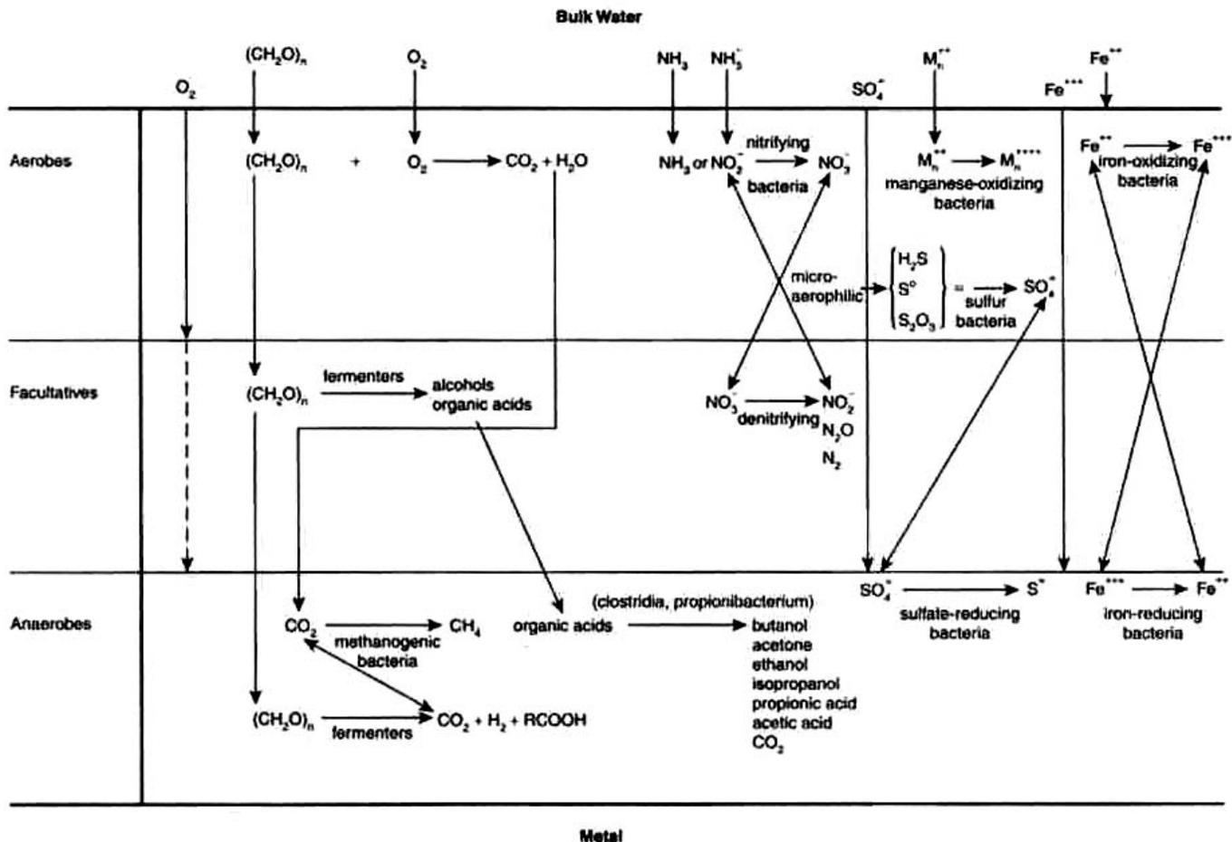
Figure 2.6: Conceptual Model of Stratified Biofilm [1]
