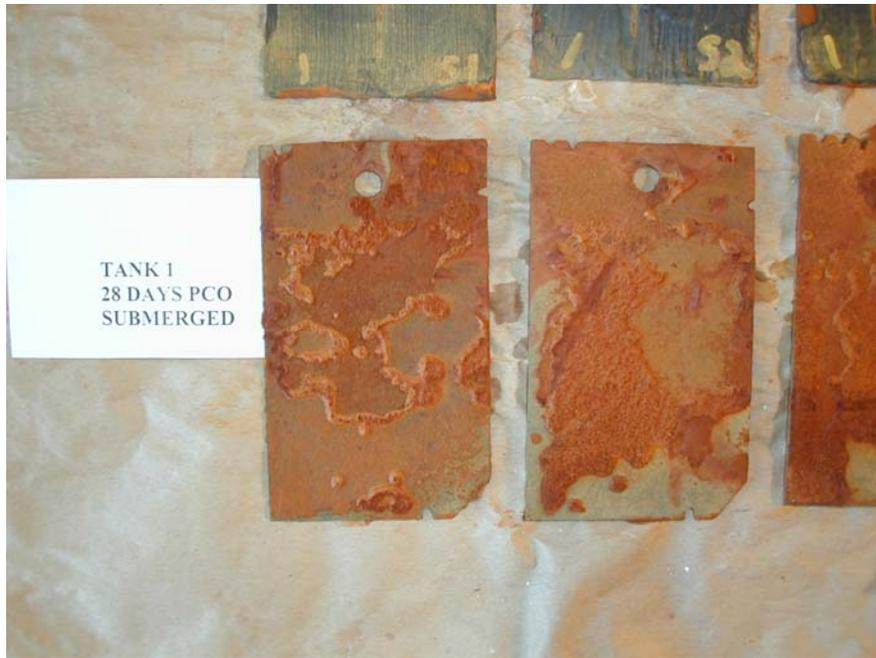
Figure G7: Corroded Plates Exposed to Submerged Environment in 15 ppt Salt Water, Tank 1, (Control Tank)
