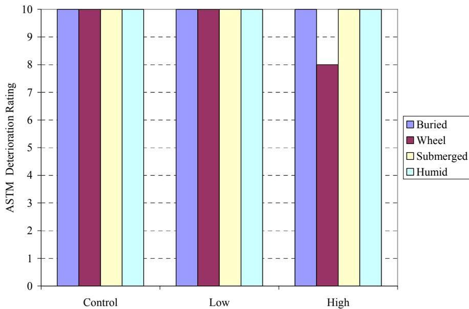
Figure F12: Coating 1 (15 ppt) - Deterioration Rating vs. Concentration (SeaKleen™)
