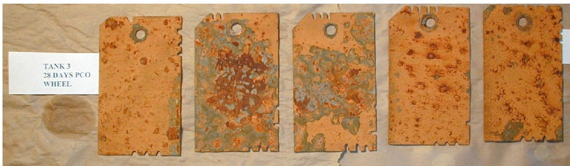
Figure G3: Corroded Plates Exposed to Splash Zone Environment in 15 ppt Salt Water, Tank 3, (High Dosage, PERACLEAN® OCEAN)
