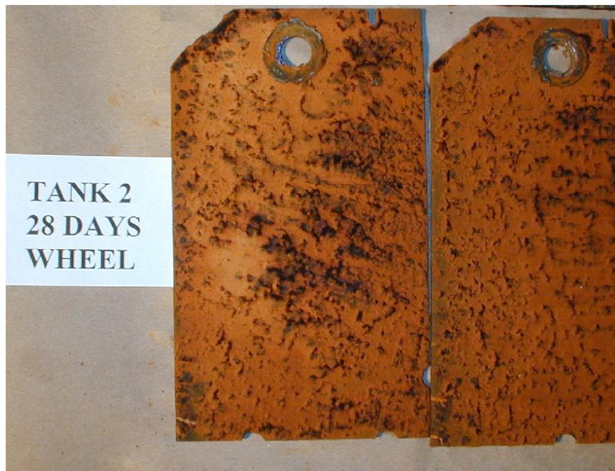
Figure E2: Corroded Plates Exposed to Splash Zone Environment in 15 ppt Salt Water, Tank 2, (Low Dosage,SeaKleen™)
