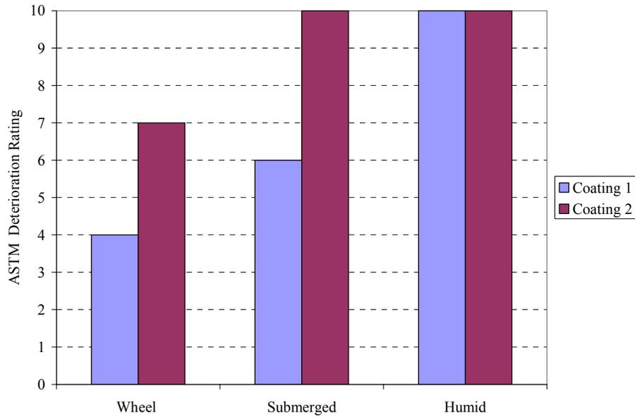
Figure H3: Tank 3 (Fresh Water) - Deterioration Rating vs. Location (PERACLEAN® OCEAN)
