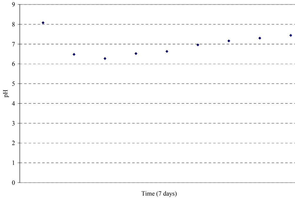
**Figure 4.26: Bulk Solution pH vs. Time for Single dose of PERACLEAN® OCEAN (150 ppm) Treated Salt Water (35 ppt Salinity)**
