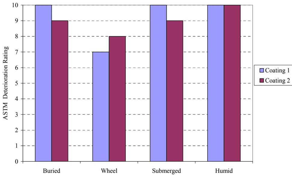
**Figure 4.33(a): ASTM Score vs. Location in Tanks, 15 ppt Salt Water (Average across Control and PERACLEAN® OCEAN Treated Tanks)**
