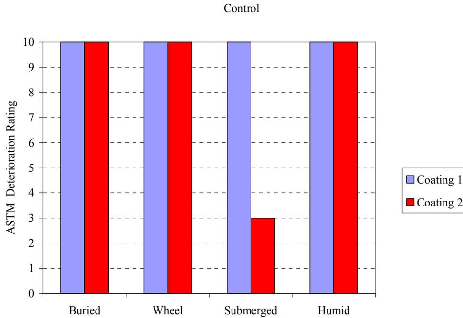
Figure H9: Tank 4 (35 ppt) - Deterioration Rating vs. Location (PERACLEAN® OCEAN)
