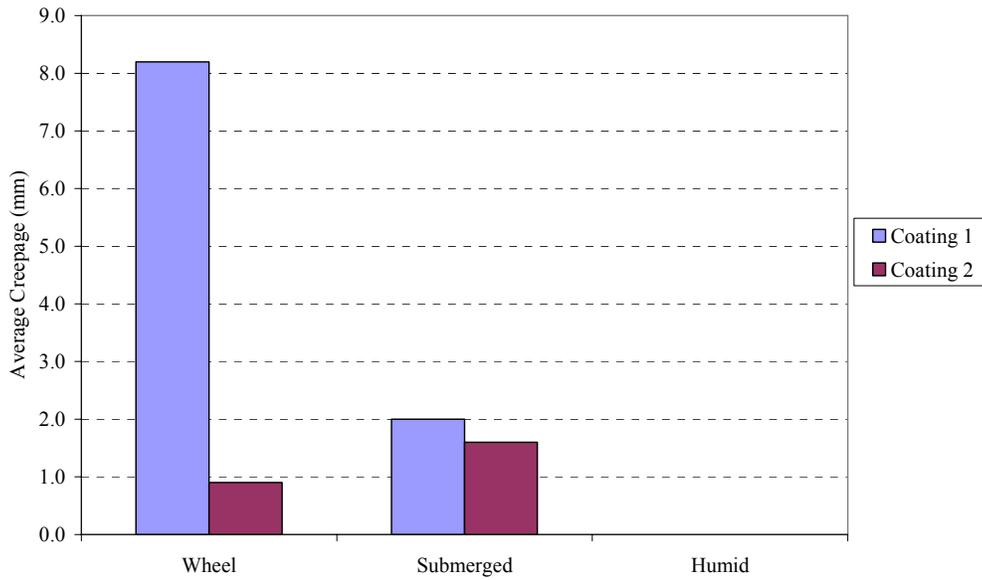
**Figure 4.16(c): Average Creepage vs. Location in Tank, Fresh Water**
