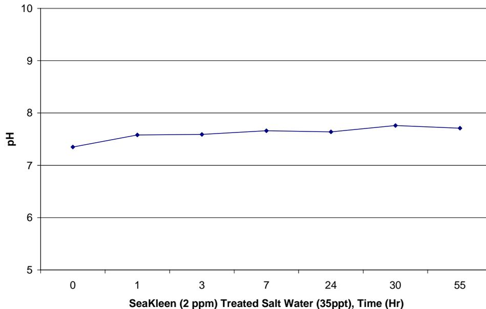
**Figure 4.9(b): pH vs. Time for SeaKleen™ (2ppm) Treated Salt Water (35ppt salinity)**
