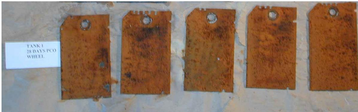
Figure G1: Corroded Plates Exposed to Splash Zone Environment in 15 ppt Salt Water, Tank 1, (Control Tank)
