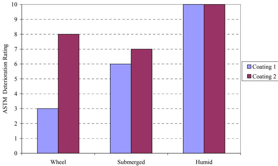
**Figure 4.16(a): ASTM Score vs. Location in Tanks, Fresh Water (Average across Control and SeaKleen™ Treated Tanks)**
