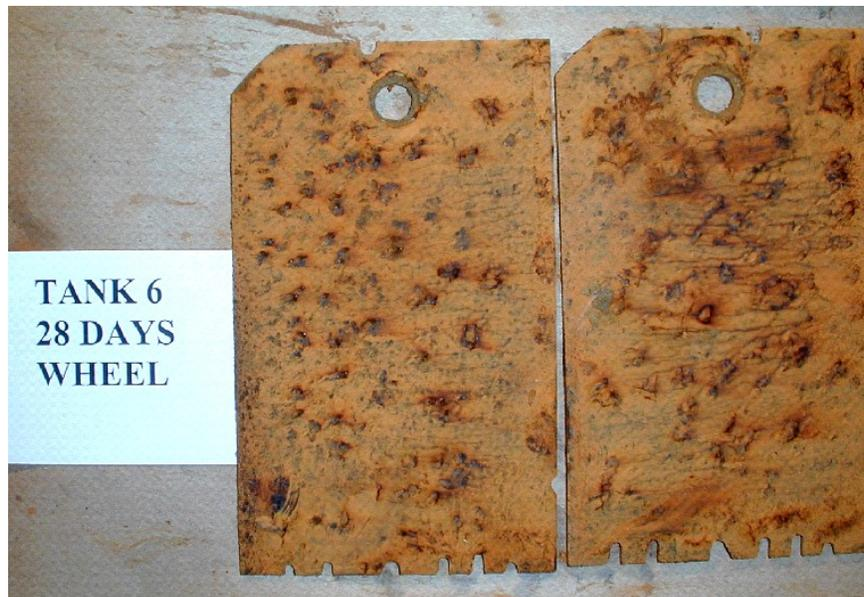
Figure E6: Corroded Plates Exposed to Splash Zone Environment in 35 ppt Salt Water, Tank 6, (High Dosage, SeaKleen™)
