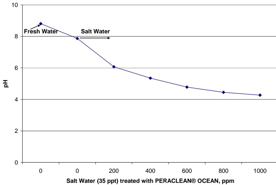
**Figure 4.19(c): Effect of PERACLEAN® OCEAN Concentration on pH of Salt Water (35 ppt Salinity)**
