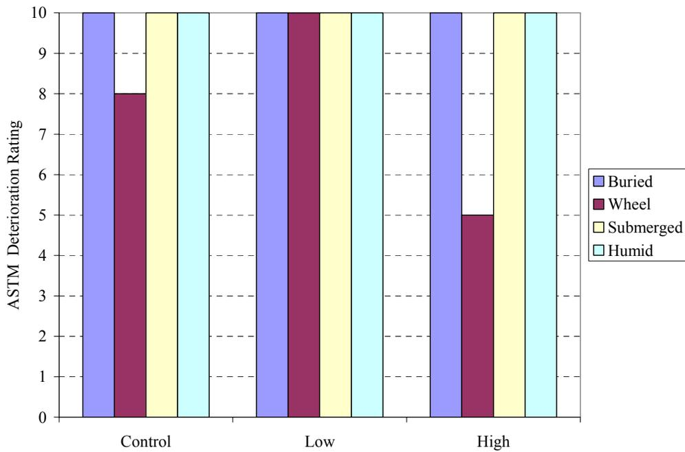
Figure H12: Coating 1 (15 ppt) - Deterioration Rating vs. Concentration (PERACLEAN® OCEAN)
