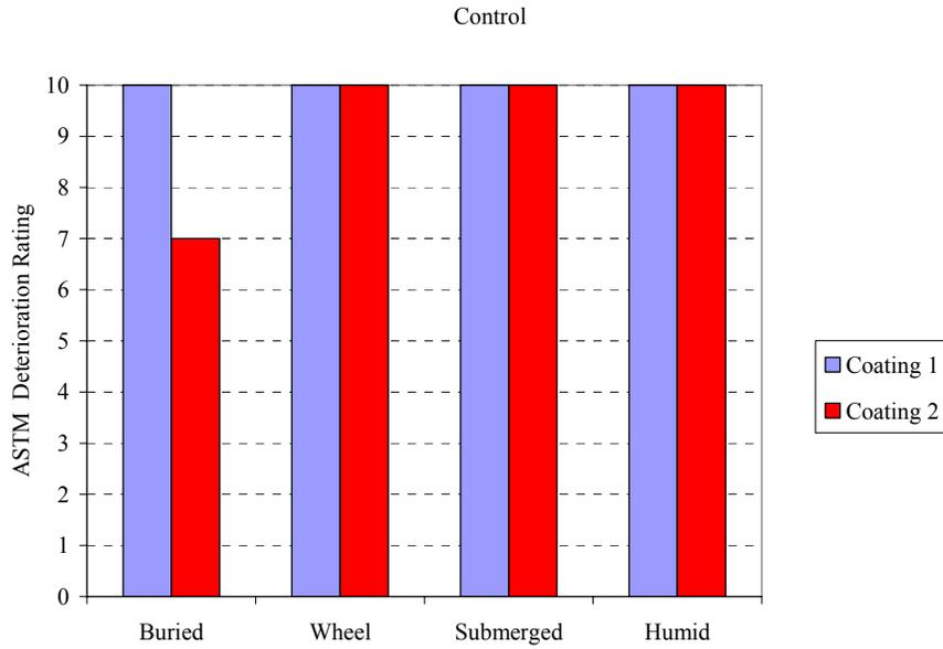
Figure F9: Tank 4 (35 ppt) - Deterioration Rating vs. Location (SeaKleen™)
