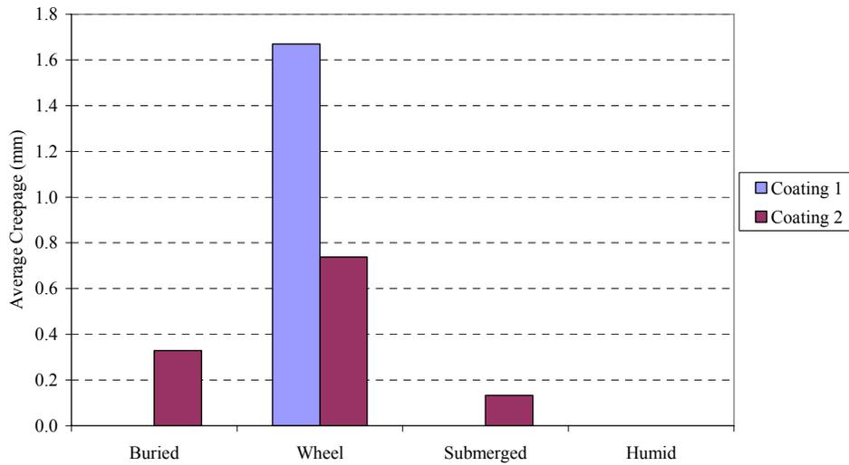
**Figure 4.33(c): Average Creepage vs. Location in Tank, 15 ppt Salt Water**
