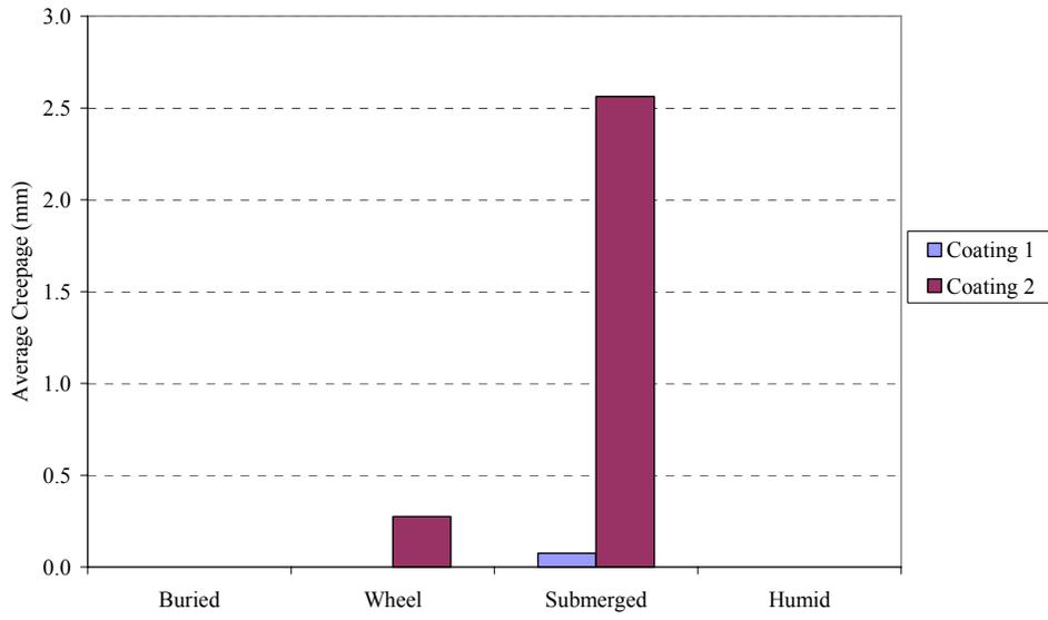
**Figure 4.34(c): Average Creepage vs. Location in Tank, 35 ppt Salt Water**
