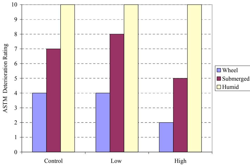
Figure F4: Coating 1 (Fresh Water) - Deterioration Rating vs. Concentration (SeaKleen™)
