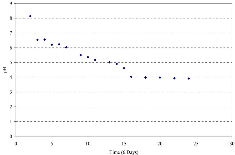
**Figure 4.27: Effect of Addition of PERACLEAN® OCEAN on Bulk Solution pH in 35 ppt Salt Water Every 4 Hours to Maintain Half Strength**
