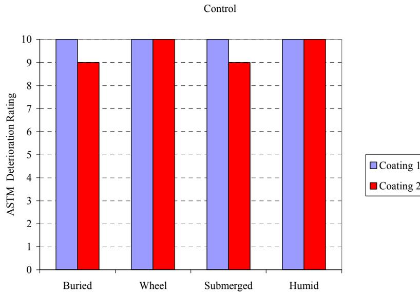
Figure F6: Tank 1 (15 ppt) - Deterioration Rating vs. Location (SeaKleen™)
