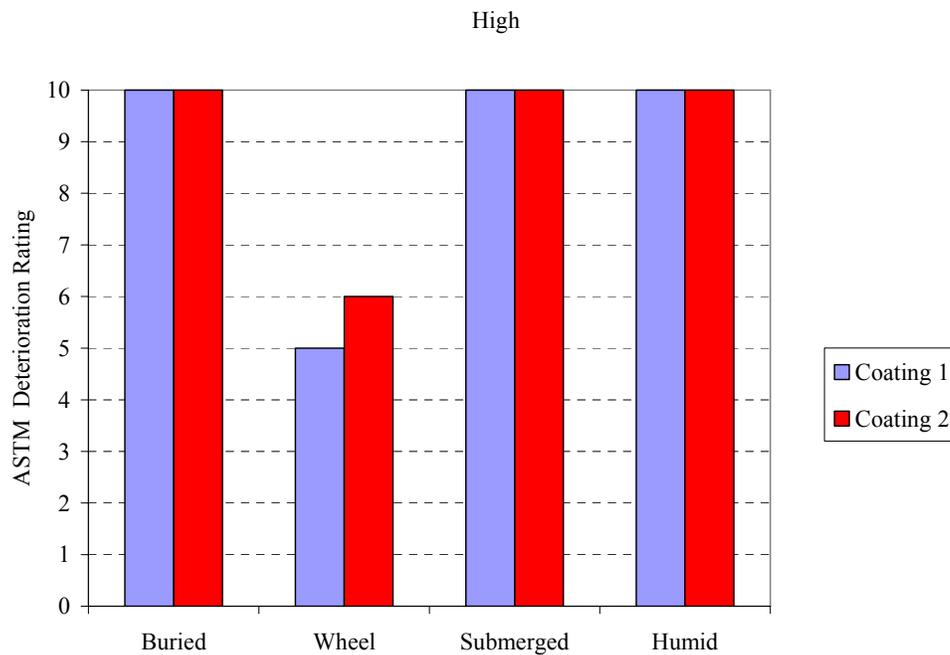
Figure H8: Tank 3 (15 ppt) - Deterioration Rating vs. Location (PERACLEAN® OCEAN)
