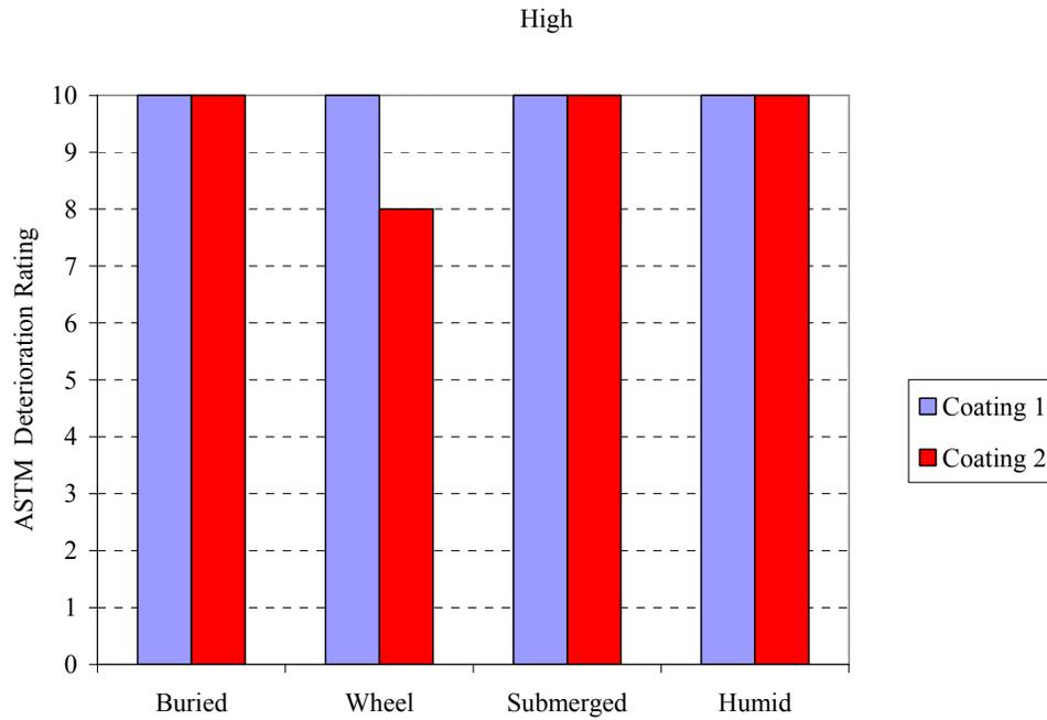
Figure H11: Tank 6 (35 ppt) - Deterioration Rating vs. Location (PERACLEAN® OCEAN)
