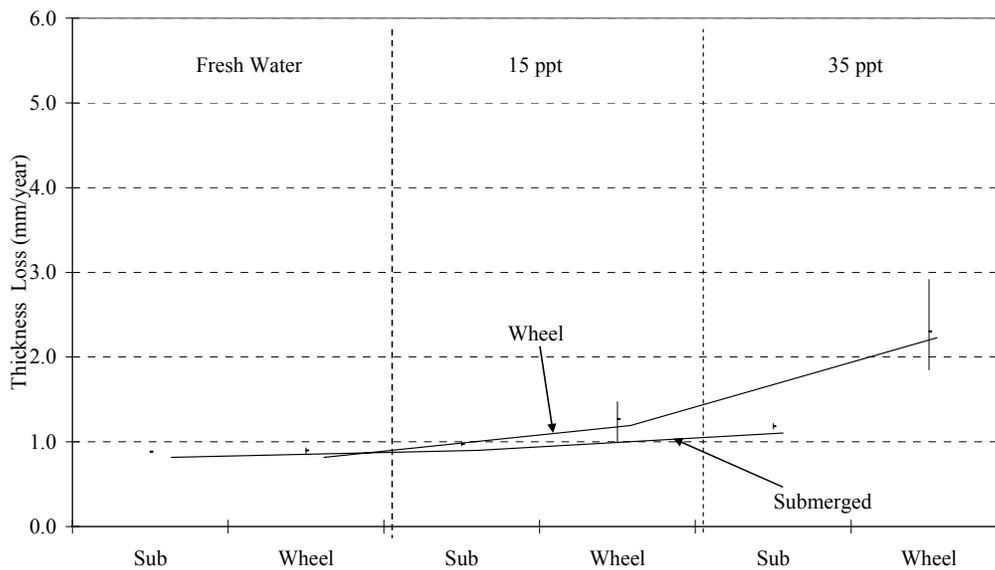
**Figure 4.31(b): Comparison of Corrosion Rates in Fresh Water, 15 ppt Salt Water and 35 ppt Salt Water for Wheel and Submerged Coupons exposed to High Dosage PERACLEAN® OCEAN Concentration**
