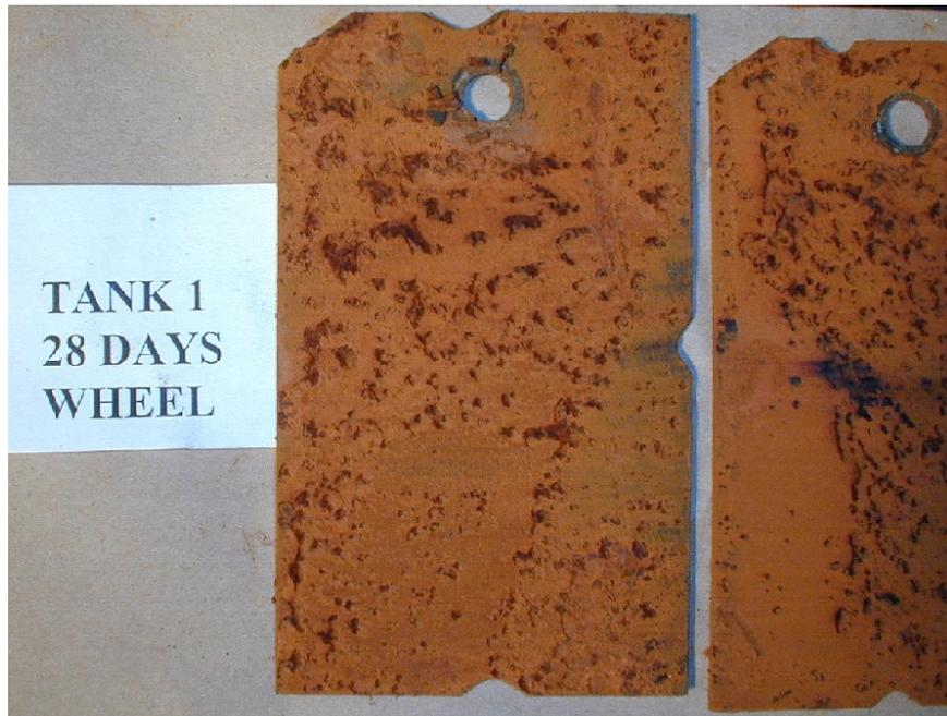
Figure E1: Corroded Plates Exposed to Splash Zone Environment in 15 ppt Salt Water, Tank 1, (Control Tank)
