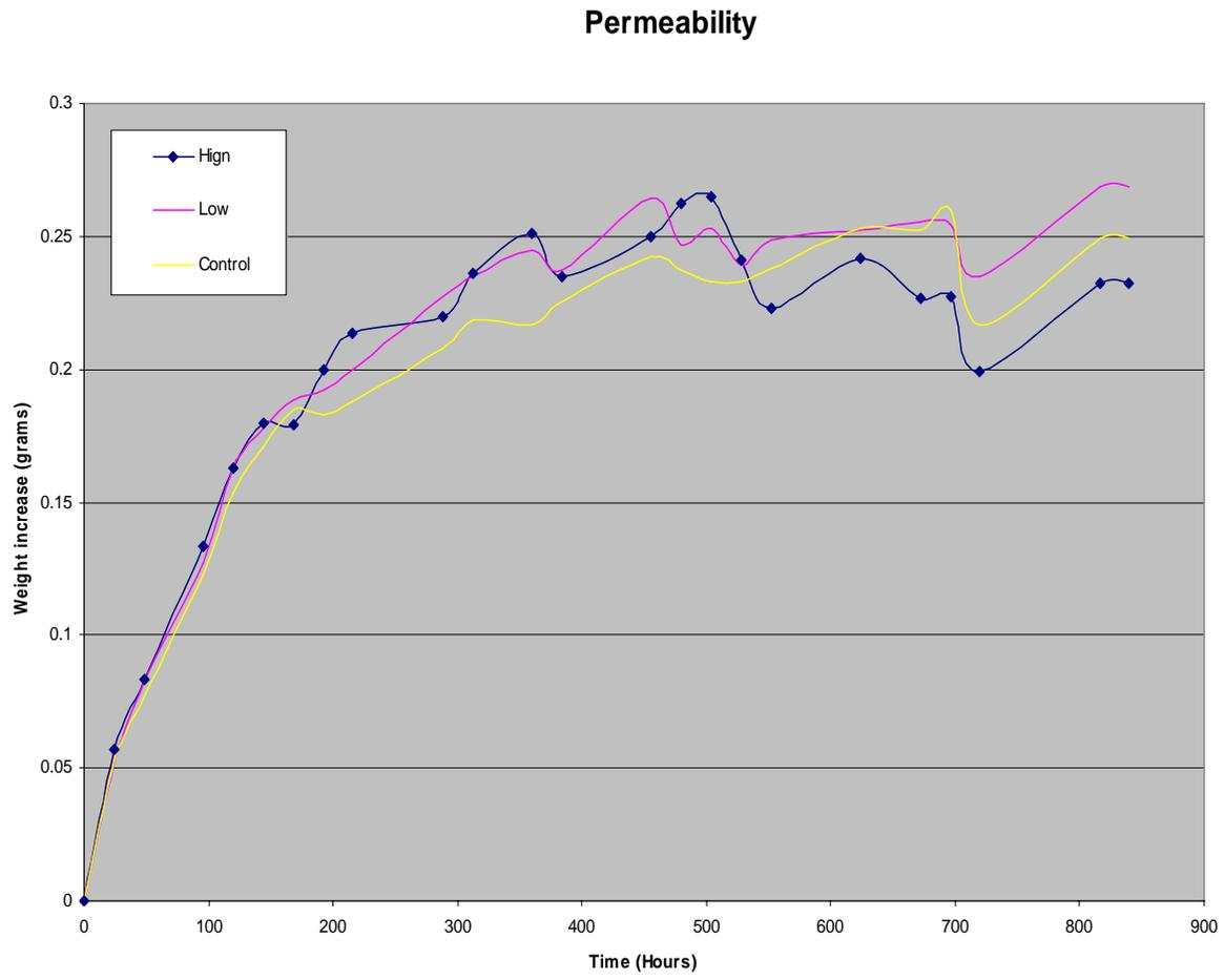
**Figure 2.9: Water Take-up Increase over Time Varying Exposure to Hypochlorite**
