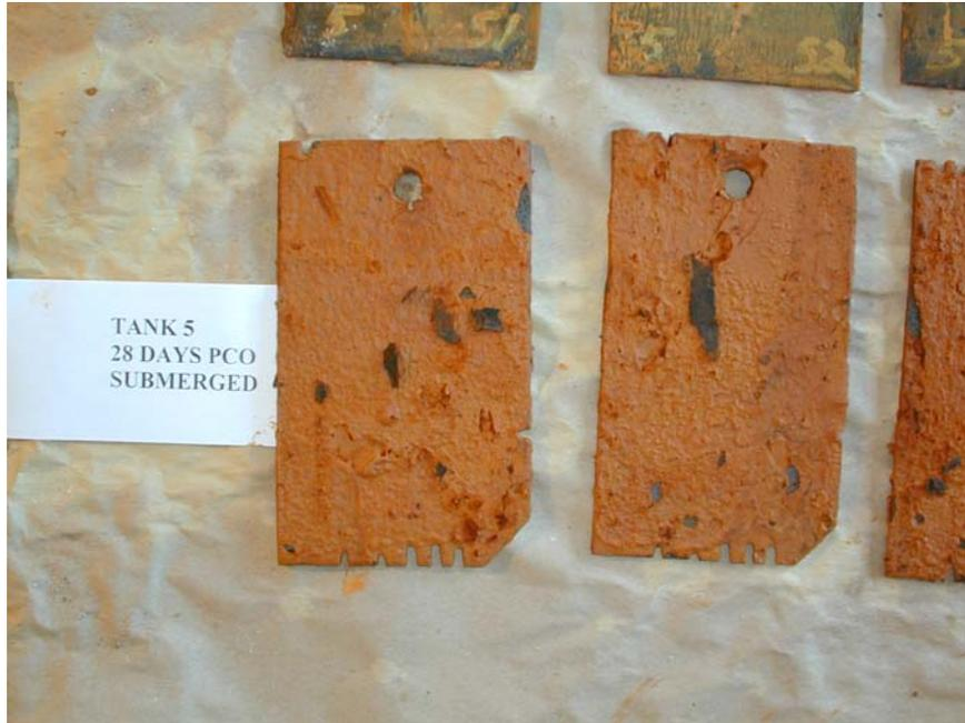
Figure G11: Corroded Plates Exposed to Submerged Environment in 35 ppt Salt Water, Tank 5, (Low Dosage, PERACLEAN® OCEAN)
