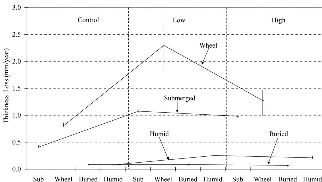
**Figure 4.29: Loss of Thickness in Corrosion Tank, 15 ppt Salt Water Tests**
