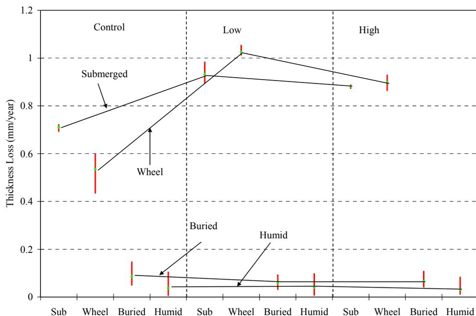
**Figure 4.28: Loss of Thickness in Corrosion Tank, Fresh Water Tests**
