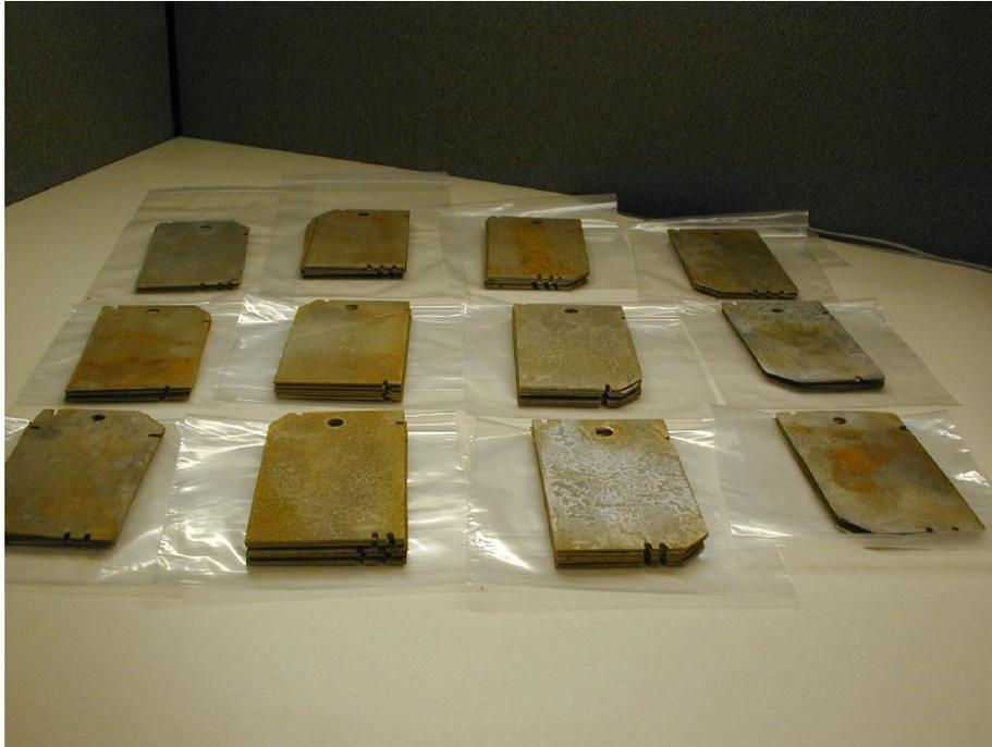
**Figure 4.6(b): Post Experiment, Cleaned, Bare Steel Plates**
