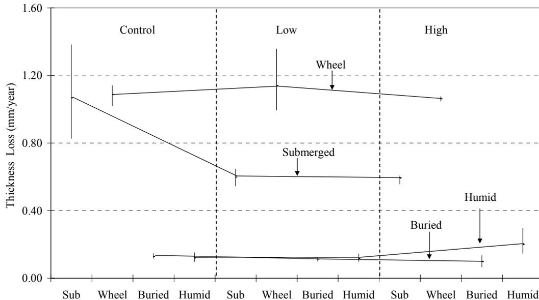
**Figure 4.13: Loss of Thickness in Corrosion Tank, 15 ppt Salt Water**
