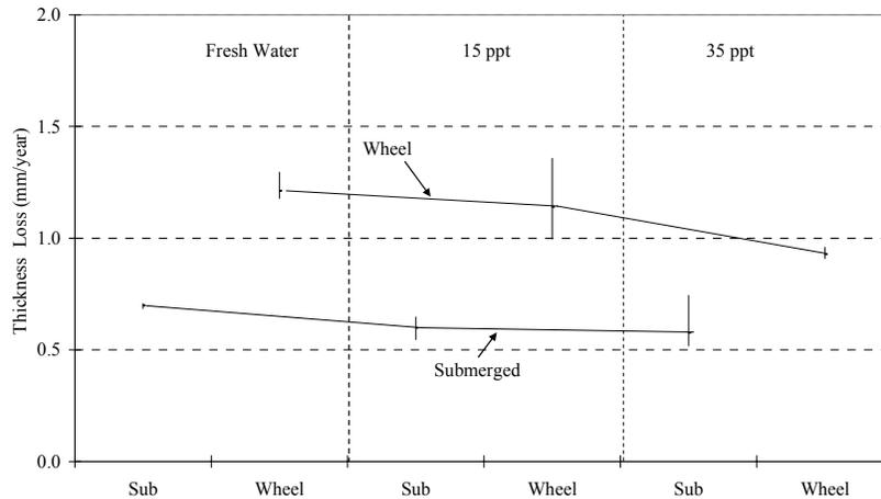
**Figure 4.15(a): Comparison of Corrosion Rates in Fresh Water, 15 ppt Salt Water and 35 ppt Salt Water for Wheel and Submerged Coupons exposed to Low Dosage SeaKleen™ Concentration**
