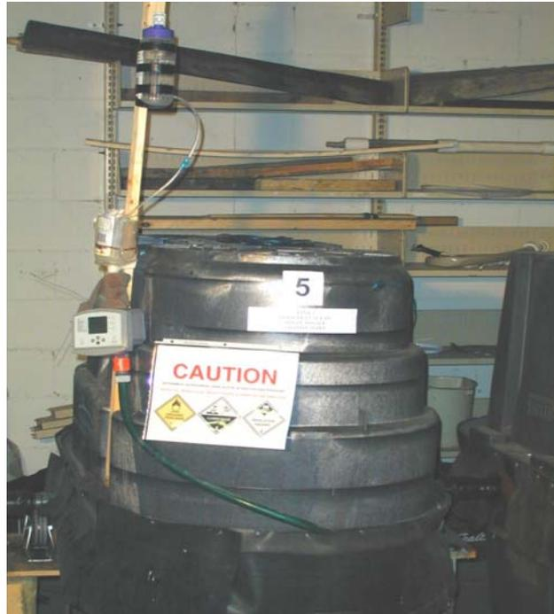
**Figure 4.24: Experimental Set Up showing Automatic Dosing Arrangement for PERACLEAN® OCEAN during Salt Water Corrosion Tests**
