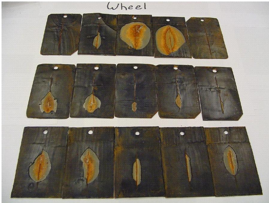
**Figure 4.7(b): Creepage in Coated Plates**
