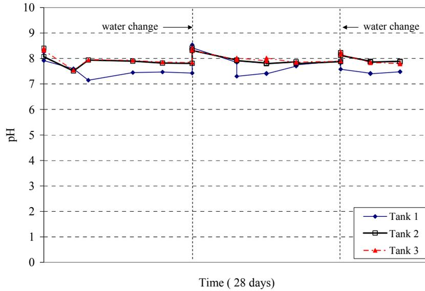
**Figure 4.11(a): Bulk Solution pH Measurements for Tanks 1, 2 and 3 for the Duration of the Salt Water Corrosion Test**
