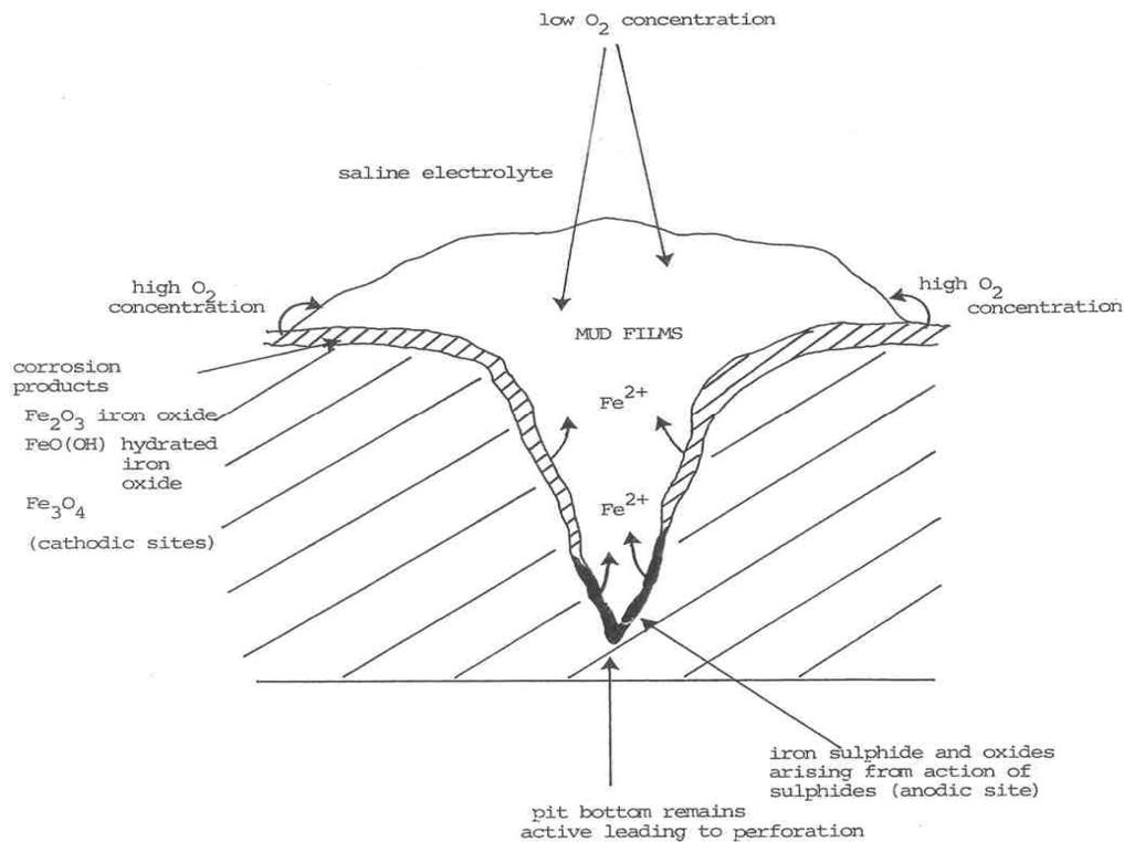
**Figure 2.8: Corrosion Cells that Can Arise under Mud Films and in the Presence of Biofilms [5]**
