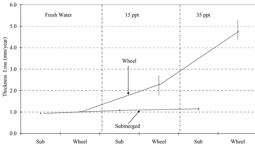
**Figure 4.31(a): Comparison of Corrosion Rates in Fresh Water, 15 ppt Salt Water and 35 ppt Salt Water for Wheel and Submerged Coupons exposed to Low Dosage PERACLEAN® OCEAN Concentration.**
