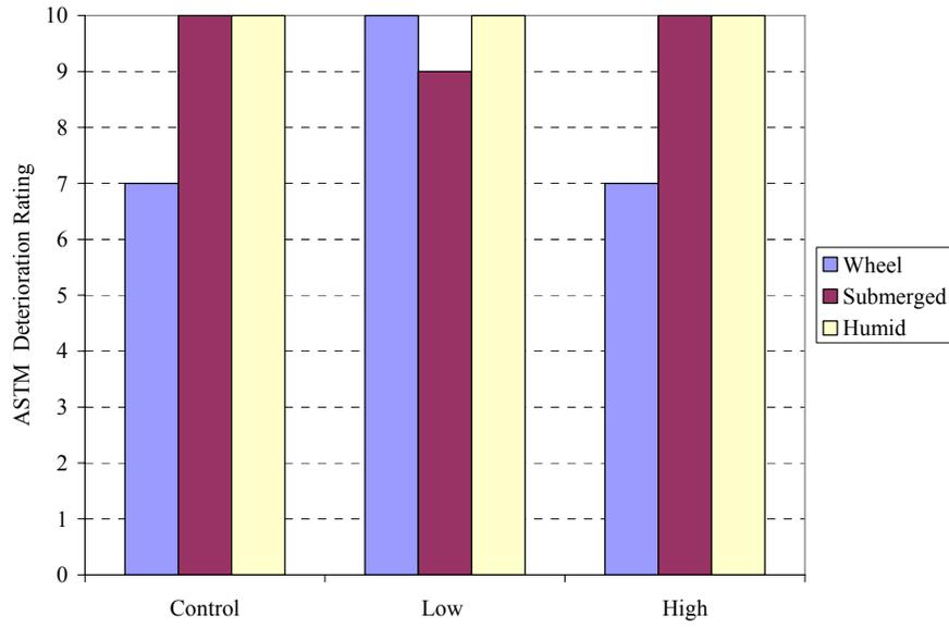
Figure H5: Coating 2 (Fresh Water) - Deterioration Rating vs. Concentration (PERACLEAN® OCEAN)
