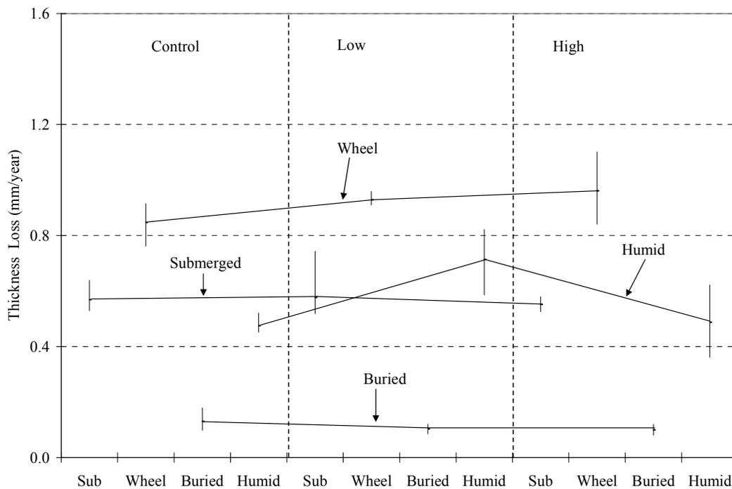
**Figure 4.14: Loss of Thickness in Corrosion Tank, 35 ppt Salt Water**
