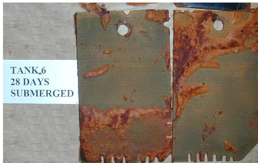
Figure E12: Corroded Plates Exposed to Submerged Environment in 35 ppt Salt Water, Tank 6, (High Dosage, SeaKleen™)
