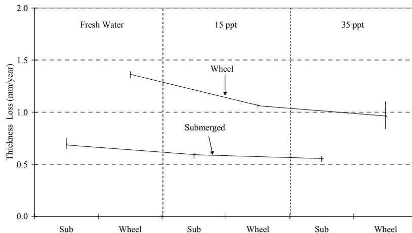
**Figure 4.15(b): Comparison of Corrosion Rates in Fresh Water, 15 ppt Salt Water and 35 ppt Salt Water for Wheel and Submerged Coupons exposed to High Dosage SeaKleen™ Concentration**
