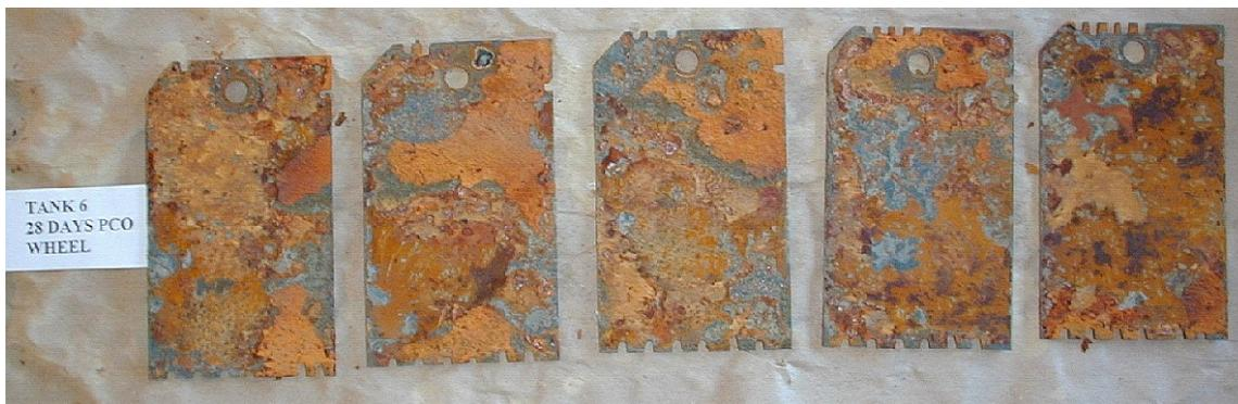
Figure G6: Corroded Plates Exposed to Splash Zone Environment in 35 ppt Salt Water, Tank 6, (High Dosage, PERACLEAN® OCEAN)
