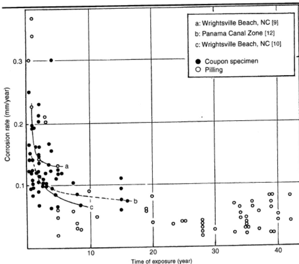
**Figure 2.1: Compilation of Data by Matsushima [3] for Steels Exposed to Sea Water for up to 40 Years**
