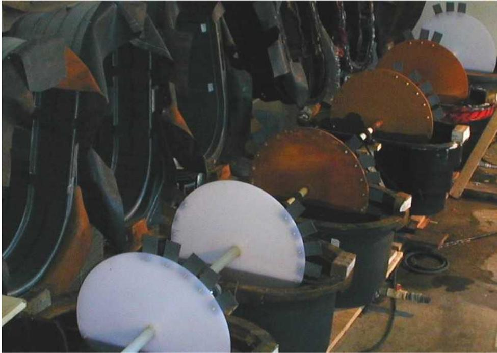
**Figure 4.4: Six Test Tank Arrangement for Salt Water Corrosion Testing**
