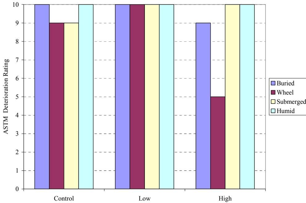
**Figure 4.33(b): ASTM Score vs. Exposure (Average across all Coatings), 15 ppt Salt Water**
