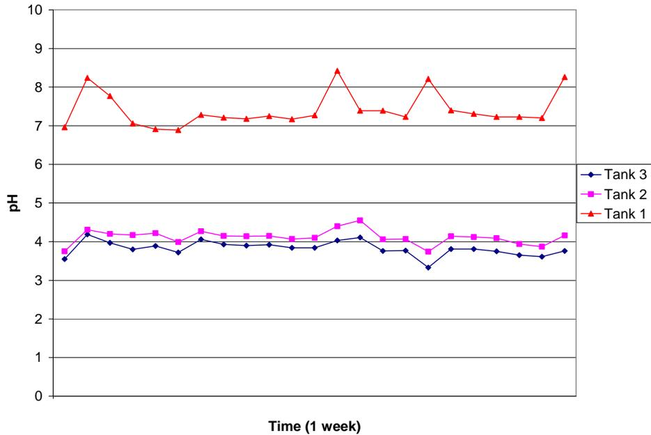
**Figure 4.22: Bulk Solution pH Measurements Carried out in the Three Tanks for One Week During Fresh Water Tests**
