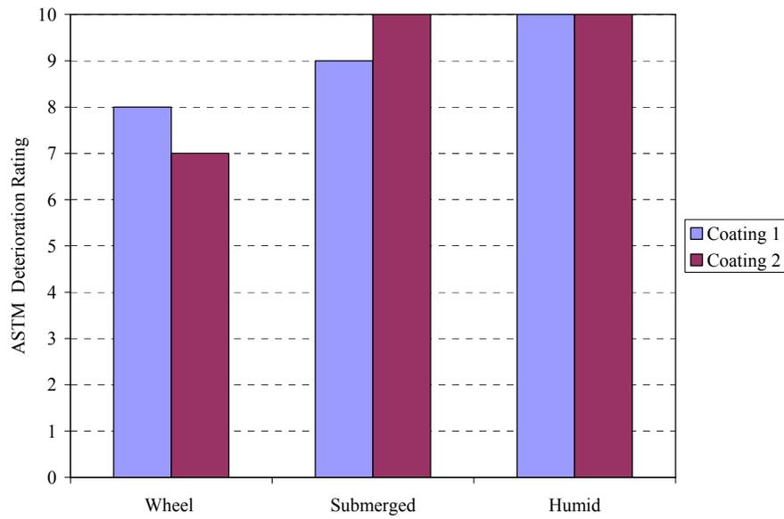
Figure H1: Tank 1 (Fresh Water) - Deterioration Rating vs. Location (PERACLEAN® OCEAN)
