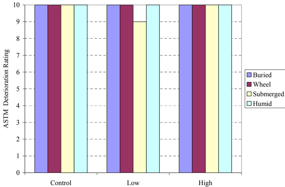
Figure H14: Coating 1 (35 ppt) - Deterioration Rating vs. Concentration (PERACLEAN® OCEAN)
