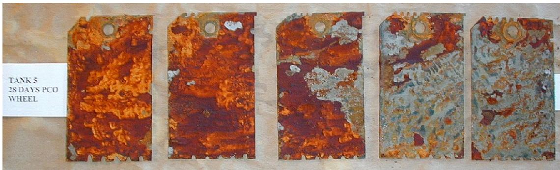
Figure G5: Corroded Plates Exposed to Splash Zone Environment in 35 ppt Salt Water, Tank 5, (Low Dosage, PERACLEAN® OCEAN)
