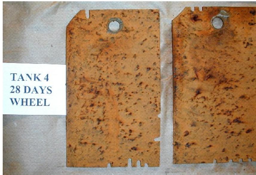
Figure E4: Corroded Plates Exposed to Splash Zone Environment in 35 ppt Salt Water, Tank 4, (Control Tank)
