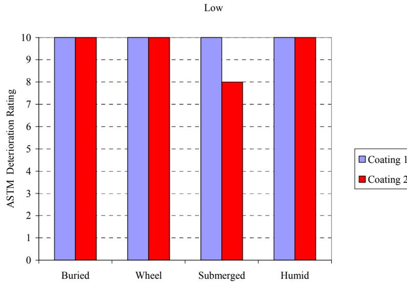
Figure F7: Tank 2 (15 ppt) - Deterioration Rating vs. Location (SeaKleen™)
