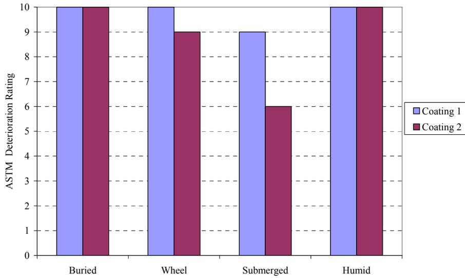
**Figure 4.34(a): ASTM Score vs. Location in Tanks, 35 ppt Salt Water (Average across Control and PERACLEAN® OCEAN Treated Tanks)**
