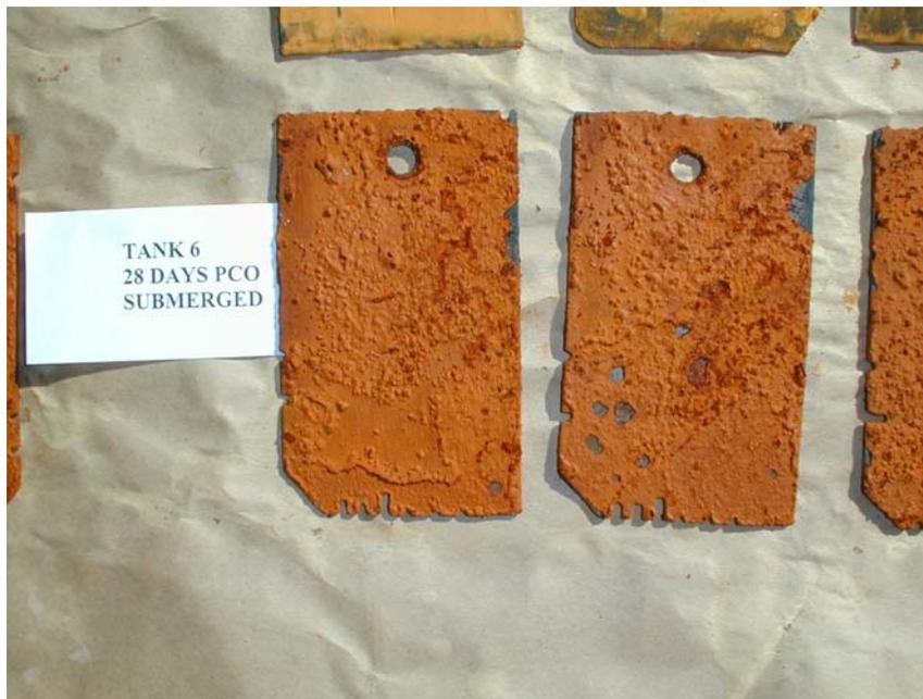
Figure G12: Corroded Plates Exposed to Submerged Environment in 35 ppt Salt Water, Tank 6, (High Dosage, PERACLEAN® OCEAN)
