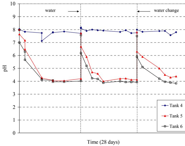
**Figure 4.25(b): Bulk Solution pH Measurements Carried out during 35 ppt Salt Water Tests Treated with PERACLEAN® OCEAN**
