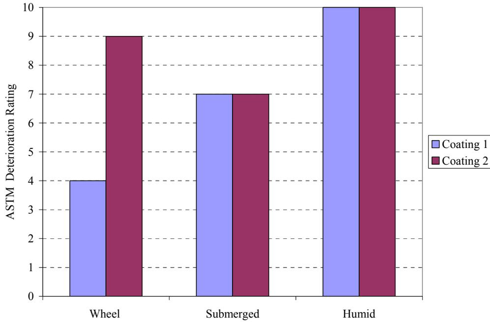
Figure F1: Tank 1 (Fresh Water) - Deterioration Rating vs. Location (SeaKleen™)
