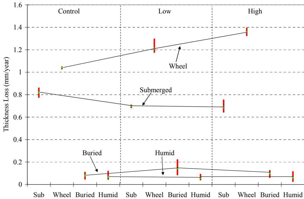
**Figure 4.12: Loss of Thickness in Corrosion Tank, Fresh Water**
