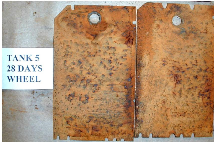
Figure E5: Corroded Plates Exposed to Splash Zone Environment in 35 ppt Salt Water, Tank 5, (Low Dosage, SeaKleen™)
