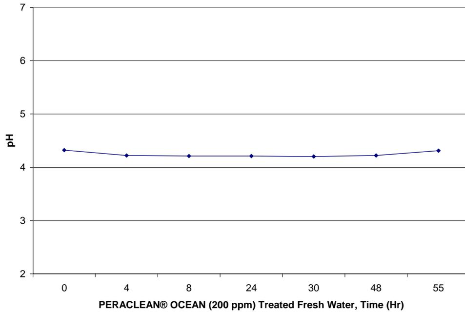
**Figure 4.20(a): pH vs. Time for PERACLEAN® OCEAN (200 ppm) Treated Fresh Water**
