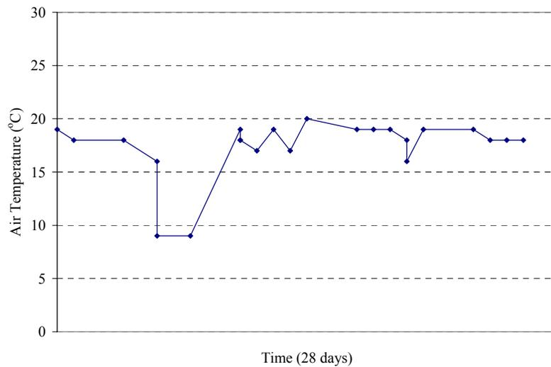
**Figure 4.23: Test Temperature for the Duration of the Salt Water Corrosion Test**
