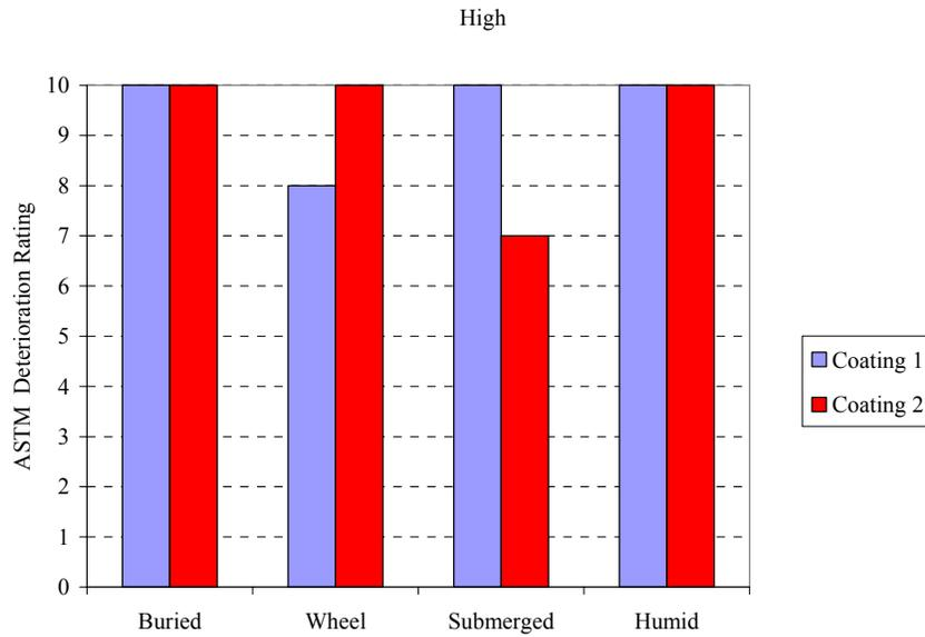
Figure F11: Tank 6 (35 ppt) - Deterioration Rating vs. Location (SeaKleen™)
