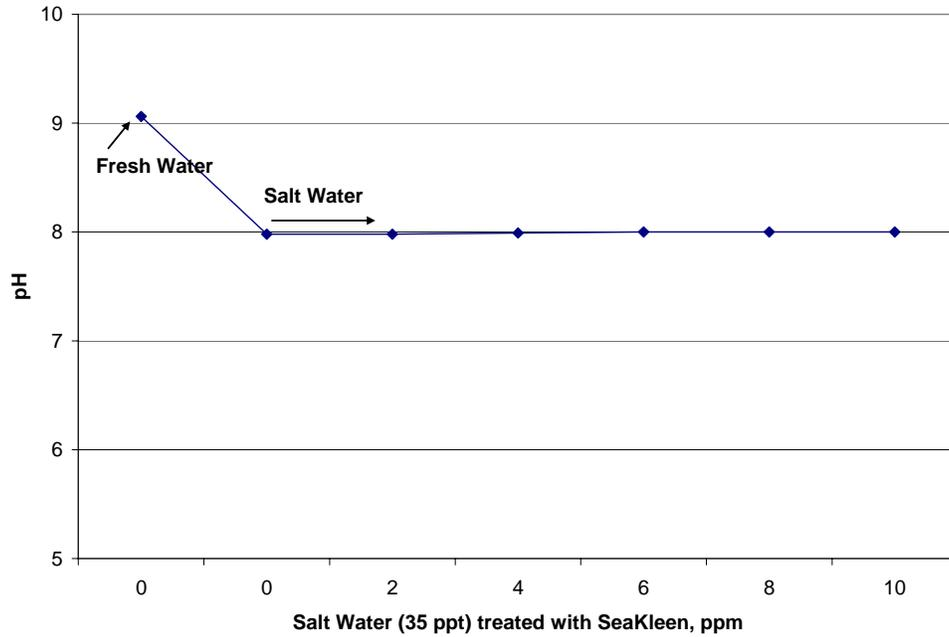
**Figure 4.8(c): Effect of SeaKleen™ Concentration on pH of Salt Water (35 ppt salinity)**
