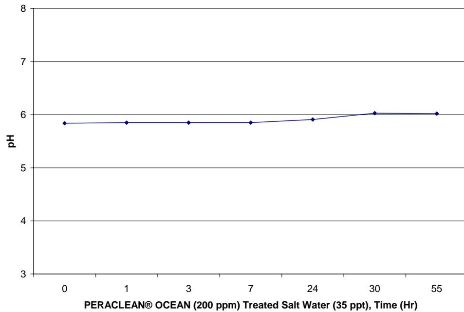
**Figure 4.20(b): pH vs. Time for PERACLEAN® OCEAN (200 ppm) Treated Salt Water (35 ppt Salinity)**
