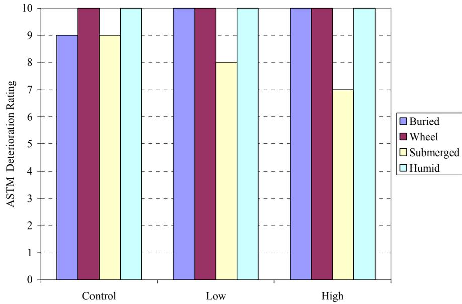
Figure F13: Coating 2 (15 ppt) - Deterioration Rating vs. Concentration (SeaKleen™)
