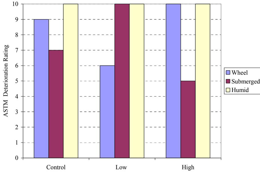
Figure F5: Coating 2 (Fresh Water) - Deterioration Rating vs. Concentration (SeaKleen™)
