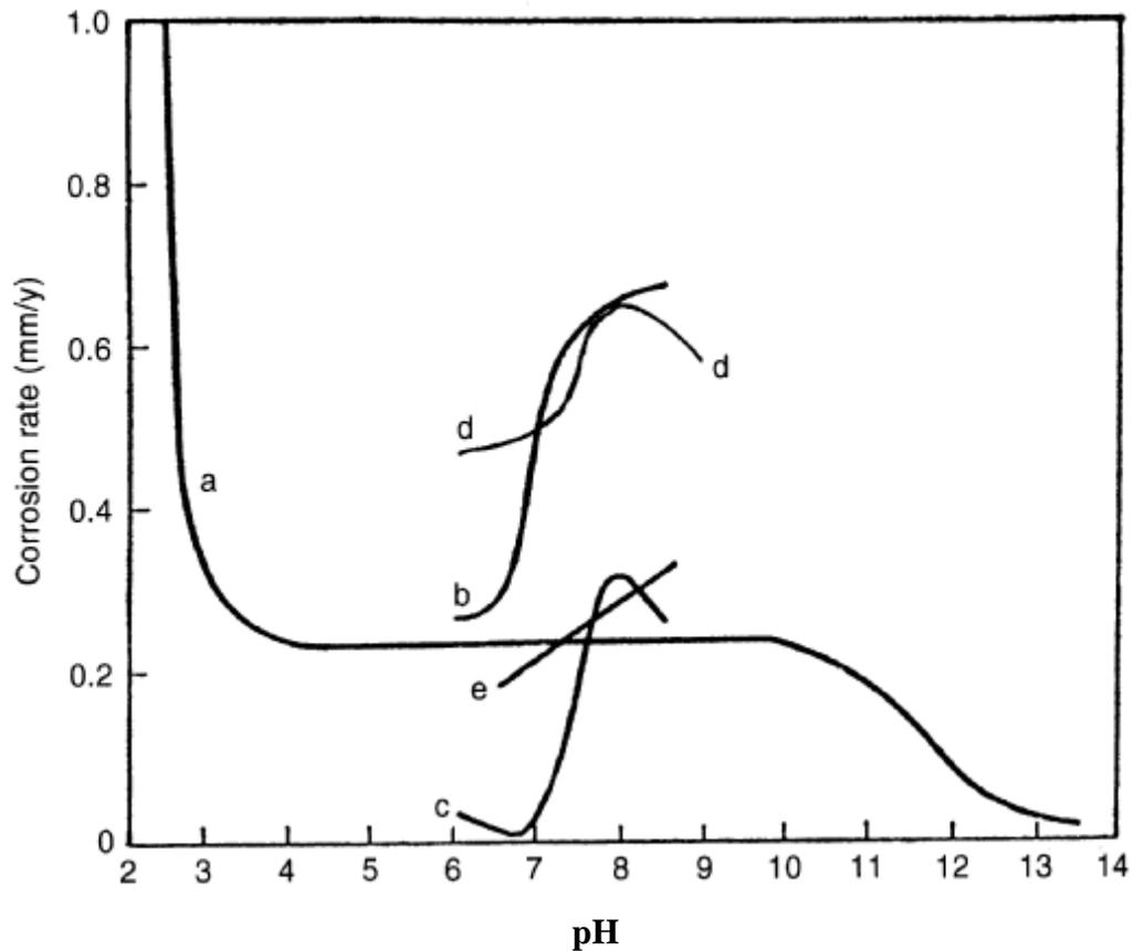
**Figure 2.3: Matsushima's [7] Results of the Effect of pH in Fresh Water Environments of Various Water Quality**
