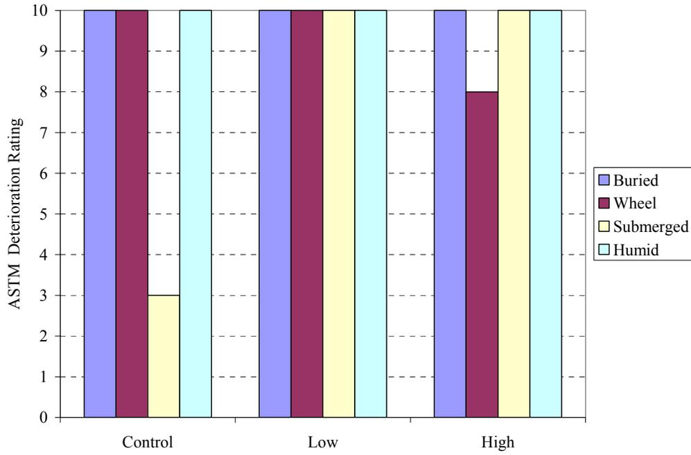
Figure H15: Coating 2 (35 ppt) - Deterioration Rating vs. Concentration (PERACLEAN® OCEAN)
