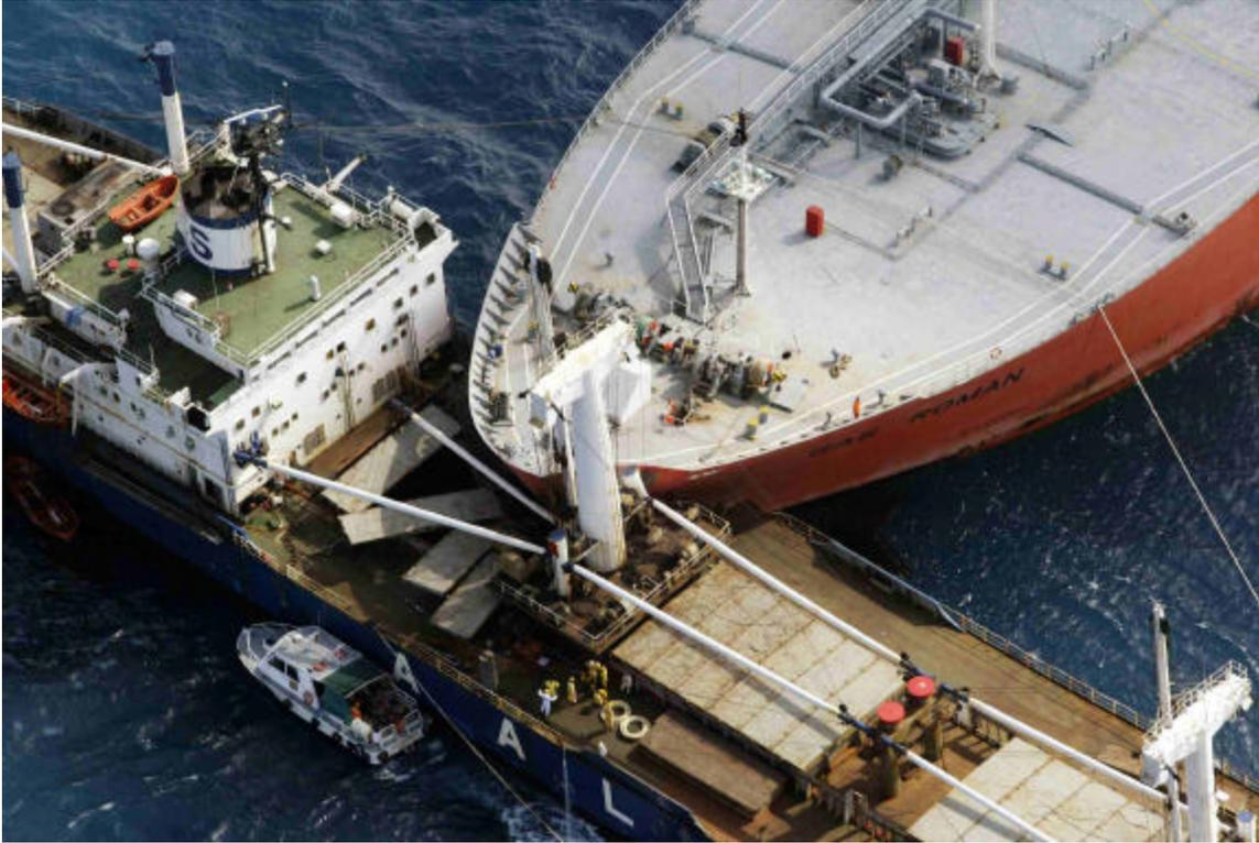
Figure 6 - Bow Damage of Collision of M/T Gas Roman and M/V Springbok
