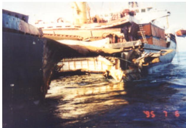
Figure 3 - Damage to M/V Enif
