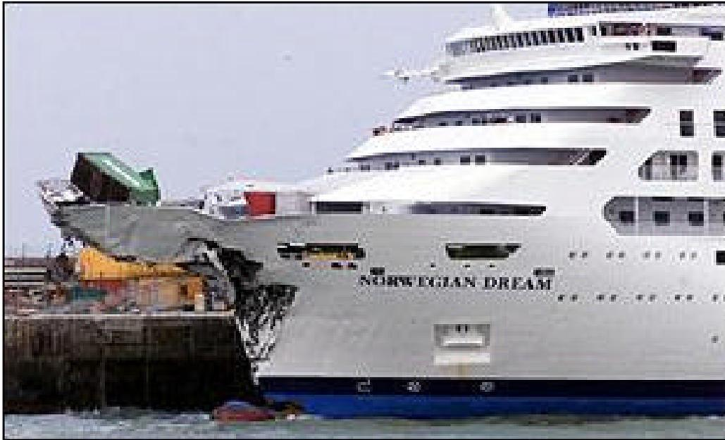
Figure 9 - Bow Damage to Norwegian Dream
