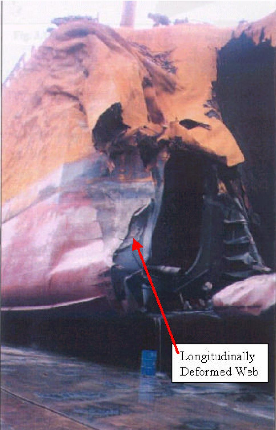
Figure 108 - Actual Longitudinally Deformed Web [89]
