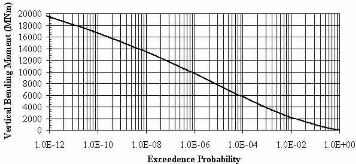
**Figure 4.11: Tanker Load Cycle Midship Vertical Bending Moments Exceedance Probabilities**
