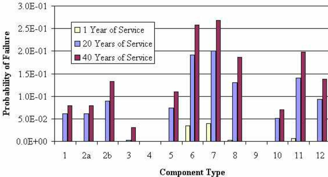
**Figure 4.43: Bulk Carrier Midship Type 1 Frame Component Failure Probability History**
