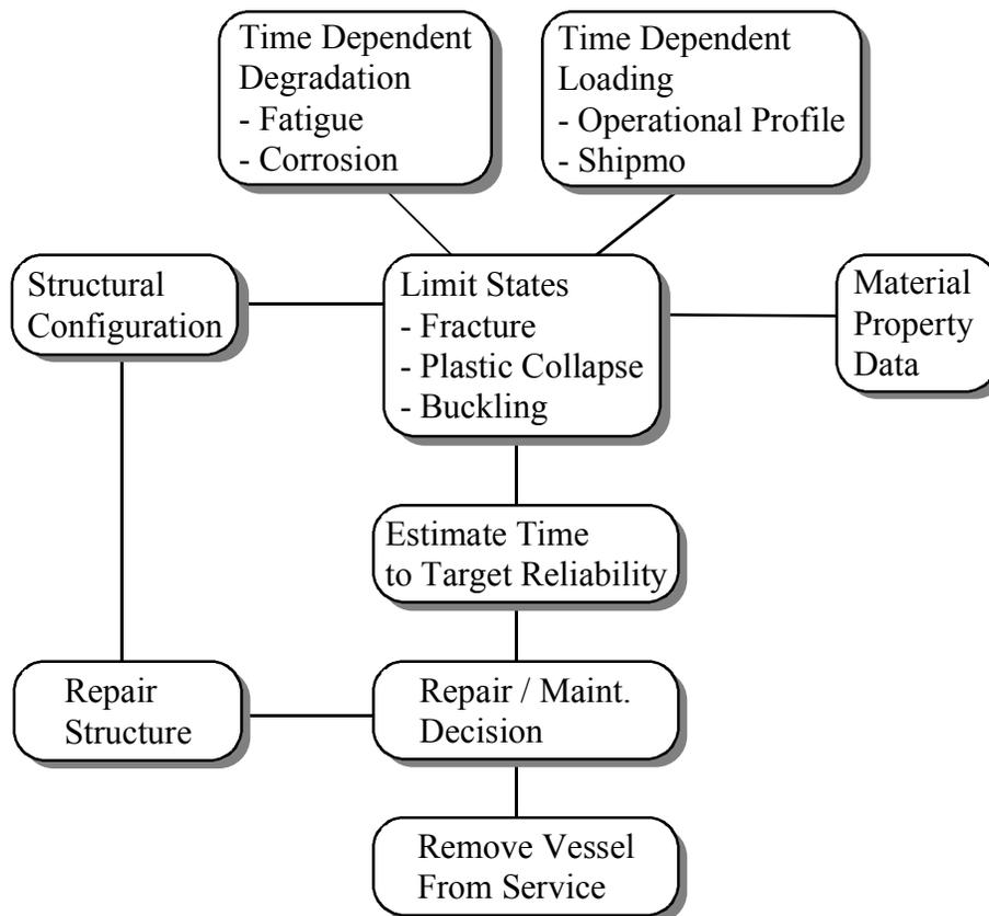
**Figure 2.5: Reliability-Based Vessel Life Cycle Management Process**
