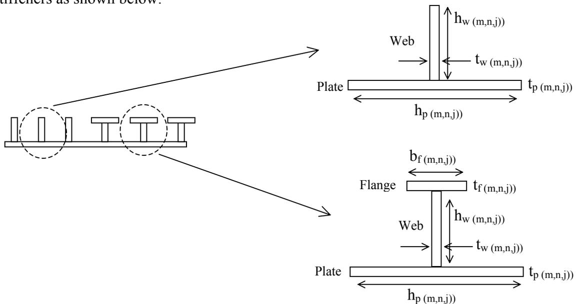
**Figure 3.5: Component Geometric Definition**
