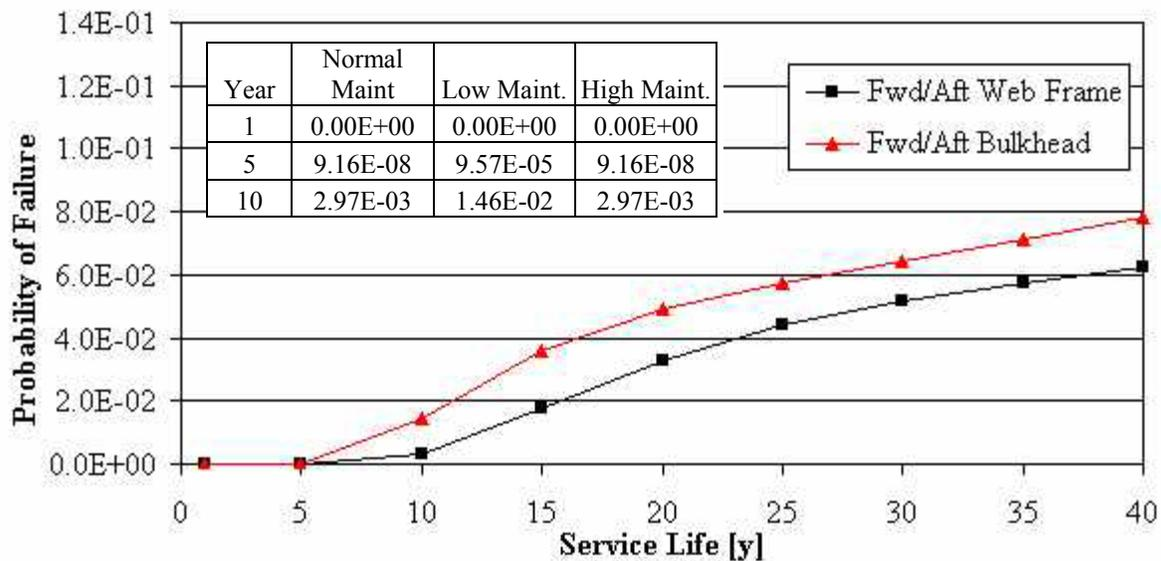
**Figure 4.40: Tanker Fwd/Aft Frame Fatigue Initiation Failure Probability**
