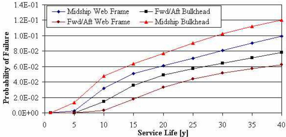
**Figure 4.27: Tanker Frame Type Time Dependant Reliability Comparison**
