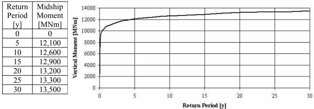
**Figure 4.13: Tanker Extreme Load Return Period**
