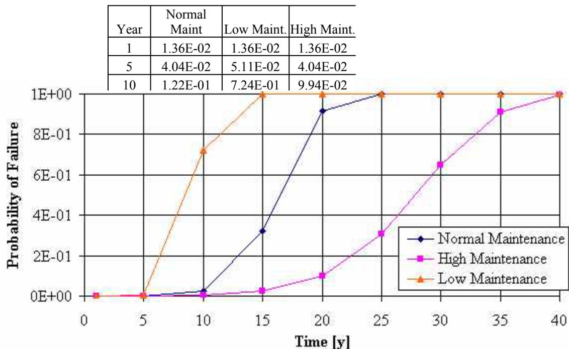
**Figure 4.25: Tanker Component Failure Probability in Compression**
