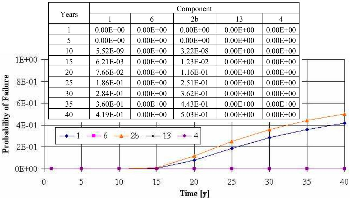
**Figure 4.16: Bulk Carrier Component Probability of Diminution Failure**
