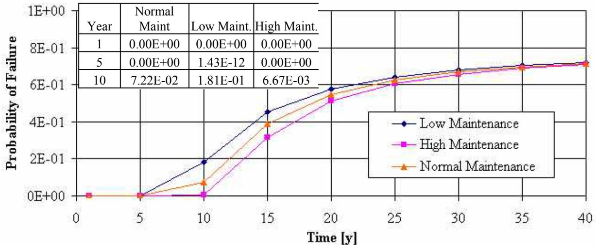
**Figure 4.18: Sensitivity of Bulk Carrier Pitting Time Dependant Reliability to Maintenance**
