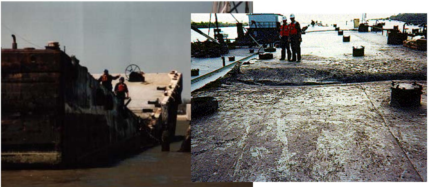
**Figure 2.4: Global Buckling Failure**
