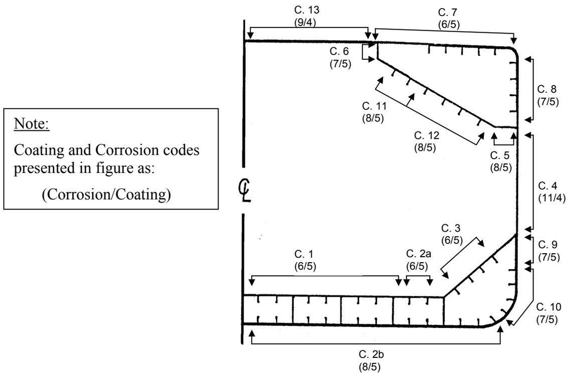
**Figure 4.14: Bulk Carrier Component Coating and Corrosion Codes**
