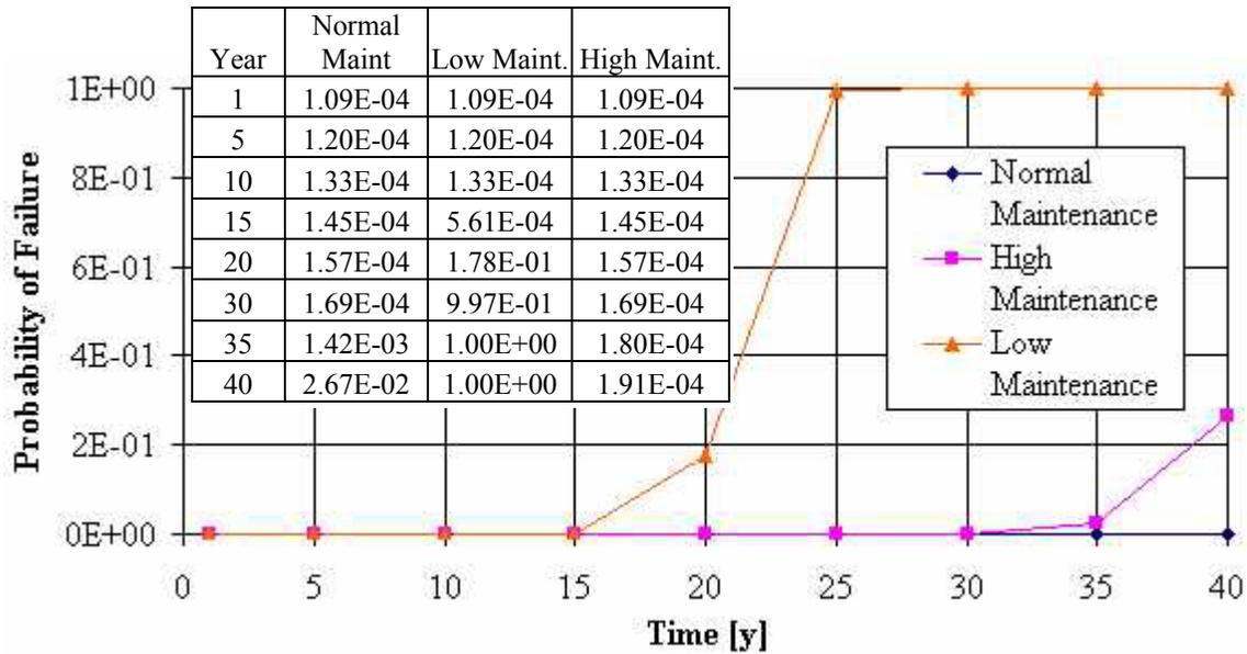
**Figure 4.34: Bulk Carrier Vessel Buckling and Ultimate Strength Failure Probability**
