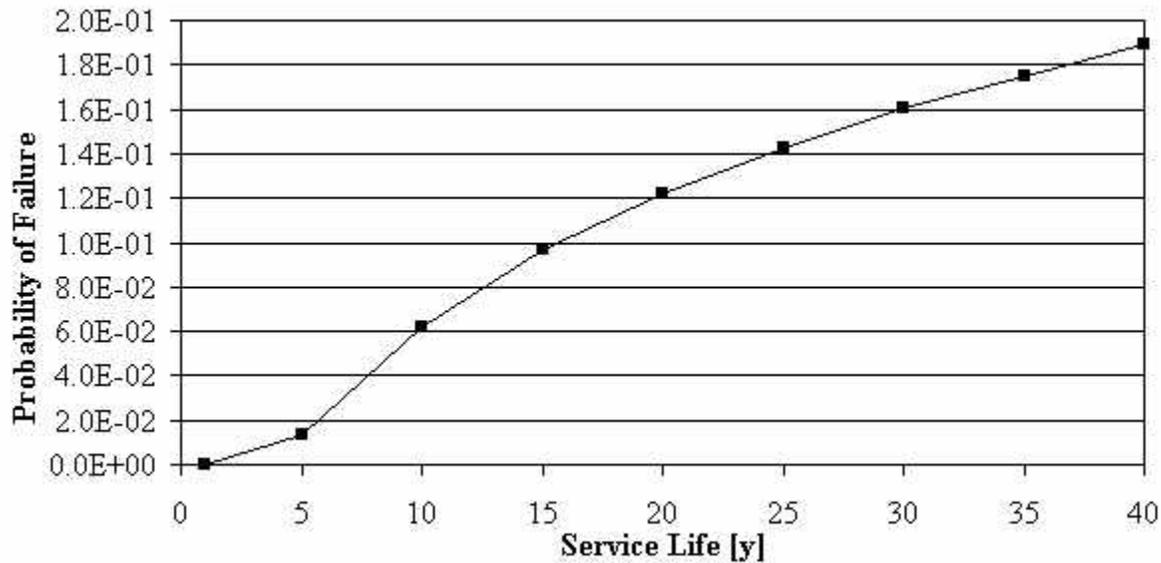
**Figure 4.41: Tanker Vessel Fatigue Initiation Failure Probability**
