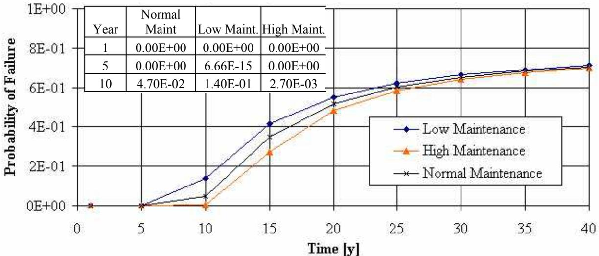
**Figure 4.23: Sensitivity of Tanker Pitting Time Dependant Reliability to Maintenance**
