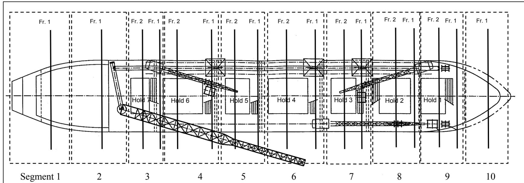
**Figure 4.3: General Arrangement of Segments and Frames in the Bulk Carrier**
