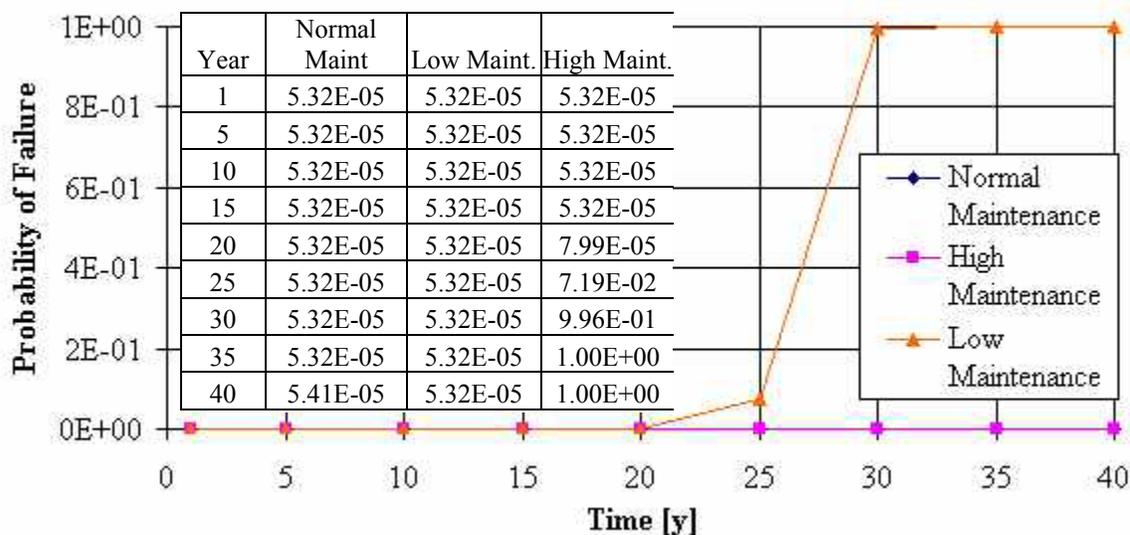
**Figure 4.24: Bulk Carrier Component Failure Probability in Compression**
