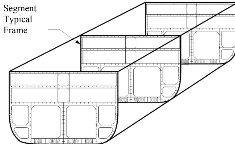
**Figure 3.2: Definition of Typical Frames for a Given Ship Segment**
