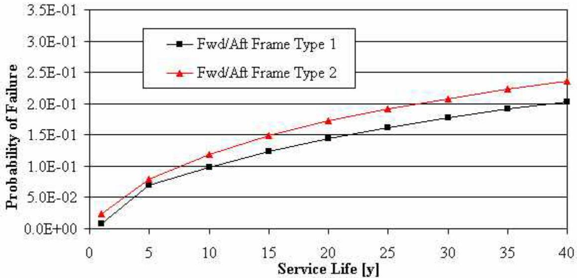
**Figure 4.37: Bulk Carrier Fwd/Aft Frame Fatigue Initiation Failure Probability**
