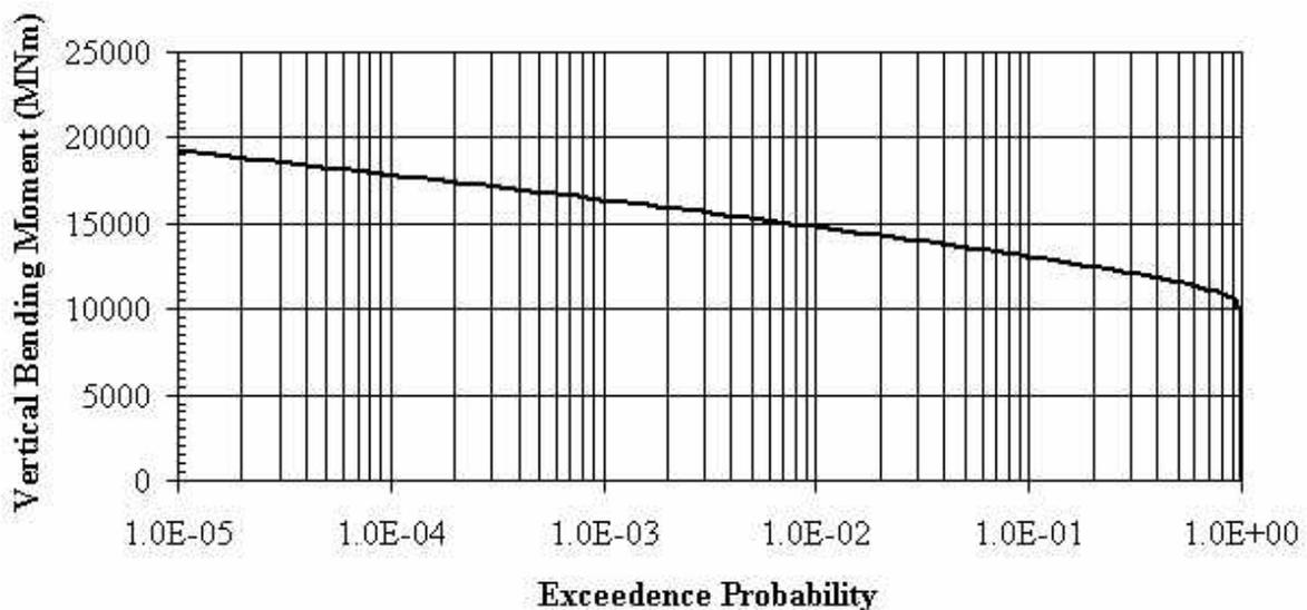
**Figure 4.12: Tanker Lifetime Midship Vertical Bending Moment Exceedance Probability**
