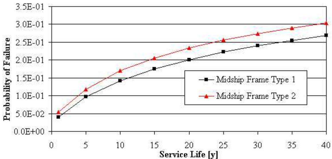
**Figure 4.36: Bulk Carrier Midship Frame Fatigue Initiation Failure Probability**
