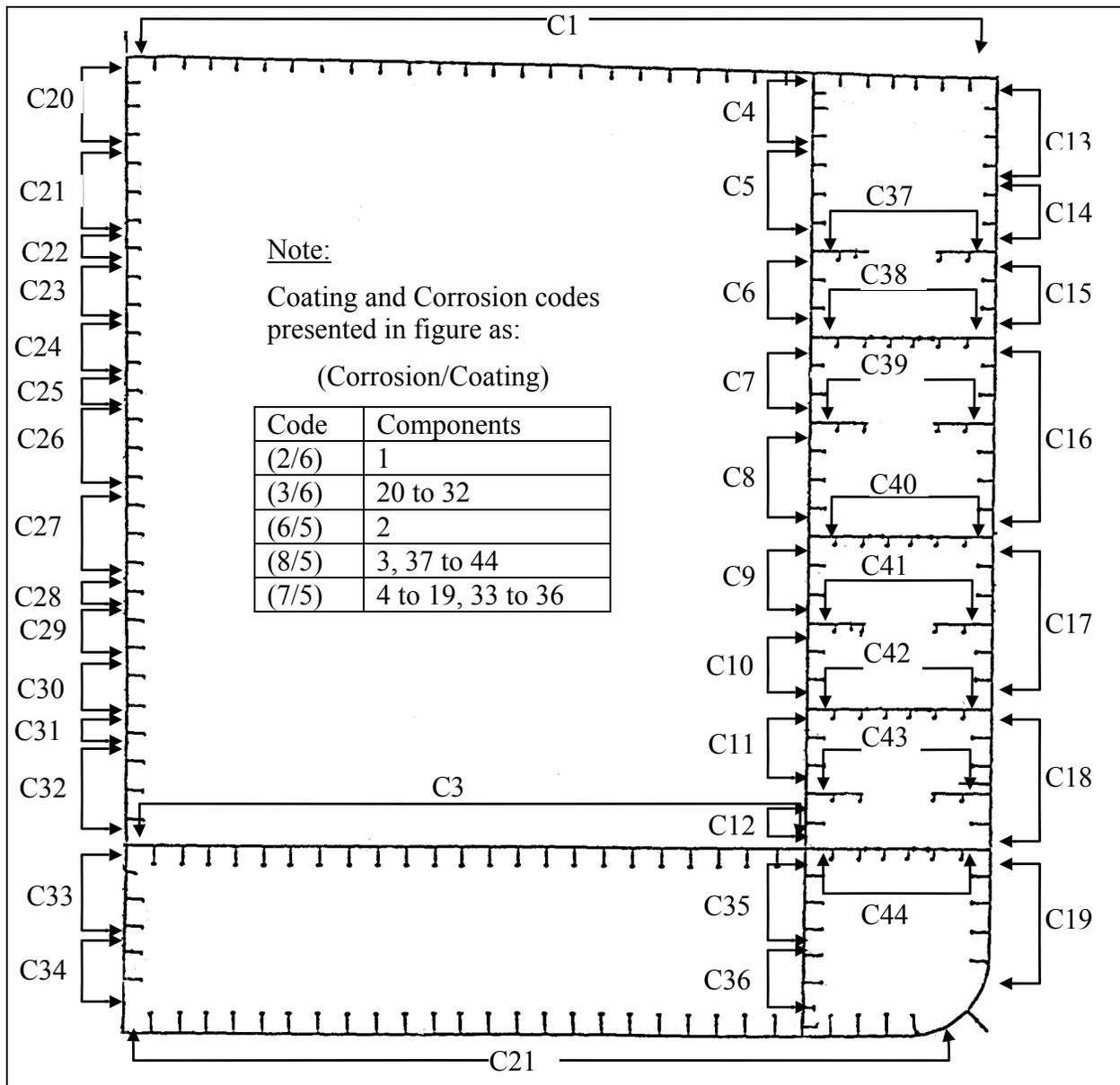
**Figure 4.19: Tanker Component Coating and Corrosion Codes**
