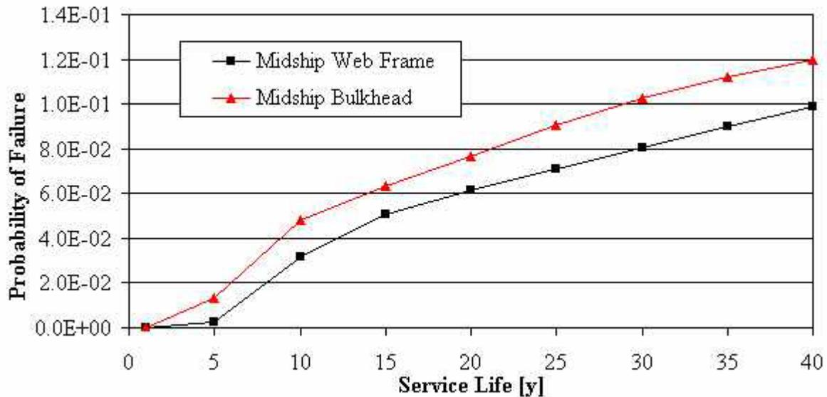
Figure 4.39: Tanker Midship Frame Fatigue Initiation Failure Probability
