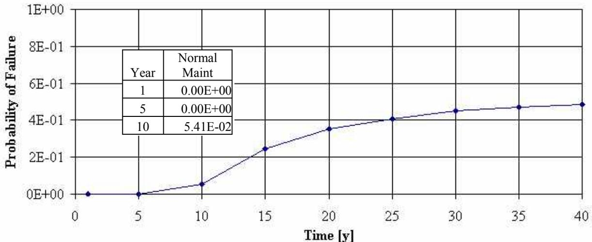
**Figure 4.17: Bulk Carrier Probability of Frame Average Diminution Failure**
