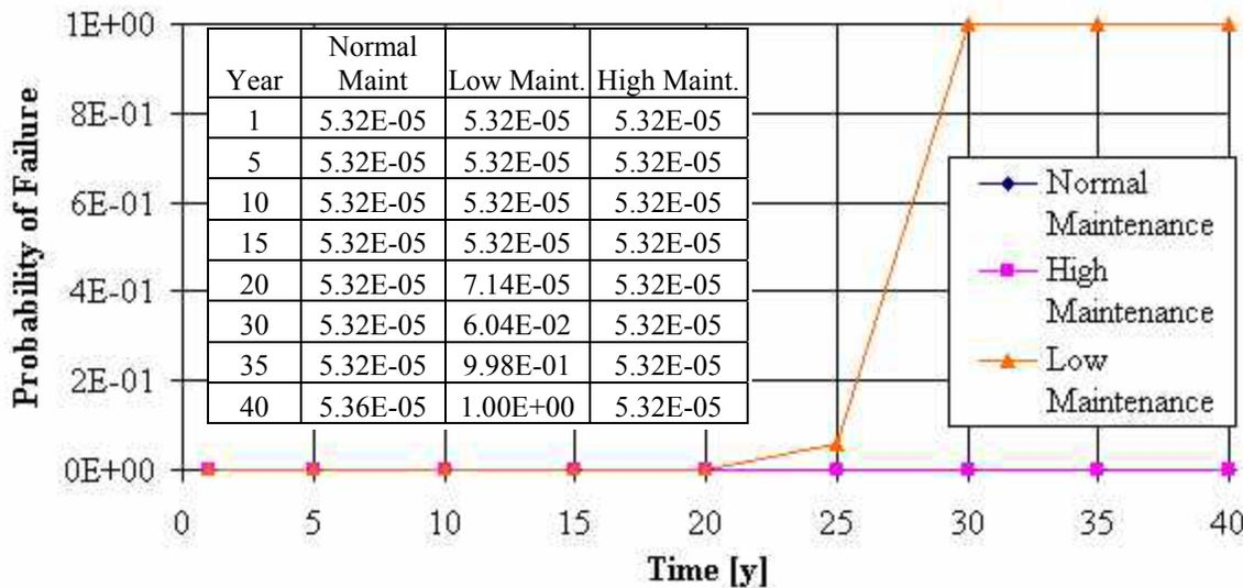
**Figure 4.33: Bulk Carrier Fwd/Aft Frame Buckling and Ultimate Strength Failure Probability**
