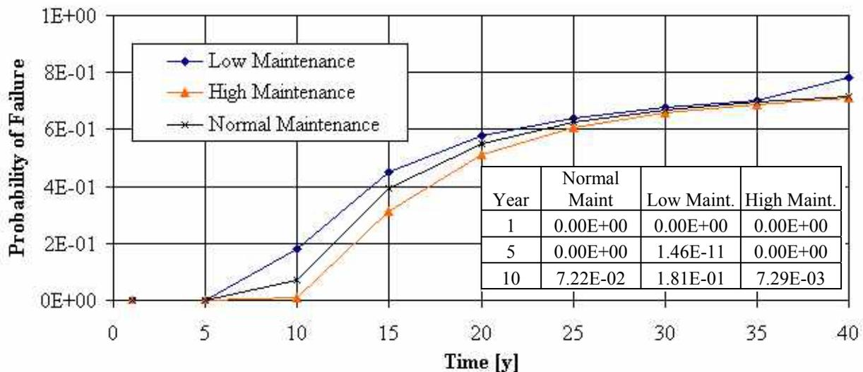
**Figure 4.28: Bulk Carrier Frame Pitting Corrosion Diminution Failure Probability**
