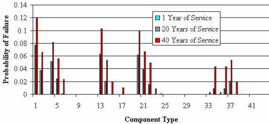
**Figure 4.44: Tanker Midship Bulkhead Frame Component Failure Probability History**
