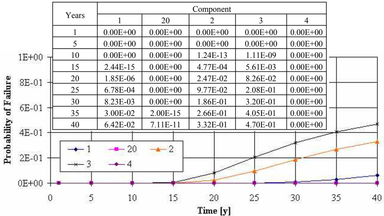
**Figure 4.21: Tanker Component Probability of Diminution Failure**
