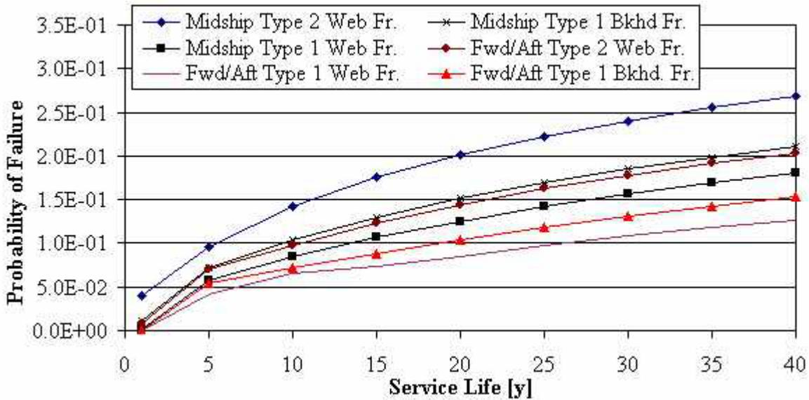
**Figure 4.26: Bulk Carrier Frame Type Time Dependant Reliability Comparison**
