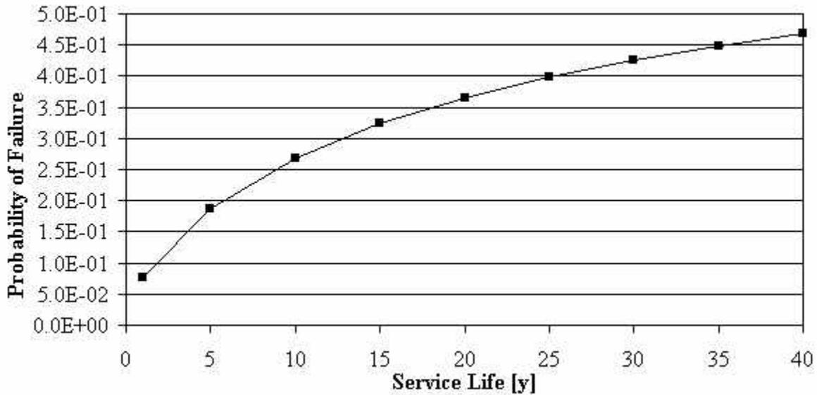
**Figure 4.38: Bulk Carrier Vessel Fatigue Initiation Failure Probability**
