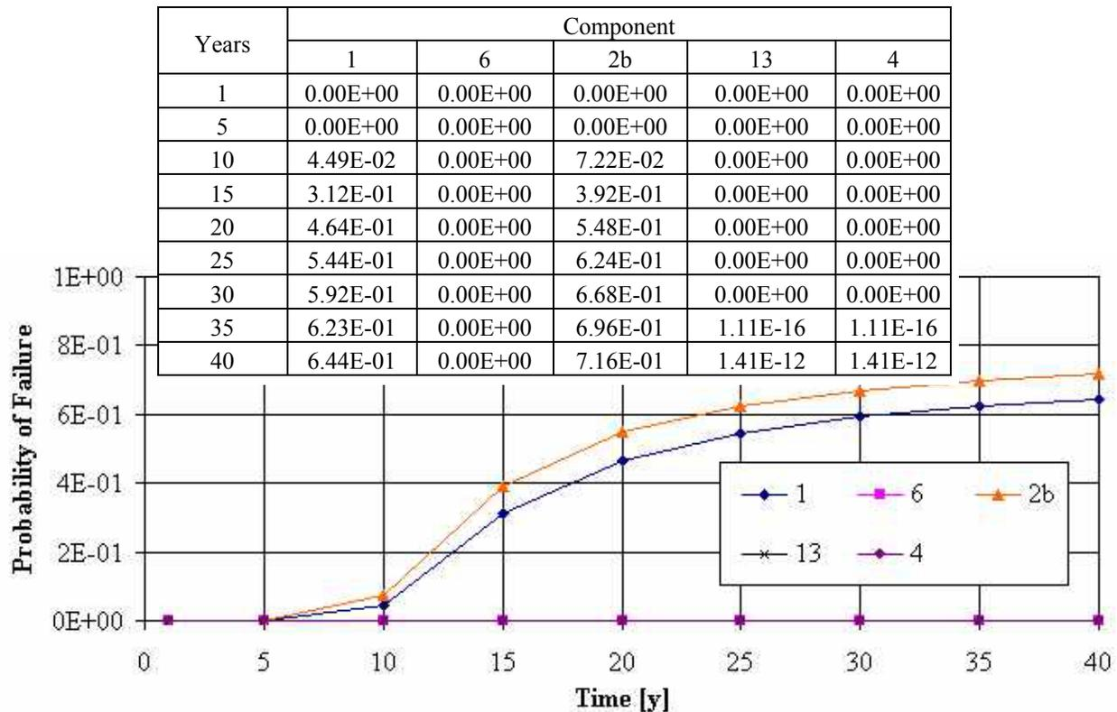
**Figure 4.15: Bulk Carrier Component Probability of Pitting Failure**
