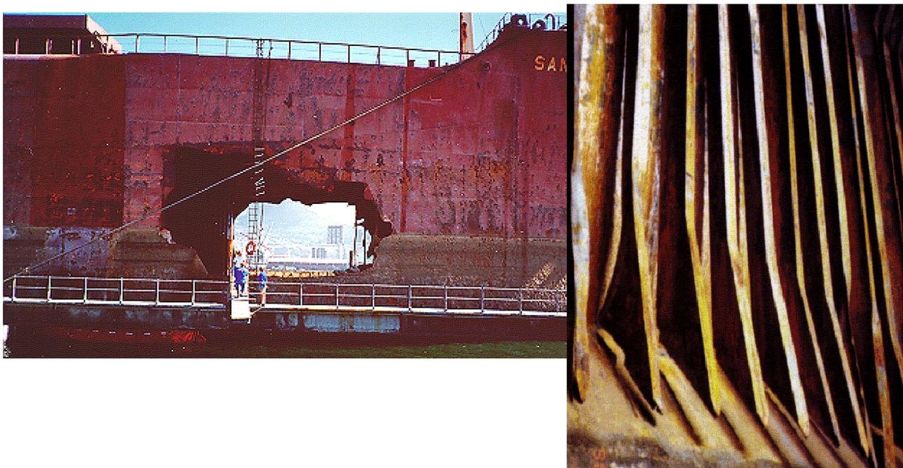
**Figure 2.2: Unchecked Structural Degradation**
