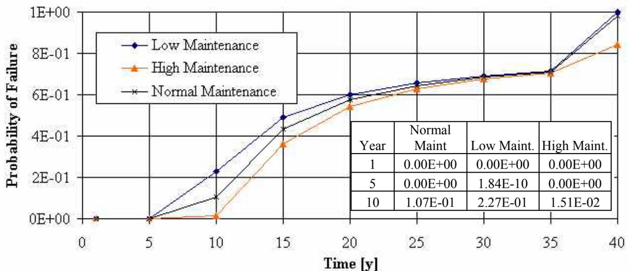
**Figure 4.30: Tanker Frame Pitting Corrosion Diminution Failure Probability**
