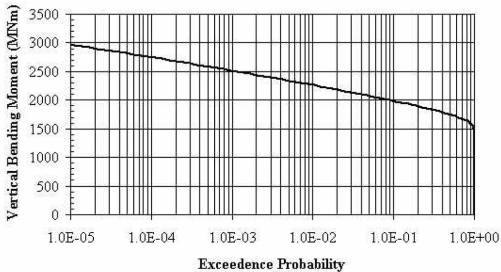
**Figure 4.9: Bulk Carrier Lifetime Midship Vertical Bending Moment Exceedance Probability (20 yrs)**
