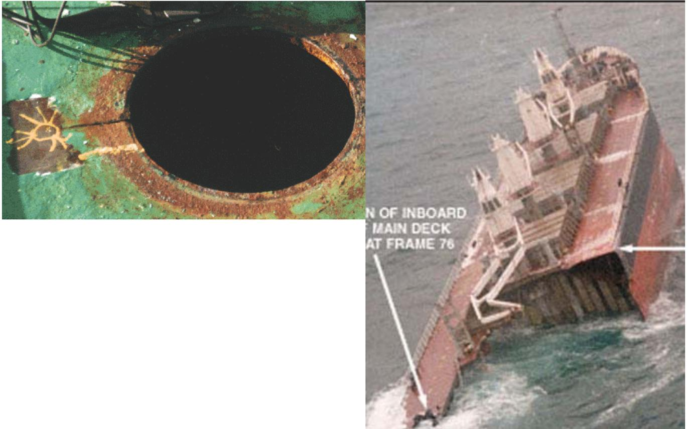
**Figure 2.3: Strength Deck Cracks Initiating at Grain Filling Ports**
