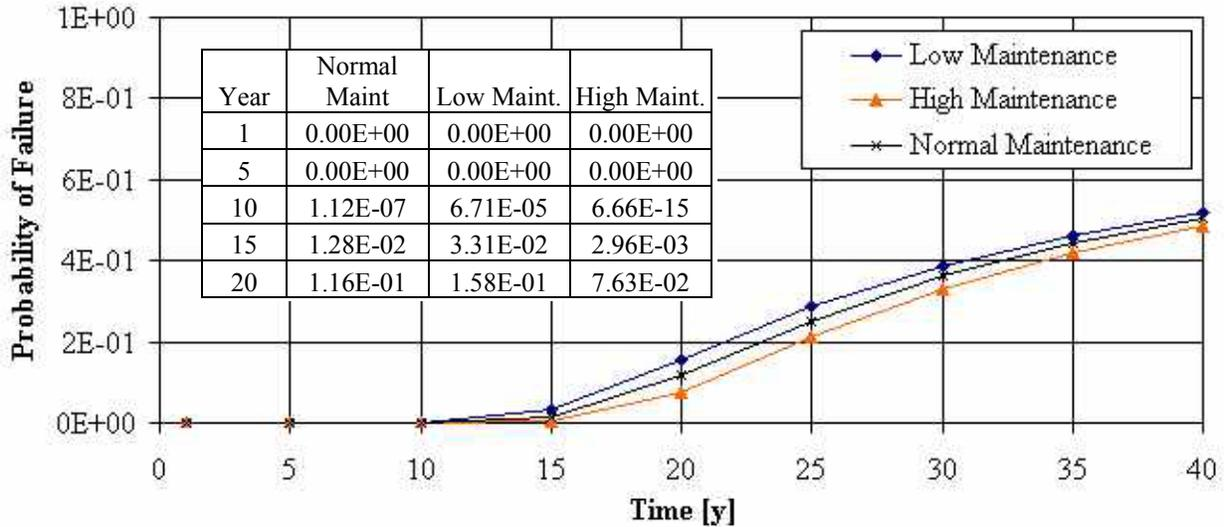
**Figure 4.29: Bulk Carrier Frame Component Corrosion Diminution Failure Probability**
