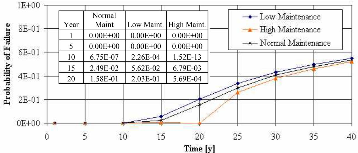
**Figure 4.31: Tanker Frame Component Corrosion Diminution Failure Probability**
