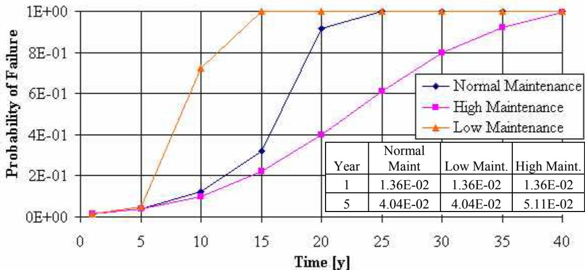
**Figure 4.35: Tanker Midship Frame Buckling and Ultimate Strength Failure Probability**
