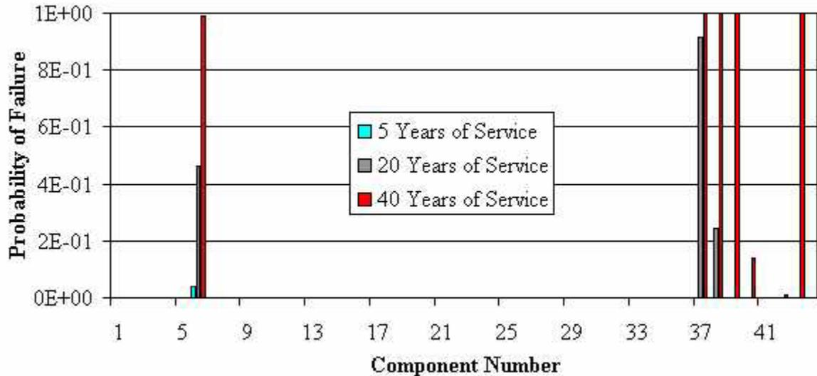
**Figure 4.42: Time History of Tanker Yield and Buckling Component Failure Probability**
