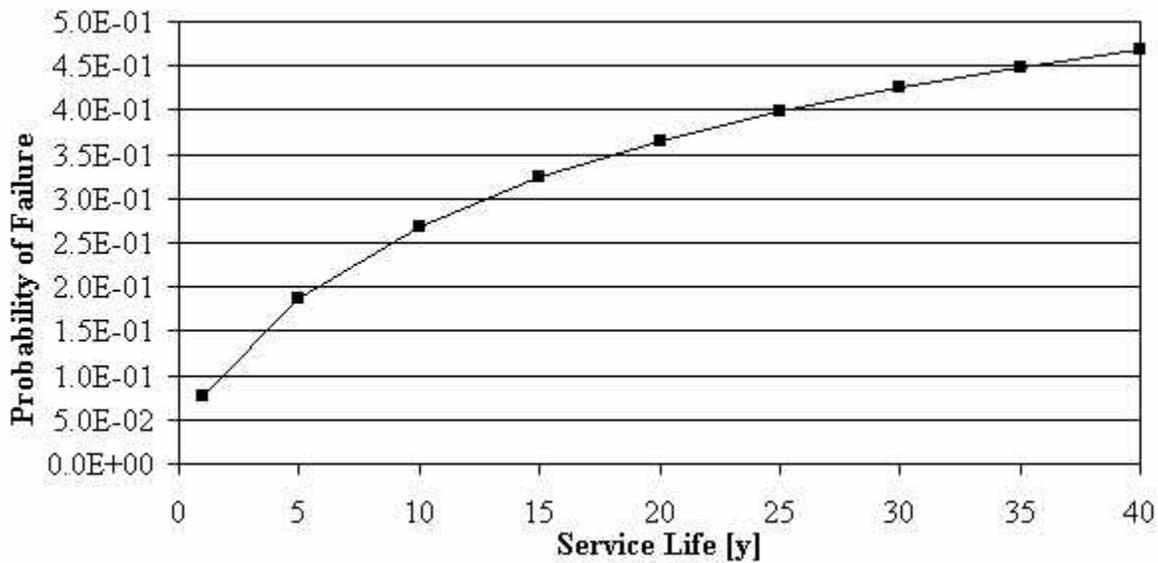
**Figure 4.38: Bulk Carrier Vessel Fatigue Initiation Failure Probability**
