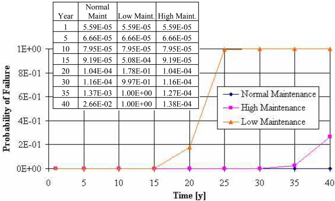
**Figure 4.32: Bulk Carrier Midship Frame Buckling and Ultimate Strength Failure Probability**
