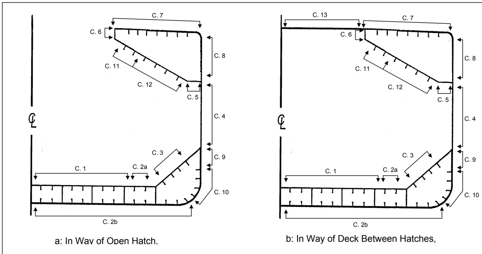
**Figure 4.4: Section View of the Bulk Carrier Describing Component Location**
