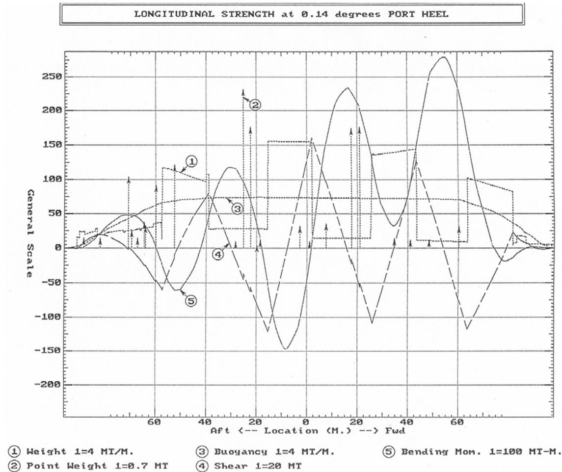
**Figure 4.7: Bulk Carrier Still Water Loads for Alternate Hold Loading Arrangement**
