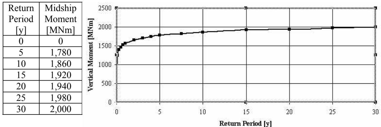
**Figure 4.10: Bulk Carrier Extreme Load Return Period**
