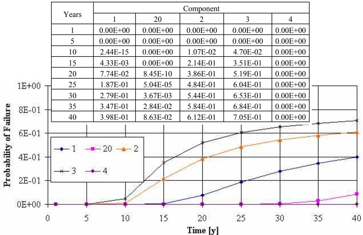
**Figure 4.20: Tanker Component Probability of Pitting Failure**
