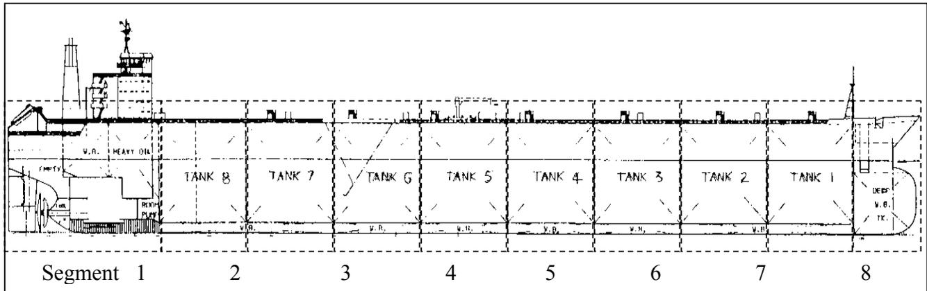
**Figure 4.5: General Arrangement of Segments in the Tanker**
