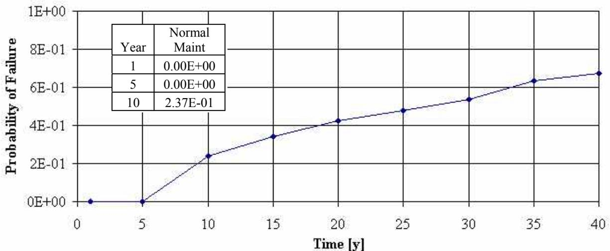
**Figure 4.22: Tanker Probability of Frame Average Diminution Failure**
