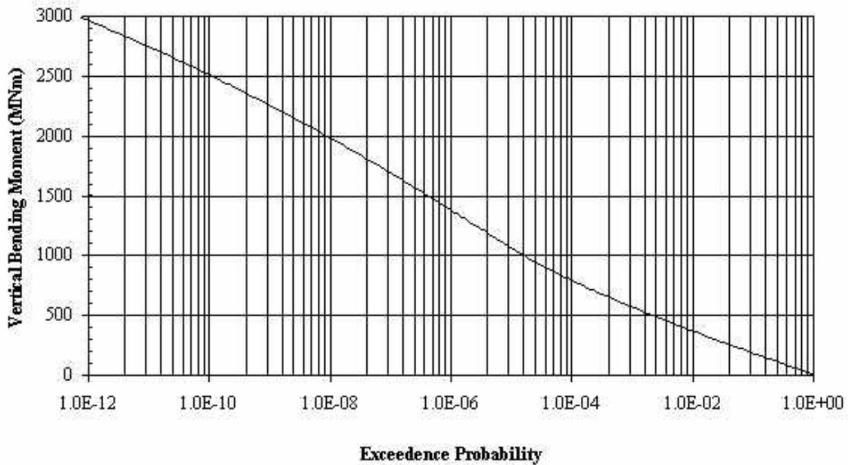
**Figure 4.8: Bulk Carrier Load Cycle Midship Vertical Bending Moment Exceedance Probability**
