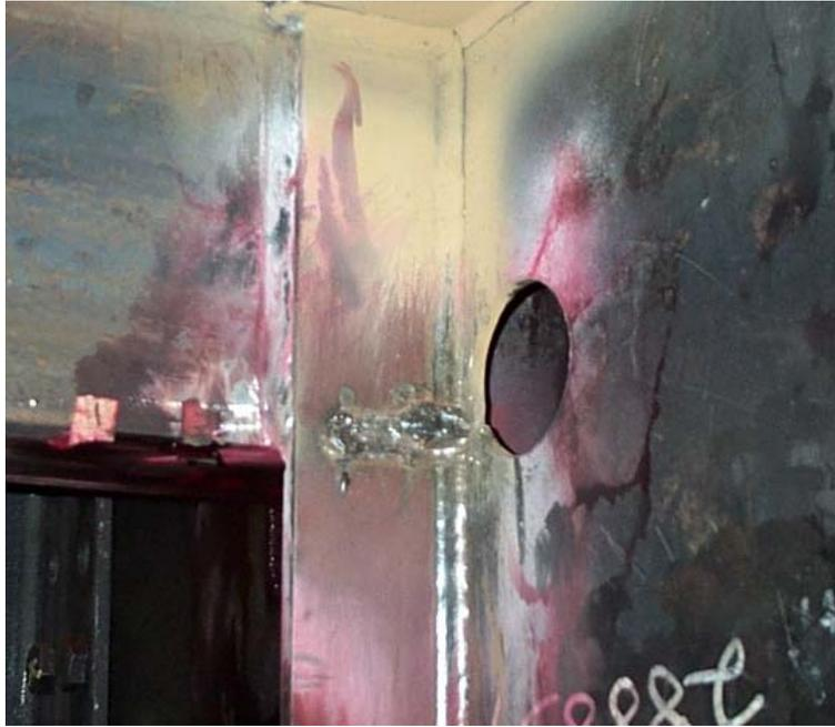
Figure 3.84: First weld repair of cracked flat bar stiffener (specimen 1)
