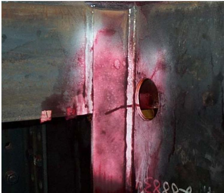
Figure 3.83: Crack propagating from stop hole into flat bar stiffener (specimen 1)
