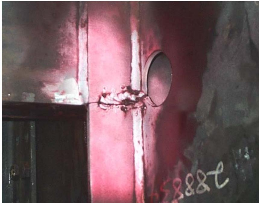
Figure 3.85: Complete failure of flat bar stiffener (specimen 1)
