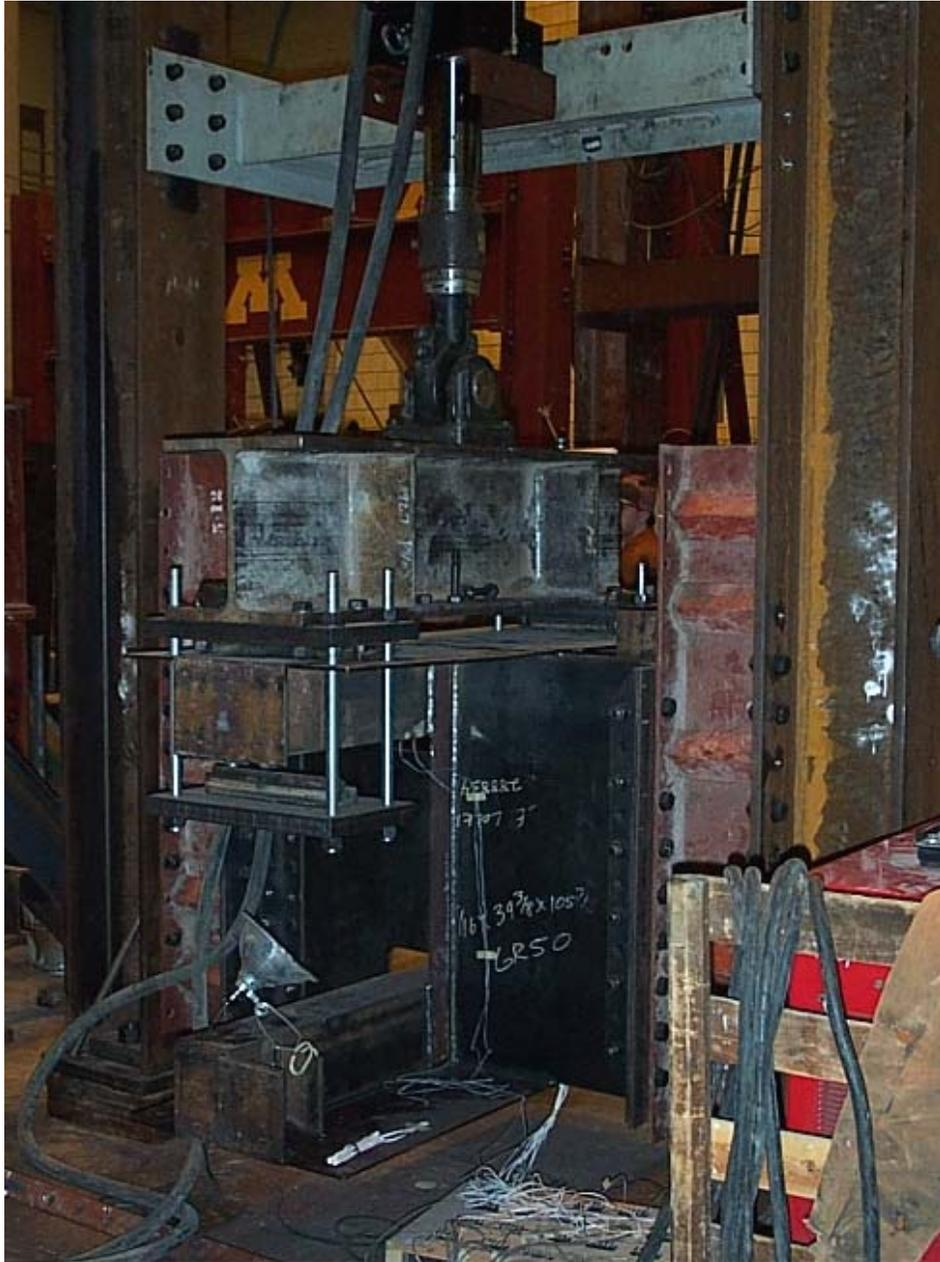
Figure 3.71 Photo of full scale web frame specimen in test fixture
