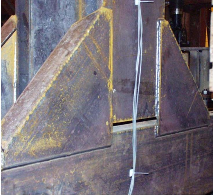
Figure 3.22: Complex-attachment brackets.
