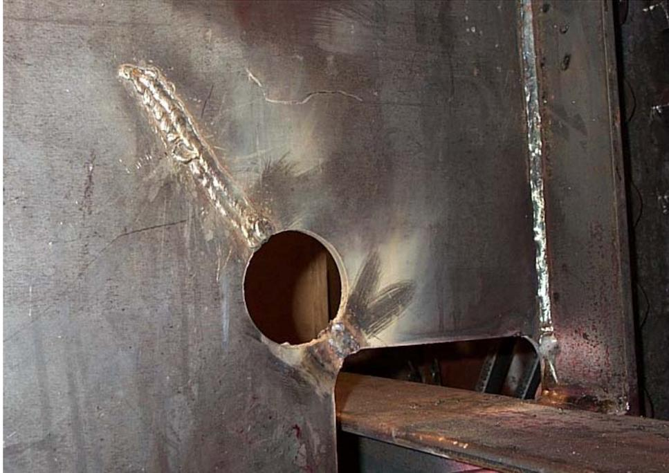
Figure 3.57 130 mm long crack after weld repairing
