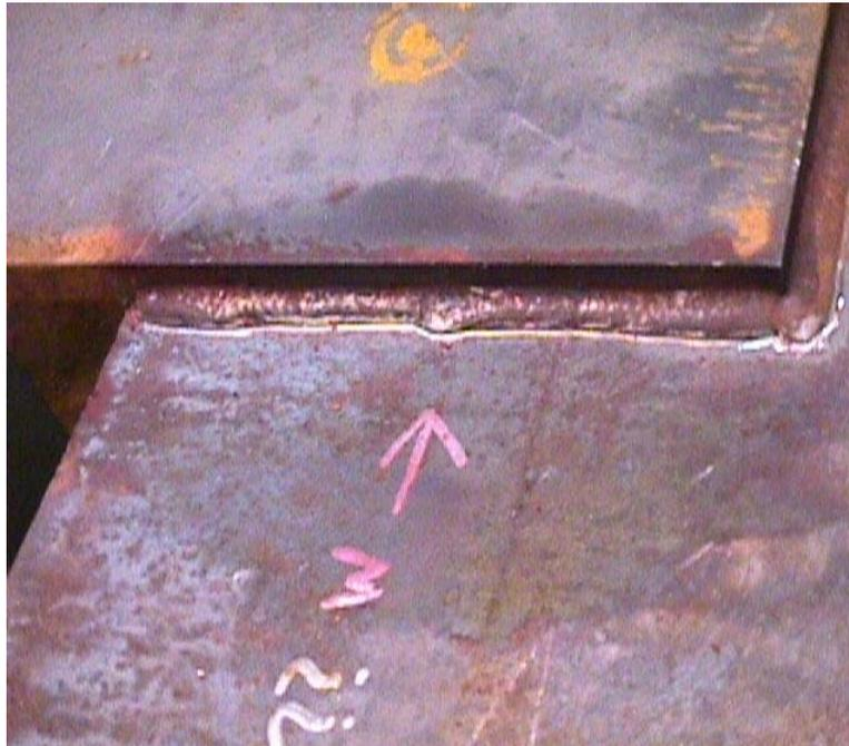
Figure 5: Peened weld that had a surface crack at fillet welded attachment
