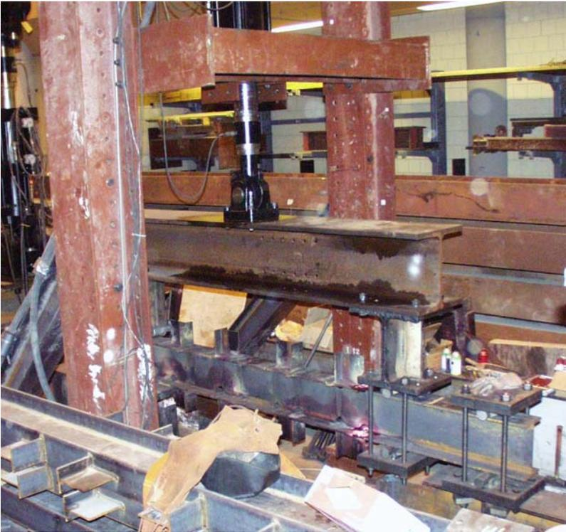
Figure 3.3: Simple-attachment specimen in test setup.
