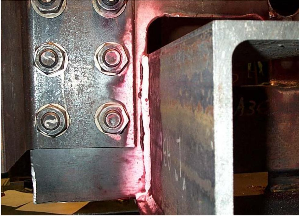
Figure 3.61 Crack forming at web frame-longitudinal connection
