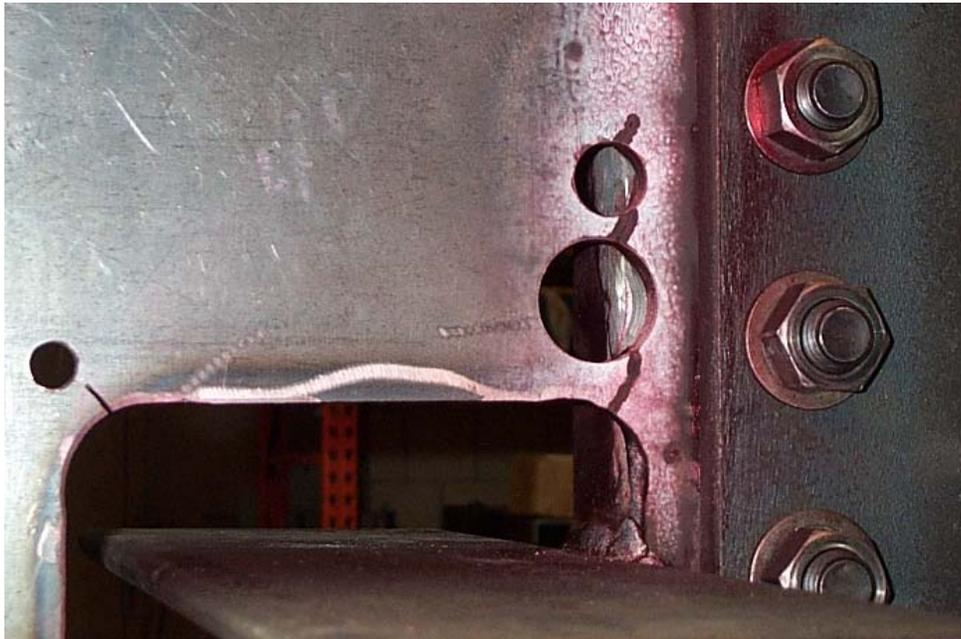
Figure 3.55 Repair failures at other radius at cutout C
