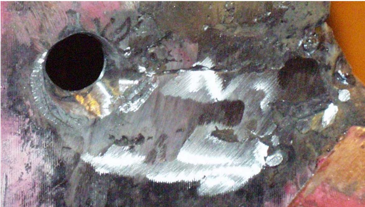
Figure 3.32: Weld repair with ground termination holes.
