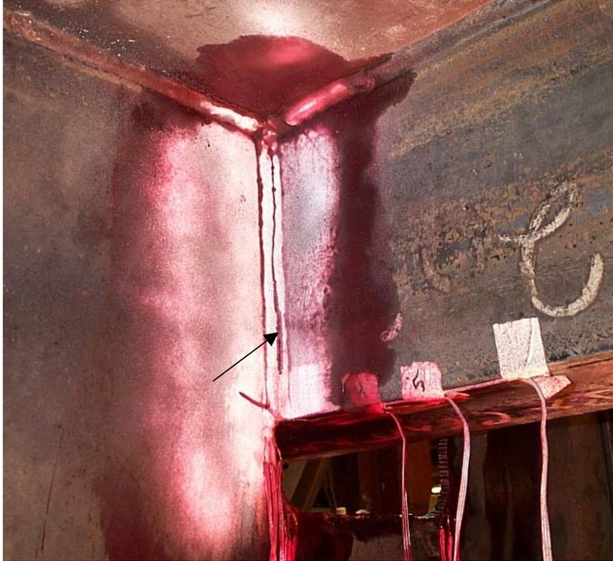
Figure 3.80: Crack along back of longitudinal at connection to web frame (specimen 1)
