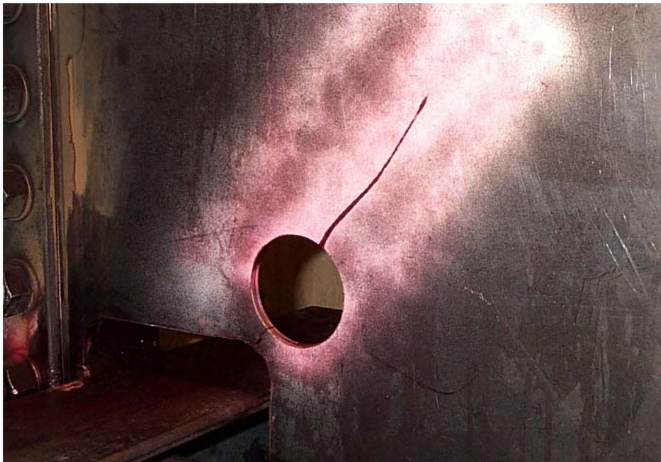
Figure 3.56 130 mm long crack after failure of 76 mm stop hole
