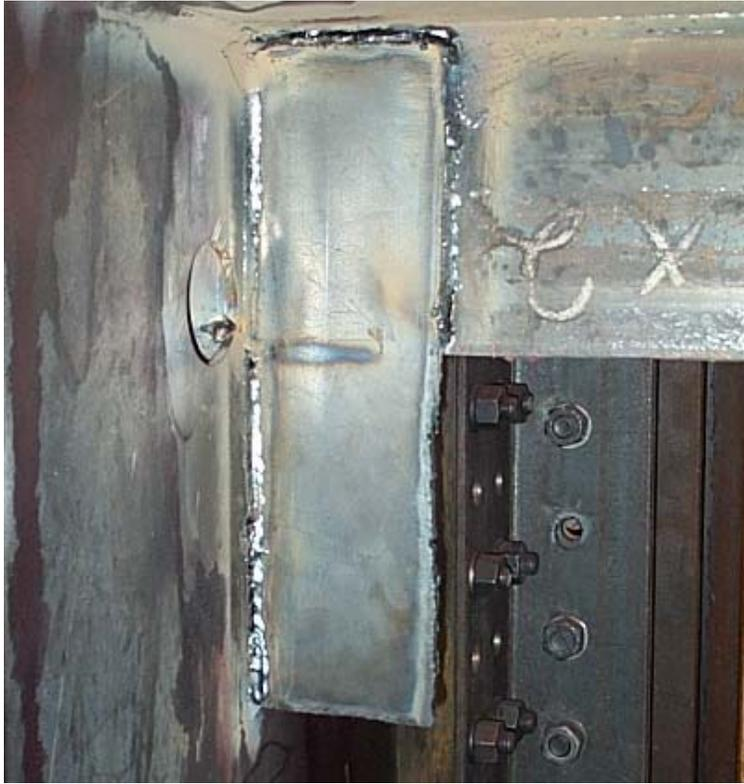
Figure 3.82: Bracket added to stiffen connection (specimen 1)
