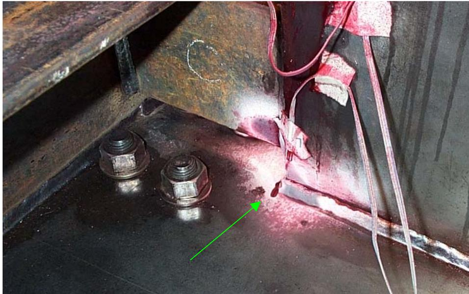
Figure 3.64 Crack forming in bottom hull at cutout
