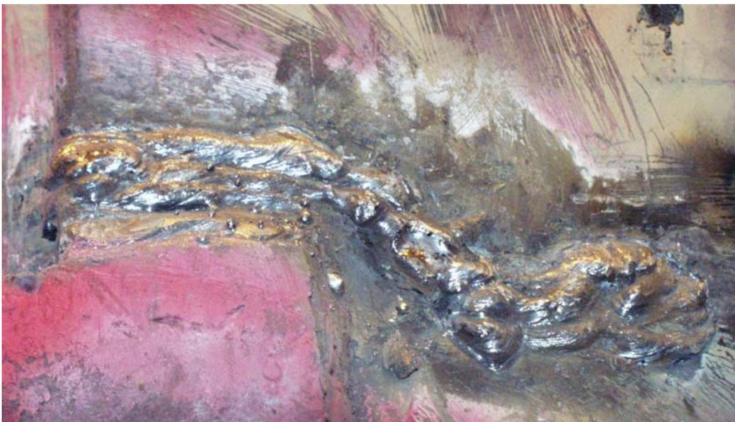
Figure 3.30: Weld repair of crack not yet through-thickness without termination holes.
