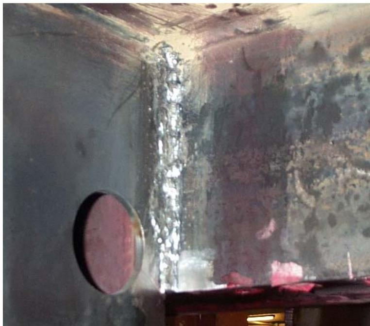
Figure 3.81: Vee-and-weld repair along back of longitudinal (specimen 1)
