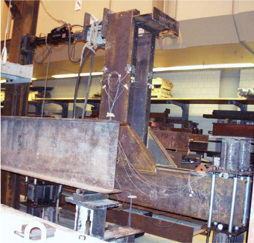
Figure 3.23: Complex-attachment test setup.
