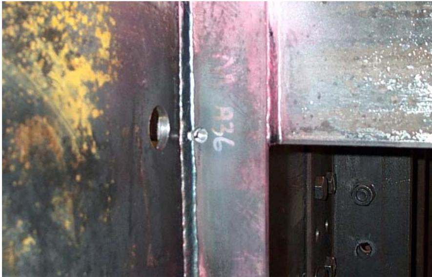
Figure 3.79: Stop hole repairs in specimen 2
