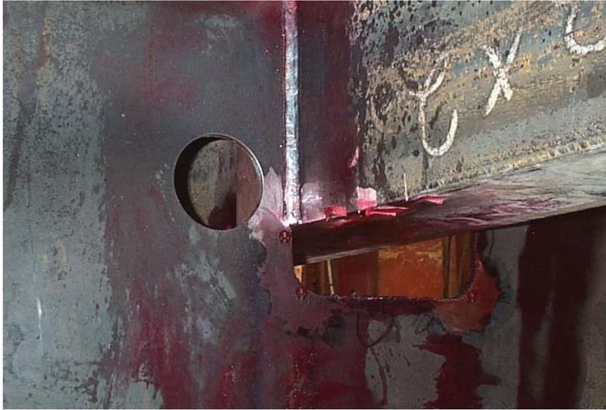
Figure 3.78: 76 mm stop hole in web frame (specimen 1)
