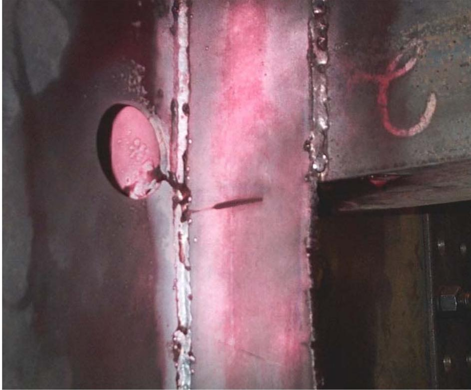
Figure 3.86: Failure of added bracket (specimen 1)
