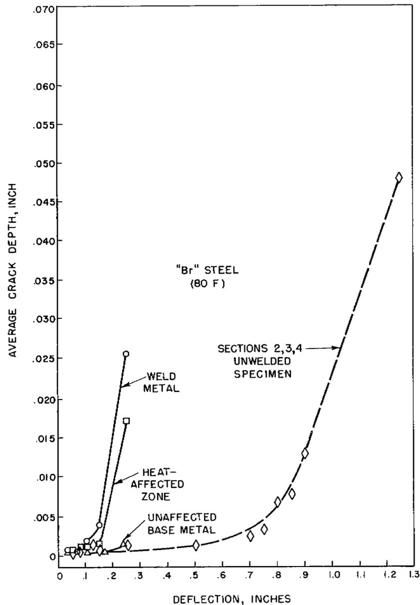
FIGURE B-7. COMPARISON OF AVERAGE CRACK DEPTH IN UNAFFECTED BASE METAL, HEAT-AFFECTED ZONE, AND WELD METAL OF WELDED "Br" STEEL KINZEL SPECIMENS, AND SECTIONS 2, 3, 4 OF UNWELDED "Br" STEEL KINZEL SPECIMENS, ALL TESTED ABOVE THE TRANSITION TEMPERATURE AT 80 F.
