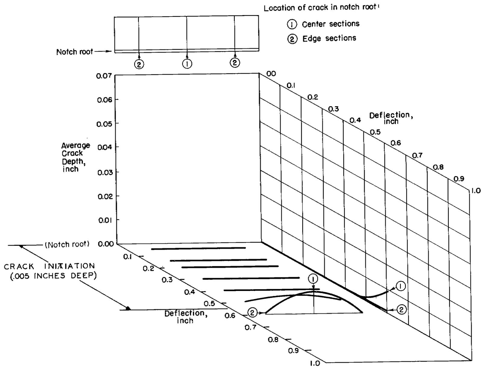
FIGURE 14B. CRACK INITIATION AND PROPAGATION IN UNWELDED "C" STEEL KINZEL-TYPE SPECIMENS TESTED AT 40F.
