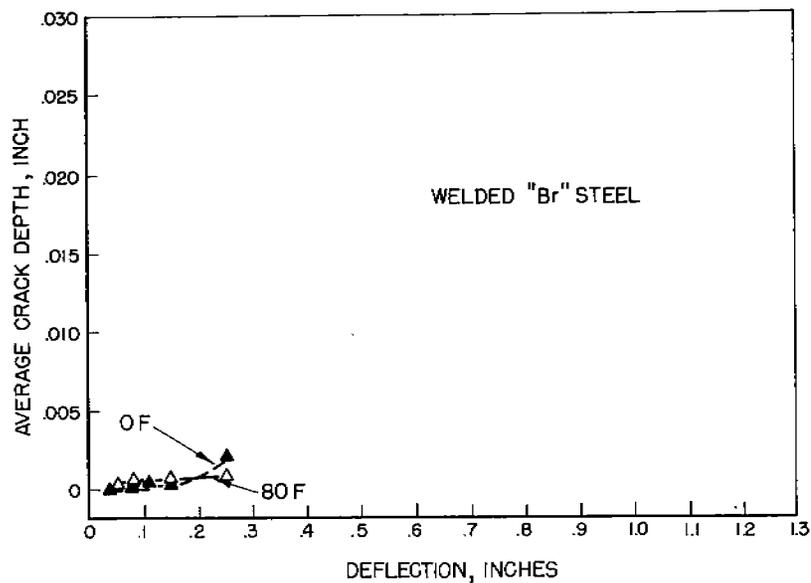
FIGURE B-6. COMPARISON OF AVERAGE CRACK DEPTH IN UNAFFECTED BASE METAL OF WELDED "Br" STEEL KINZEL SPECIMENS TESTED ABOVE (80 F) AND BELOW (0 F) THE TRANSITION TEMPERATURE.
