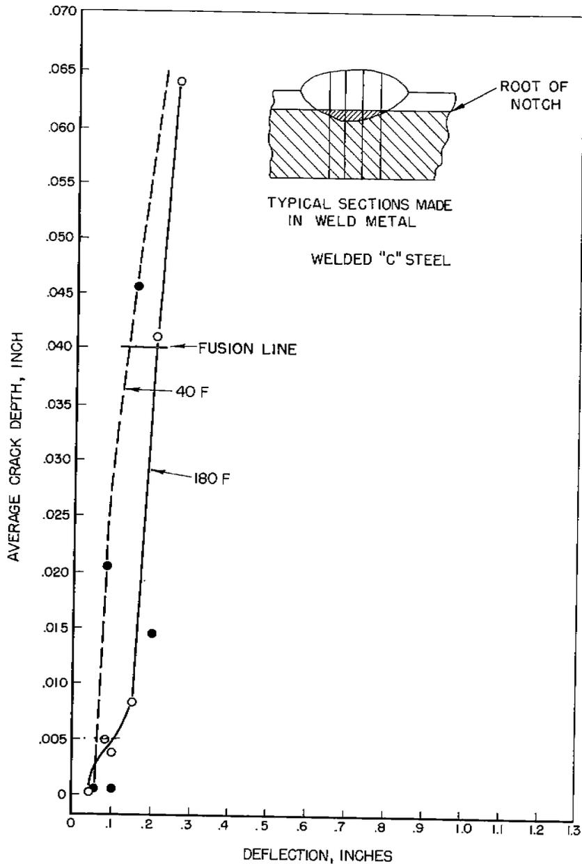
FIGURE B-4. COMPARISON OF AVERAGE CRACK DEPTH IN WELD-METAL ZONE OF WELDED "C" STEEL KINZEL SPECIMENS TESTED ABOVE (180 F) AND BELOW (40 F) THE TRANSITION TEMPERATURE.
