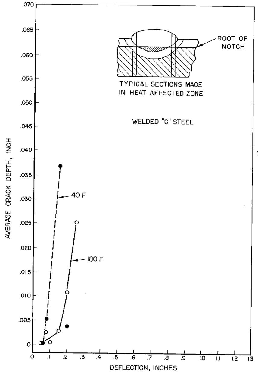
FIGURE B-5. COMPARISON OF AVERAGE CRACK DEPTH IN HEAT-AFFECTED ZONE OF WELDED "C" STEEL KINZEL SPECIMENS TESTED ABOVE (180 F) AND BELOW (40 F) THE TRANSITION TEMPERATURE.
