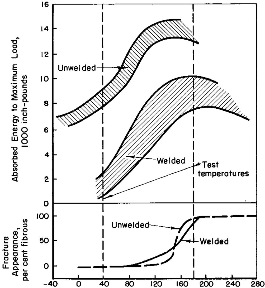
FIGURE 3. ABSORBED ENERGY AND FRACTURE APPEARANCE CURVES FOR WELDED AND UNWELDED "C" STEEL KINZEL-TYPE SPECIMENS, SHOWING TEST TEMPERATURES USED IN FRACTURE STUDIES.<sup>12</sup>
