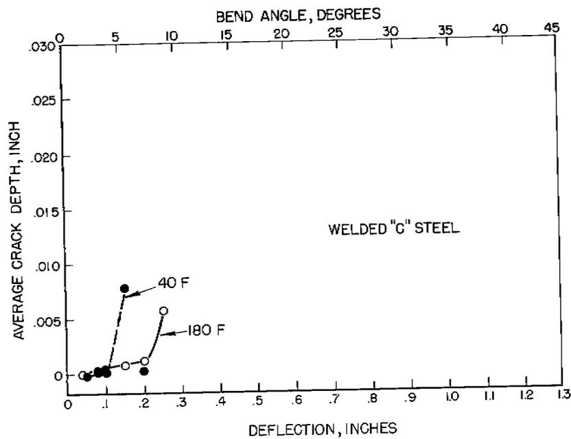
FIGURE B16. COMPARISON OF AVERAGE CRACK DEPTH IN UNAFFECTED BASE-METAL ZONE OF WELDED "C" STEEL KINZEL SPECIMENS TESTED ABOVE (180 F) AND BELOW (40 F) THE TRANSITION TEMPERATURE.
