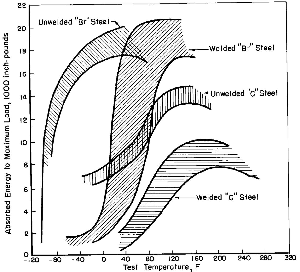
FIGURE 23. ABSORBED ENERGY DATA FOR WELDED AND UNWELDED KINZEL-TYPE SPECIMENS OF "Br" AND "C" STEEL <sup>12</sup>
