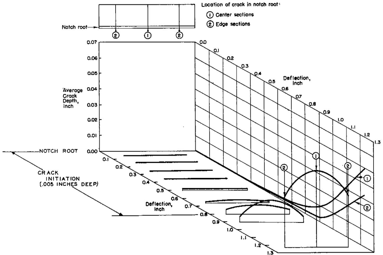
FIGURE 12 B. CRACK INITIATION AND PROPAGATION IN UNWELDED "Br" STEEL KINZEL-TYPE SPECIMENS. CURVES ARE SIMILAR FOR SPECIMENS TESTED AT 80 F AND 0 F
