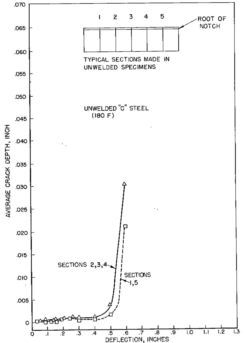
FIGURE B9. COMPARISON OF AVERAGE CRACK DEPTH OF SECTIONS 2,3,4 AND SECTIONS 1,5 OF UNWELDED "C" STEEL KINZEL SPECIMENS TESTED ABOVE THE TRANSITION TEMPERATURE AT 180 F.
