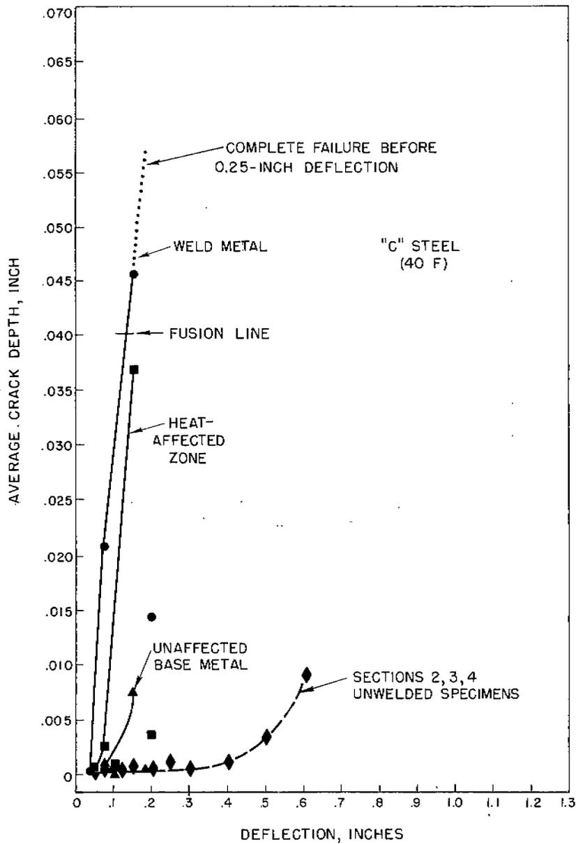
FIGURE B-12. COMPARISON OF AVERAGE CRACK DEPTH OF WELD METAL, HEAT-AFFECTED ZONE, AND UNAFFECTED BASE METAL OF WELDED "C" STEEL KINZEL SPECIMENS, AND SECTIONS 2, 3, 4 OF UNWELDED "C" STEEL KINZEL SPECIMENS, ALL TESTED BELOW THE TRANSITION TEMPERATURE AT 40 F.
