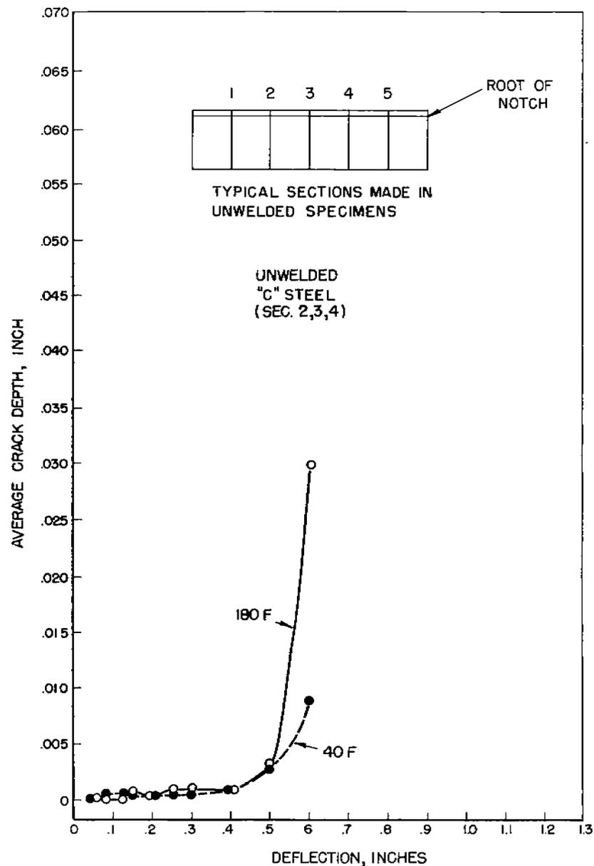
FIGURE B11. COMPARISON OF AVERAGE CRACK DEPTH OF SECTIONS 2, 3, 4 OF UNWELDED "C" STEEL KINZEL SPECIMENS TESTED ABOVE (180 F) AND BELOW (40 F) THE TRANSITION TEMPERATURE.
