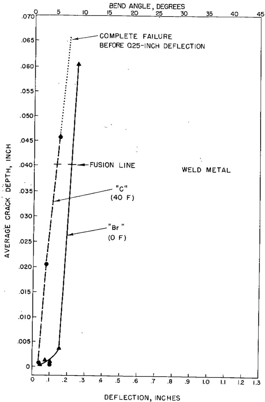
FIGURE B-20. COMPARISON OF AVERAGE CRACK DEPTH IN WELD METAL OF WELDED "Br" AND "C" STEEL KINZEL SPECIMENS TESTED BELOW THEIR TRANSITION TEMPERATURES.
