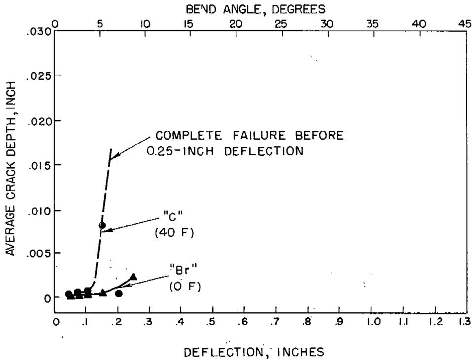
FIGURE B-24. COMPARISON OF AVERAGE CRACK DEPTH IN UNAFFECTED BASE METAL OF WELDED "Br" AND "C" STEEL KINZEL SPECIMENS TESTED BELOW THEIR TRANSITION TEMPERATURES.
