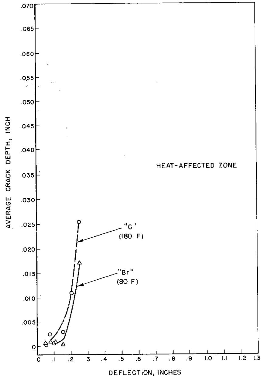
FIGURE B-21. COMPARISON OF AVERAGE CRACK DEPTH IN HEAT-AFFECTED ZONE OF WELDED "Br" AND "C" STEEL KINZEL SPECIMENS TESTED ABOVE THE TRANSITION TEMPERATURE.
