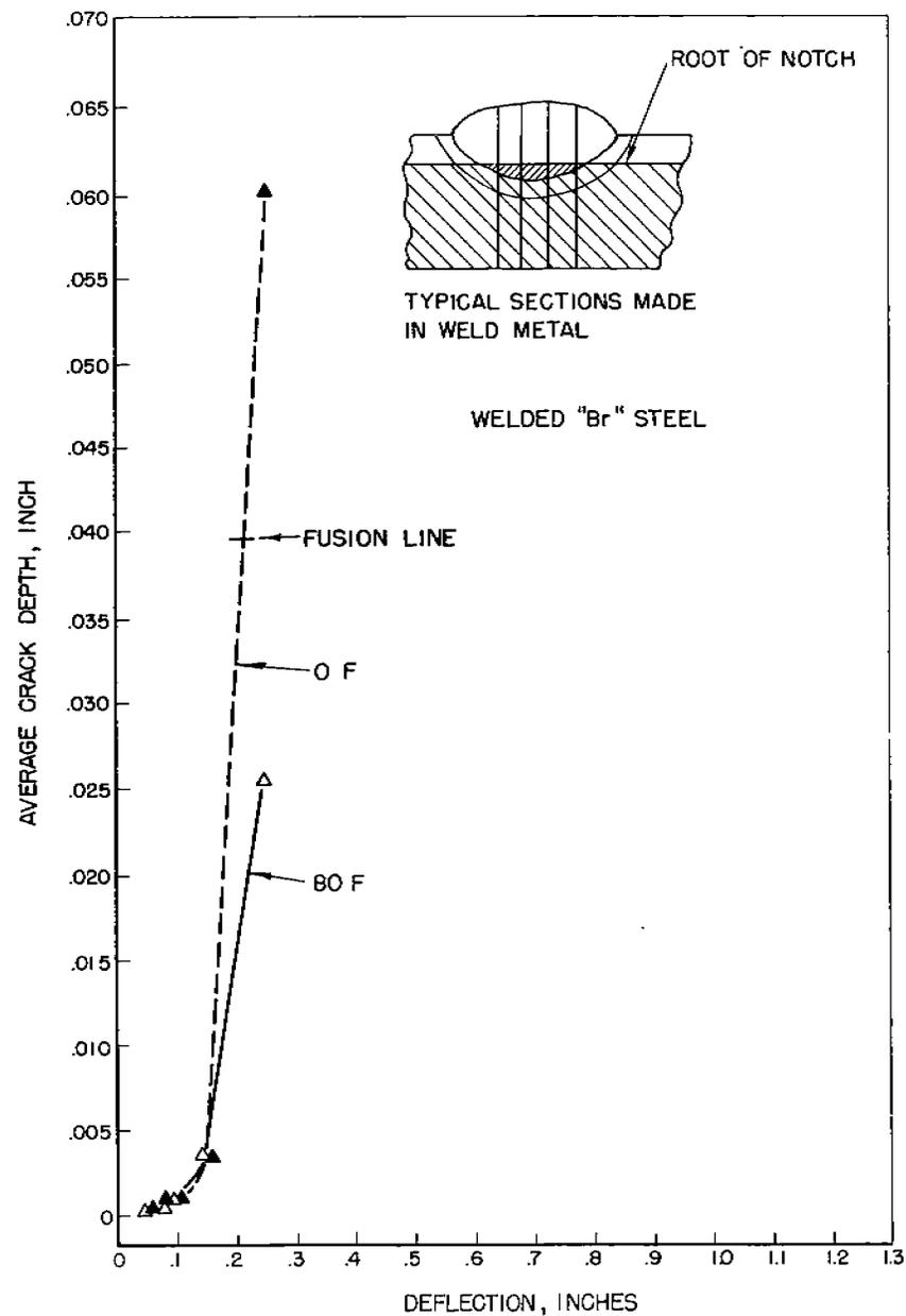
FIGURE B4. COMPARISON OF AVERAGE CRACK DEPTH IN WELD-METAL ZONE OF WELDED "Br" STEEL KINZEL SPECIMENS TESTED ABOVE (80 F) AND BELOW (0 F) THE TRANSITION TEMPERATURE.
