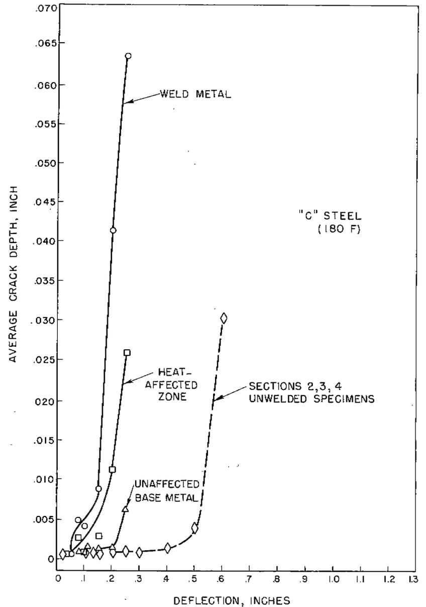
FIGURE B-13. COMPARISON OF AVERAGE CRACK DEPTH OF WELD METAL, HEAT-AFFECTED ZONE, AND UNAFFECTED BASE METAL OF WELDED "C" STEEL KINZEL SPECIMENS, AND SECTIONS 2, 3, 4 OF UNWELDED "C" STEEL KINZEL SPECIMENS, ALL TESTED ABOVE THE TRANSITION TEMPERATURE AT 180 F.
