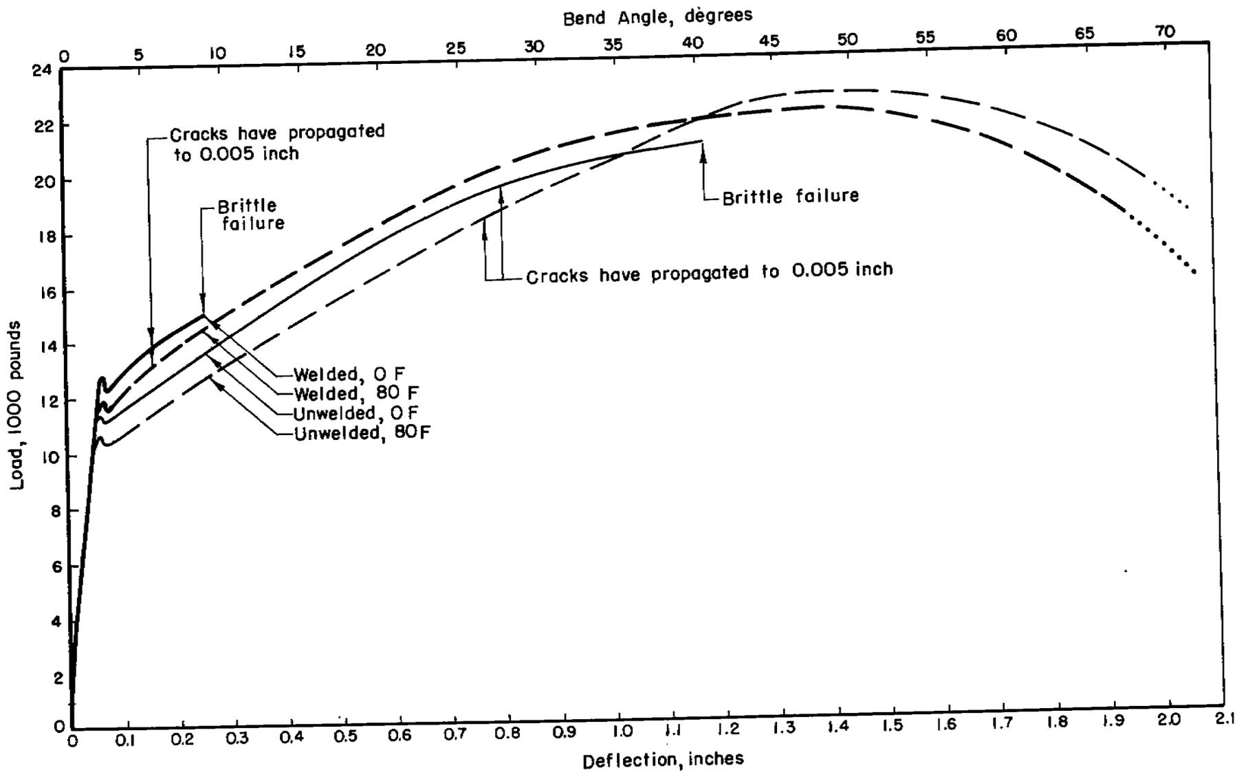
FIGURE 24. AVERAGE LOAD-DEFLECTION CURVES FOR WELDED AND UNWELDED "Br" STEEL KINZEL-TYPE SPECIMENS TESTED AT VARIOUS TEMPERATURES.
