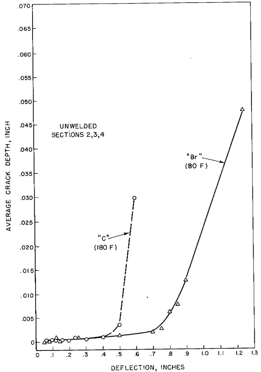
FIGURE B17. COMPARISON OF AVERAGE CRACK DEPTH IN SECTIONS 2,3,4 OF UNWELDED "Br" AND "C" STEEL KINZEL SPECIMENS TESTED ABOVE THEIR TRANSITION TEMPERATURES.
