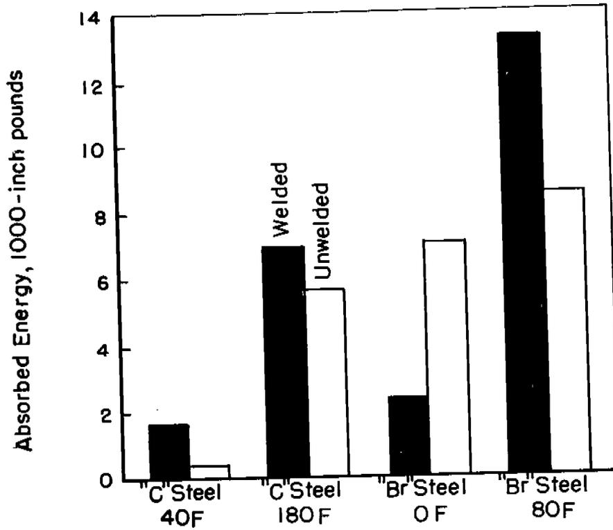
FIGURE 27. ENERGY AFTER CRACKING ABSORBED BY WELDED AND UNWELDED KINZEL-TYPE SPECIMENS OF "Br" AND "C" STEELS.
