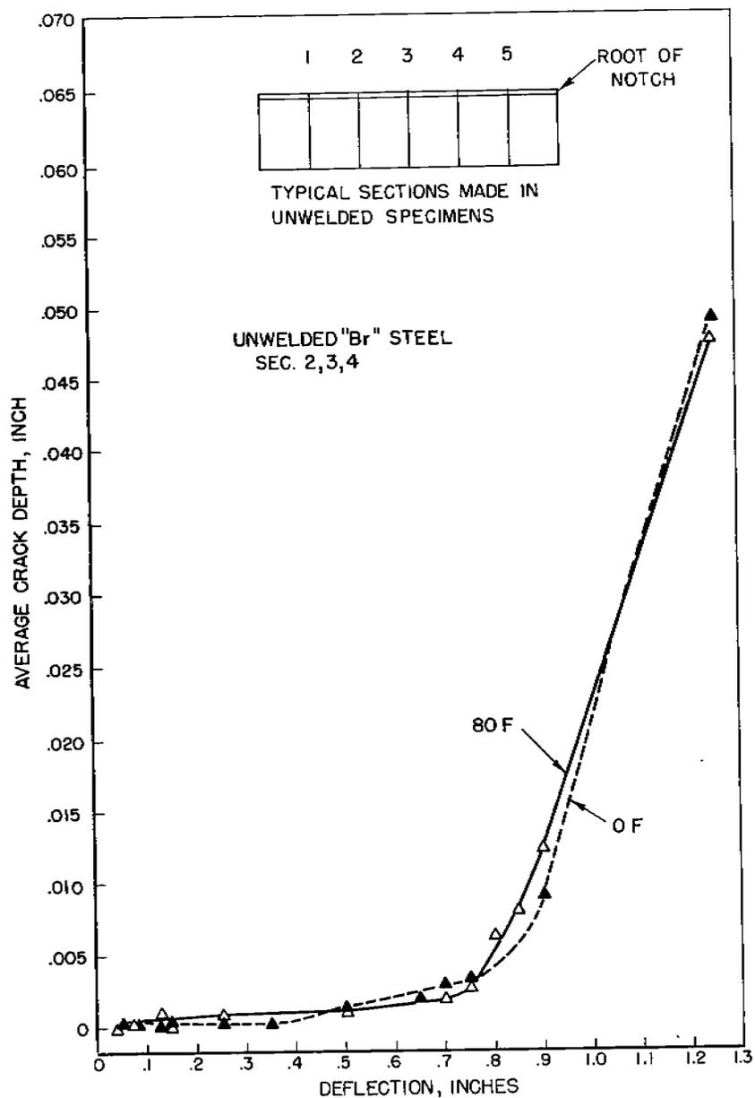
FIGURE B3. COMPARISON OF AVERAGE CRACK DEPTH IN SECTIONS 2, 3, 4 OF UNWELDED "Br" STEEL KINZEL SPECIMENS TESTED AT 80 F AND 0 F.
