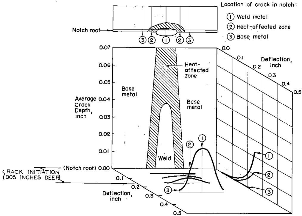
FIGURE 13. CRACK INITIATION AND PROPAGATION IN WELDED "B" STEEL KINZEL-TYPE SPECIMENS TESTED AT 80F.
