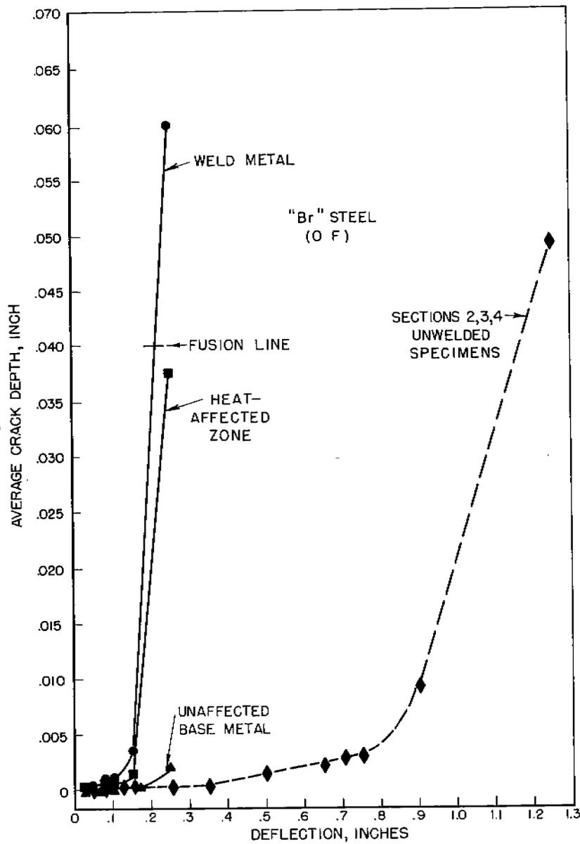
FIGURE B8. COMPARISON OF AVERAGE CRACK DEPTH IN UNAFFECTED BASE METAL, HEAT-AFFECTED ZONE, AND WELD METAL OF WELDED "Br" STEEL KINZEL SPECIMENS, AND SECTIONS 2, 3, 4 OF UNWELDED "Br" STEEL KINZEL SPECIMENS, ALL TESTED AT 0 F.
