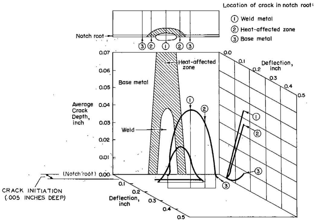
FIGURE 14A. CRACK INITIATION AND PROPAGATION IN WELDED "C" STEEL KINZEL-TYPE SPECIMENS TESTED AT 40F.
