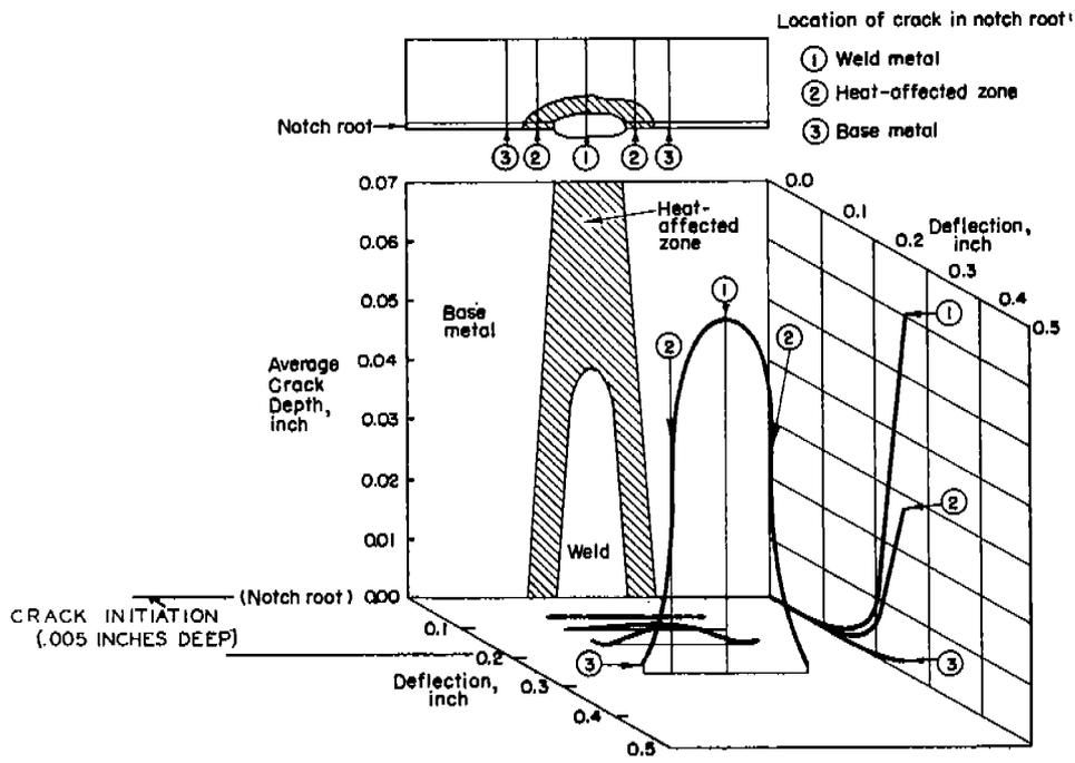
FIG. 12 A. CRACK INITIATION AND PROPAGATION IN WELDED "Br" STEEL KINZEL-TYPE SPECIMENS TESTED AT 0 F
