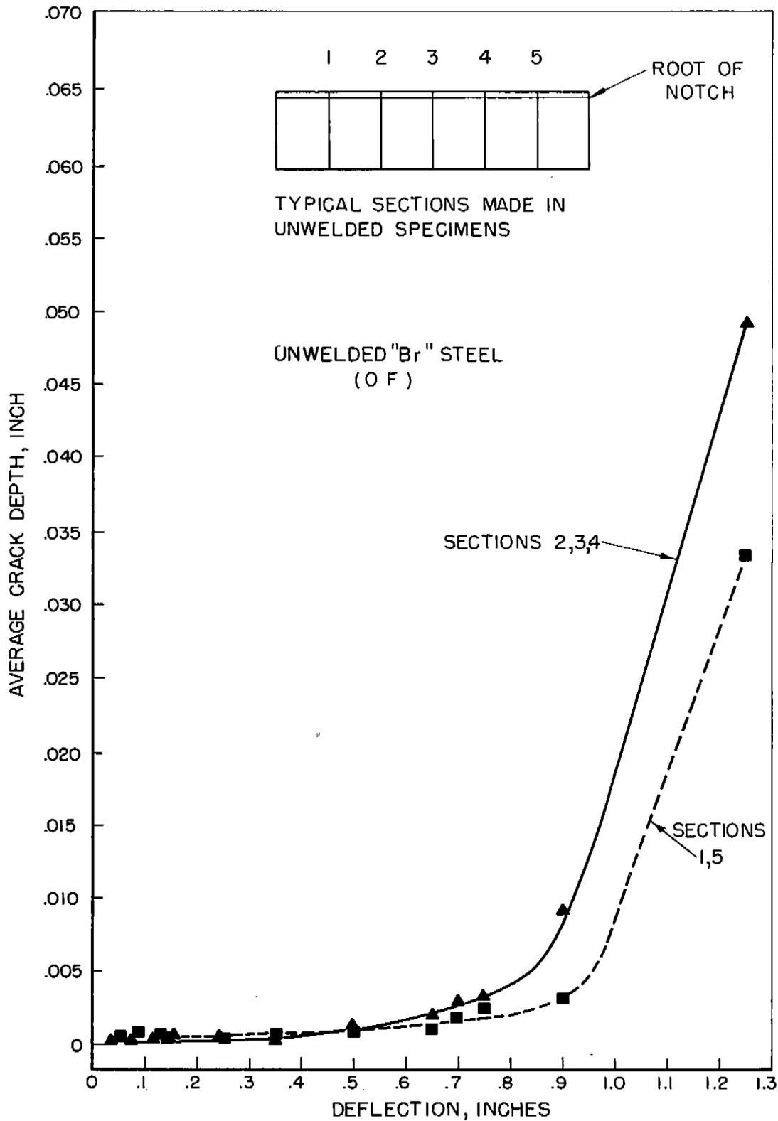
FIGURE B-2. COMPARISON OF AVERAGE CRACK DEPTH IN SECTIONS 2,3,4 AND SECTIONS 1,5 OF UNWELDED "Br" STEEL KINZEL SPECIMENS TESTED AT O F.
