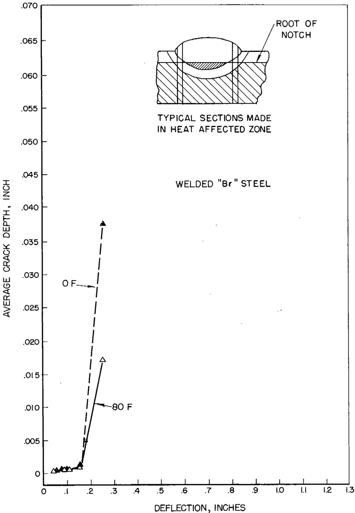
FIGURE B-5. COMPARISON OF AVERAGE CRACK DEPTH OF HEAT-AFFECTED ZONE OF WELDED "Br" STEEL KINZEL SPECIMENS TESTED ABOVE (80 F) AND BELOW (0 F) THE TRANSITION TEMPERATURE.
