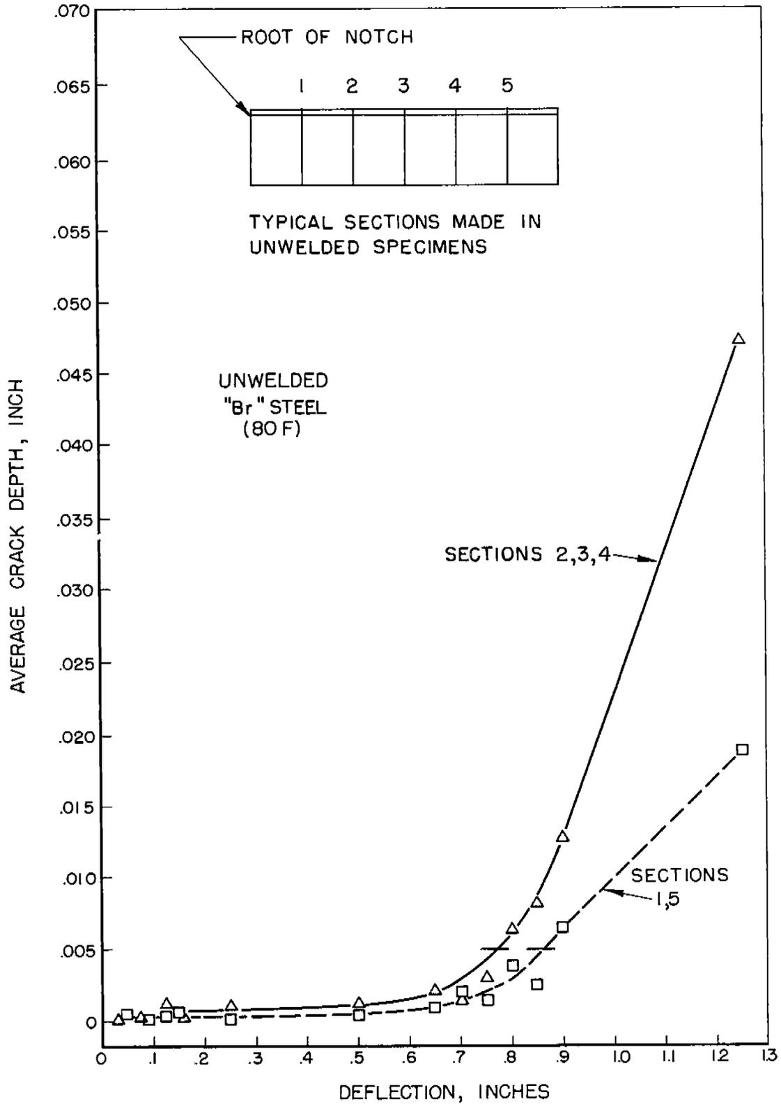
FIGURE B1. COMPARISON OF AVERAGE CRACK DEPTH IN SECTIONS 2, 3, 4, AND SECTIONS 1, 5 OF UNWELDED "Br" STEEL KINZEL SPECIMENS TESTED ABOVE THE TRANSITION TEMPERATURE AT 80 F.
