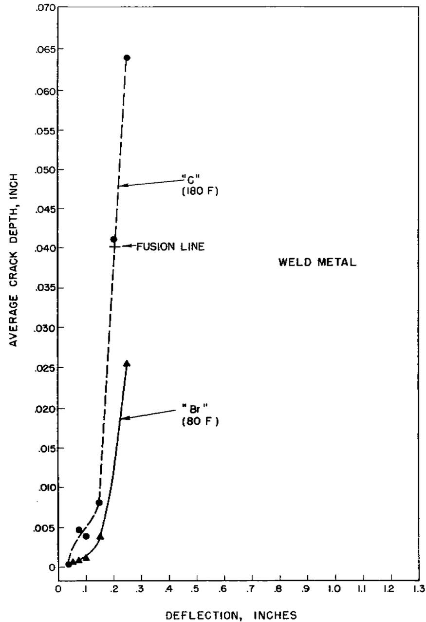
FIGURE B-19. COMPARISON OF AVERAGE CRACK DEPTH IN WELD METAL OF WELDED "Br" AND "C" STEEL SPECIMENS TESTED ABOVE THEIR TRANSITION TEMPERATURES.
