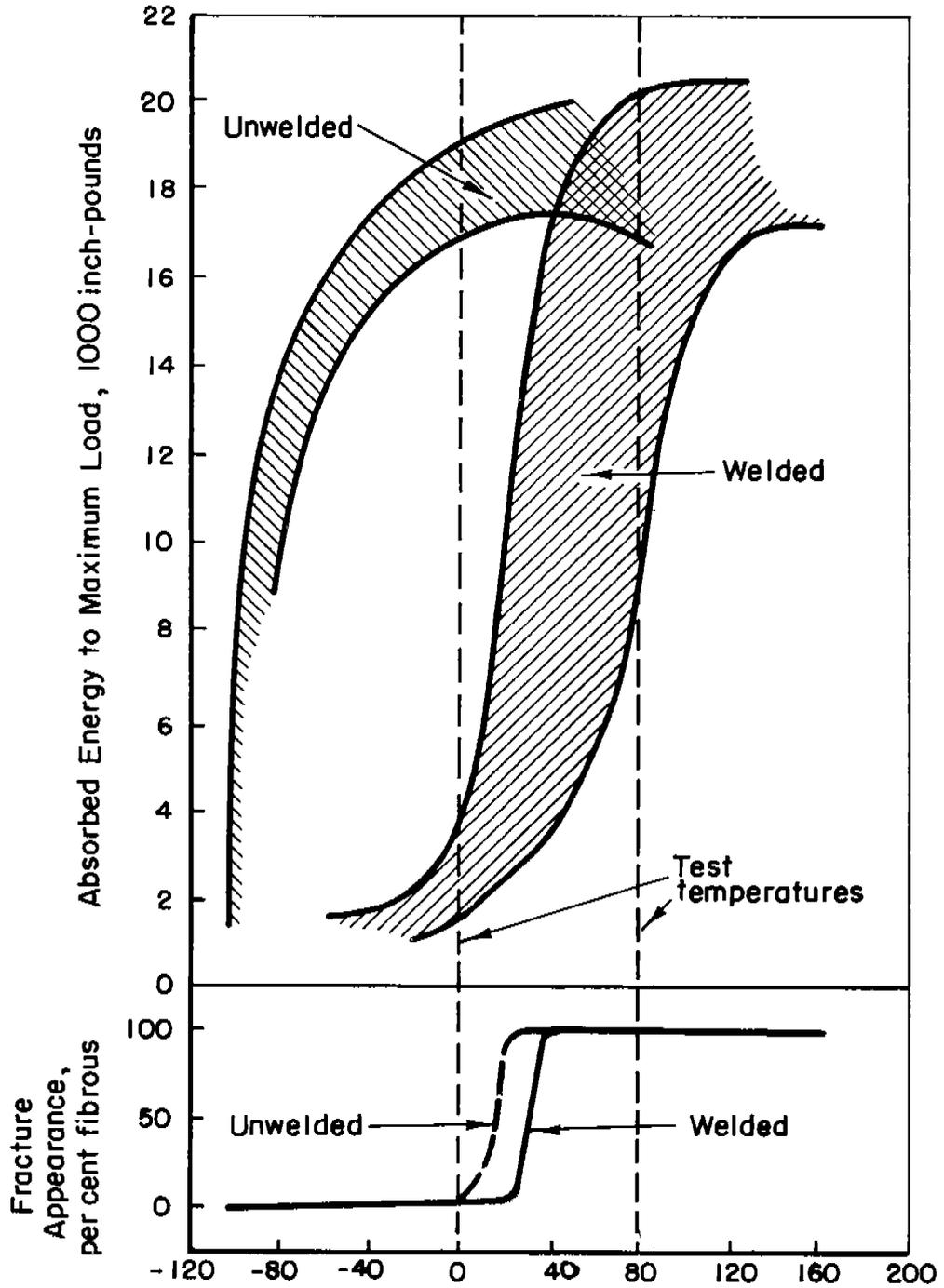
FIGURE 2. ABSORBED ENERGY AND FRACTURE APPEARANCE CURVES FOR WELDED AND UNWELDED "Br" STEEL KINZEL-TYPE SPECIMENS, SHOWING TEST TEMPERATURES USED IN FRACTURE STUDIES.<sup>12</sup>
