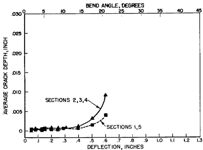
FIGURE B10. COMPARISON OF AVERAGE CRACK DEPTH OF SECTIONS 2,3,4 AND SECTIONS 1,5 OF UNWELDED "C" STEEL KINZEL SPECIMENS TESTED BELOW THE TRANSITION TEMPERATURE AT 40 F.
