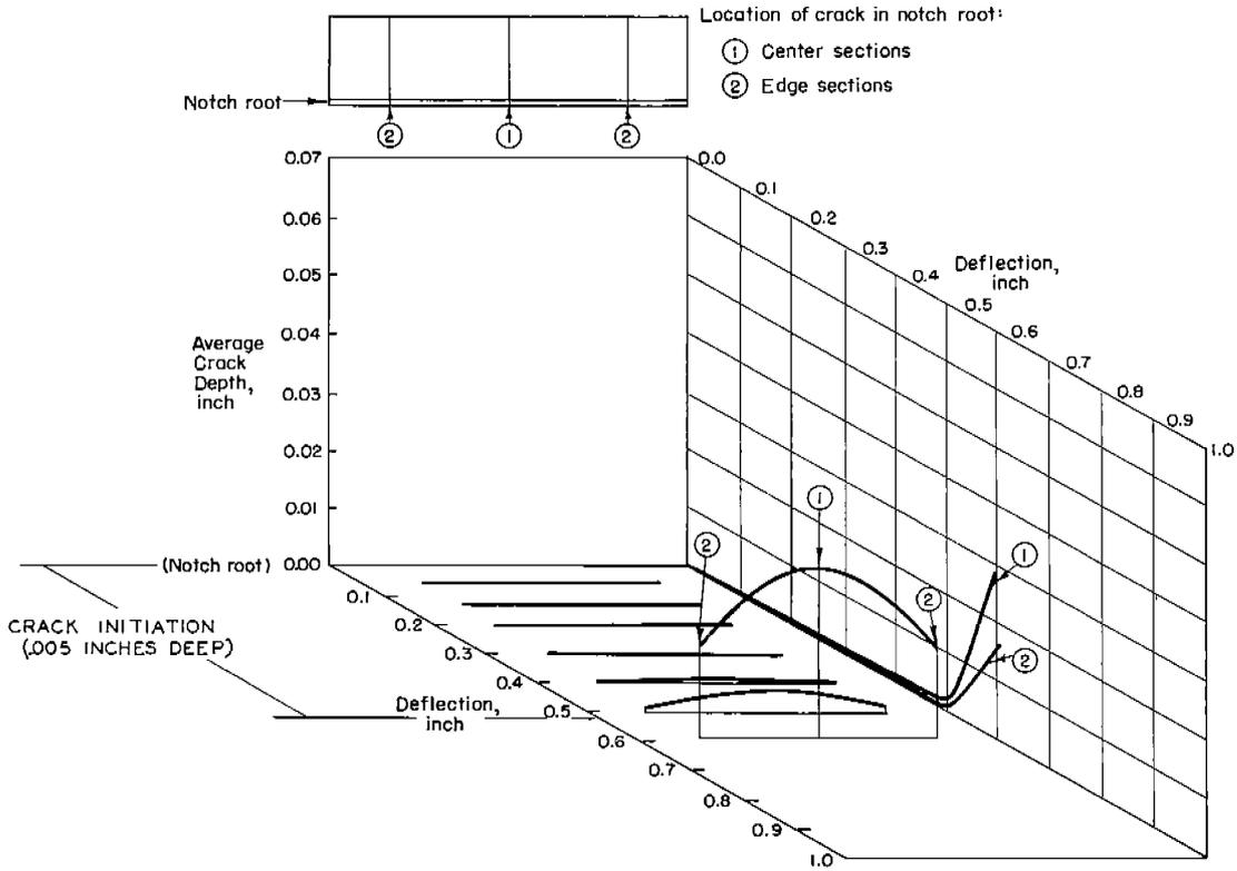
FIGURE 15B. CRACK INITIATION AND PROPAGATION IN UNWELDED "C" STEEL KINZEL-TYPE SPECIMENS TESTED AT 180 F.
