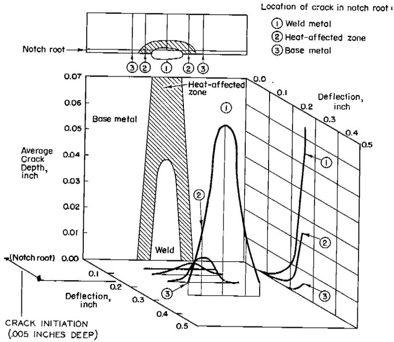
FIGURE 15A. CRACK INITIATION AND PROPAGATION IN WELDED "C" STEEL KINZEL-TYPE SPECIMENS TESTED AT 180 F.
