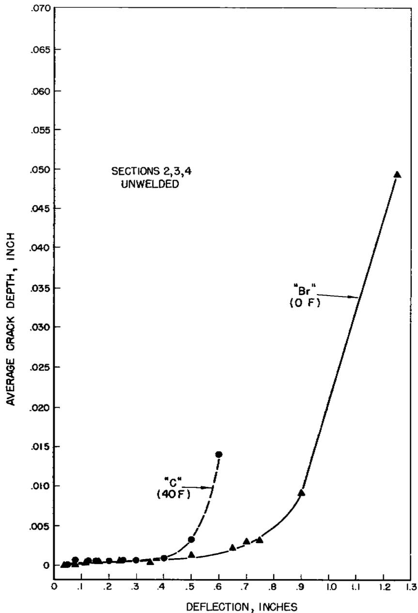
FIGURE B-18. COMPARISON OF AVERAGE CRACK DEPTH IN SECTIONS 2,3,4 OF UNWELDED "Br" AND "C" STEEL KINZEL SPECIMENS TESTED BELOW THEIR TRANSITION TEMPERATURES.
