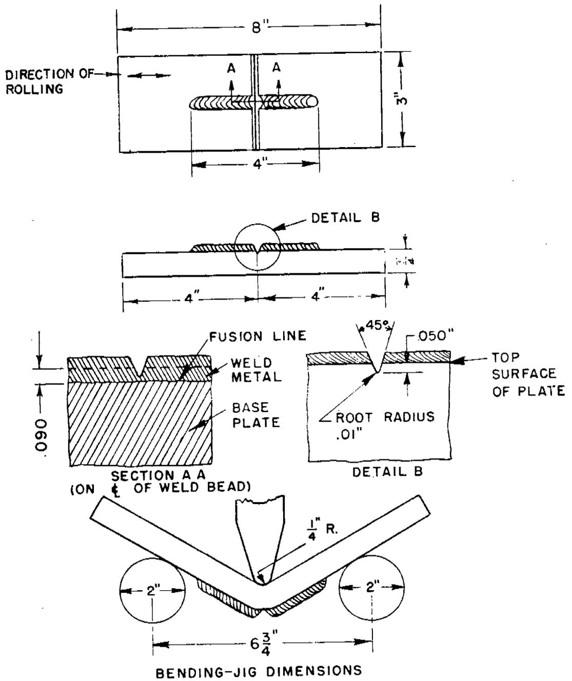
FIGURE 1. BEND SPECIMEN WITH LONGITUDINAL WELD BEAD AND TRANSVERSE NOTCH (KINZEL DESIGN)
