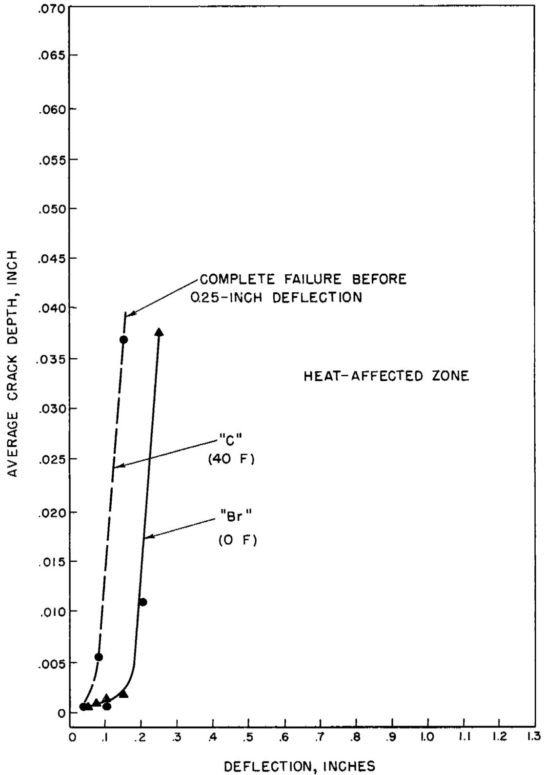
FIGURE B-22. COMPARISON OF AVERAGE CRACK DEPTH IN HEAT-AFFECTED ZONE OF WELDED "Br" AND "C" STEEL KINZEL SPECIMENS TESTED BELOW THE TRANSITION TEMPERATURE.
