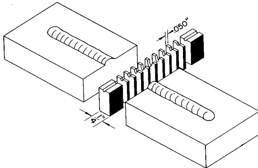
FIGURE 4. CUTTING AND SECTIONING DETAILS FOR WELDED KINZEL-TYPE SPECIMENS
