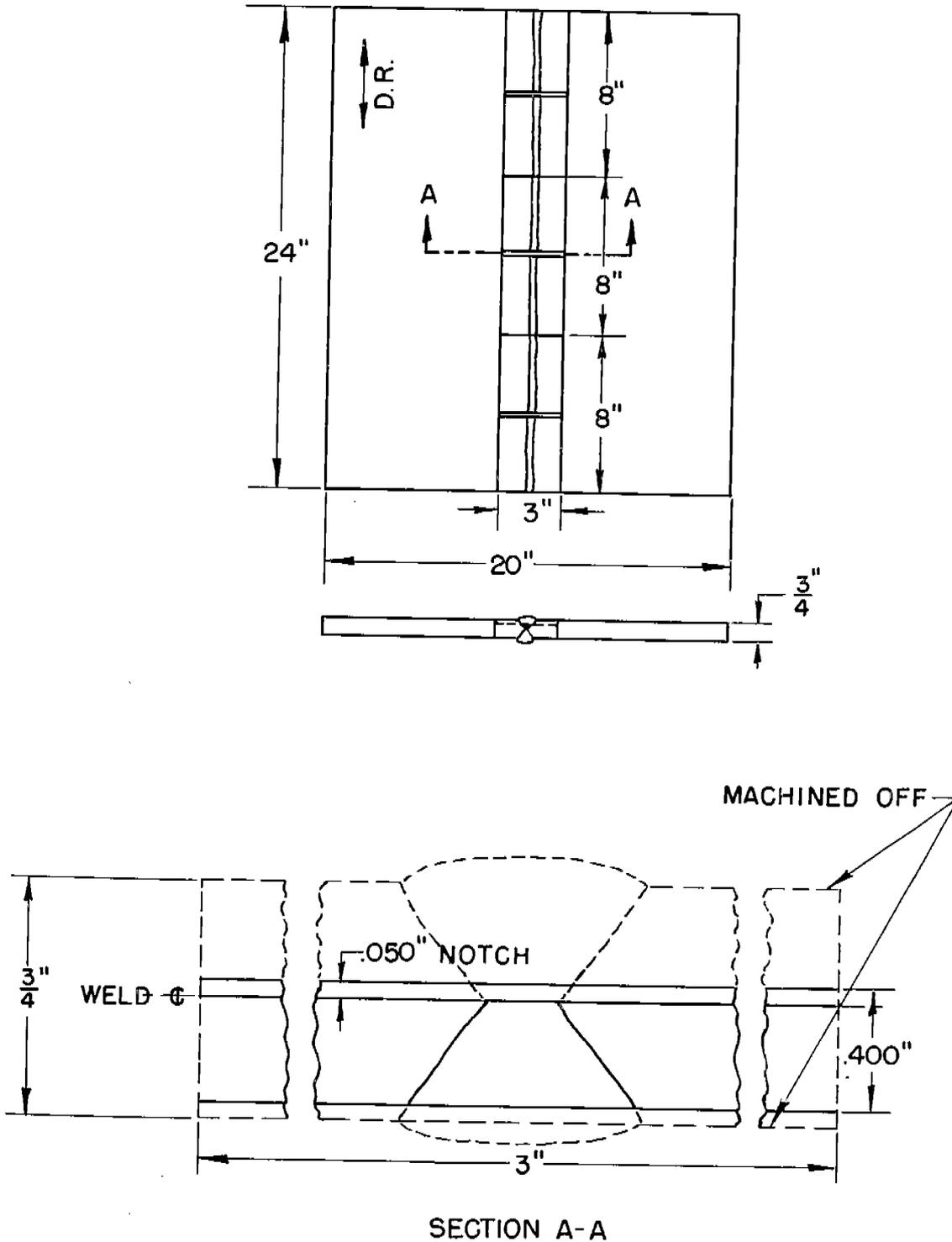
FIGURE 22. WELDMENT SIMILAR TO THOSE STUDIED AT CASE INSTITUTE OF TECHNOLOGY SHOWING LOCATION AND PREPARATION OF KINZEL-TYPE SPECIMENS
