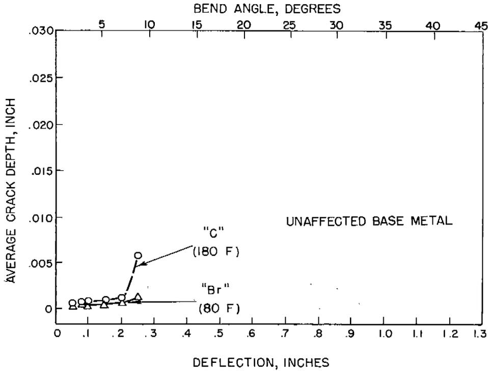
FIGURE B-23. COMPARISON OF AVERAGE CRACK DEPTH IN UNAFFECTED BASE METAL OF WELDED "Br" AND "C" STEEL KINZEL SPECIMENS TESTED ABOVE THEIR TRANSITION TEMPERATURES.
