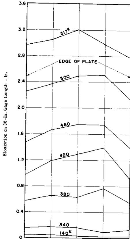
Fig. 16. Distribution across Plate of Elongation on 36-In. Gage Length. Spec. No. 5. Circular Opening. Face Bar Reinforcement.
