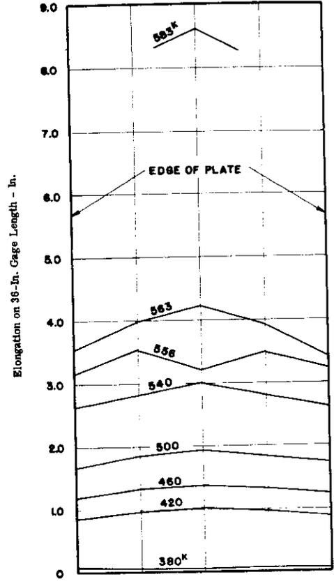
Fig. 12. Distribution across Plate of Elongation on 36-In. Gage Length. Spec. No. 23. Plain Plate.
