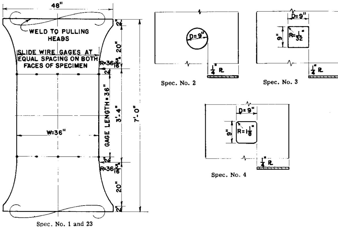
Fig. 2. Details of Plain Plates and Plates with Unreinforced Openings.
