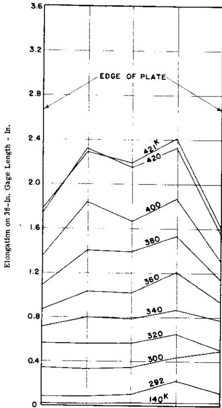
Fig. 15. Distribution across Plate of Elongation on 36-In. Gage Length. Spec. No. 4. Square Opening with Rounded Corners.
