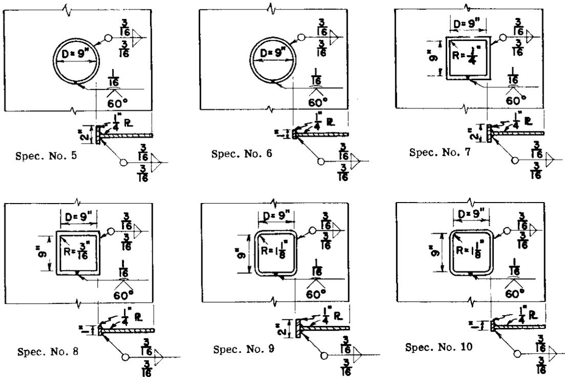
Fig. 3. Details of Plates with Openings Reinforced by a Face Bar.
