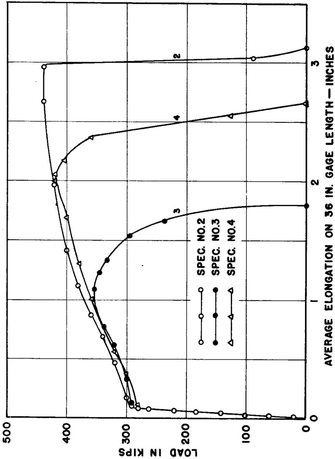
Fig. 36. Comparison of Load and Average Elongation on 36-In. Gage Length for Plates with an Unreinforced Opening.
