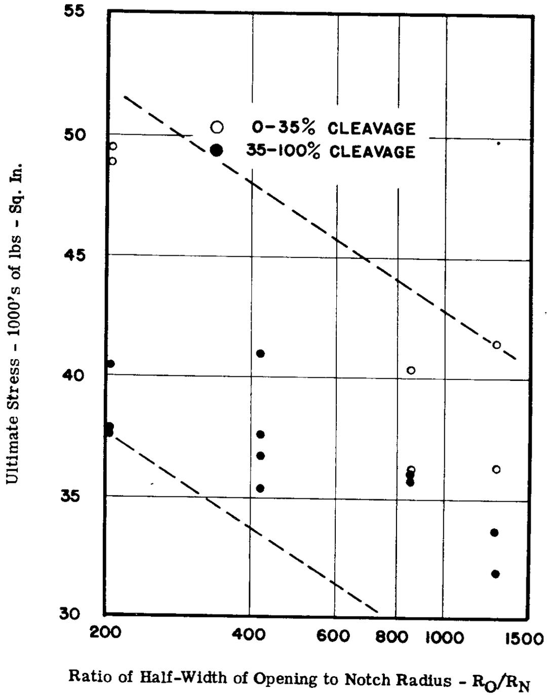
Fig. 81. Relation between the Ultimate Strength and the Notch Acuity of the Opening for Illinois Wide Plate Tests. Steel E as Rolled.
