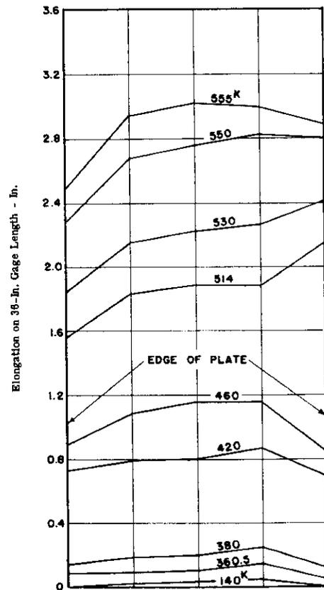
Fig. 22. Distribution across Plate of Elongation on 36-In. Gage Length. Spec. No. 11. Circular Opening. Single Doubler Plate Reinforcement.
