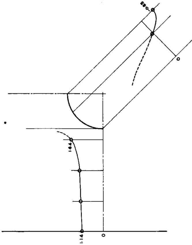
Fig. 52. Unit Strain Concentration in Region of Opening. Spec. No. 2. Circular Opening. No Reinforcement.
