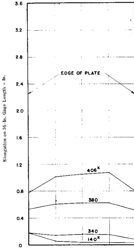
Fig. 25. Distribution across Plate of Elongation on 36-In. Gage Length. Spec. No. 14. Square Opening. Single Doubler Plate Reinforcement.
