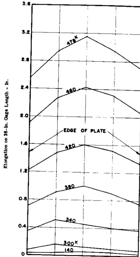
Fig. 32. Distribution across Plate of Elongation on 36-In. Gage Length. Spec. No. 21. Square Opening with Rounded Corners. Insert Plate Reinforcement.
