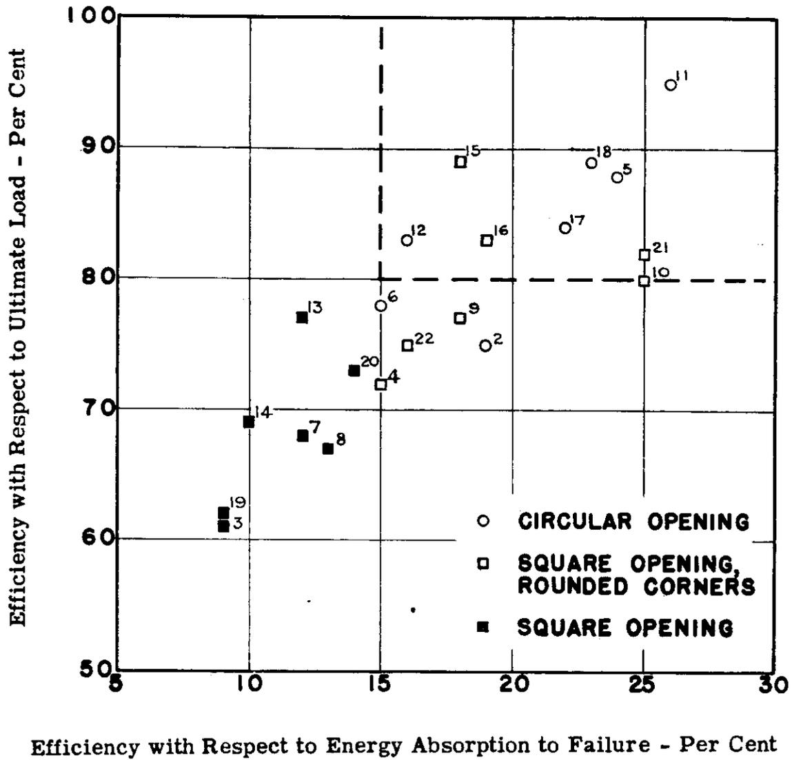
Fig. 49. Comparison of the Efficiencies with Respect to Ultimate Load and Energy Absorption to Failure for Plates with Openings.
