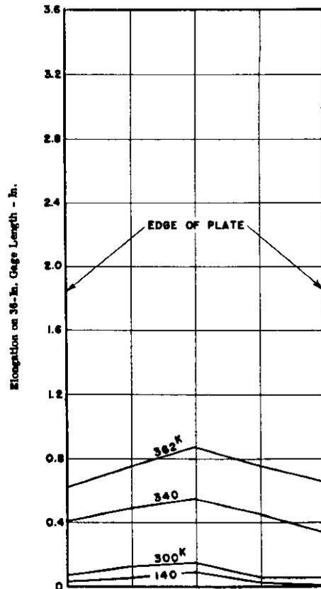
Fig. 30. Distribution across Plate of Elongation on 36-In. Gage Length. Spec. No. 19. Square Opening. Insert Plate Reinforcement.
