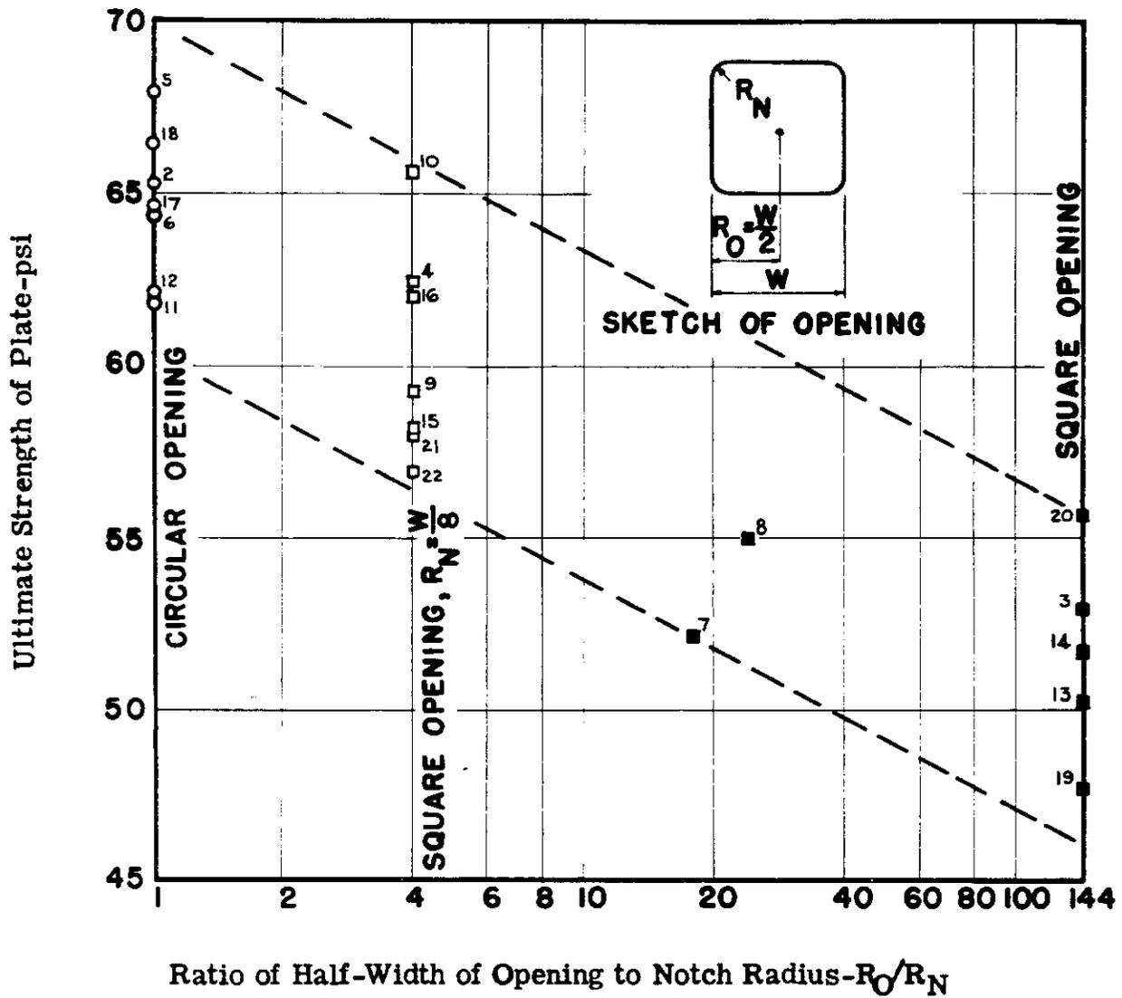
Fig. 45. Relation between the Ultimate Strength of Plates with Openings and the Notch Acuity of the Opening.
