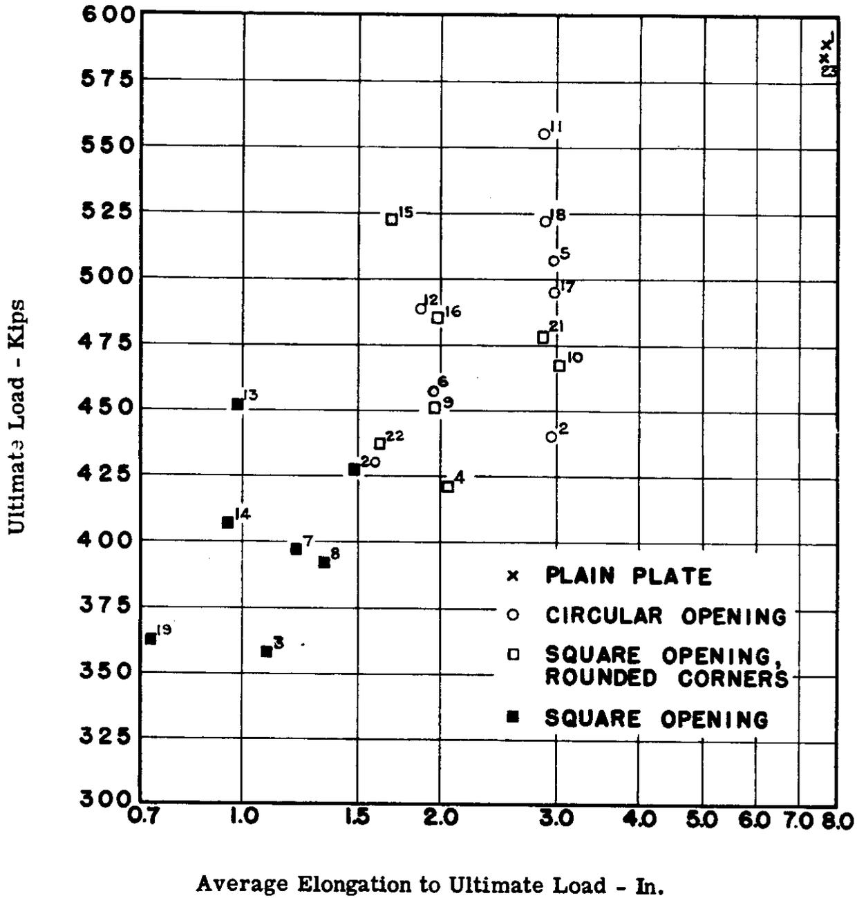
Fig. 40. Comparison of Ultimate Load and Average Elongation to Ultimate Load for Plain Plates and Plates with Openings.
