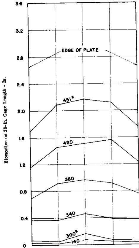
Fig. 20. Distribution across Plate of Elongation on 36-In. Gage Length. Spec. No. 9. Square Opening with Rounded Corners. Face Bar Reinforcement.
