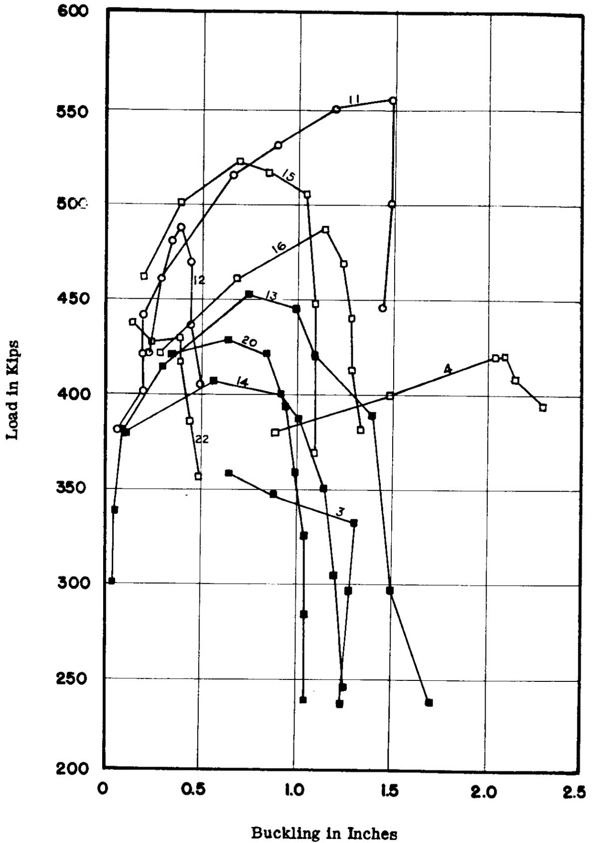
Fig. 75. Comparison of Load and the Maximum Lateral Deflection of the Buckled Edge of Opening in Plates with Openings.
