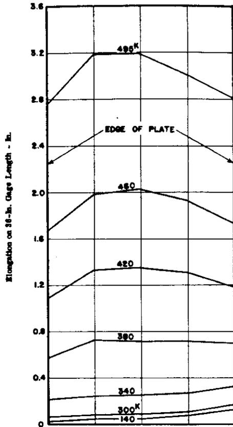
Fig. 28. Distribution across Plate of Elongation on 36-In. Gage Length. Spec. No. 17. Circular Opening. Insert Plate Reinforcement.
