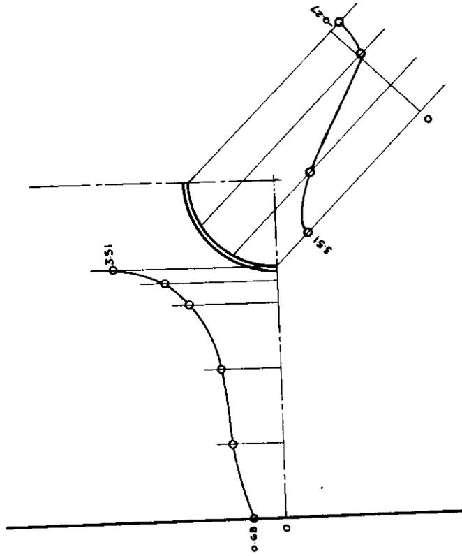
Fig. 54. Unit Strain Concentration in Region of Opening. Spec. No. 6. Circular Opening. Face Bar Reinforcement.
