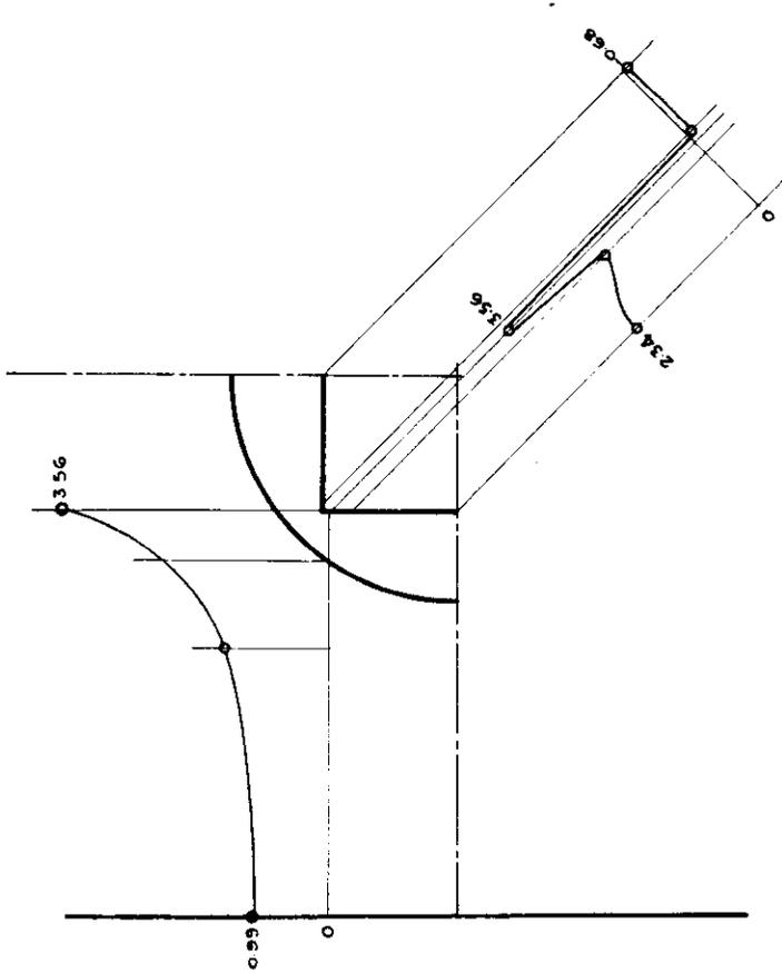
Fig. 71. Unit Strain Concentration in Region of Opening. Spec. No. 19. Square Opening. Insert Plate Reinforcement.
