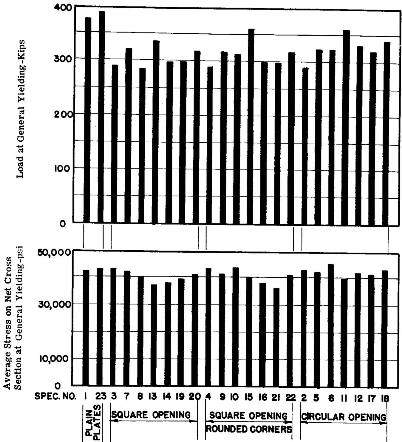
Fig. 41. Load and Average Stress on Net Cross Section at General Yielding of Plain Plates and Plates with Openings.
