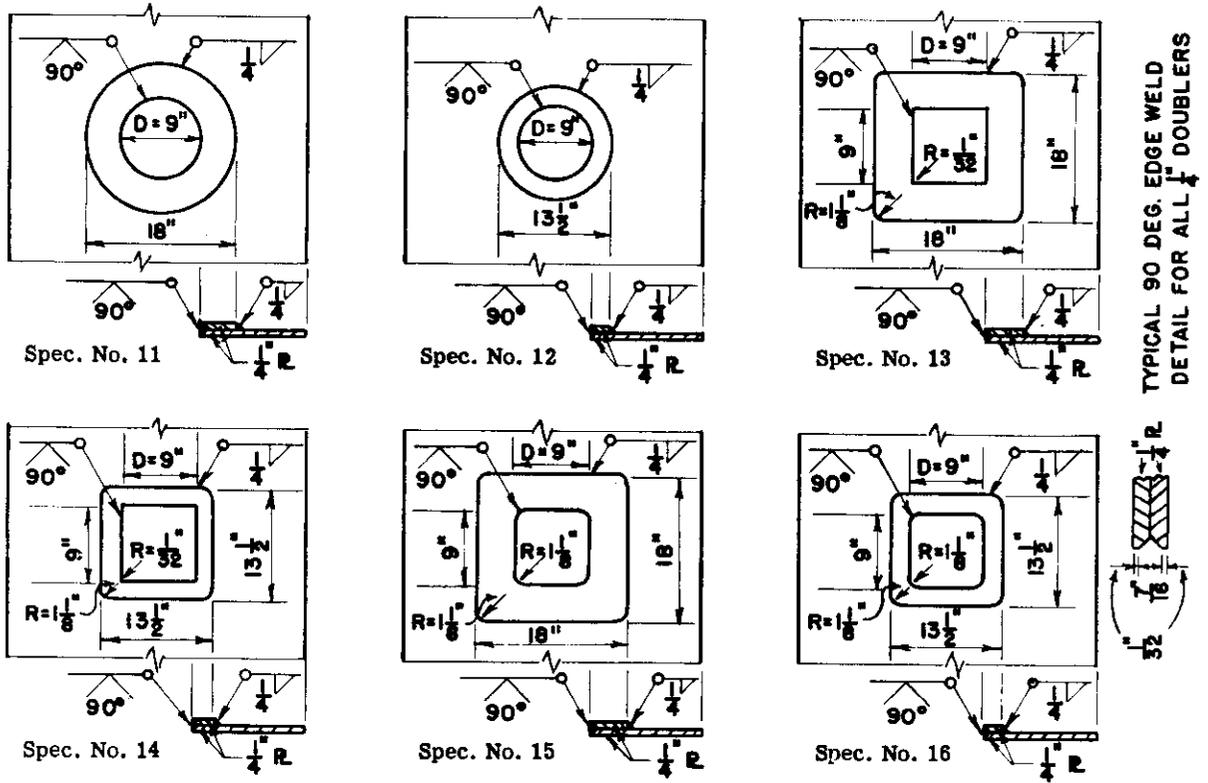
Fig. 4. Details of Plates with Openings Reinforced by a Single Doubler Plate.
