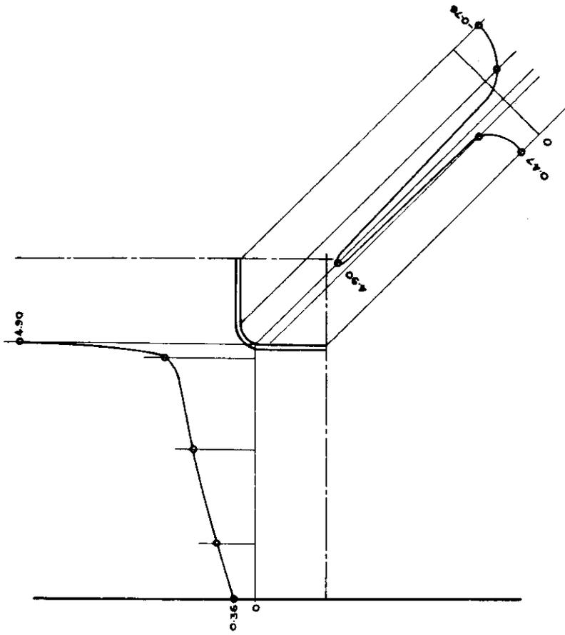
Fig. 60. Unit Strain Concentration in Region of Opening. Spec. No. 9. Square Opening, Rounded Corners. Face Bar Reinforcement.
