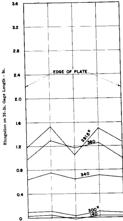
Fig. 19. Distribution across Plate of Elongation on 36-In. Gage Length. Spec. No. 8. Square Opening. Face Bar Reinforcement.
