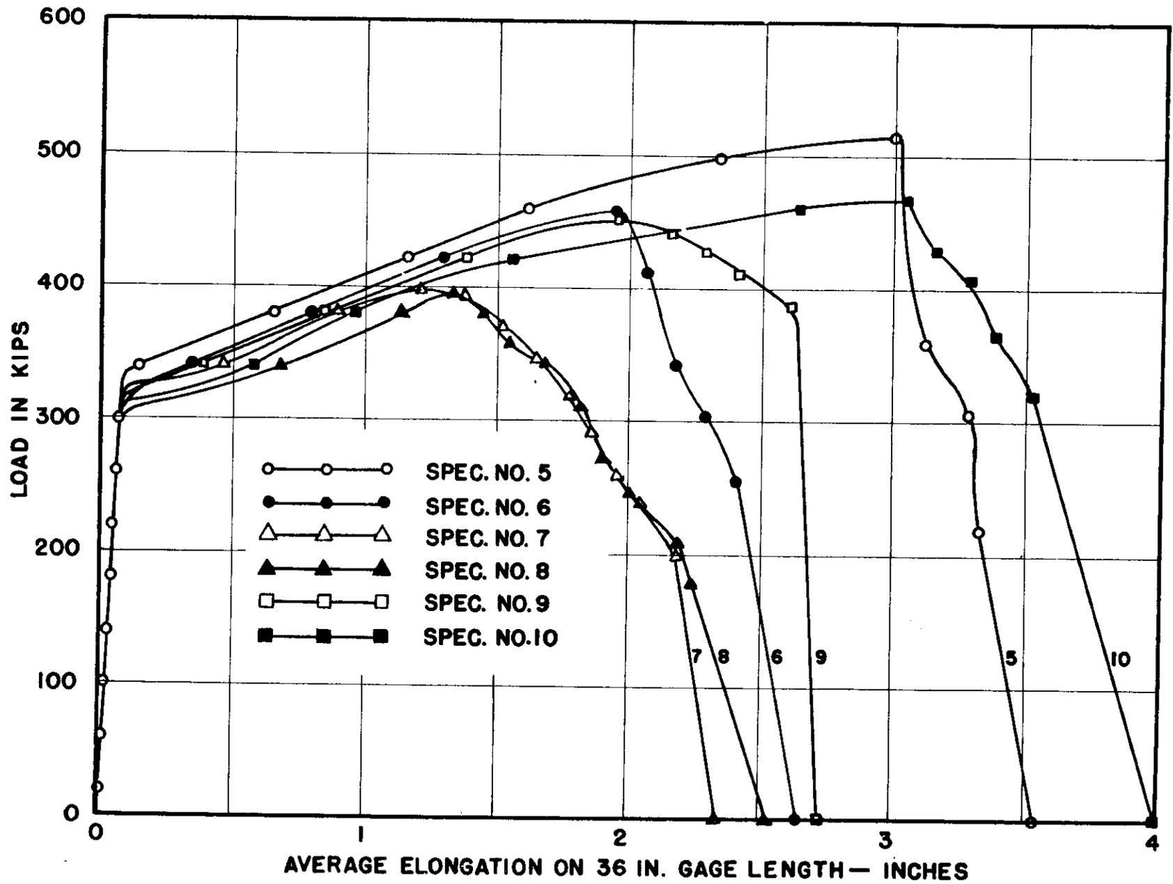
Fig. 37. Comparison of Load and Average Elongation on 36-in. Gage Length for Plates with Openings Reinforced by a Face Bar.
