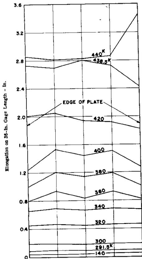
Fig. 13. Distribution across Plate of Elongation on 36-In. Gage Length. Spec. No. 2. Circular Opening.
