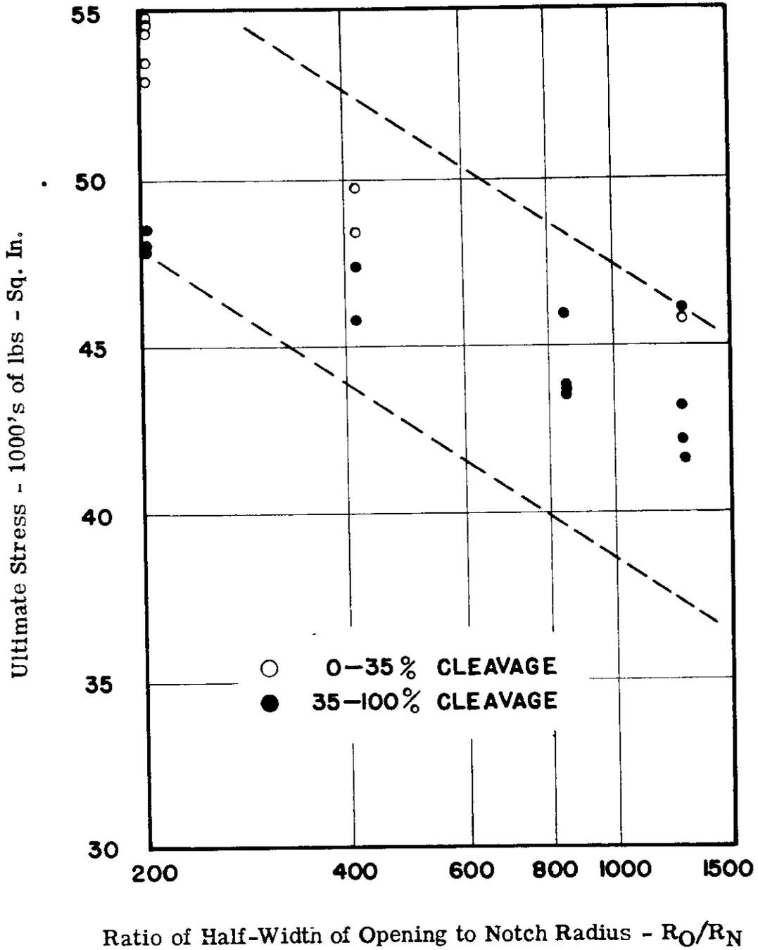
Fig. 82. Relation between the Ultimate Strength and the Notch Acuity of the Opening for Illinois Wide Plate Tests. Steel D as Rolled.
