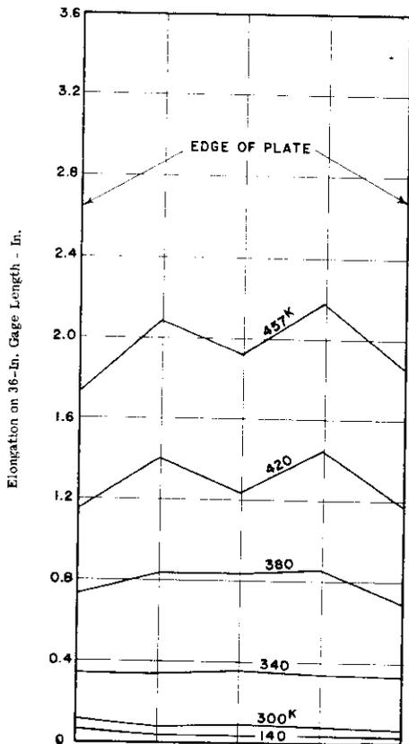
Fig. 17. Distribution across Plate of Elongation on 36-In. Gage Length. Spec. No. 6. Circular Opening. Face Bar Reinforcement.
