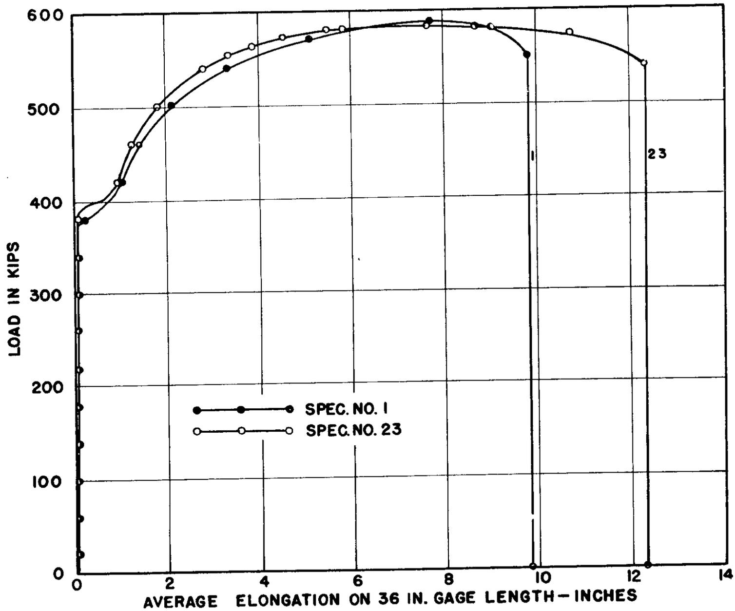
Fig. 35. Comparison of Load and Average Elongation on 36-In. Gage Length for Plain Plates
