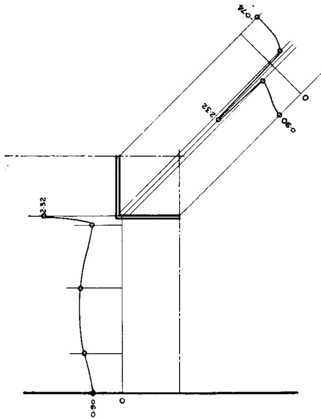
Fig. 67. Unit Strain Concentration in Region of Opening. Spec. No. 7. Square Opening. Face Bar Reinforcement.
