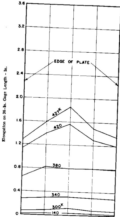
Fig. 31. Distribution across Plate of Elongation on 36-In. Gage Length. Spec. No. 20. Square Opening. Insert Plate Reinforcement.
