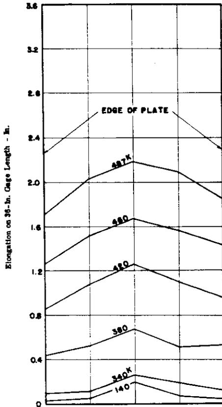
Fig. 27. Distribution across Plate of Elongation on 36-In. Gage Length. Spec. No. 16. Square Opening with Rounded Corners. Single Doubler Plate Reinforcement.
