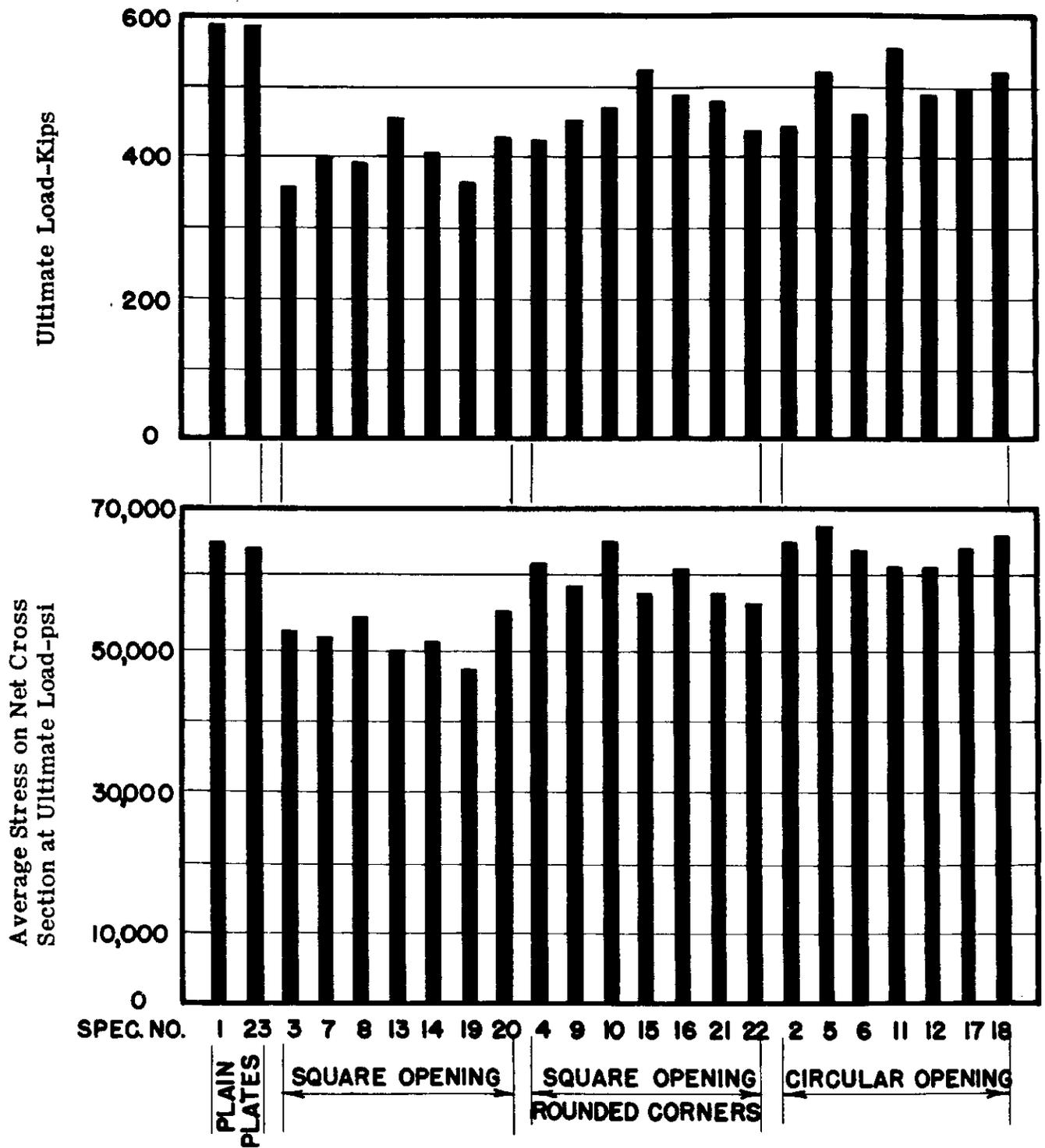
Fig. 42. Ultimate Strength of Plain Plates and Plates with Openings.
