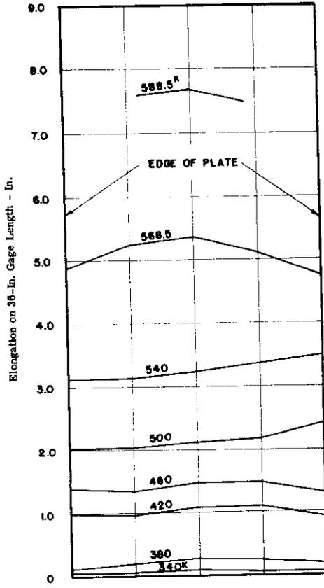
Fig. 11. Distribution across Plate of Elongation on 36-In. Gage Length. Spec. No. 1. Plain Plate.
