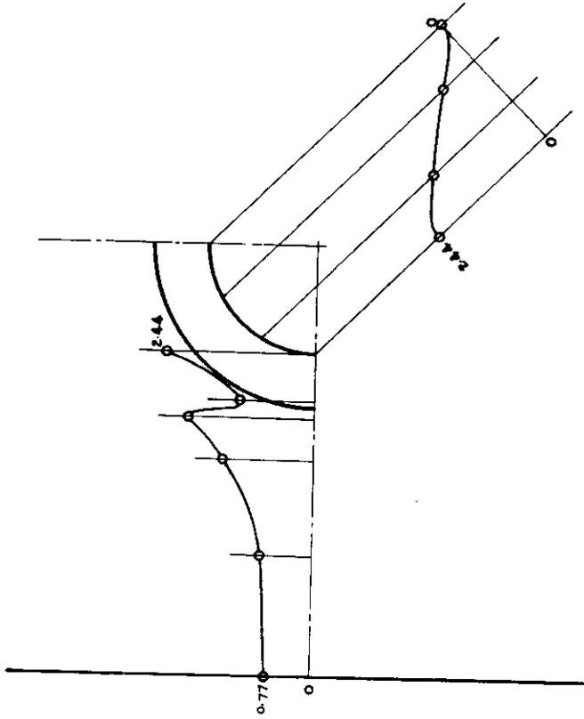
Fig. 56. Unit Strain Concentration in Region of Opening. Spec. No. 12. Circular Opening. Single Doubler Plate Reinforcement.
