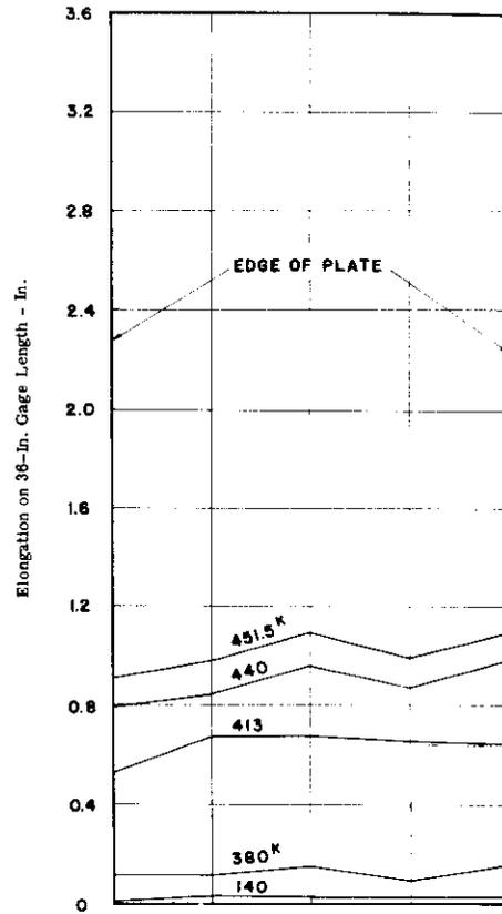
Fig. 24. Distribution across Plate of Elongation on 36-In. Gage Length. Spec. No. 13. Square Opening. Single Doubler Plate Reinforcement.
