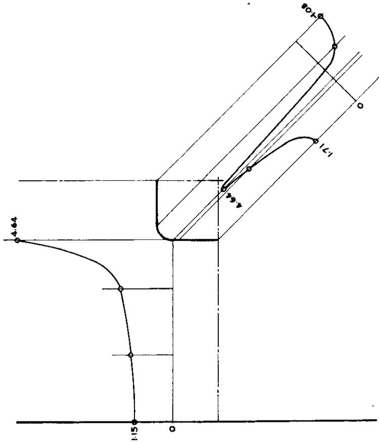
Fig. 59. Unit Strain Concentration in Region of Opening. Spec. No. 4. Square Opening, Rounded Corners. No Reinforcement.
