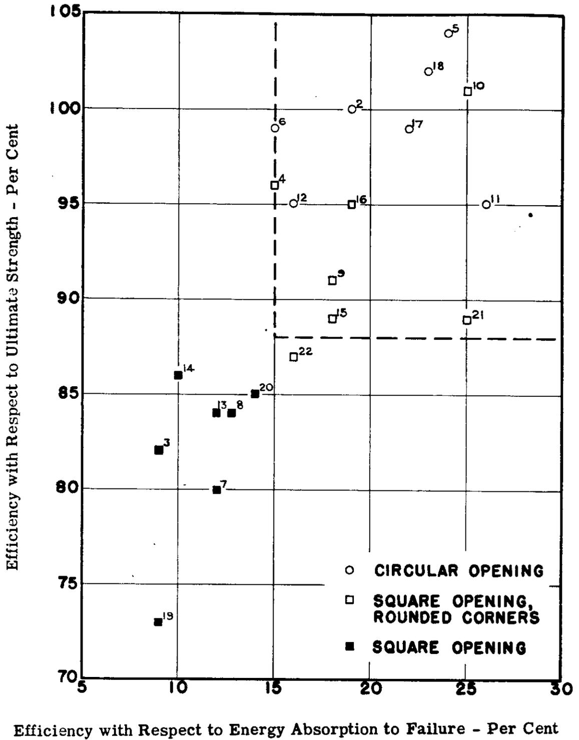
Fig. 50. Comparison of Efficiencies with Respect to Ultimate Strength and Energy Absorption to Failure for Plates with Openings.
