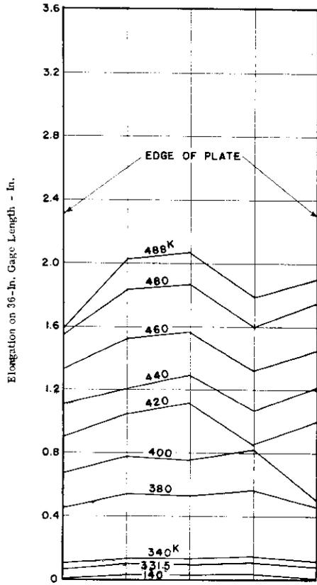
Fig. 23. Distribution across Plate of Elongation on 36-In. Gage Length. Spec. No. 12. Circular Opening. Single Doubler Plate Reinforcement.
