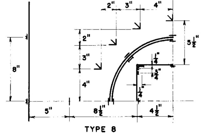
Fig. 9. Location of SR-4 Electric Strain Gages on Specimens with Opening Reinforced by a Single Doubler Plate.
