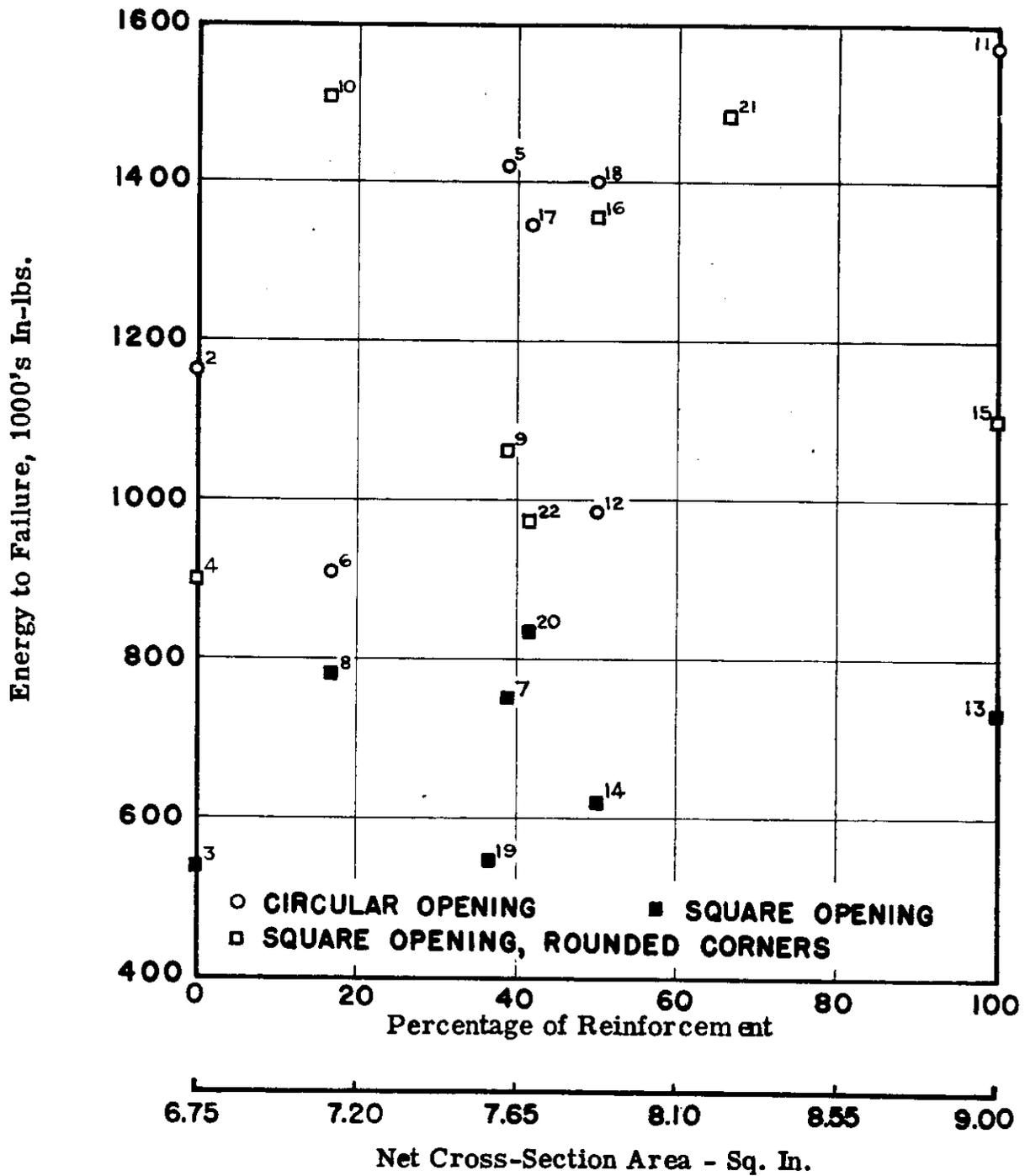
Fig. 47. Comparison of Energy Absorption to Failure and Percentage of Reinforcement for Plates with Openings.
