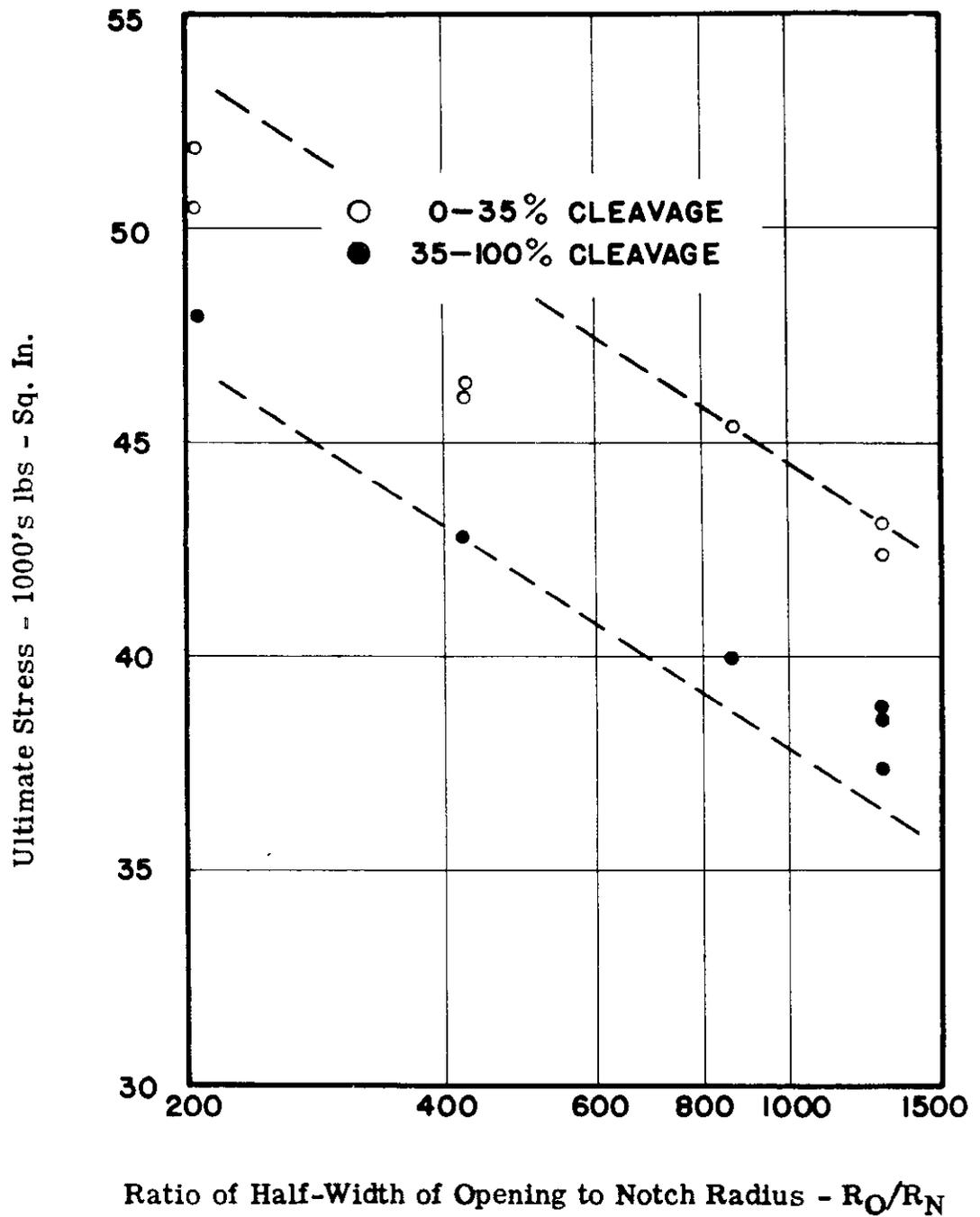
Fig. 83. Relation between the Ultimate Strength and the Notch Acuity of the Opening for Illinois Wide Plate Tests. Steel D Normalized.
