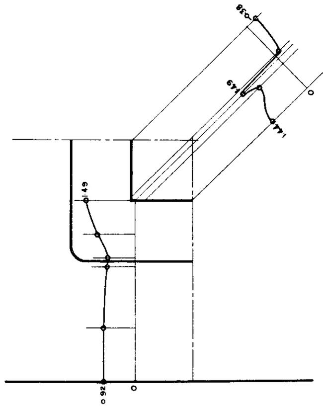
Fig. 70. Unit Strain Concentration in Region of Opening. Spec. No. 14. Square Opening. Single Doubler Plate Reinforcement.
