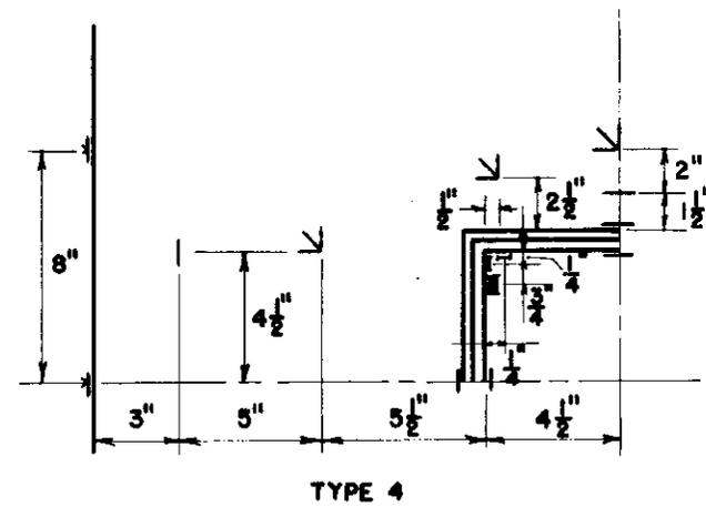
Fig. 7. Location of SR-4 Electric Strain Gages on Specimens with Unreinforced Openings.
