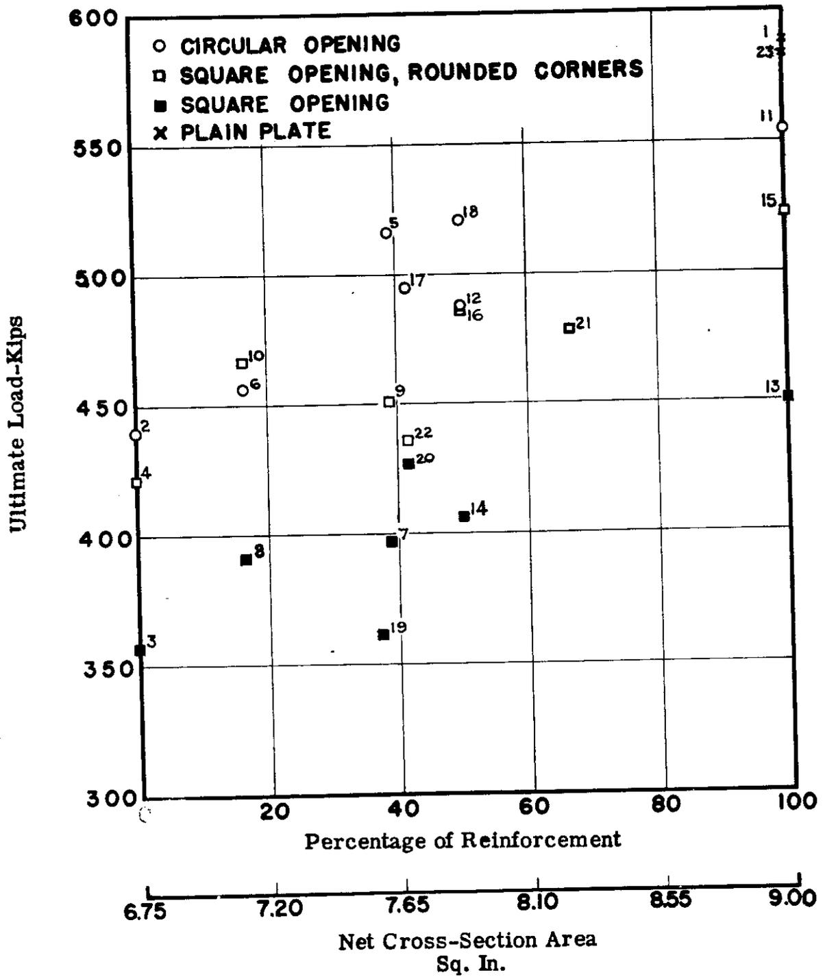
Fig. 43. Comparison of Ultimate Load and Percentage of Reinforcement for Plates with Openings.
