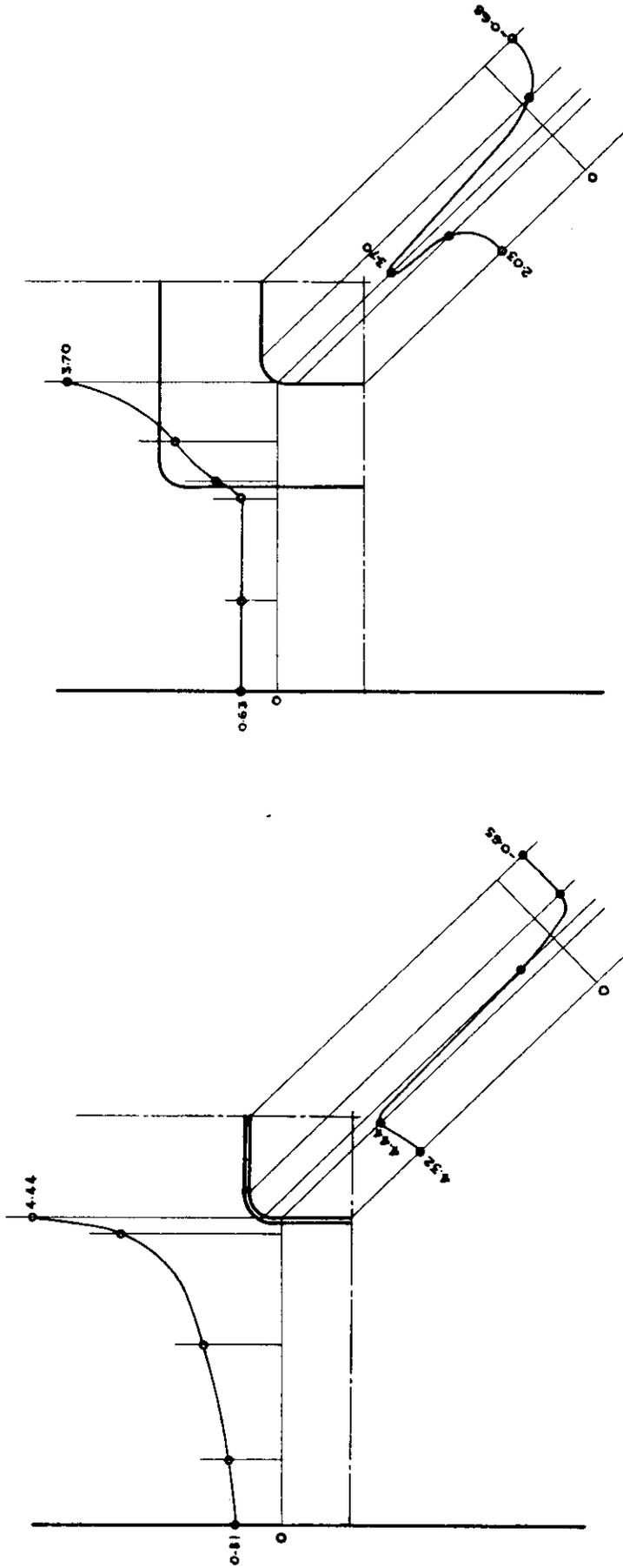
Fig. 61. Unit Strain Concentration in Region of Opening. Spec. No. 10. Square Opening, Rounded Corners. Face Bar Reinforcement.
