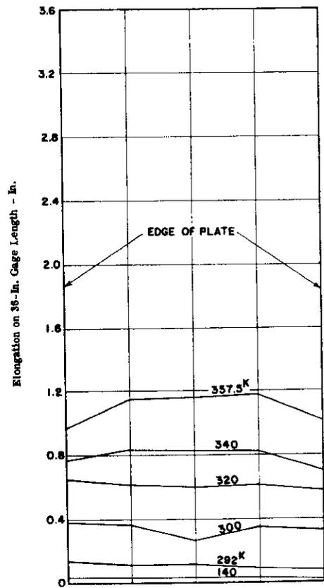
Fig. 14. Distribution across Plate of Elongation on 36-In. Gage Length. Spec. No. 3. Square Opening.
