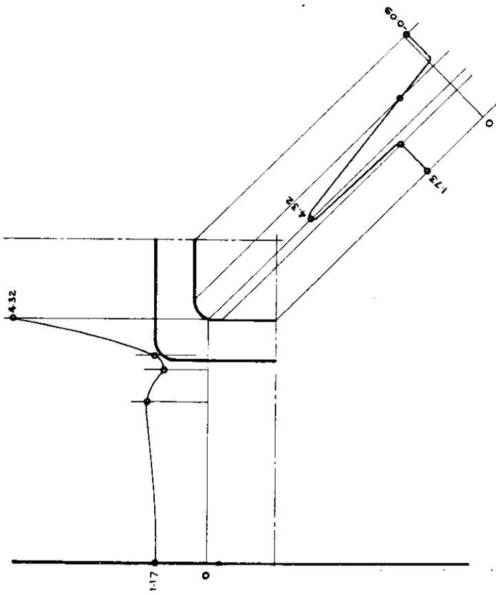
Fig. 63. Unit Strain Concentration in Region of Opening. Spec. No. 16. Square Opening, Rounded Corners. Single Doubler Plate Reinforcement.
