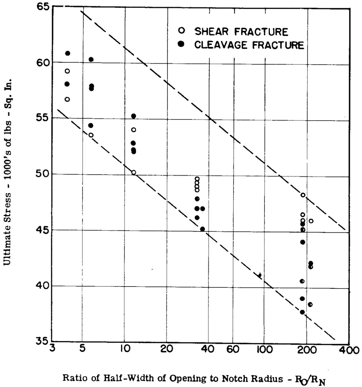
Fig. 84. Relation between the Ultimate Strength and the Notch Acuity of the Opening for Wide Plate Tests by Thomas and Windenburg. Steel E as Rolled.
