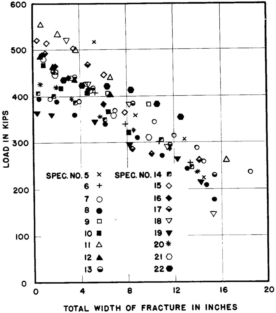
Fig. 80. Comparison of Total Load on Plate and Total Length of Fracture.
