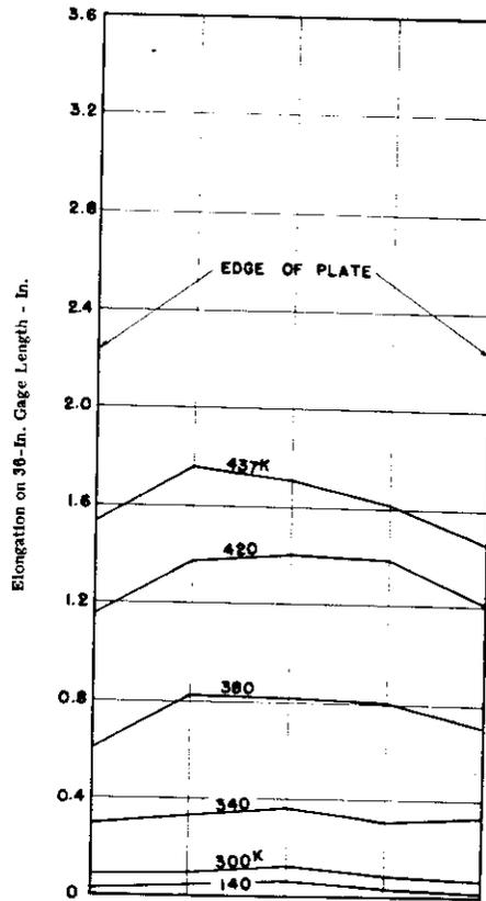
Fig. 33. Distribution across Plate of Elongation on 36-In. Gage Length. Spec. No. 22. Square Opening with Rounded Corners. Insert Plate Reinforcement.
