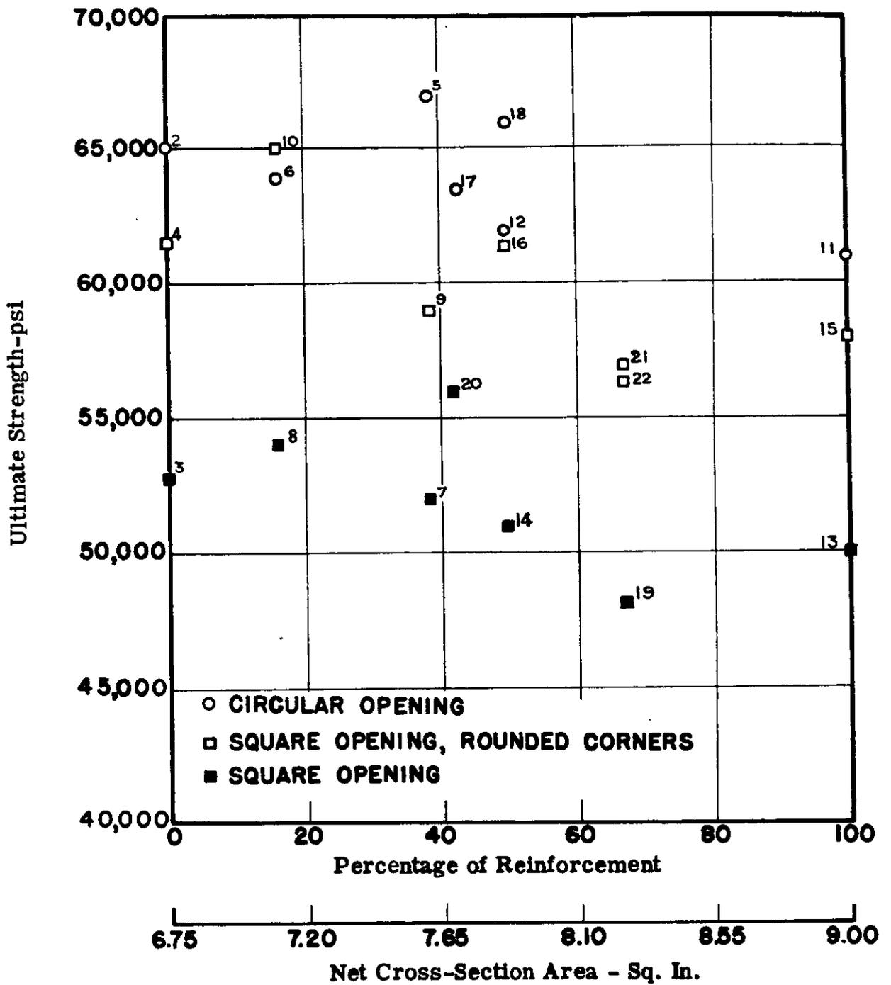
Fig. 44. Comparison of Ultimate Strength with Percentage of Reinforcement for Plates with Openings.
