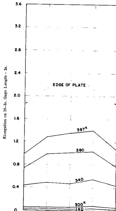
Fig. 18. Distribution across Plate of Elongation on 36-In. Gage Length. Spec. No. 7. Square Opening. Face Bar Reinforcement.
