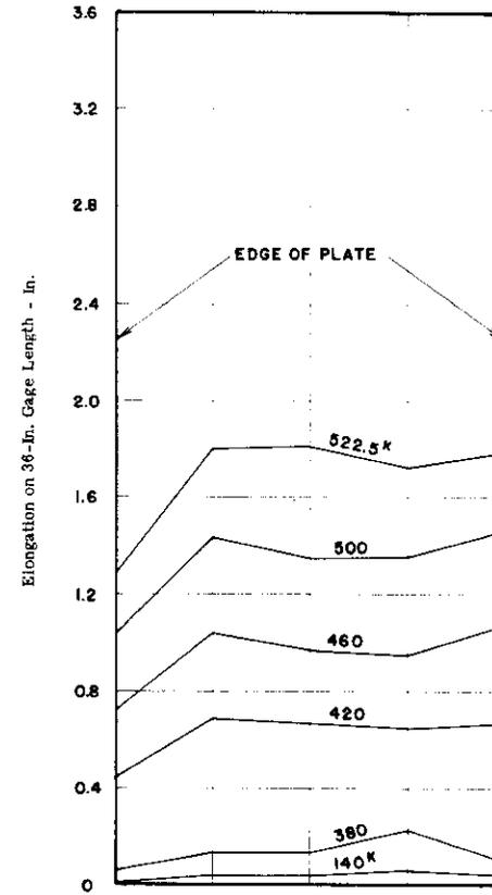
Fig. 26. Distribution across Plate of Elongation on 36-In. Gage Length. Spec. No. 15. Square Opening with Rounded Corners. Single Doubler Plate Reinforcement.
