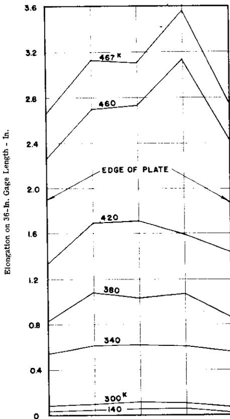
Fig. 21. Distribution across Plate of Elongation on 36-In. Gage Length. Spec. No. 10. Square Opening with Rounded Corners. Face Bar Reinforcement.
