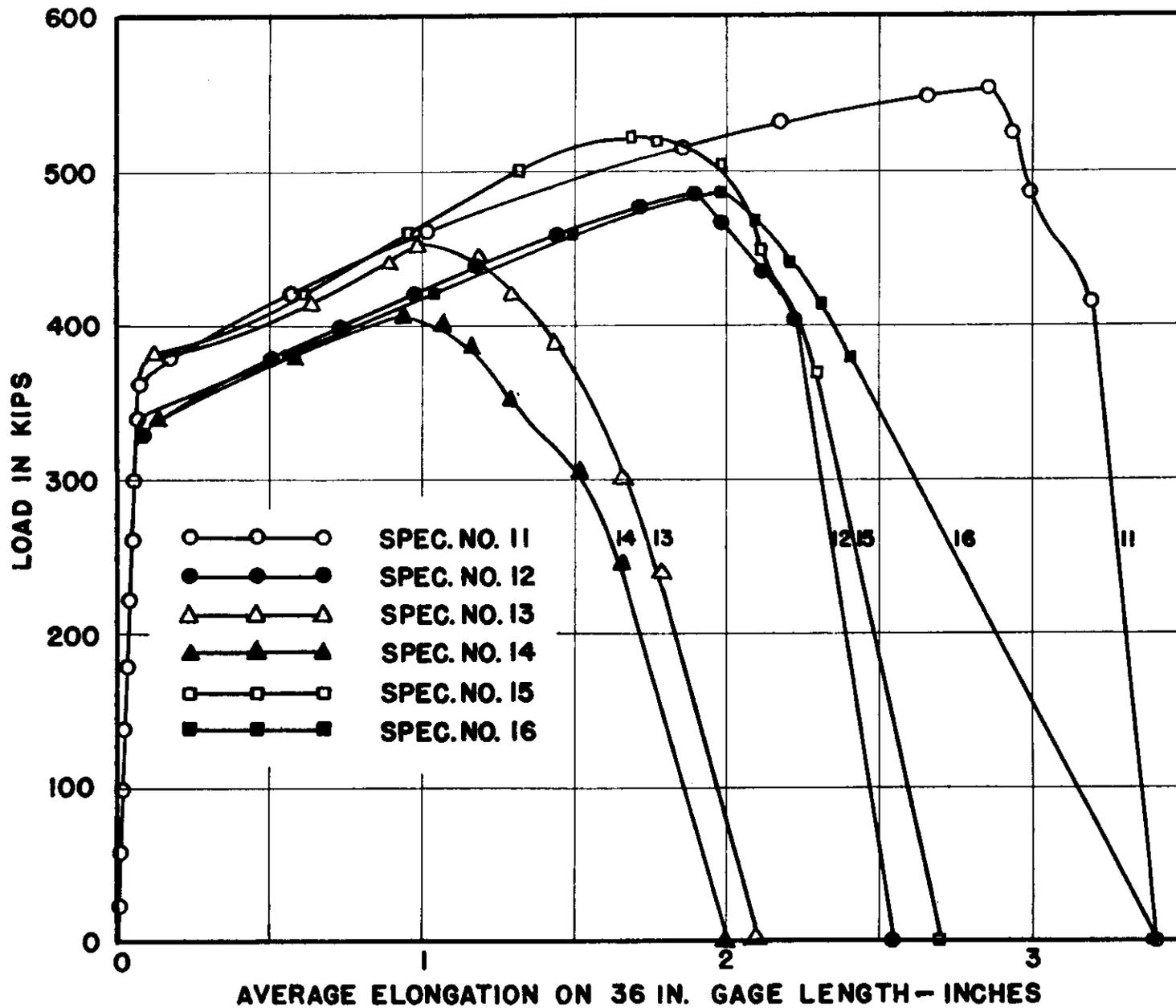
Fig. 38. Comparison of Load and Average Elongation on 36-In. Gage Length for Plates with Openings Reinforced by a Single Doubler Plate.
