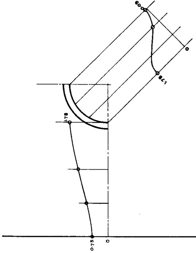
Fig. 58. Unit Strain Concentration in Region of Opening. Spec. No. 18. Circular Opening. Insert Plate Reinforcement.
