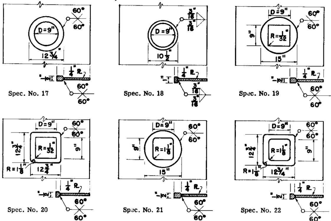
Fig. 5. Details of Plates with Openings Reinforced by an Insert Plate.
