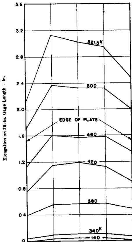
Fig. 29. Distribution across Plate of Elongation on 36-In. Gage Length. Spec. No. 18. Circular Opening. Insert Plate Reinforcement.
