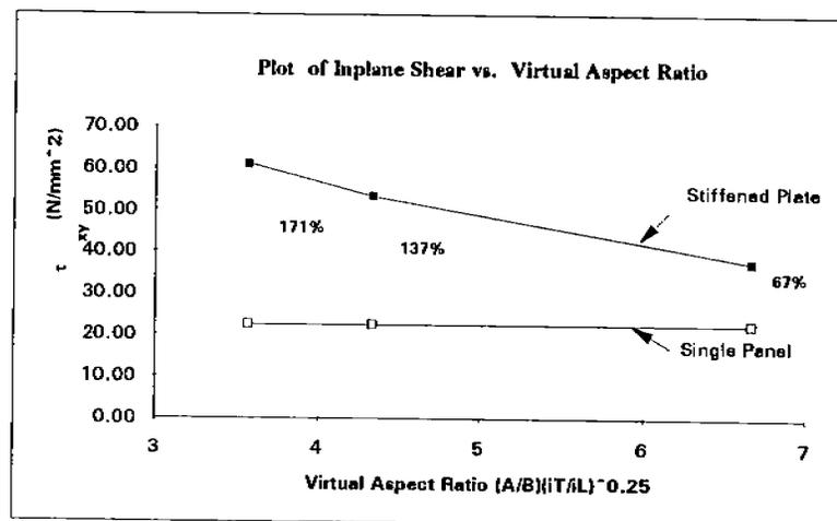
FIGURE 4.13 COMPARISON OF STRESSES IN OSS PLATE MODEL WITH SINGLE PANEL
