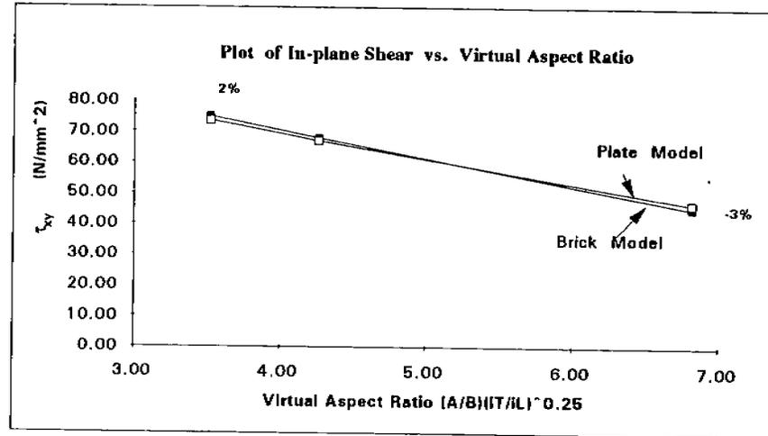
FIGURE 4.40 COMPARISON OF STRESSES IN HSS BRICK MODEL WITH HSS PLATE MODEL
