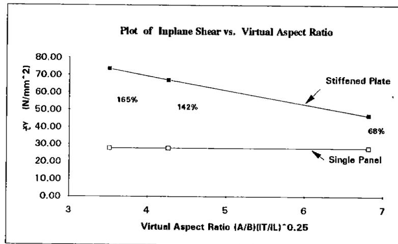
FIGURE 4.14 COMPARISON OF STRESSES IN HSS PLATE MODEL WITH SINGLE PANEL
