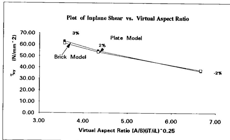
FIGURE 4.39 COMPARISION OF STRESSES IN OSS BRICK MODEL WITH OSS PLATE MODEL
