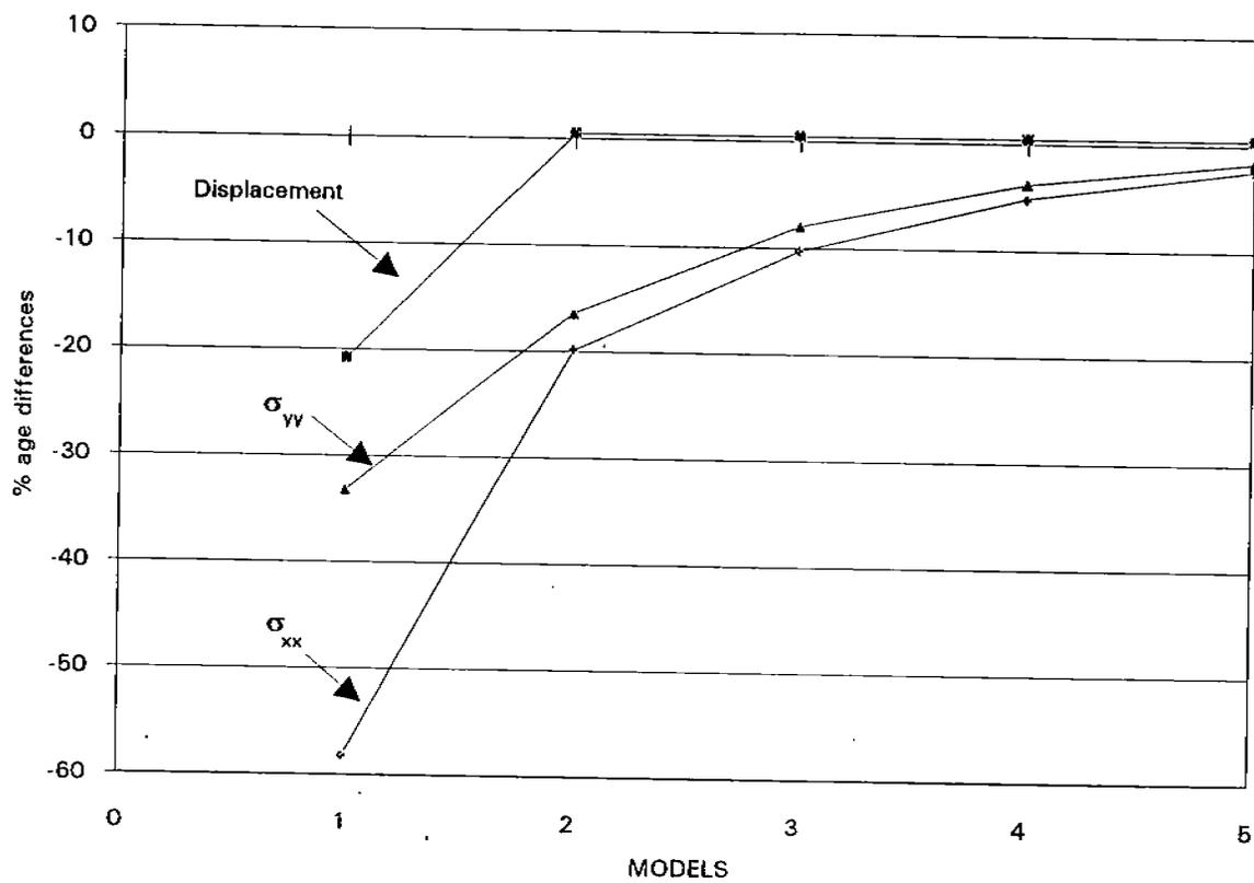
FIGURE 3.1 Mesh Size Determination using Plate Elements
