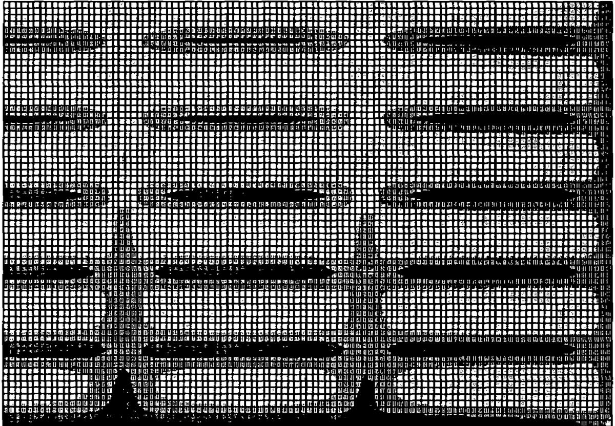
FIGURE 4.16 OSS BRICK MODEL 1;  $\sigma_{yy}$  STRESS (VIEW FROM THE BOTTOM)
