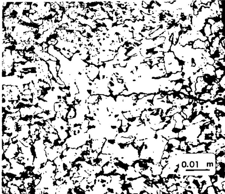
**Figure 8a. Optical micrograph of the crack tip in Mil S-24645 base metal tested in ASTM seawater with -1.0V (SCE) protection at 10Hz, R=0.1, etched in 3% Nital.**
