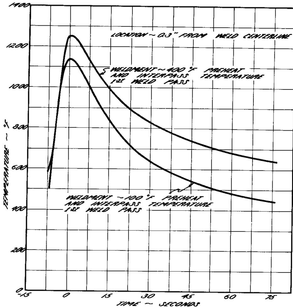
FIG.32: HEATING AND COOLING CURVES IN THE REGION OF LOWEST DUCTILITY FOR TWO WELDING CONDITIONS.
