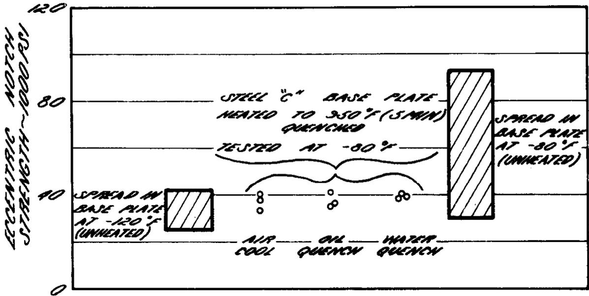
FIG. 3A: EFFECT OF SUBCRITICAL HEATING AND COOLING ON THE ECCENTRIC NOTCH STRENGTH OF UNAFFECTED BASE PLATE.
