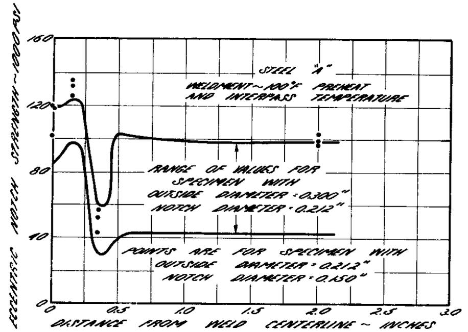
FIG.33: EFFECT OF SPECIMEN SECTION SIZE ON THE DISTRIBUTION OF ECCENTRIC NOTCH STRENGTH AT -70°F.
