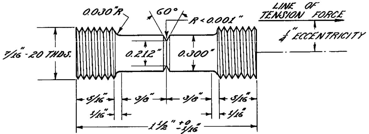
FIG. 7: SPECIMEN WITH 50 PERCENT SHARP NOTCH USED IN ECCENTRIC TESTING (50 PERCENT OF THE AREA REMOVED AT THE NOTCH BOTTOM).
