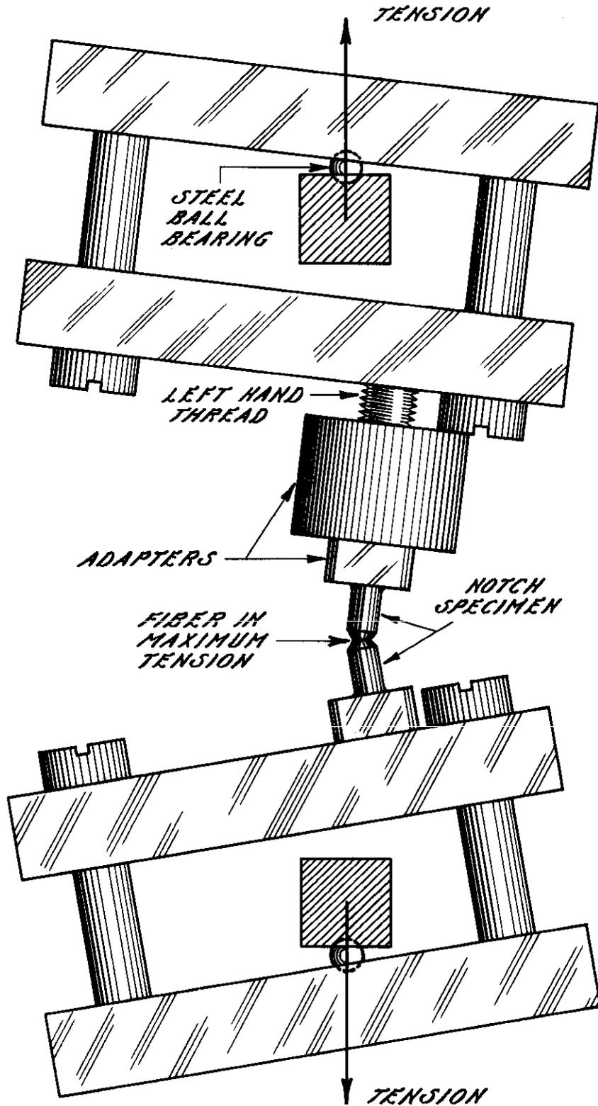
FIG. 8: METHOD OF LOADING TO OBTAIN  $\frac{1}{4}$  INCH ECCENTRICITY (ECCENTRICITY AND THE POSITION OF FIXTURES ARE EXAGGERATED).
