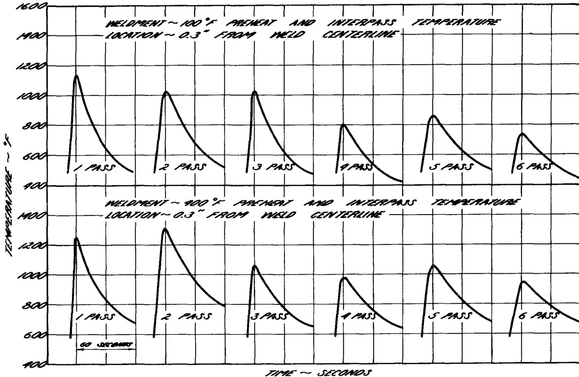
FIG.31: HEATING AND COOLING CURVES IN THE REGION OF LOWEST DUCTILITY FOR TWO 6 PASS WELDMENTS.
