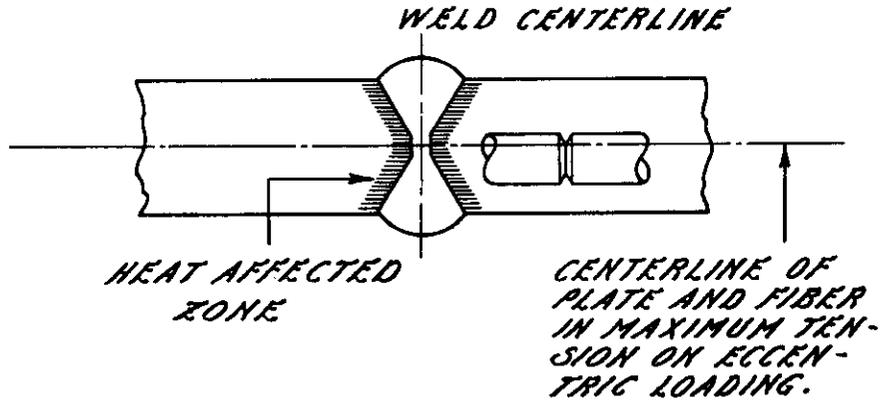
FIG. 6: LOCATION OF SPECIMEN IN THICKNESS DIMENSION OF WELDMENT.
