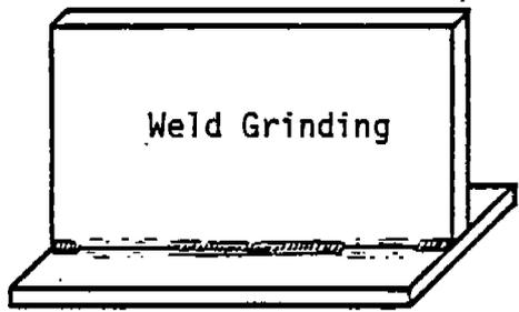
FIGURE 5.3 DETAILS TO LIMIT CRACK SIZE
