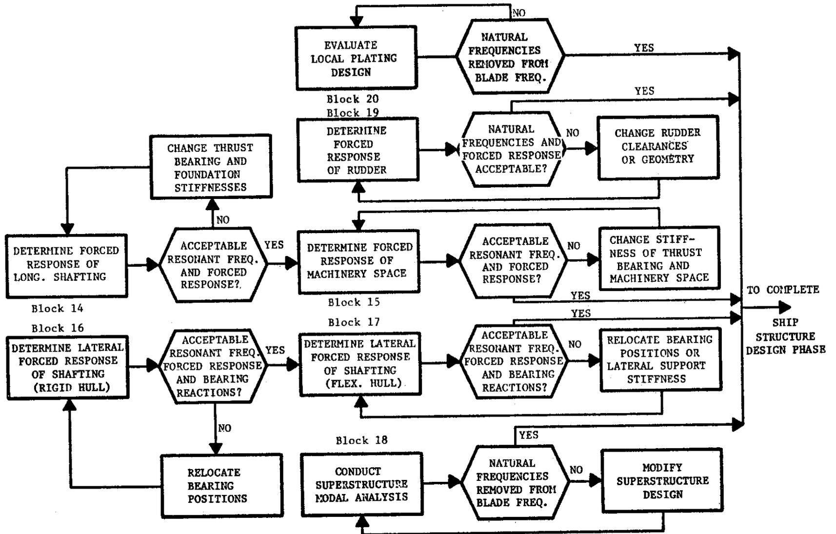
FIGURE 28. MILESTONE III - SHIP SUBSTRUCTURE EVALUATION
