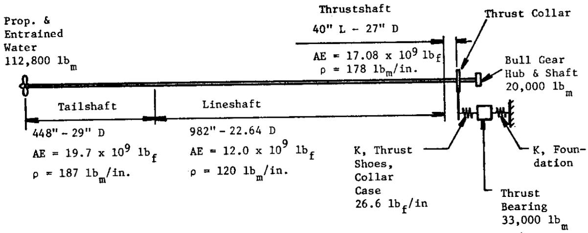
(a) Propeller and Shaft Mass-Elastic System
