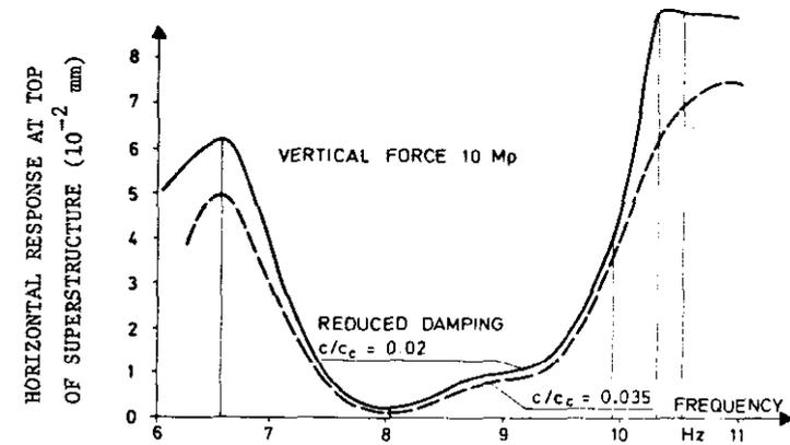
FIGURE 18. FORCED RESPONSE DEPENDING ON APPLIED GLOBAL DAMPING VALUE. 370,000 DWT TANKER, BALLAST CONDITION, FROM [75].
