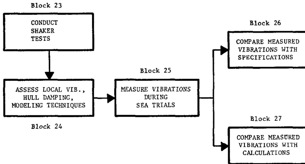
FIGURE 31. TEST AND EVALUATION DESIGN PHASE
