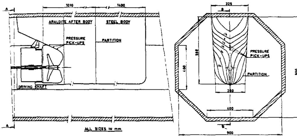
FIGURE 5. STERN GEOMETRY FOR CAVITATION TUNNEL TESTS,
