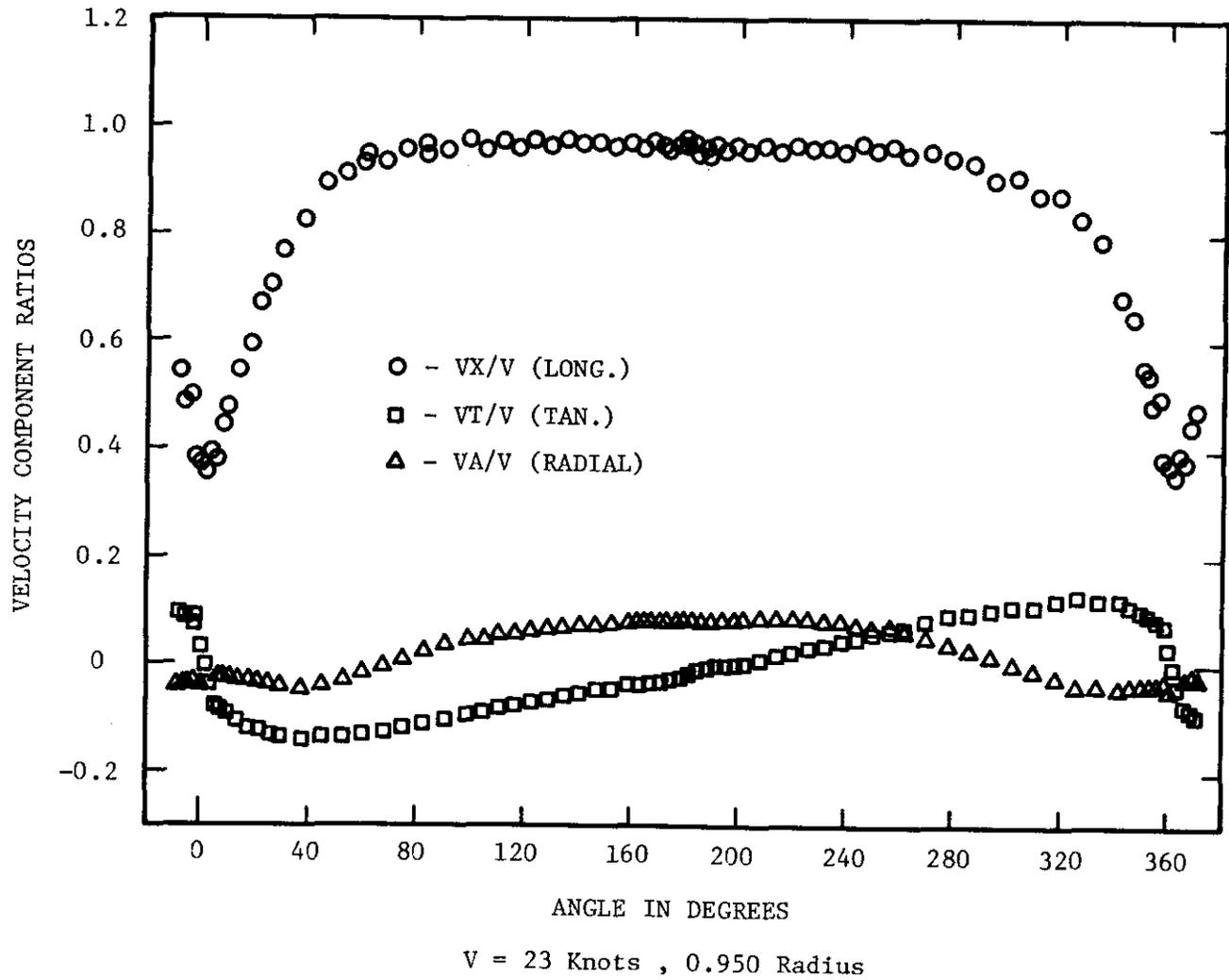
FIGURE F4. LONGITUDINAL, TANGENTIAL, AND AXIAL WAKES AT 0.950 RADIUS
