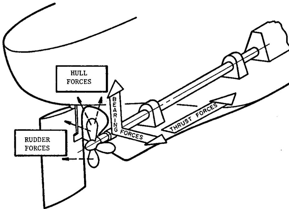
FIGURE 1. CONCEPTUAL IDENTIFICATION OF HULL VIBRATION SOURCES
