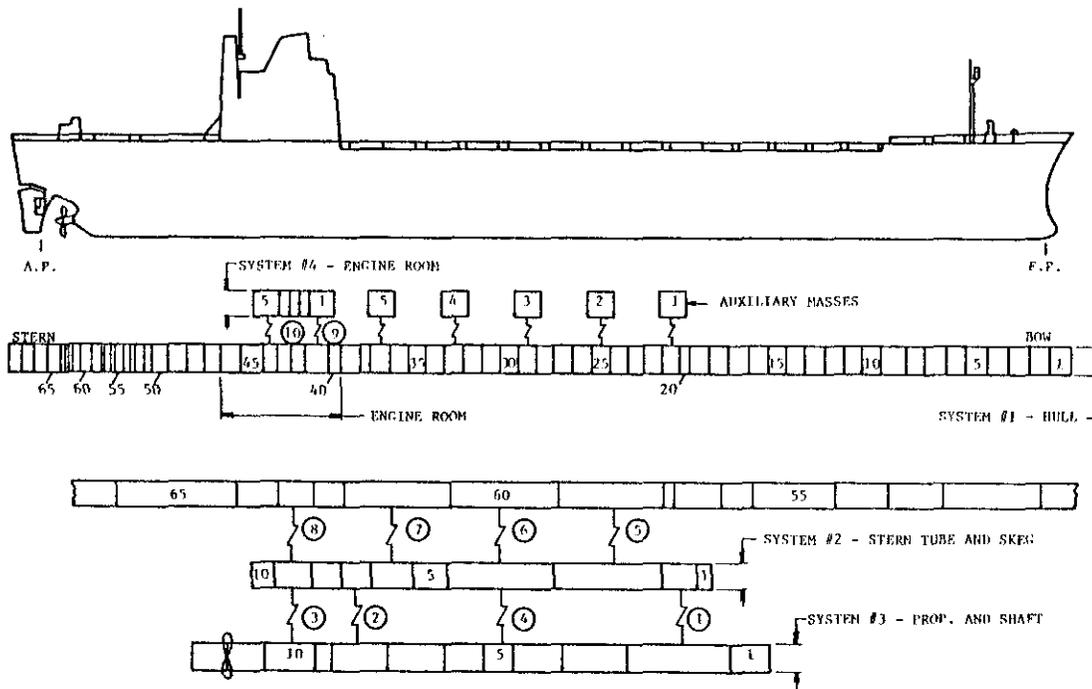
FIGURE 13. UNITIZED AND CONTAINERIZED SHIP, VERTICAL VIBRATION MODEL
