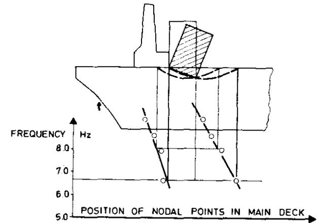
FIGURE 20. POSITION OF NODAL POINTS IN THE MAIN DECK FOR FORCED VIBRATIONS CALCULATIONS OF THE HULL GIRDER. 370,000 DWT TANKER, BALLAST CONDITION, FROM [75].
