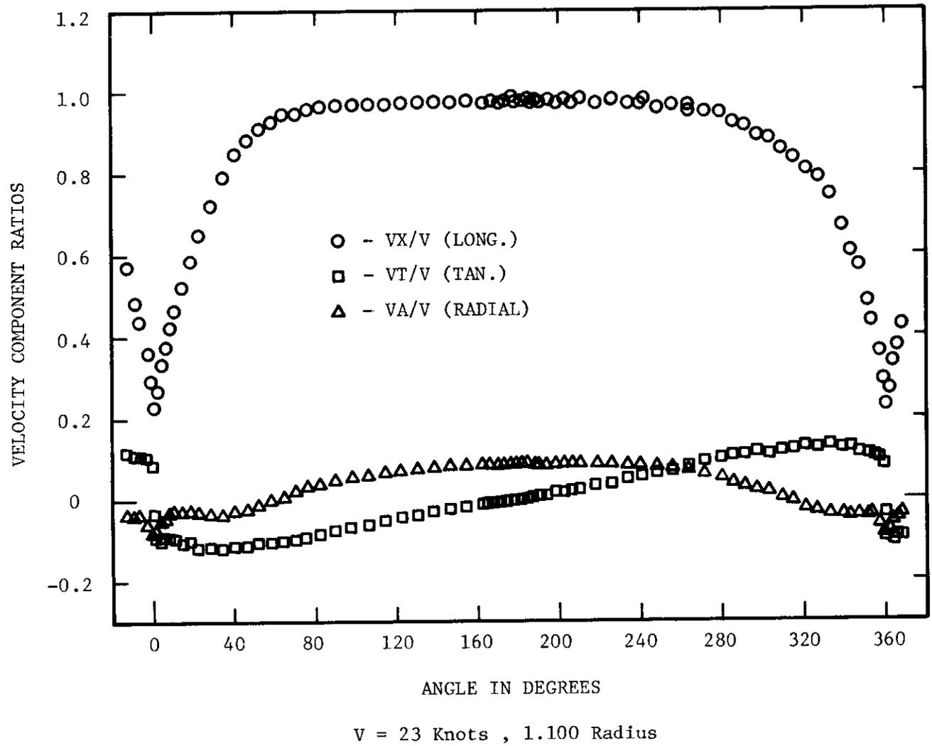
FIGURE F5. LONGITUDINAL, TANGENTIAL, AND AXIAL WAKES AT 1.100 RADIUS
