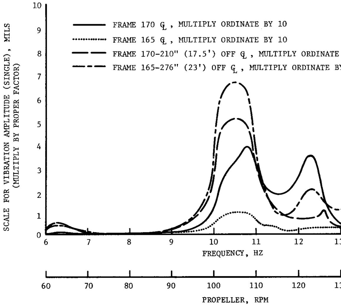
FIGURE 44. VERTICAL VIBRATION ON 36-FT FLAT GENERATED BY AXIAL PROPELLER FORCE
