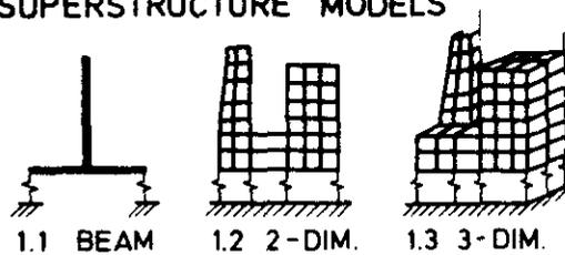
FIGURE 11. THREE LEVELS OF SUPERSTRUCTURE MATHEMATICAL MODELS, FROM [75]
