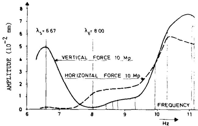
FIGURE 19. CALCULATED FORCED RESPONSE AT THE TOP OF SUPERSTRUCTURE IN LONGITUDINAL DIRECTION. 370,000 DWT TANKER, BALLAST CONDITION, FROM [75].
