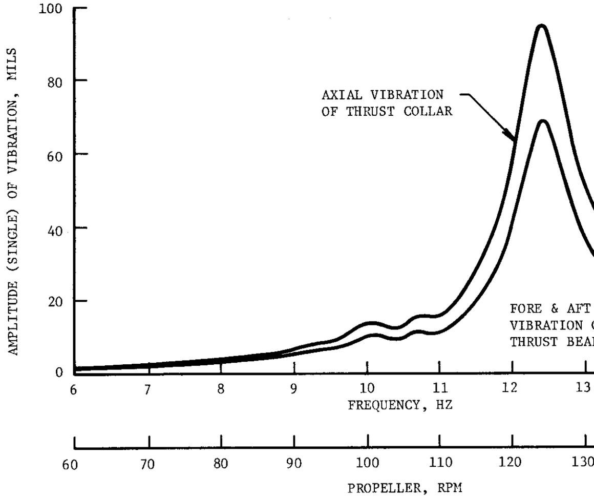
FIGURE 42. AMPLITUDE OF FORE AND AFT VIBRATION AT PROPULSION
