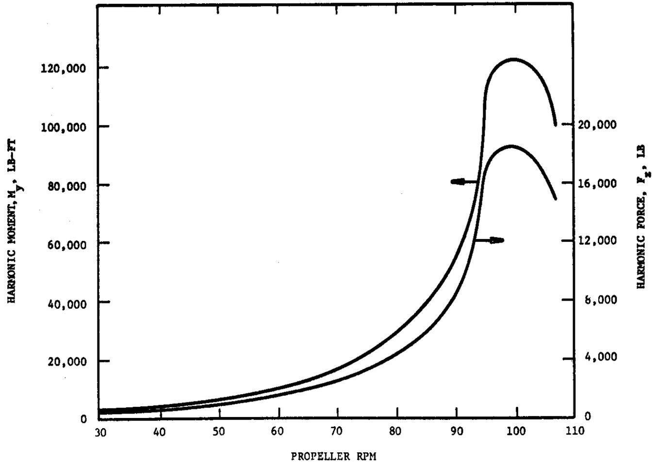
FIGURE 37. VERTICAL HARMONIC FORCE AND TRANSVERSE BENDING MOMENT GENERATED ON HULL BY THE PROPELLER
