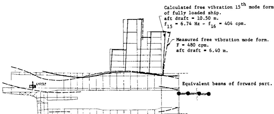
FIGURE 21. ELASTO DYNAMIC MODEL OF AFT PART AND CORRELATION OF EXCITER TESTS WITH FREE VIBRATION CALCULATIONS, FROM [94]
