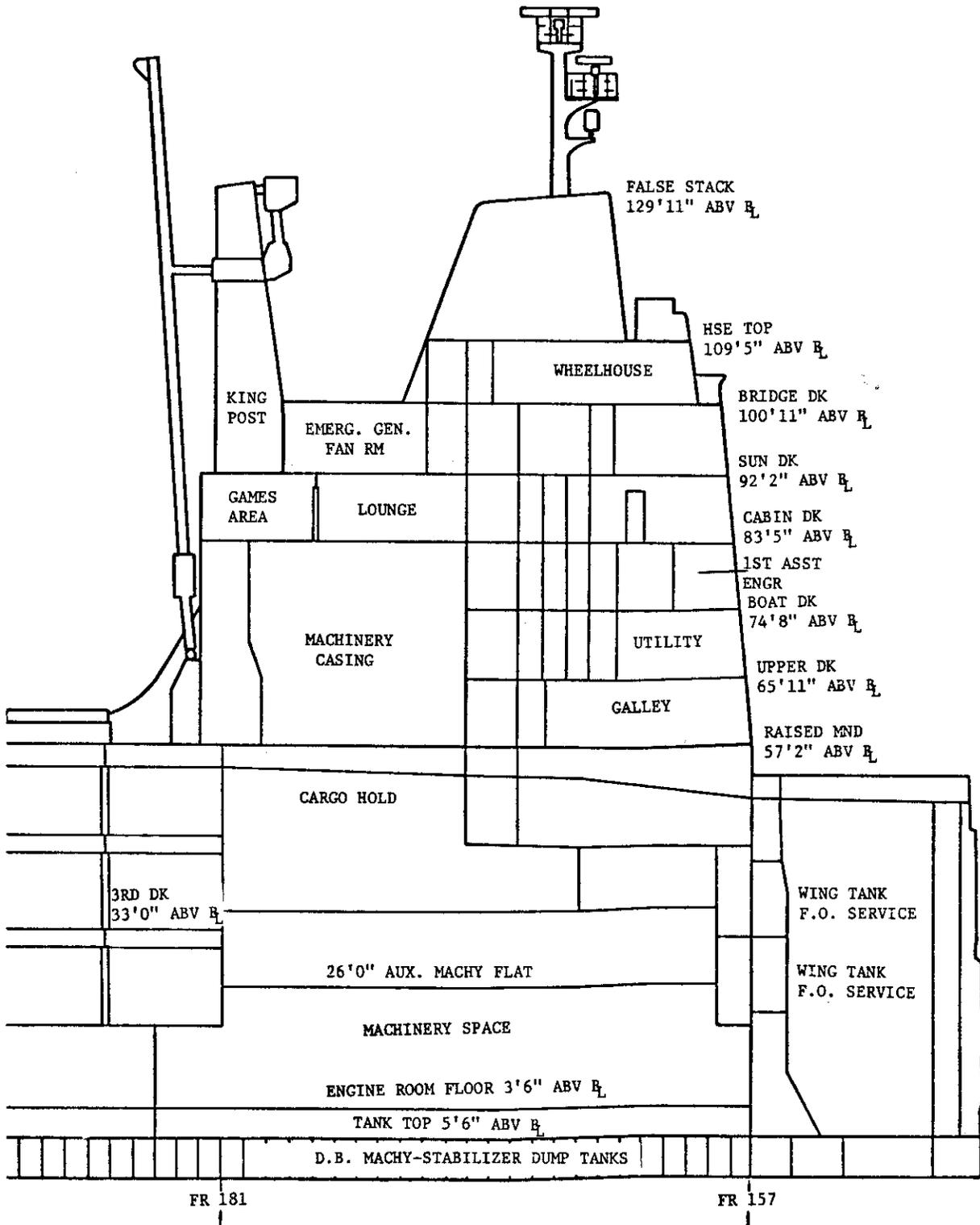
FIGURE 38. INBOARD PROFILE
