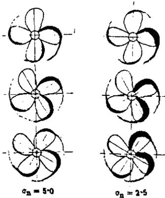
FIGURE 6. CAVITATION PROPERTIES OF MODEL
