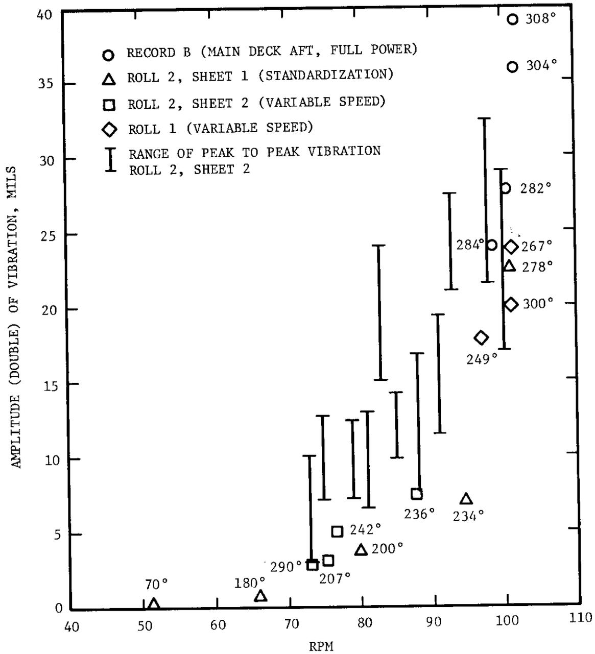
FIGURE 48. DOUBLE AMPLITUDE OF SIXTH ORDER, FORE AND AFT MOTION OF THRUST BEARING FOUNDATION
