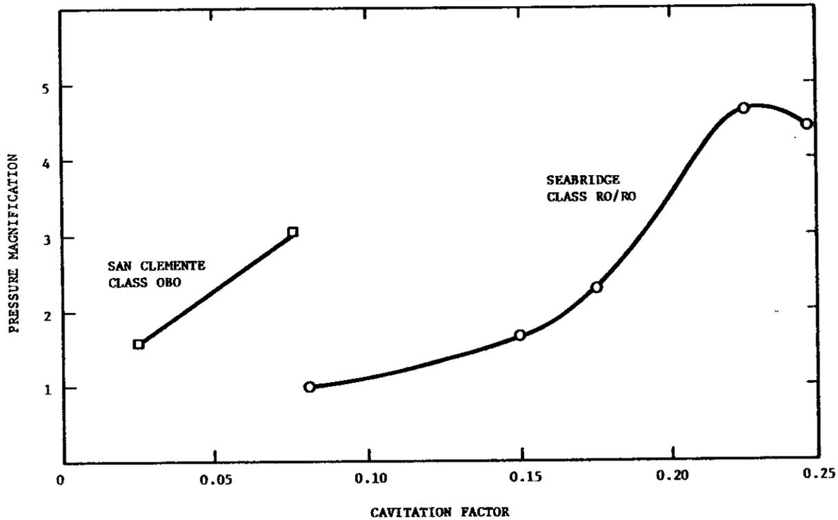
FIGURE 36. RATIO OF MEASURED HULL PRESSURES WHERE CAVITATION EXISTS TO CALCULATED, NONCAVITATING PRESSURES
