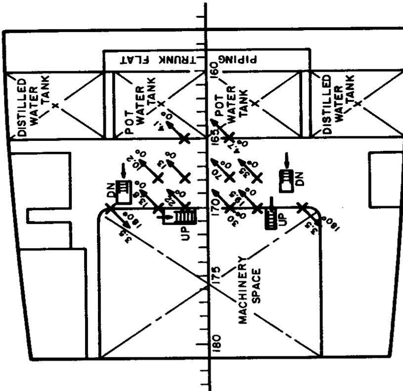
FIGURE 51. VIBRATION ON 36-FT FLAT AT ABOUT 100 RPM
