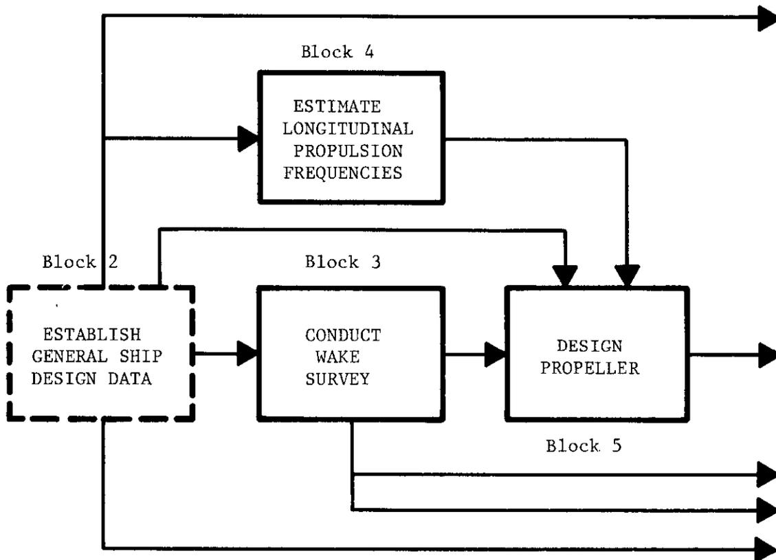
FIGURE 22. PRELIMINARY HYDRODYNAMIC DESIGN PHASE
