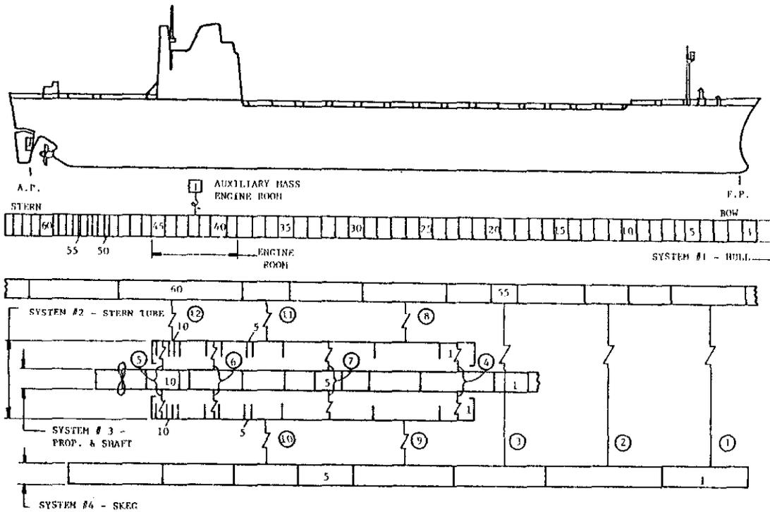
FIGURE 14. UNITIZED AND CONTAINERIZED SHIP, TRANSVERSE VIBRATION MODEL
