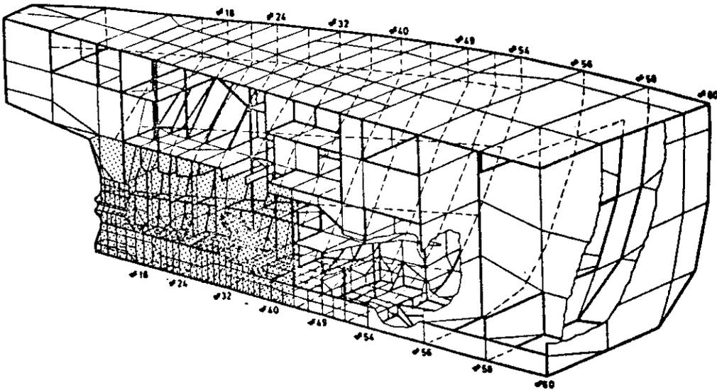
(b) Aft bearing structure is shaded
