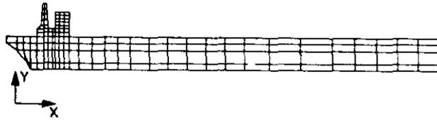
FIGURE 17. FINITE-ELEMENT MESH FOR TWO-DIMENSIONAL MODEL OF 370,000 DWT TANKER, FROM [75].
