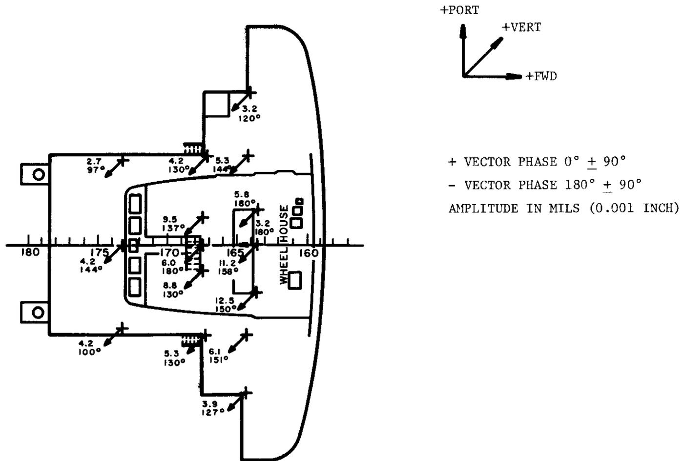
FIGURE 52. VIBRATION OF BRIDGE DECK AT ABOUT 98.6 RPM
