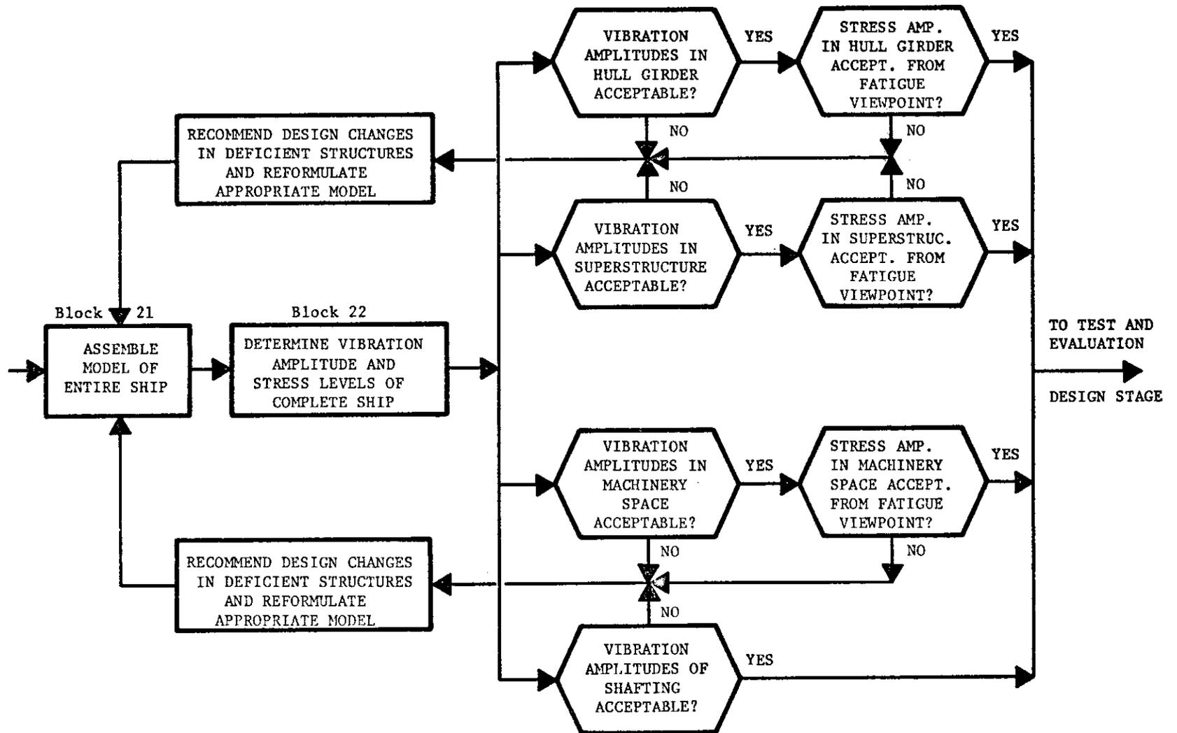
FIGURE 30. MILESTONE IV - COMPLETE SHIP STRUCTURE EVALUATION
