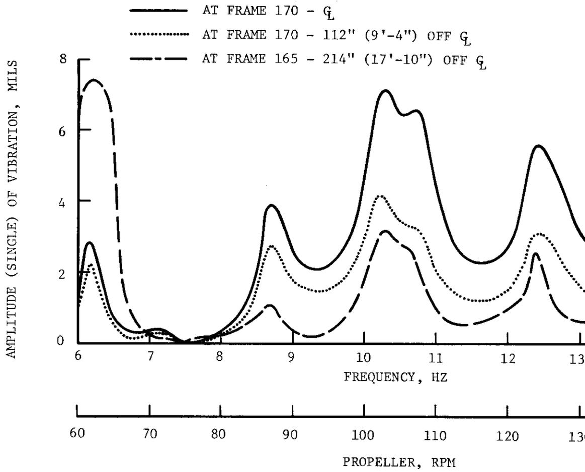
FIGURE 45. VERTICAL VIBRATION ON 26-FT FLAT EXCITED BY AXIAL HARMONIC FORCE AT THE PROPELLER
