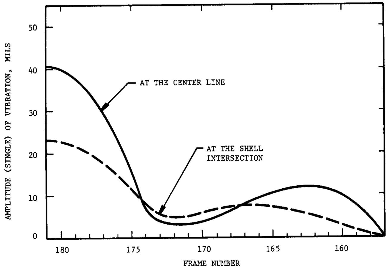
FIGURE 46. VERTICAL VIBRATION IN TANK TOP DUE TO LONGITUDINAL EXCITATION AT THE PROPELLER AT 12.43 HZ (Frequency of Longitudinal Shaft Resonance)
