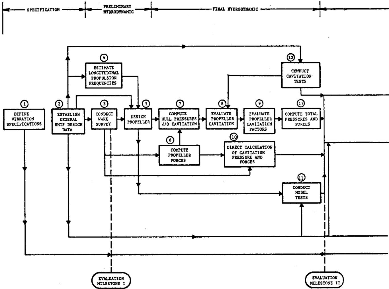
FIGURE 3. FLOW DIAGRAM OF RECOMMENDED DESIGN
