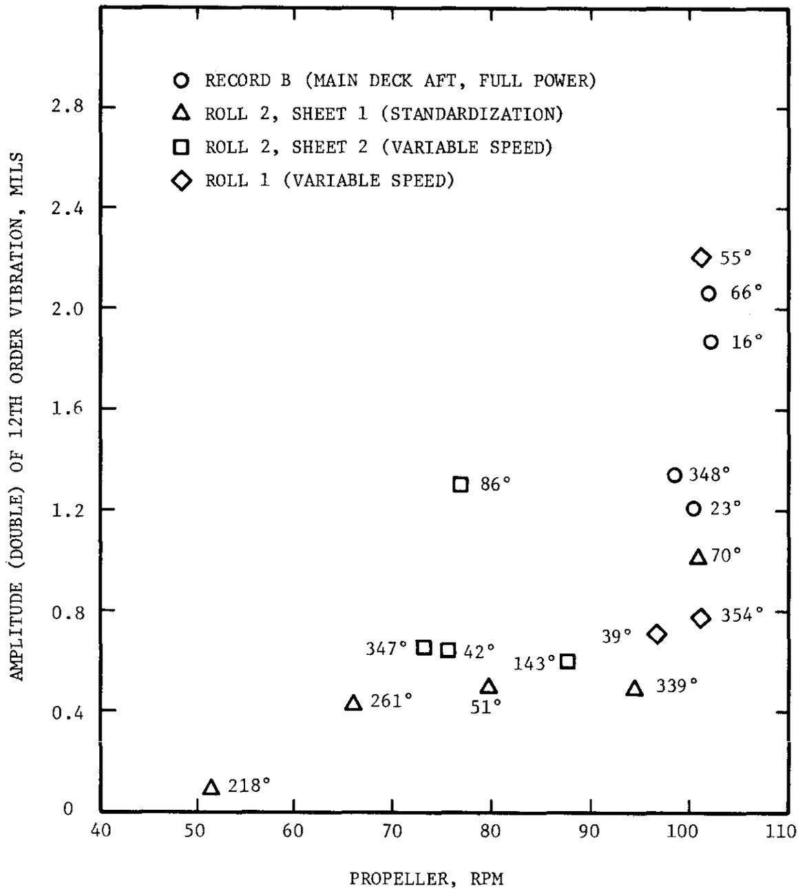
FIGURE 49. DOUBLE AMPLITUDE OF TWELFTH ORDER, FORE AND AFT VIBRATION ON THRUST BEARING FOOT
