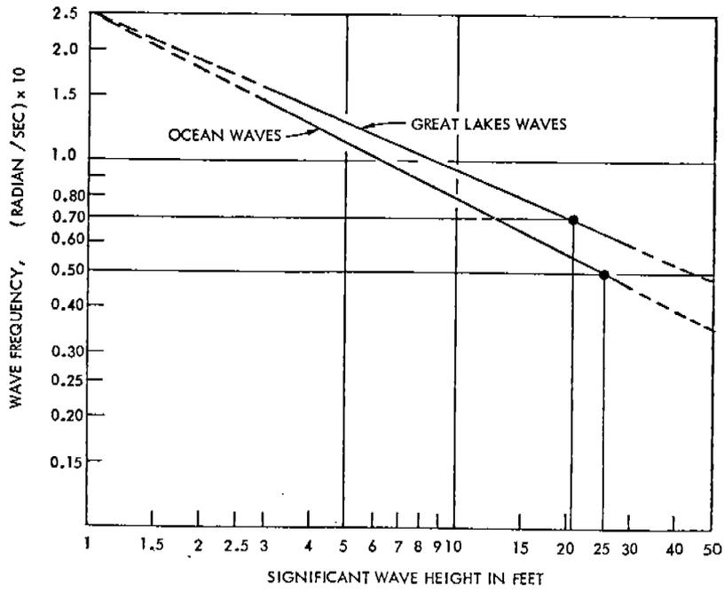
Figure 2 - Significant Wave Height VS. Peak Energy Frequency.
