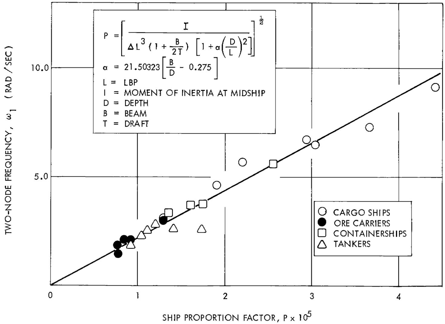
FIGURE 46 - EFFECT OF SHIP PROPORTIONS ON THE HULL FLEXIBILITY ( REPRESENTED BY THE TWO-NODE FREQUENCY )
