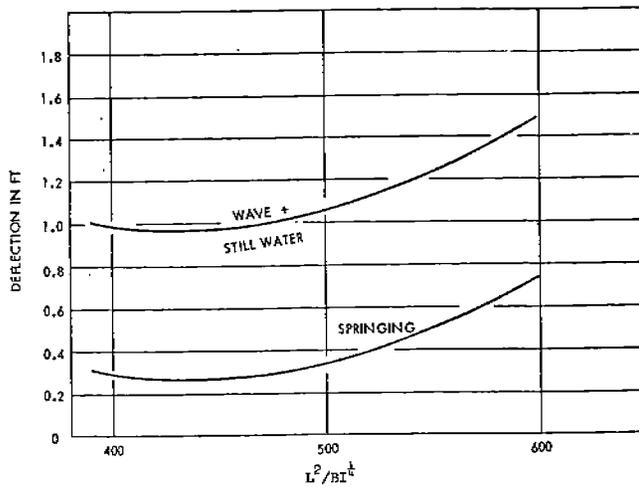
Fig. 34 - Effect of  $L^2/BI^4$  on Deflection for Containerships, Full Load Condition
