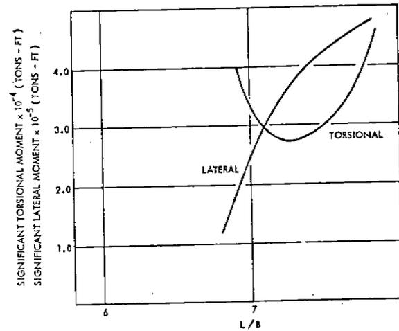
Fig. 33 - Effect of L/B on Torsional and Lateral Moment for Containerships, Full Load Condition
