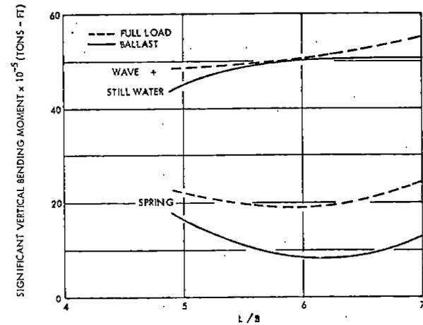
Fig. 15 - Effect of L/B on Vertical Bending Moment for Tank Vessels
