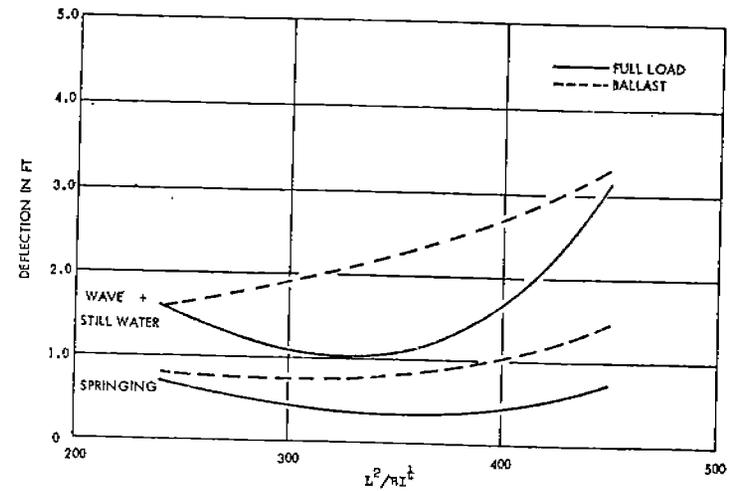
Fig. 17 - Effect of  $L^2/BI^{1/4}$  on Deflection for Tank Vessels
