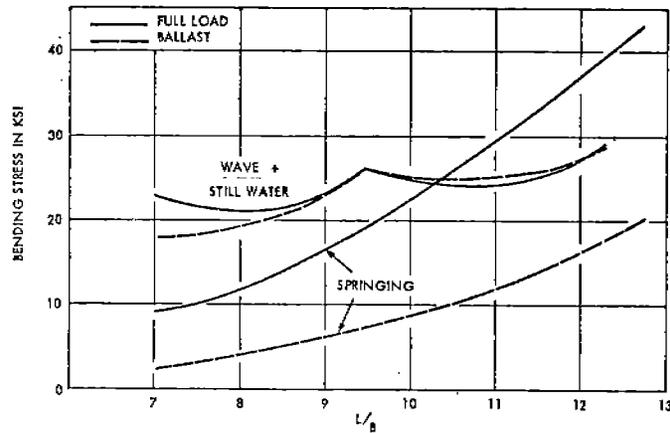
Fig. 6 - Effect of L/B on Bending Stress for Great Lakes Ore Carriers
