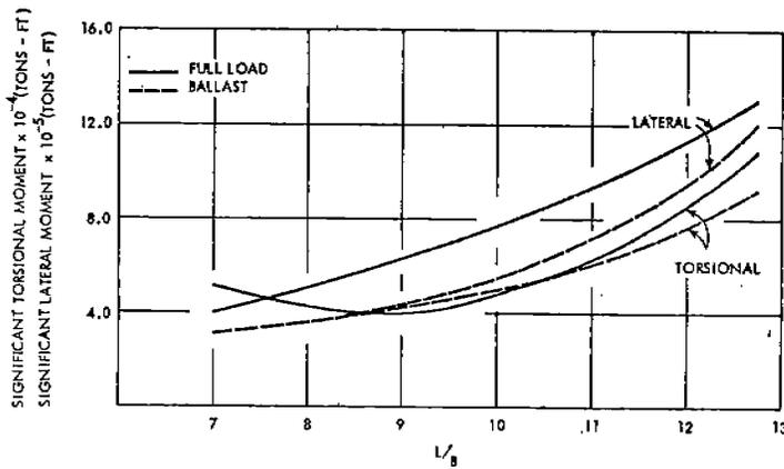
Fig. 8 - Effect of L/B on Lateral and Torsional Moment for Great Lakes Ore Carriers
