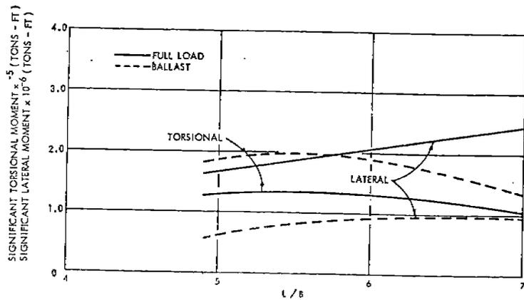
Fig. 16 - Effect of L/B on Torsional and Lateral Bending Moment for Tank Vessels
