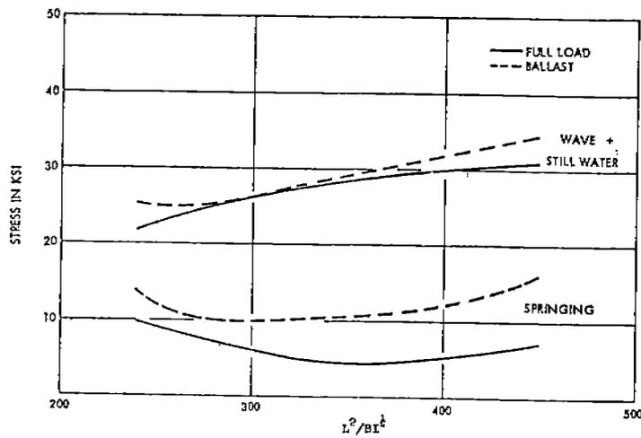
Fig. 18 - Effect of  $L^2/BI^{1/4}$  on Bending Stress for Tank Vessels
