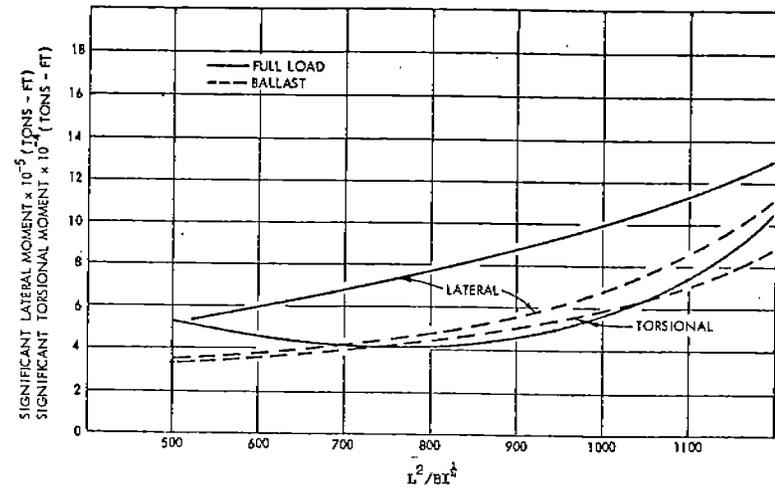
Fig. 11 - Effect of  $L^2/BI^{1/4}$  on Lateral and Torsional Moment for Great Lakes Ore Carriers
