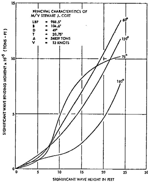
Fig. 40 - Effect of Wave Height and Heading on Sea Loads of Great Lakes Ore Carrier, Ballast Condition
