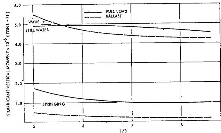
Fig. 23 - Effect of L/B on Vertical Bending Moment for Cargo Ships
