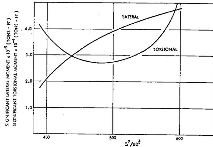
Fig. 37 - Effect of  $L^2/BI^{1/4}$  on Lateral and Torsional Moment for Containerships, Full Load Condition
