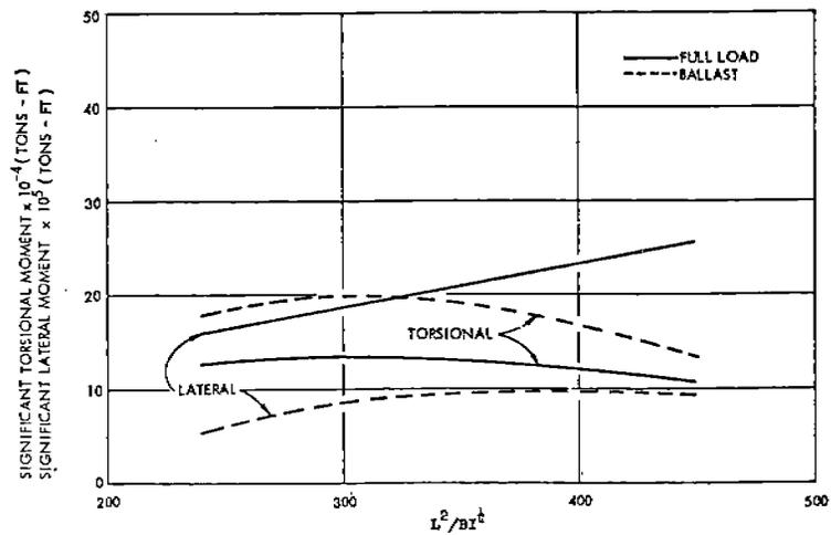
Fig. 20 - Effect of  $L^2/BI^4$  on Lateral and Torsional Moment for Tank Vessels
