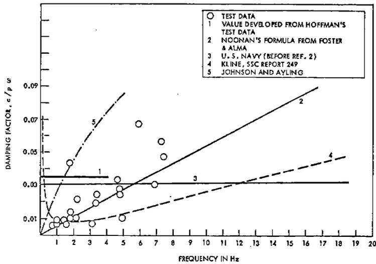
Fig. 4 - Damping Coefficients Used by Various Investigators
