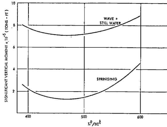
Fig. 36 - Effect of  $L^2/BI^{1/4}$  on Vertical Bending Moment for Containerships, Full Load Condition
