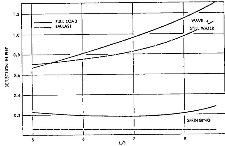
Fig. 21 - Effect of L/B on Deflection for Cargo Ships
