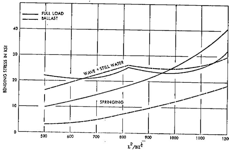
Fig. 10 - Effect of  $L^2/BI^{1/4}$  on Bending Stress for Great Lakes Ore Carriers
