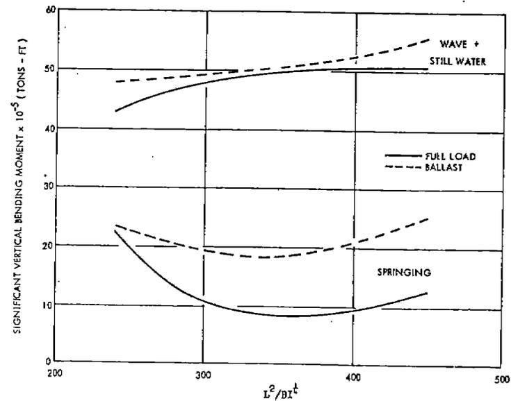
Fig. 19 - Effect of  $L^2/BI^{1/4}$  on Vertical Moment for Tank Vessels
