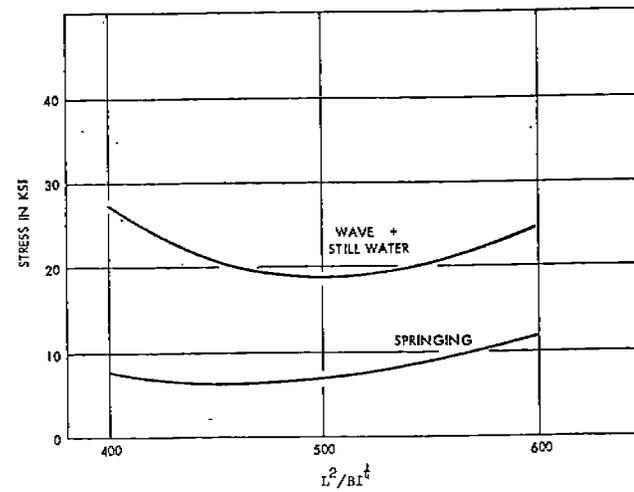
Fig. 35 - Effect of  $L^2/BI^4$  on Bending Stress for Containerships, Full Load Condition
