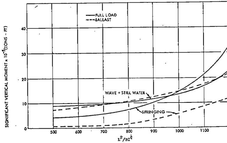
Fig. 12 - Effect of  $L^2/BI^{3/4}$  on Vertical Moment for Great Lakes Ore Carriers
