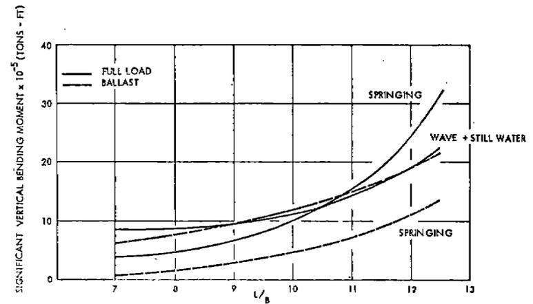
Fig. 7 - Effect of L/B on Vertical Bending Moment for Great Lakes Ore Carriers
