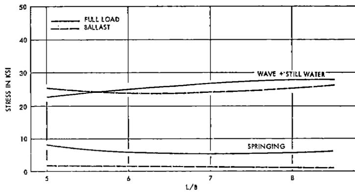
Fig. 22 - Effects of L/B on Vertical Bending Stress for Cargo Ships
