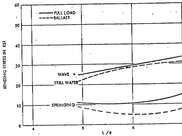
Fig. 14 - Effect of L/B on Bending Stress for Tank Vessels
