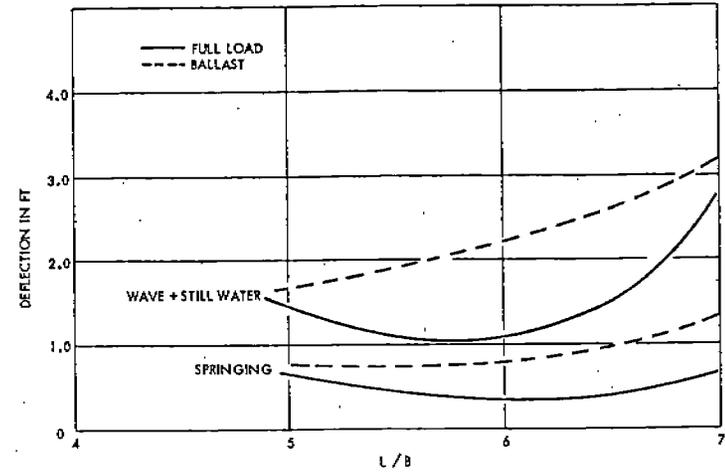
Fig. 13 - Effect of L/B On Deflection for Tank Vessels
