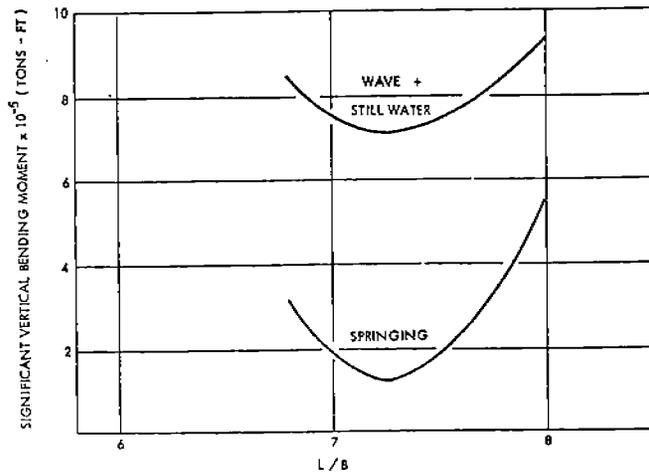
Fig. 32 - Effect of L/B on Vertical Bending Moment for Containerships, Full Load Condition
