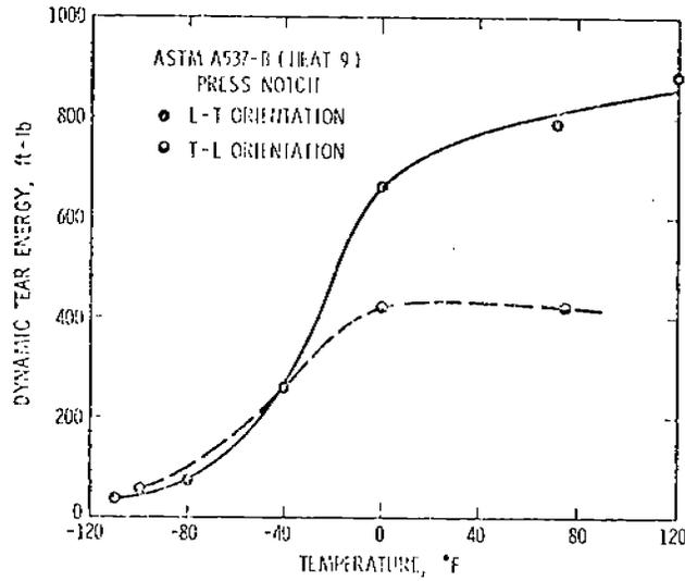
Figure 42. A537-B (Heat 9), 5/8" Parent DT, Press-Notch
