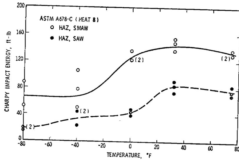
Figure 31. A678-C (Heat 8),  $C_V$ , HAZ
