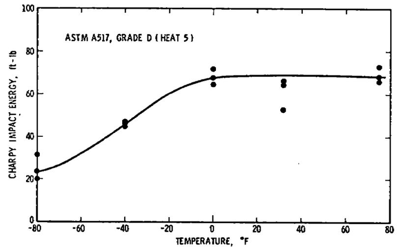
Figure 19. ASTM A517, Grade D (Heat 5) Parent Material CVN
