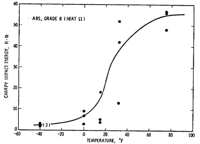
Figure 25. ABS, Grade B (Heat 11) Parent Material CVN
