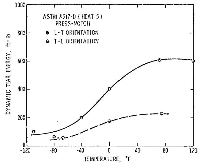
Figure 38. A517-D (Heat 5), 5/8" Parent DT, Press-Notch
