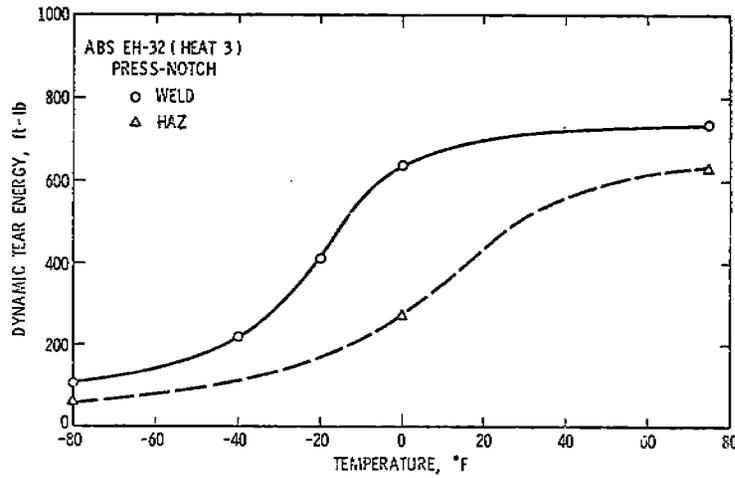
Figure 45. EH-32 (Heat 3), 5/8" Weldment DT, Press-Notch
