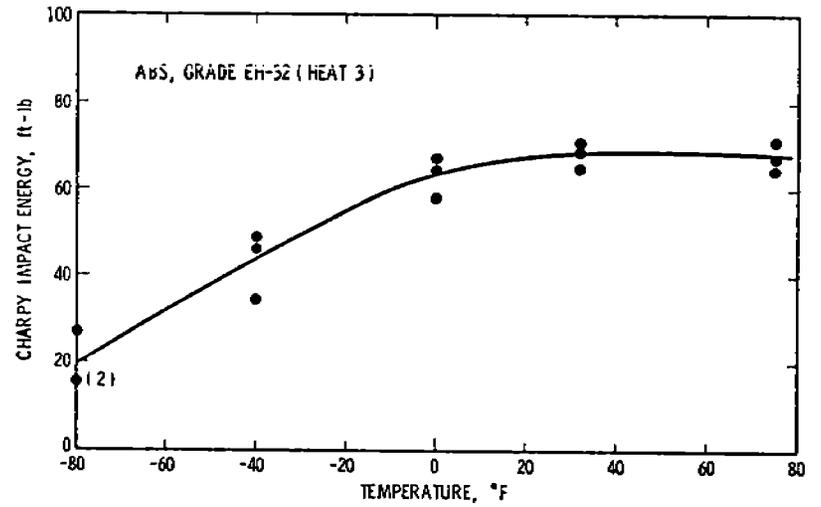
Figure 17. ABS, Grade EH-32 (Heat 3) Parent Material CVN
