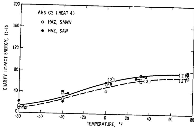
Figure 29. ABS-CS (Heat 4),  $C_V$ , HAZ
