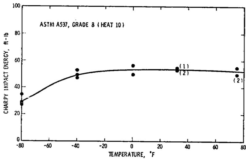
Figure 24. ASTM A537, Grade B (Heat 10) Parent Material CVN
