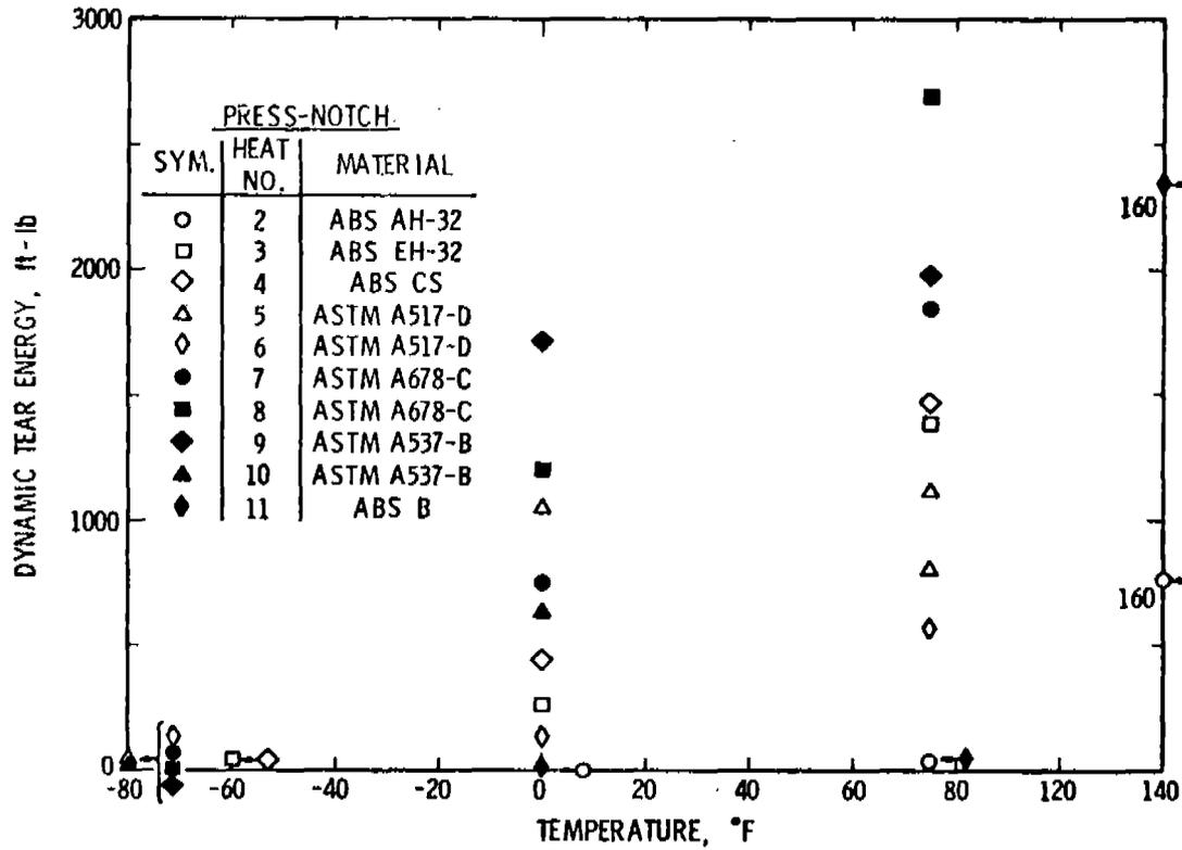
Figure 53. 1" Parent DT, Press-Notch.
