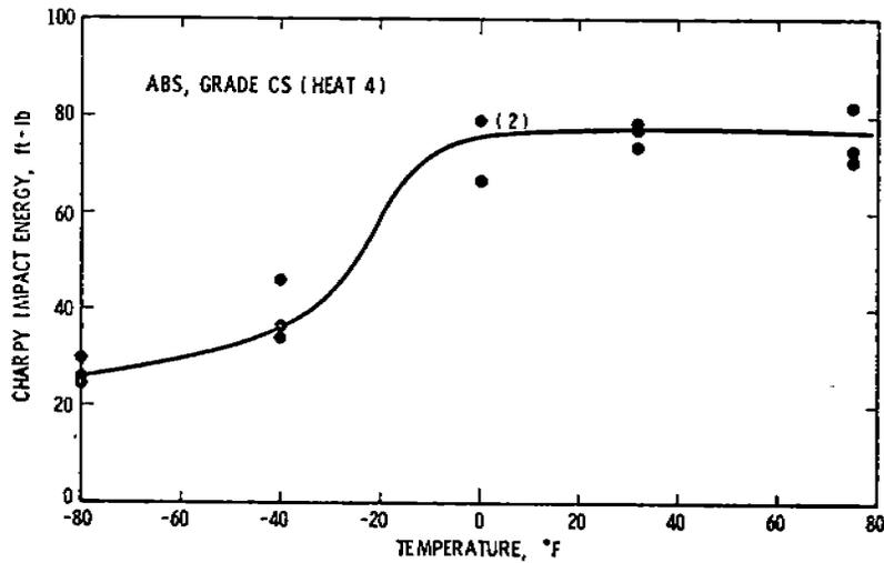
Figure 18. ABS, Grade CS (Heat 4) Parent Material CVN
