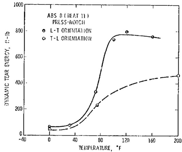
Figure 44. ABS-B (Heat 11), 5/8" Parent DT, Press-Notch
