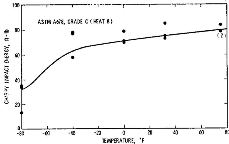
Figure 22. ASTM A678, Grade C (Heat 8) Parent Material CVN
