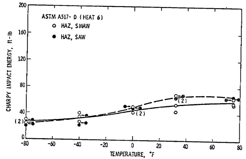
Figure 30. A517-D (Heat 6),  $C_V$ , HAZ
