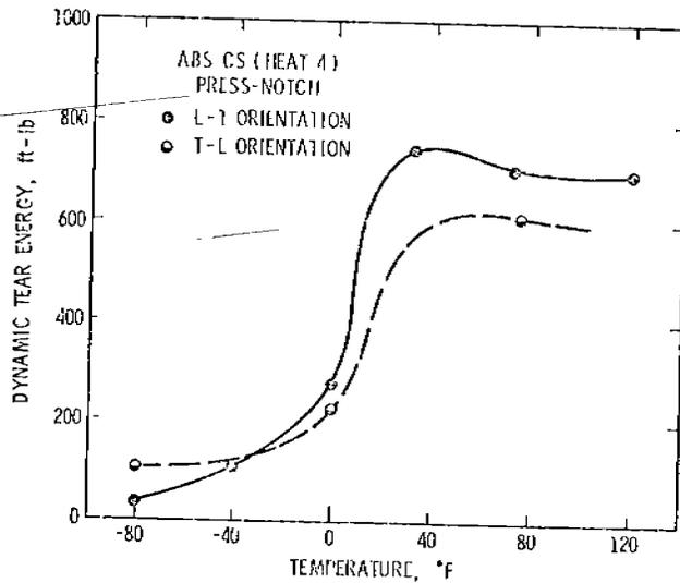
Figure 37. ABS-CS (Heat 4), 5/8" Parent DT, Press-Notch
