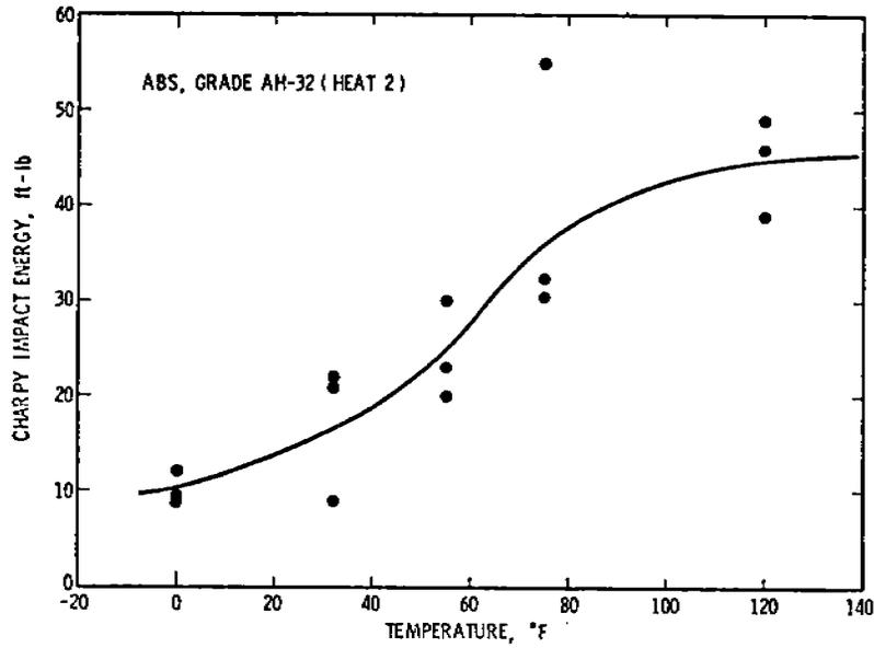
Figure 16. ABS, Grade AH-32 (Heat 2) Parent Material CVN
