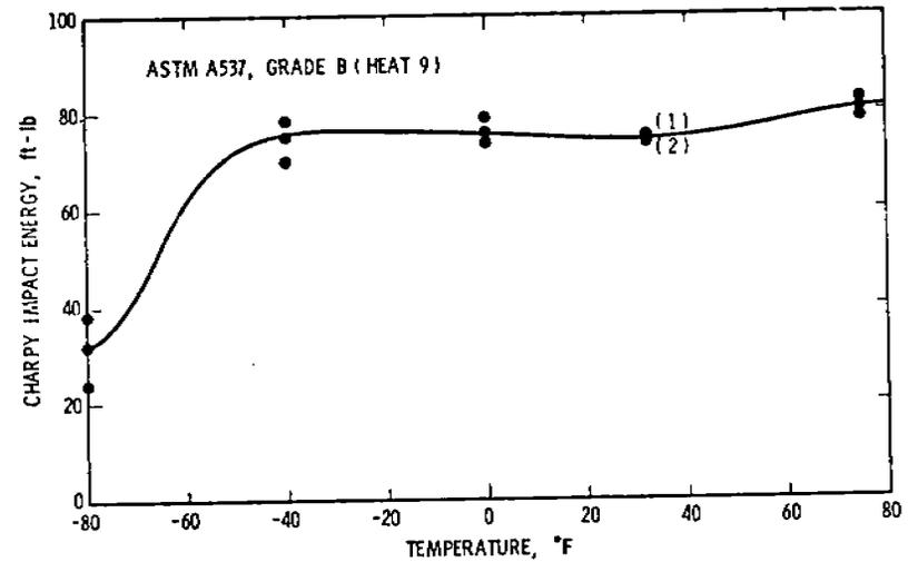
Figure 23. ASTM A537, Grade B (Heat 9) Parent Material CVN
