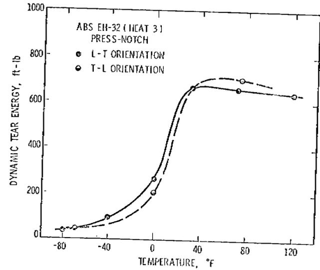
Figure 36. EH-32 (Heat 3), 5/8" Parent DT, Press-Notch
