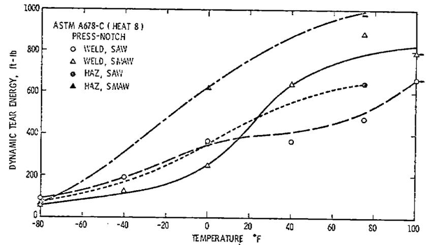
Figure 48. A678-C (Heat 8), 5/8" Weldment DT, Press-Notch
