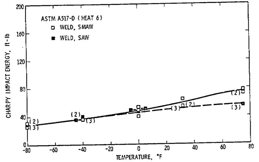
Figure 33. A517-D (Heat 6),  $C_V$ , Weld
