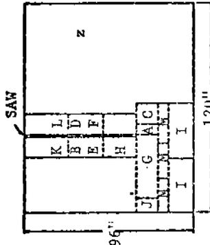
Fig. 3. Plate No. 3 - ABS Gr EH-32, 1" Thick
