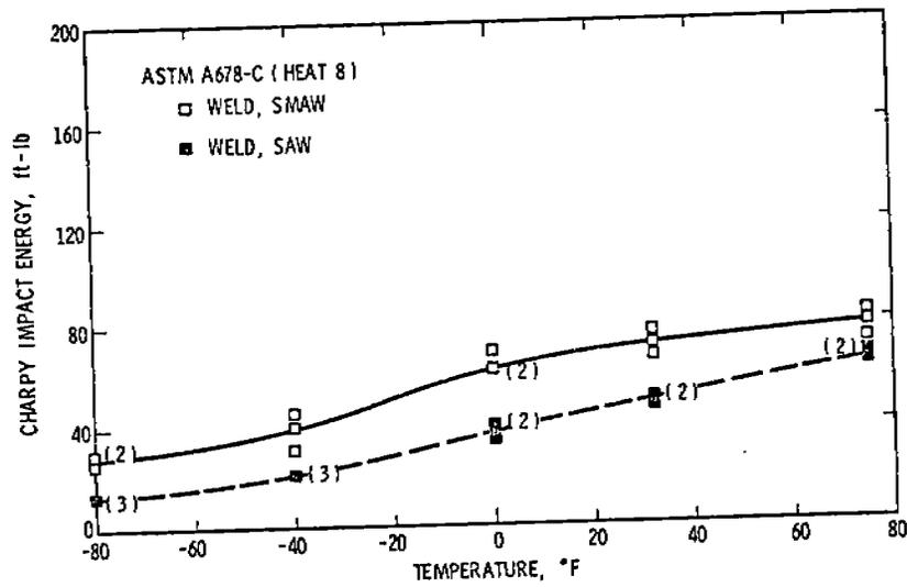
Figure 34. A678-C (Heat 8),  $C_V$ , Weld
