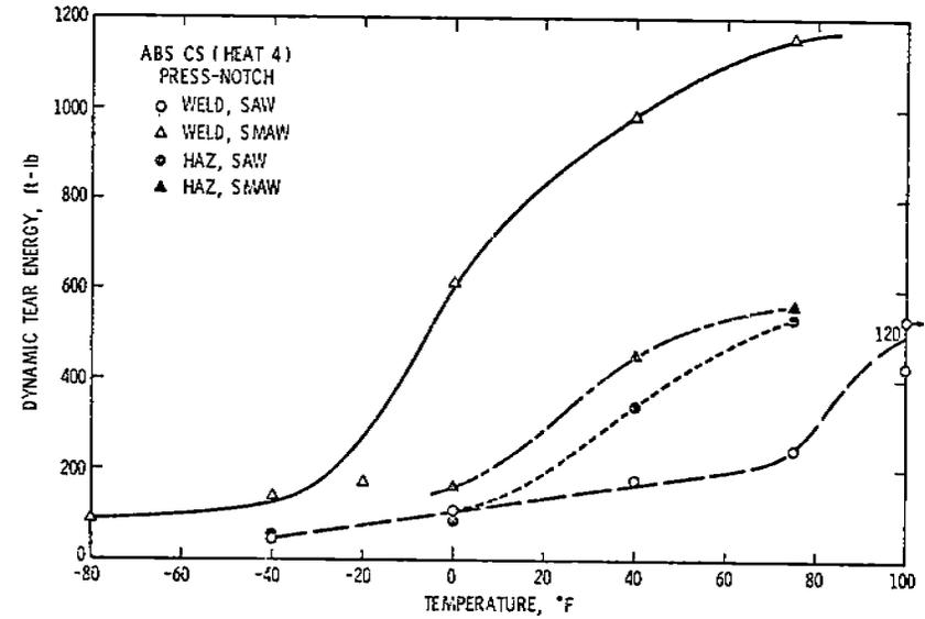
Figure 46. ABS-CS (Heat 4), 5/8" Weldment DT, Press-Notch
