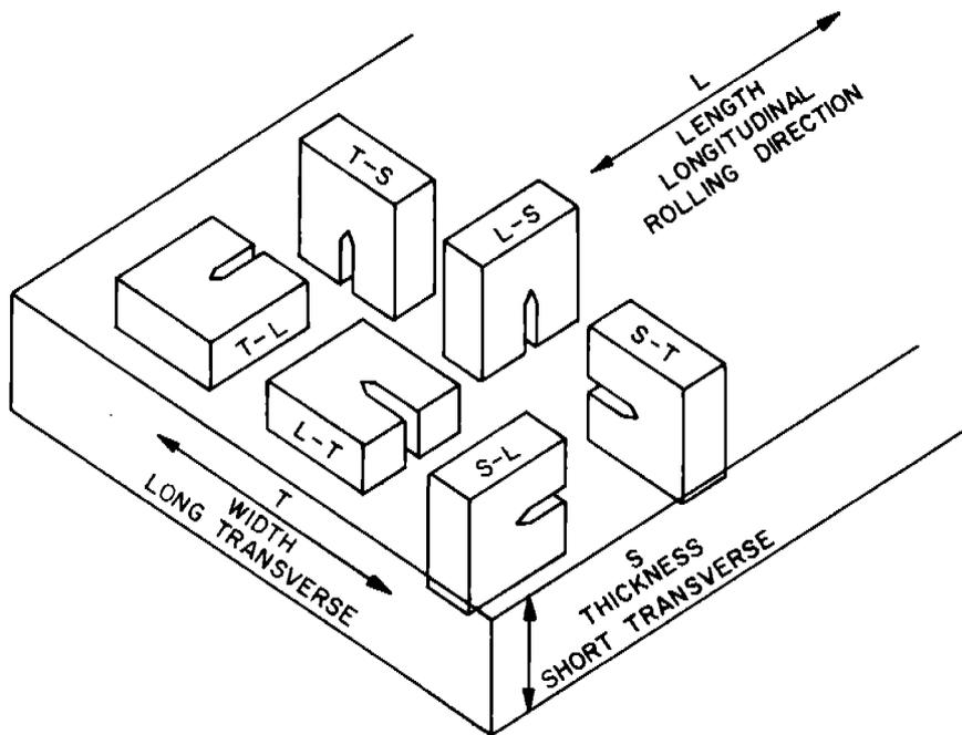
Figure 13. Specimen Orientation Code
