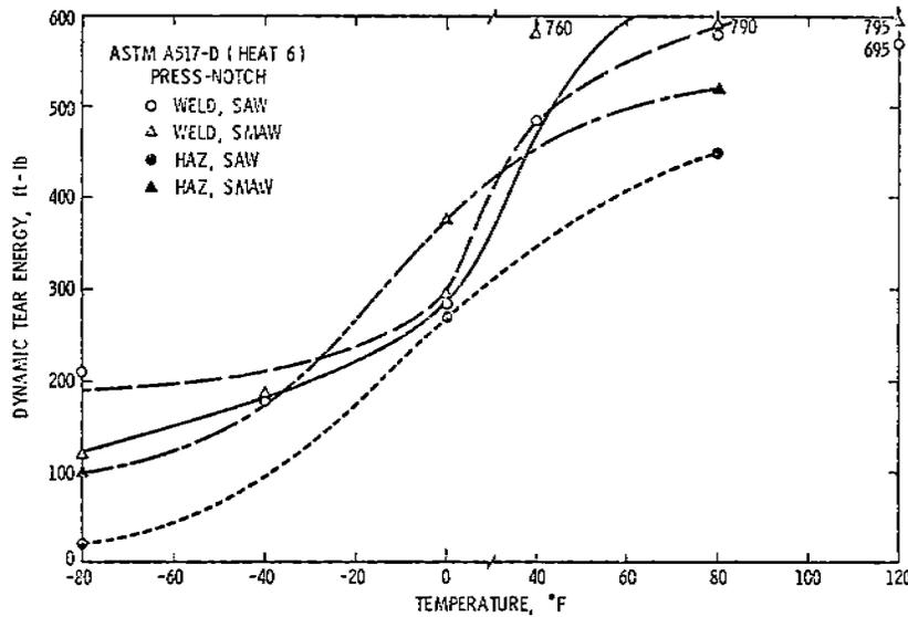
Figure 47. A517-D (Heat 6), 5/8" Weldment DT, Press-Notch
