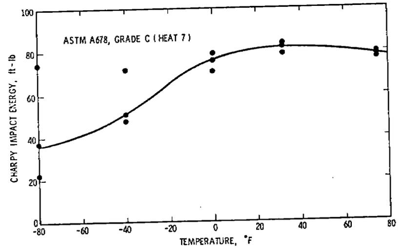
Figure 21. ASTM A678, Grade C (Heat 7) Parent Material CVN
