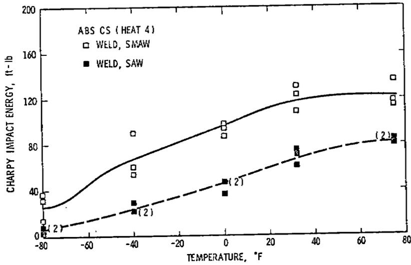
Figure 32. ABS-CS (Heat 4),  $C_V$ , Weld
