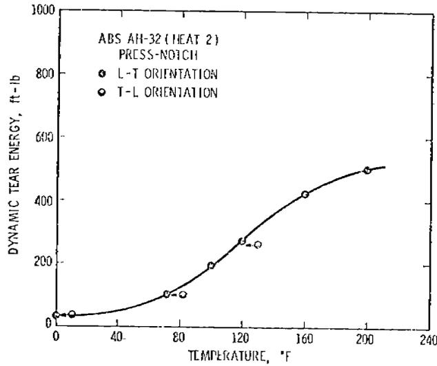
Figure 35. 5/8" Parent DT, Press-Notch, AH-32 (Heat 2)
