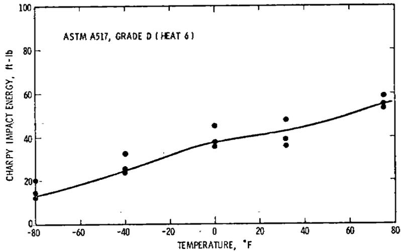
Figure 20. ASTM A517, Grade D (Heat 6) Parent Material CVN
