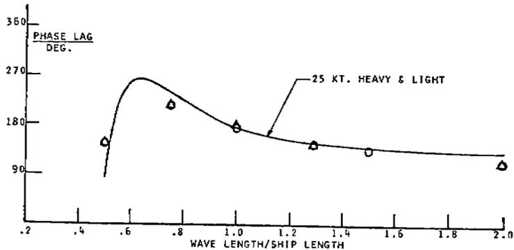
FIGURE 1 - Pitch and phase lag, 180° heading
