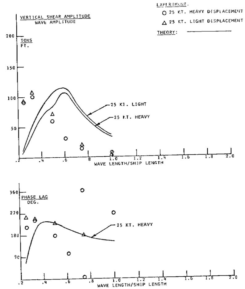
FIGURE 14 - Midship vertical shear and phase lag, 240° heading
