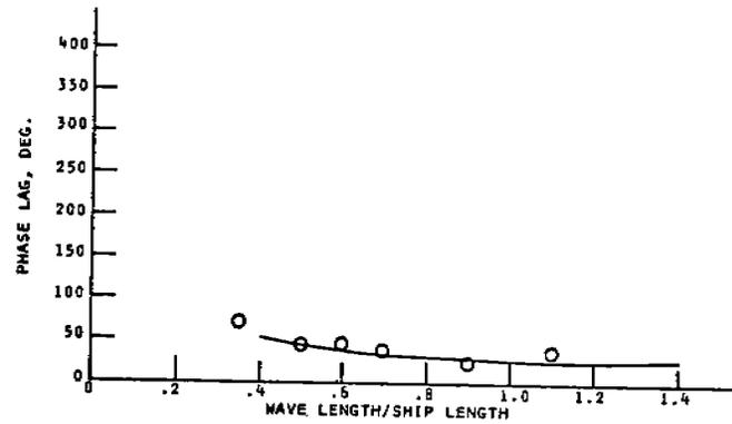
FIGURE 71 - Dutch container ship,  $F_n = .245$ , heading =  $65^\circ$
