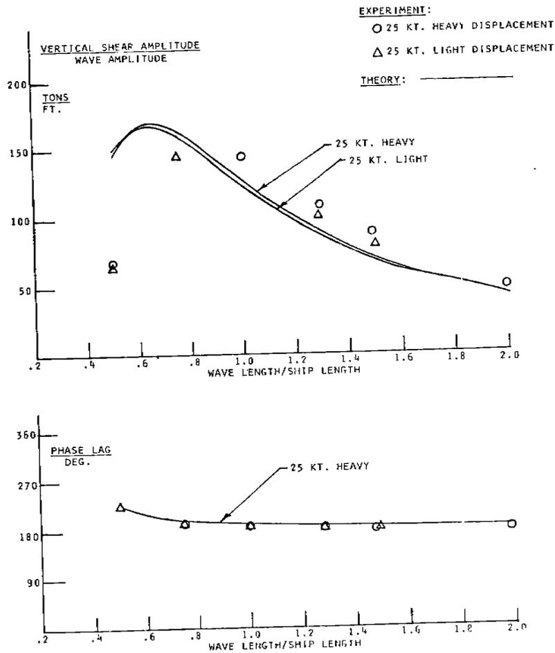
FIGURE 25 - Frame 258 vertical shear and phase lag, 30° heading
