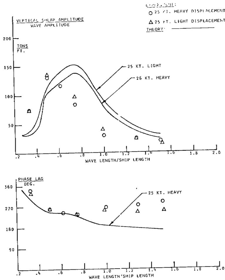
FIGURE 9 - Midship vertical shear and phase lag, 210° heading
