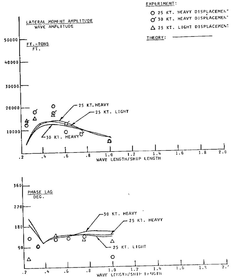
FIGURE 38 - Frame 258 lateral wave bending moments and phase lag, 240° heading
