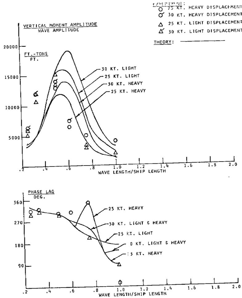
FIGURE 13 - Frame 258 vertical wave bending moment and phase lag, 240° heading
