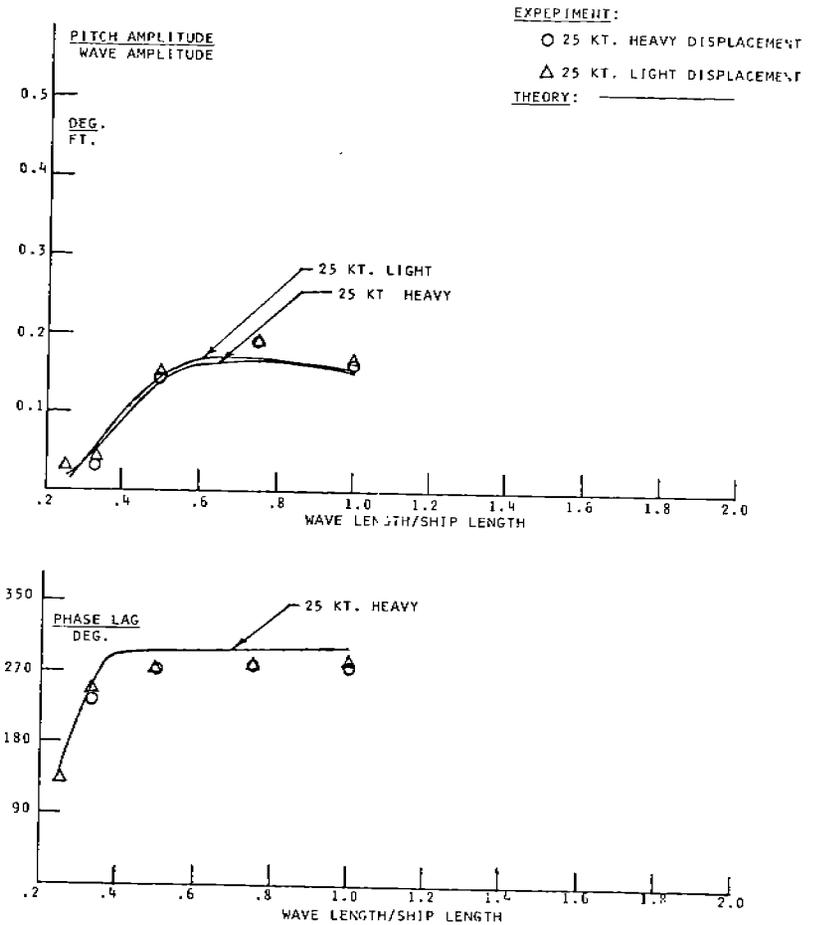
FIGURE 16 - Pitch and phase lag, 60° heading
