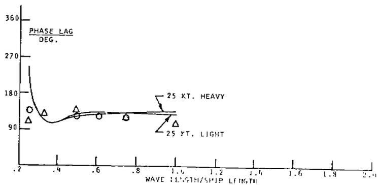
FIGURE 39 - Frame 258 lateral shear and phase, 240° heading
