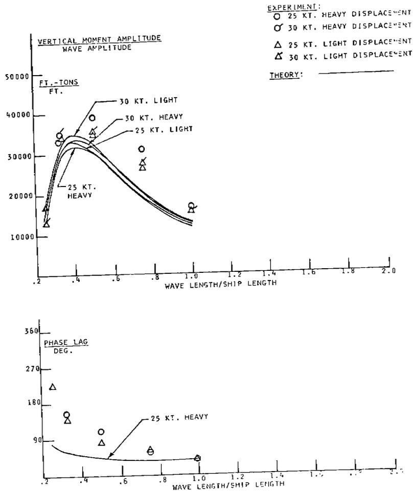
FIGURE 17 - Midship vertical wave bending moments and phase lag, 60° heading
