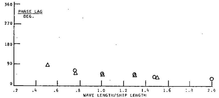
FIGURE 87 - Midship vertical wave bending moments and wave phase lag, 30° heading
