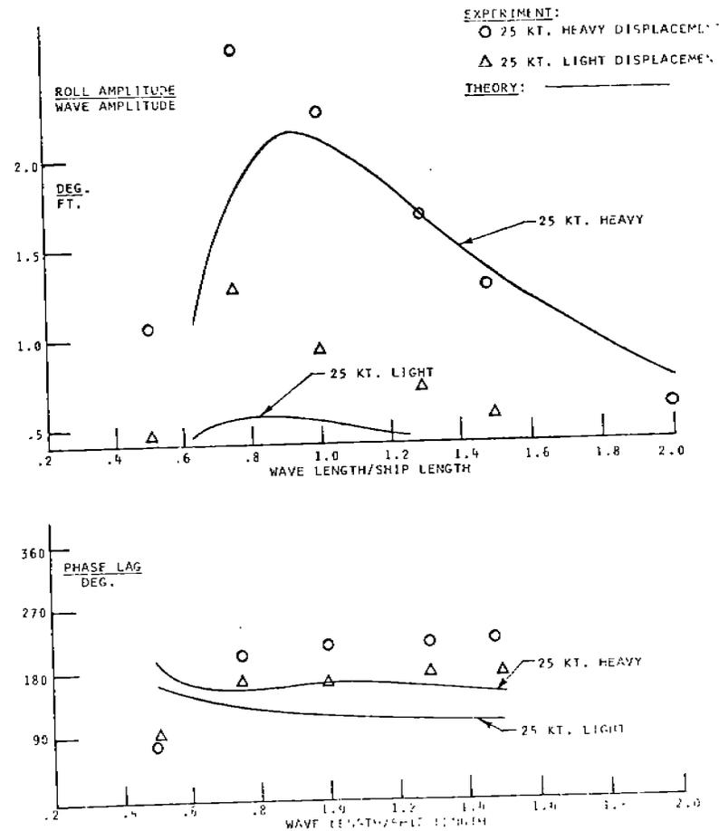
FIGURE 50 - Roll and phase lag, 30° heading.
