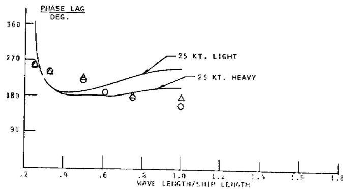
FIGURE 40 - Midship lateral shear and phase lag, 240° heading
