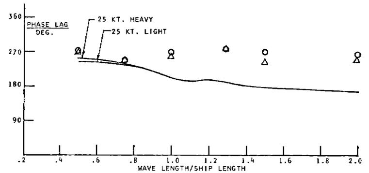
FIGURE 3 - Frame 258 vertical wave bending moments and phase lag, 180° heading
