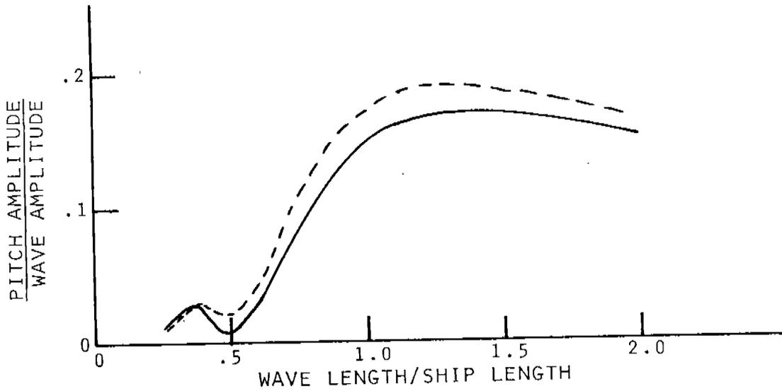
FIGURE 85 - Heave and pitch, 0° heading
