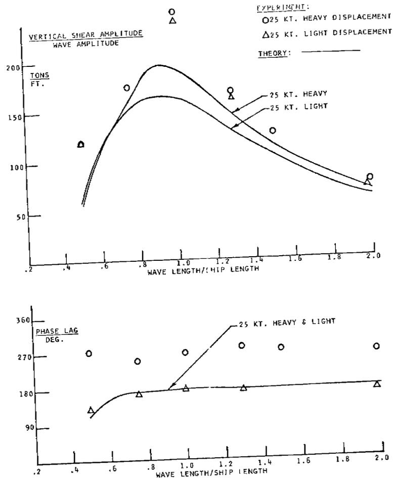
FIGURE 5 - Frame 258 vertical shear and lag, 180° heading
