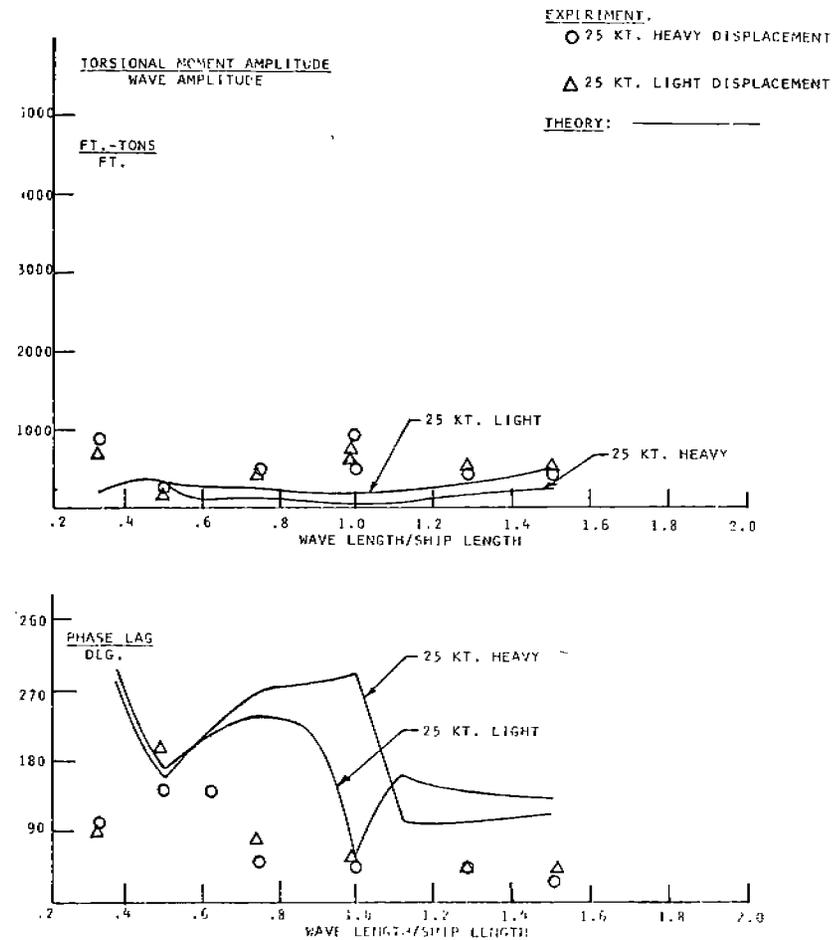
FIGURE 36 - Frame 258 torsional wave bending moments and phase lag, 210° heading
