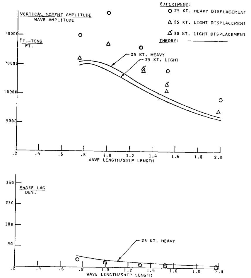
FIGURE 28 - Frame 258 vertical wave bending moments and phase lag, 0° heading
