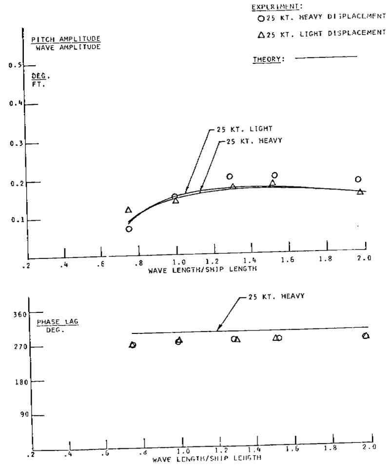
FIGURE 26 - Pitch and phase lag, 0° heading
