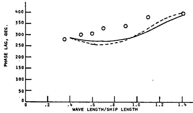
FIGURE 70 - Dutch container ship,  $F_n = .245$ , heading =  $225^\circ$
