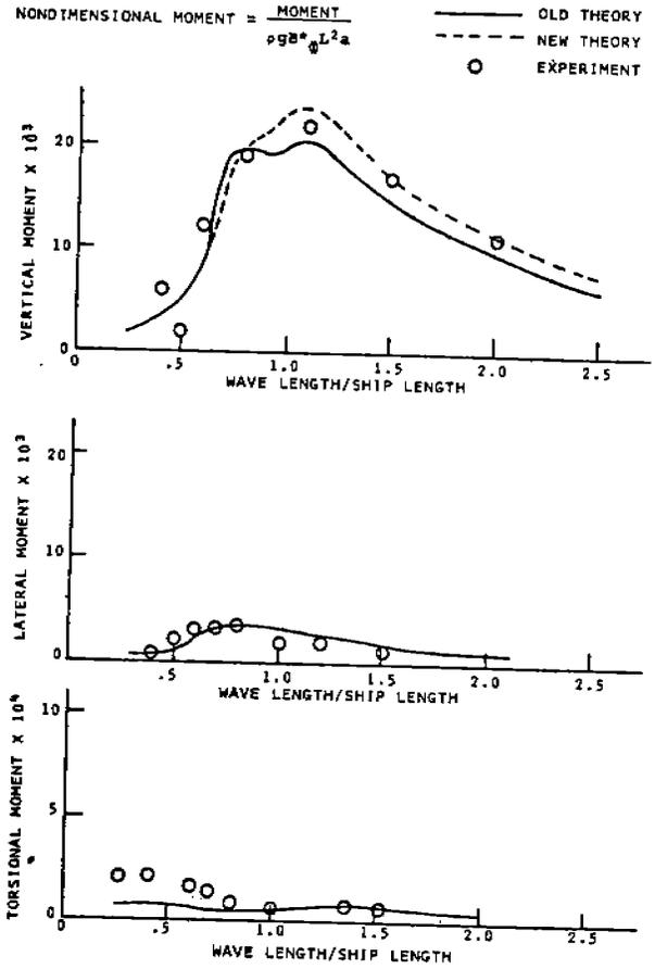
FIGURE 80 - Non-dimensional midship wave moments on Series 60, Block .80 hull,  $F_n = 0.15$ , 170° heading
