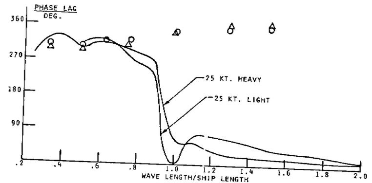
FIGURE 8 - Frame 258 vertical wave bending moments and phase lag, 210° heading
