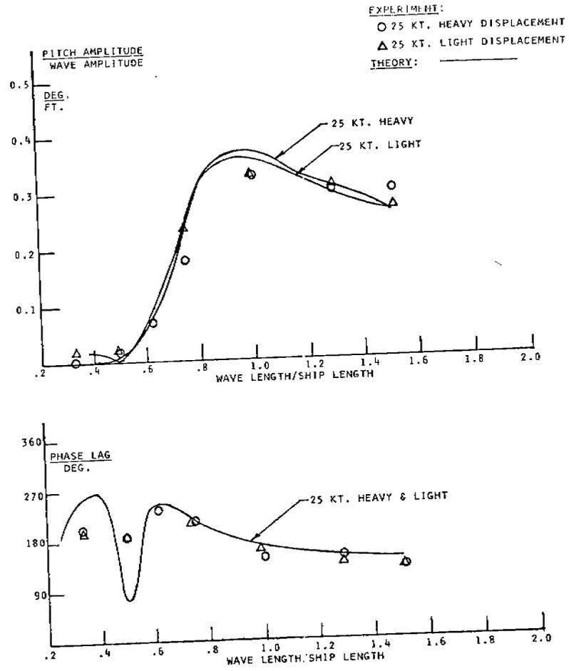
FIGURE 6 - Pitch and phase lag, 210° heading
