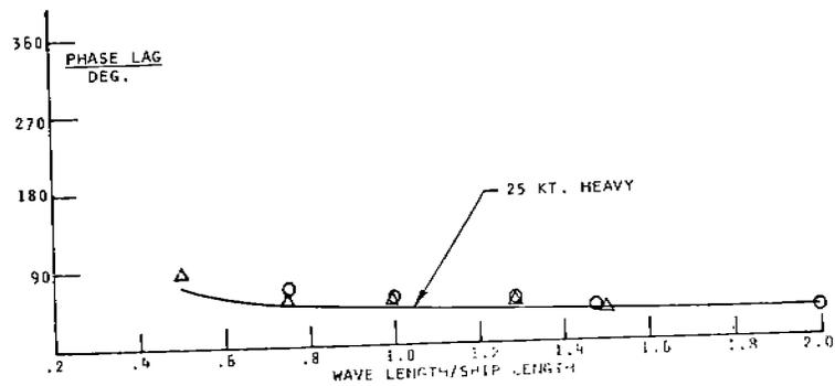
FIGURE 22 - Midship vertical wave bending moments and phase lag, 30° heading
