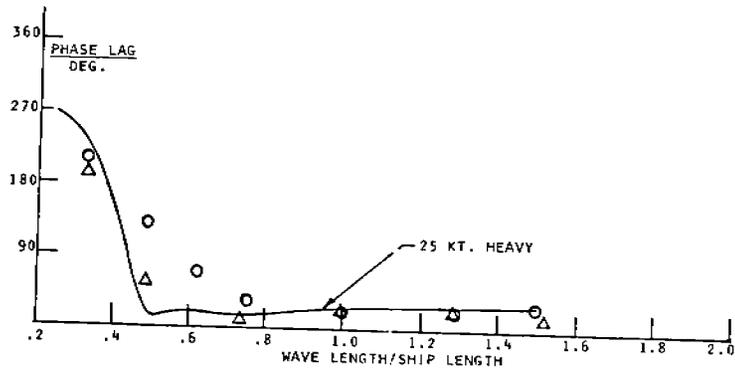
FIGURE 7 - Midship vertical wave bending moments and phase lag, 210° heading
