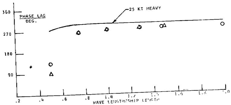
FIGURE 21 - Pitch and phase lag, 30° heading
