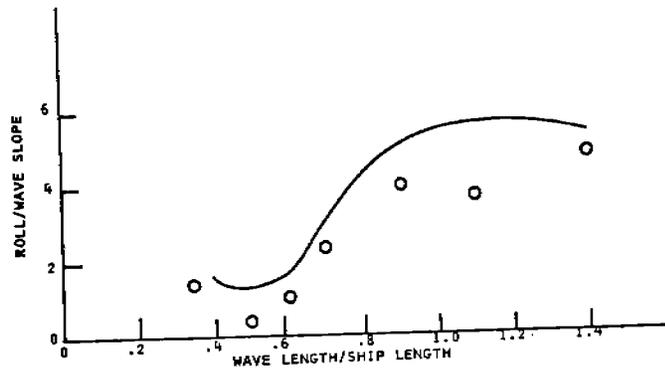
FIGURE 78 - Dutch container ship,  $F_n = .245$ , heading =  $25^\circ$
