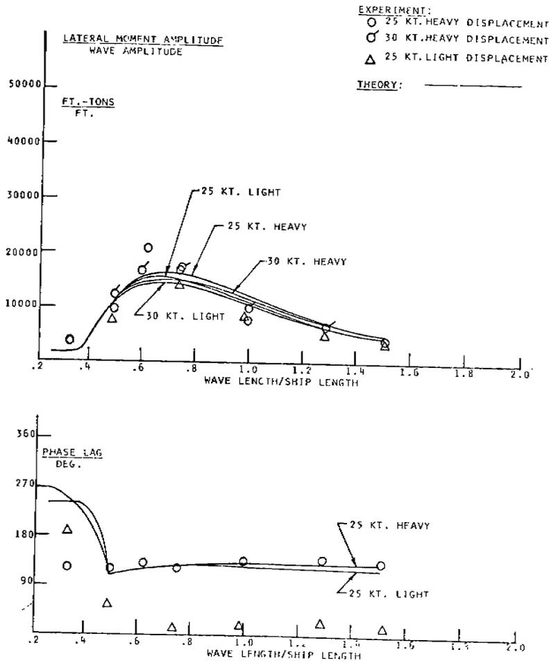
FIGURE 31 - Midship lateral wave bending moments and phase lag, 210° heading
