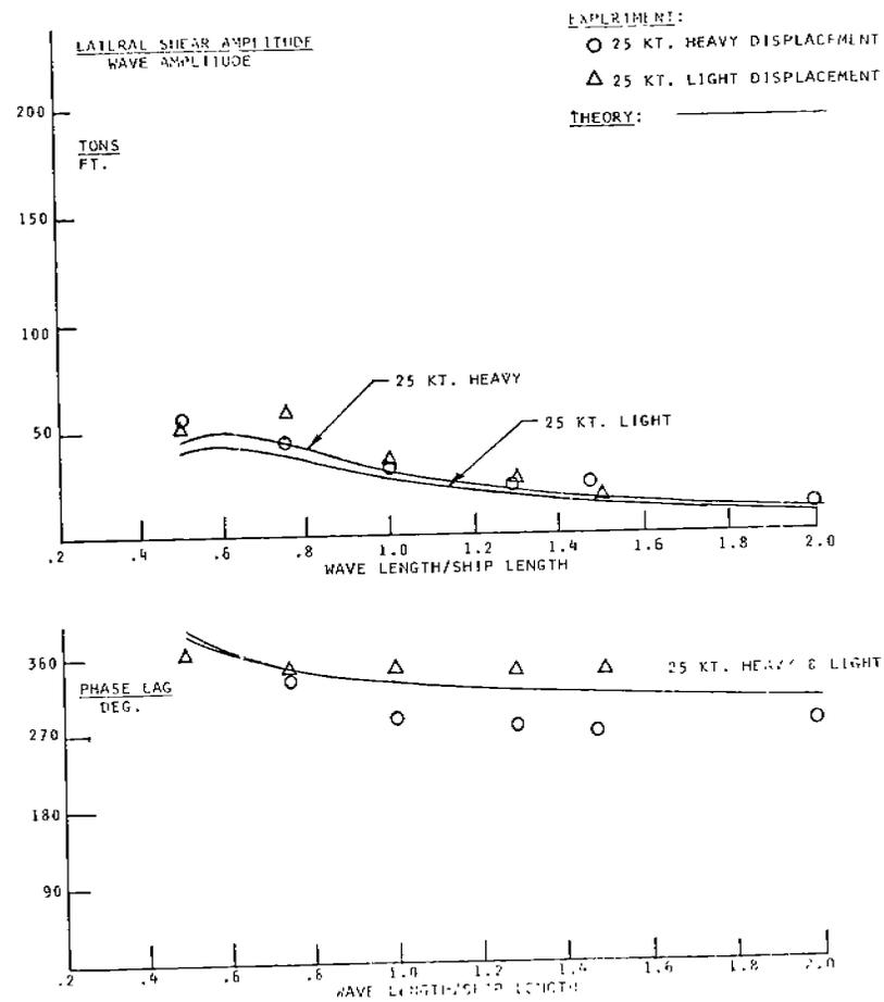
FIGURE 53 - Midship lateral shear and phase lag, 30° heading
