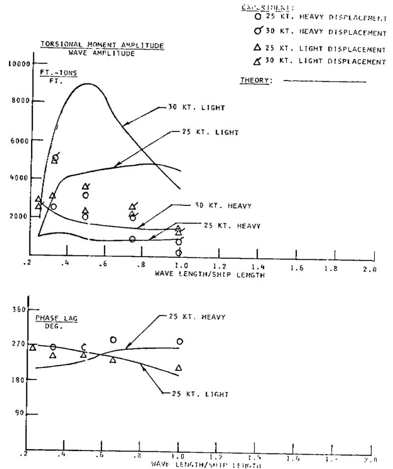
FIGURE 48 - Midship torsional wave bending moments and phase lag, 60° heading
