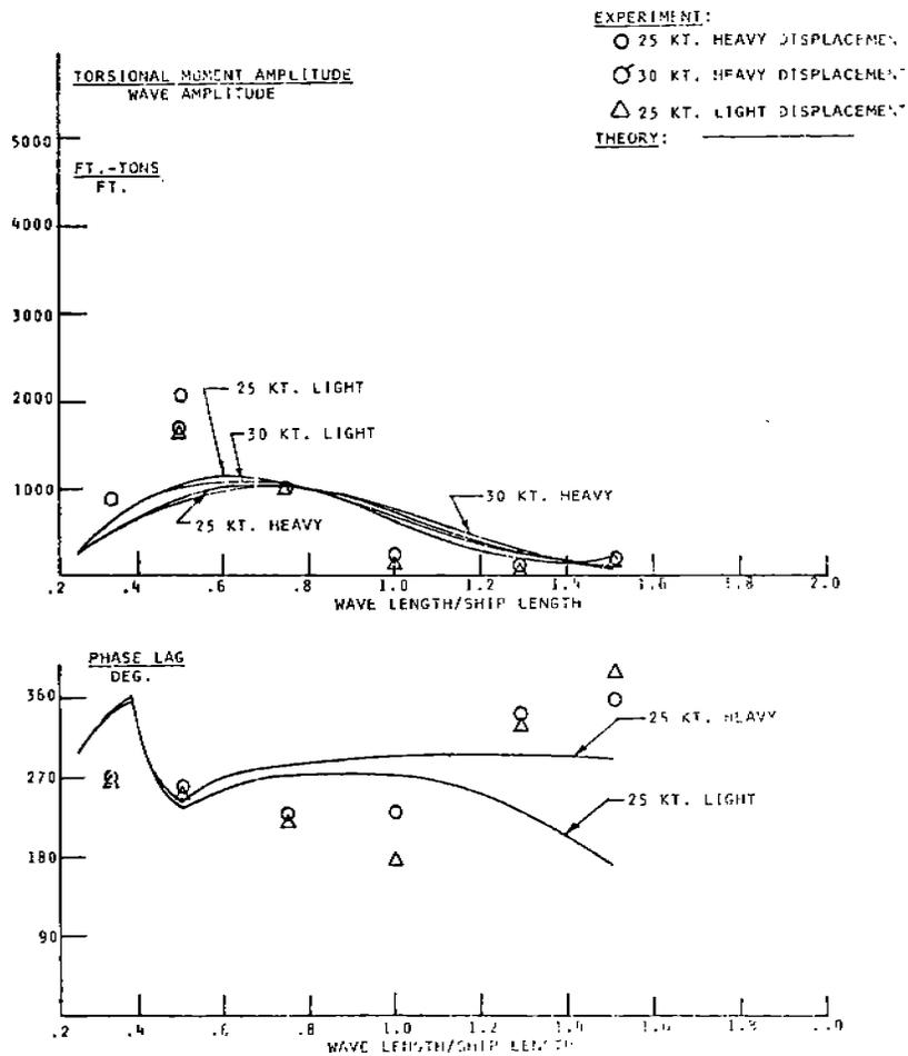
FIGURE 35 - Midship torsional wave bending moments and phase lag, 210° heading
