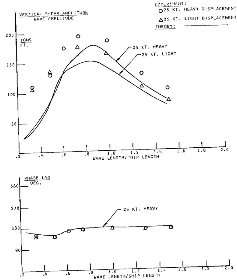
FIGURE 10 - Frame 258 vertical shear and phase lag, 210° heading
