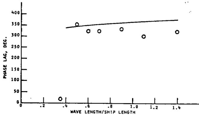
FIGURE 74 - Dutch container ship,  $F_n = .245$ , heading =  $65^\circ$
