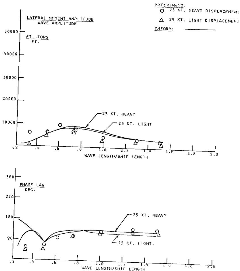
FIGURE 32 - Frame 258 lateral wave bending moments and phase lag, 210° heading
