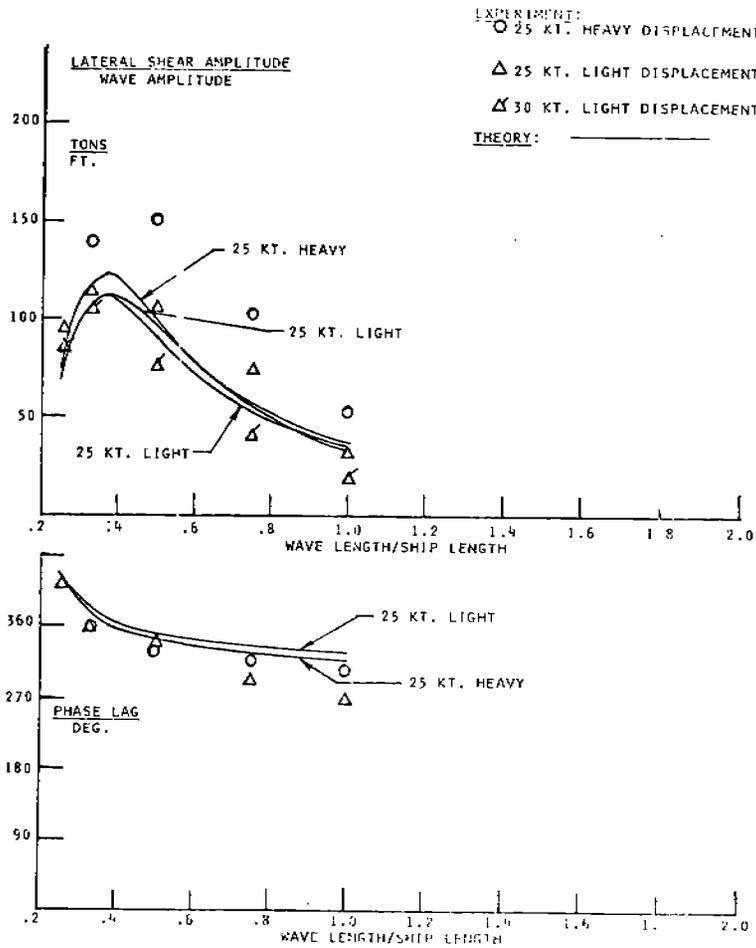
FIGURE 47 - Frame 258 lateral shear and phase lag, 60° heading
