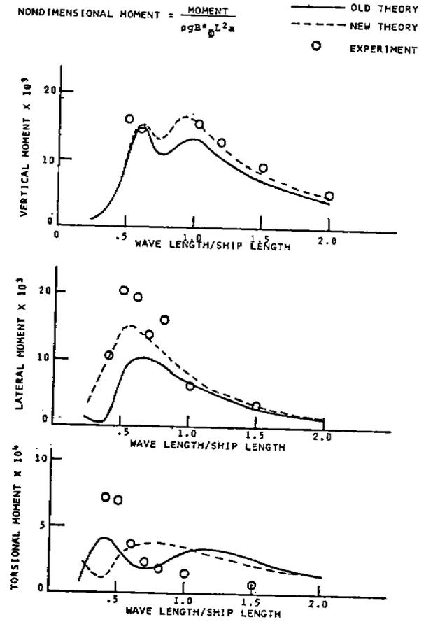
FIGURE 81 - Non-dimensional midship wave moments on Series 60, Block .80 hull,  $F_n = 0.15$ , 130° heading
