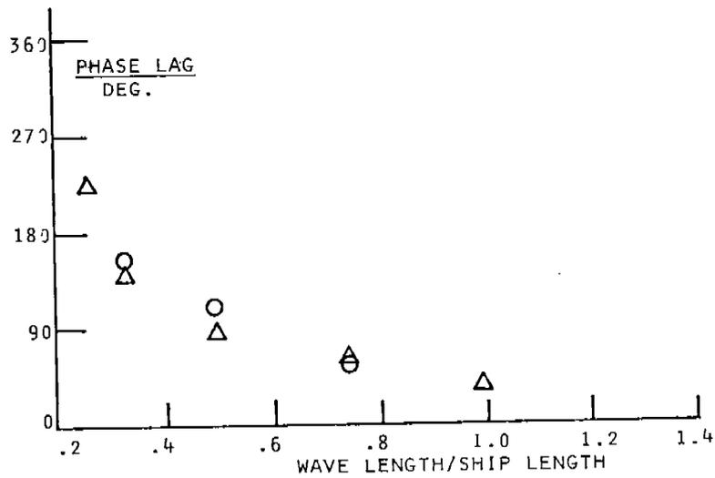
FIGURE 88 - Midship vertical wave bending moments and wave phase lag, 60° heading
