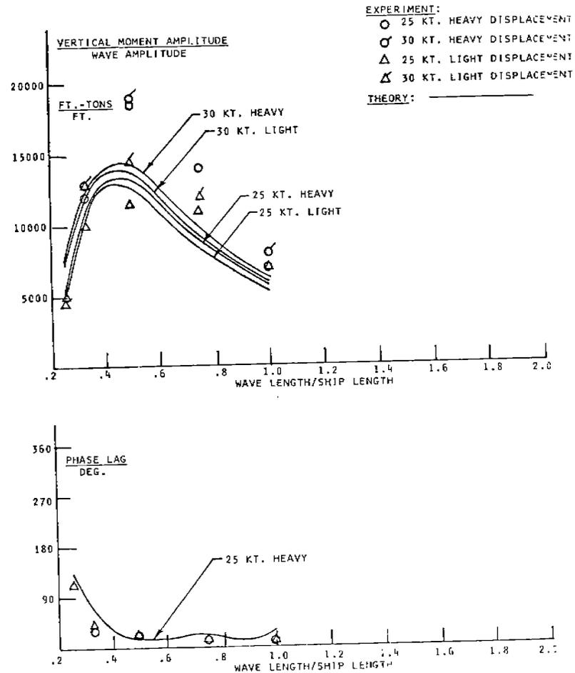
FIGURE 18 - Frame 258 vertical wave bending moments and phase lag, 60° heading
