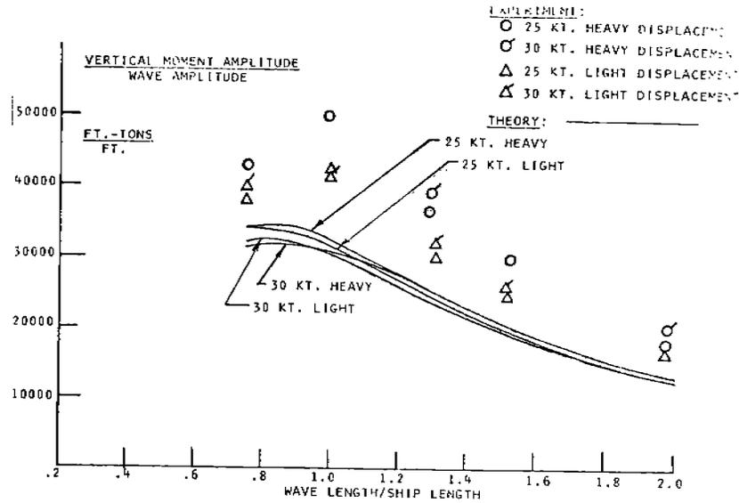
FIGURE 27 - Midship vertical wave bending moments and phase lag, 0° heading
