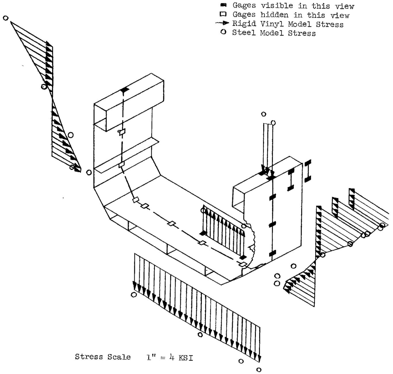
FIGURE 19 - Comparison of SL-7 Stresses at Frame 178 during Half Sagging
