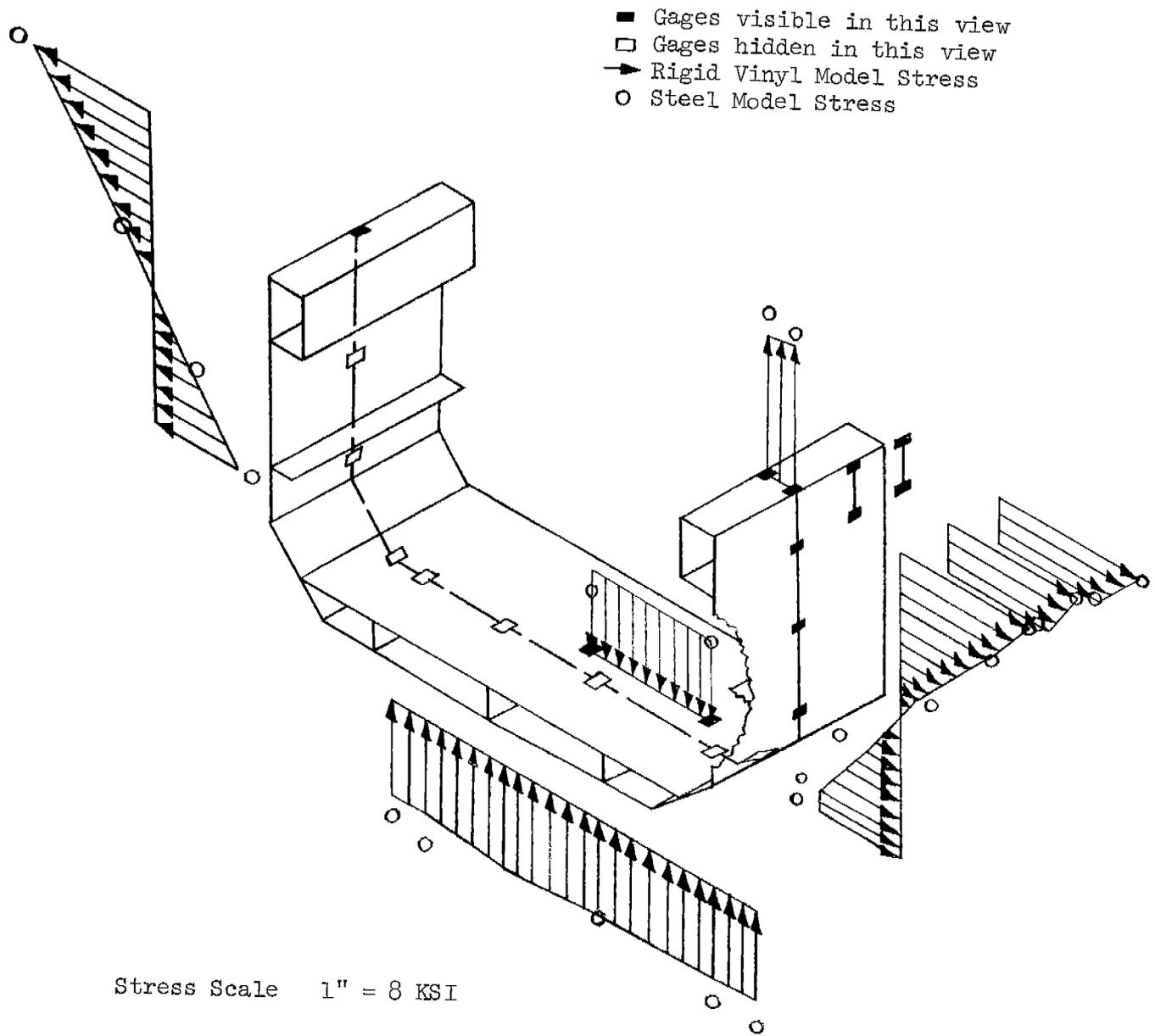
FIGURE 17 - Comparison of SL-7 Stresses at Frame 178 during Large Hogging
