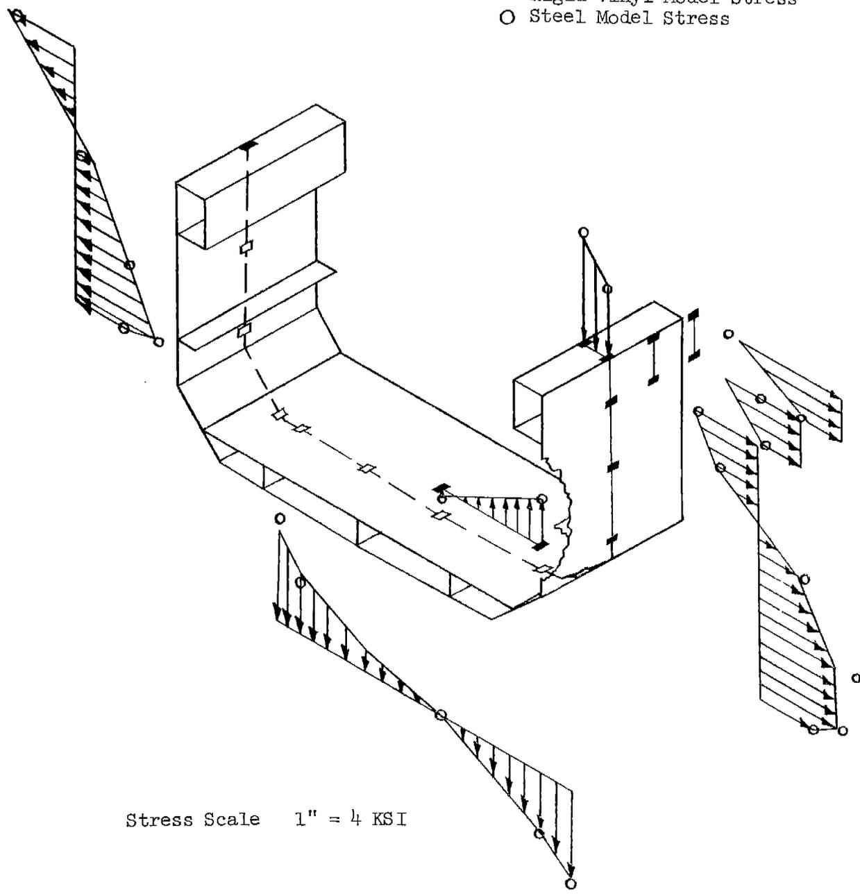
FIGURE 23 - Comparison of SL-7 Stresses at Frame 178 during Positive Torsion
