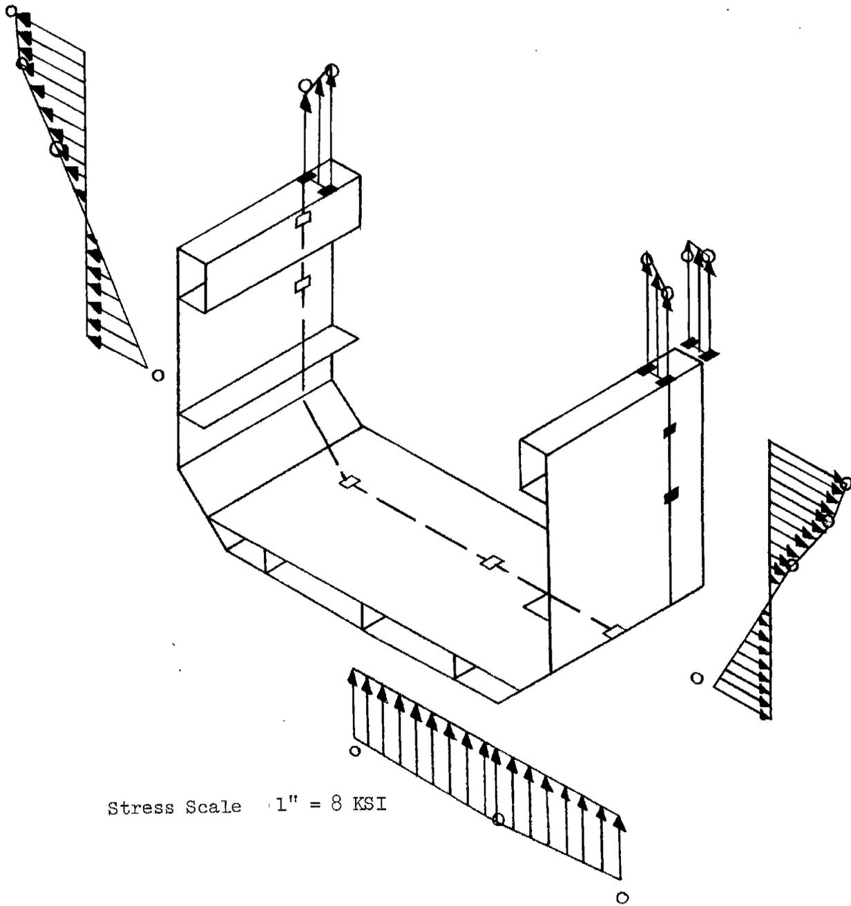
FIGURE 18 - Comparison of SL-7 Stresses at Frame 142 during Large Hogging
