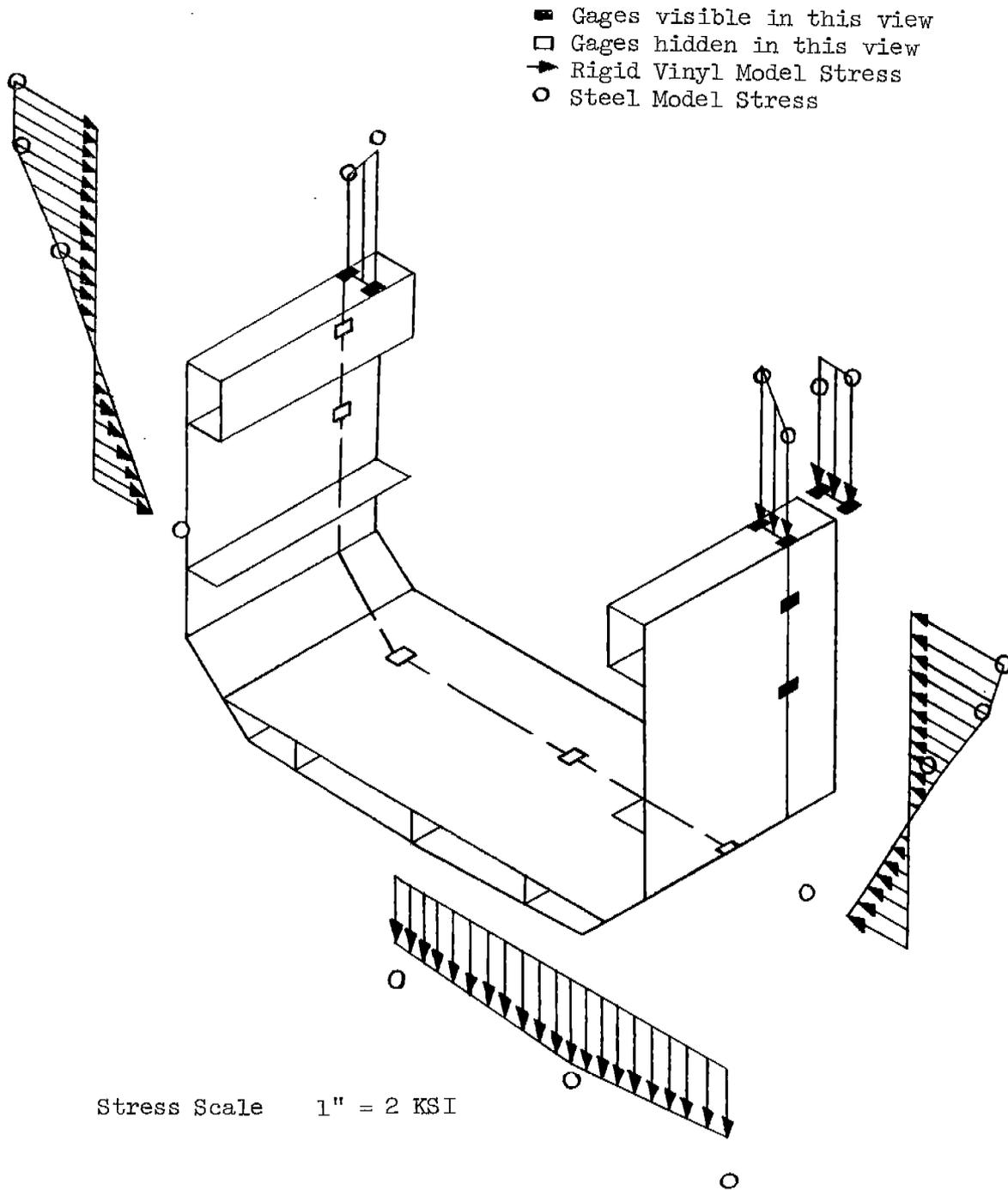
FIGURE 21 - Comparison of SL-7 Stresses at Frame 142 during Midship Shear
