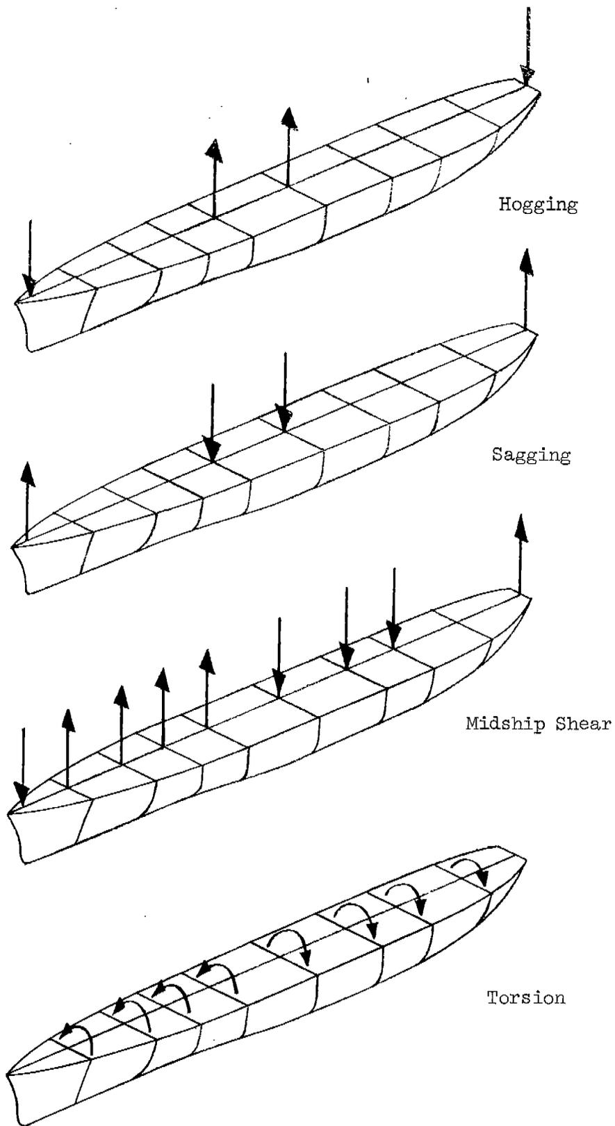
FIGURE 14 - Static Loads Applied to the SL-7
