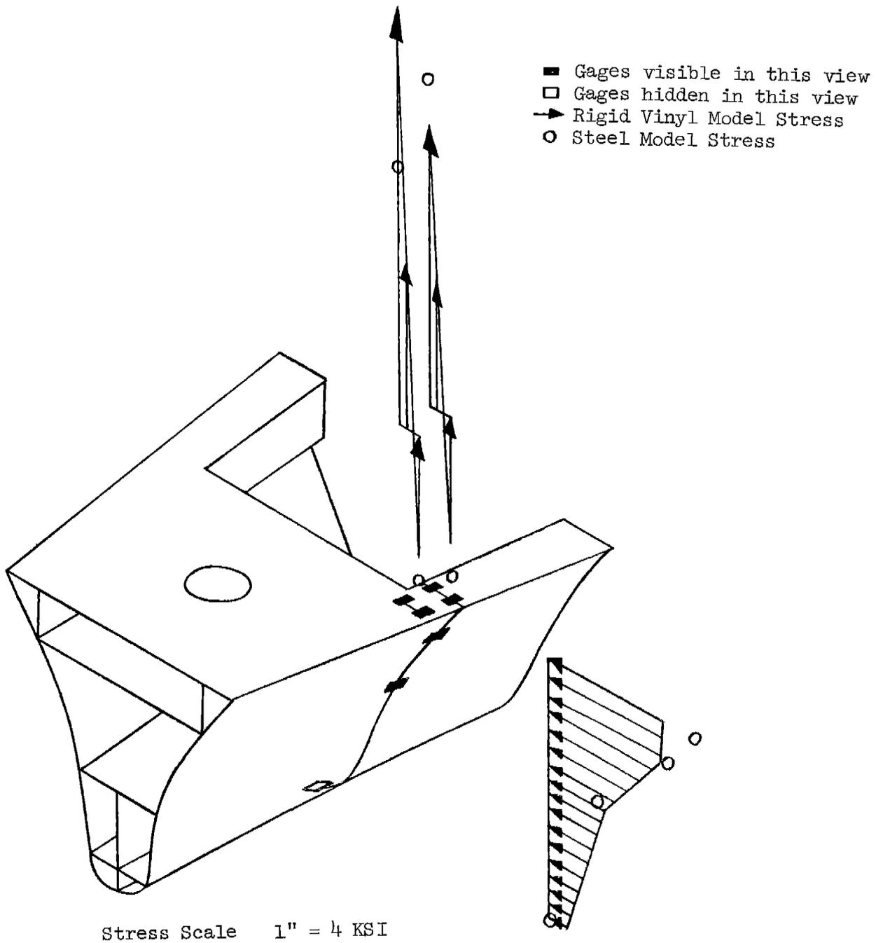
FIGURE 22 - Comparison of SL-7 Stresses at Frame 290 during Positive Torsion
