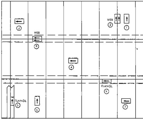
Fig. A-3 - Specimen 6, Strain Gage Locations
