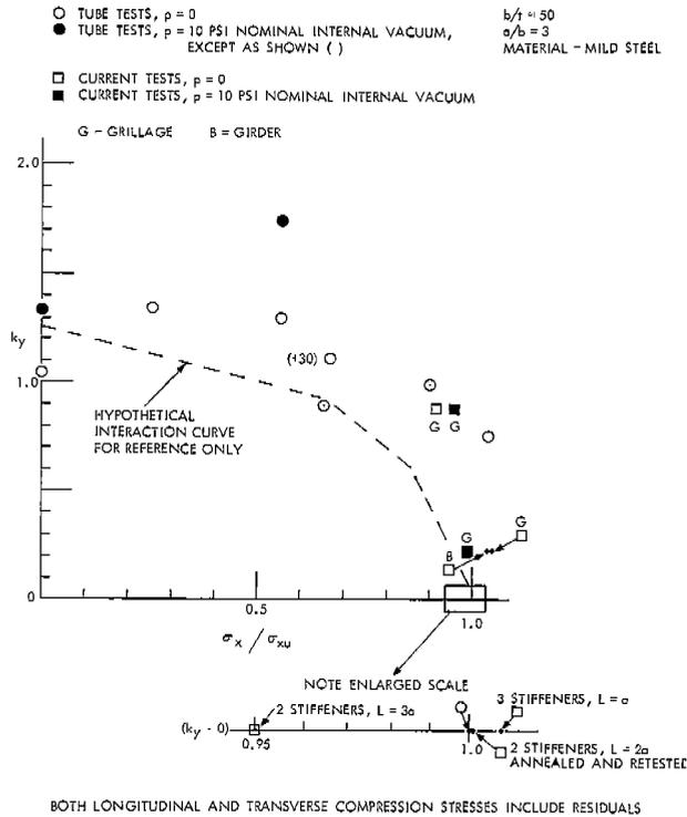
Fig. 8 - Comparison of Unstiffened and Stiffened Plate Data
