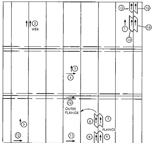
Fig. A-2 - Specimen 5, Strain Gage Locations
