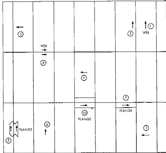
Fig. A-4 - Specimen 7, Strain Gage Locations
