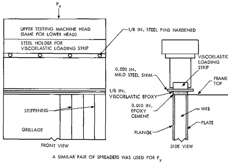
Fig. 4 - Load Spreaders for Grillage Tests
