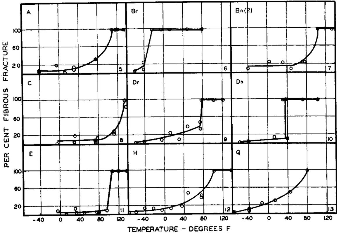
FIGURES 5-13 - FIBROUS FRACTURE VS TEMPERATURE
