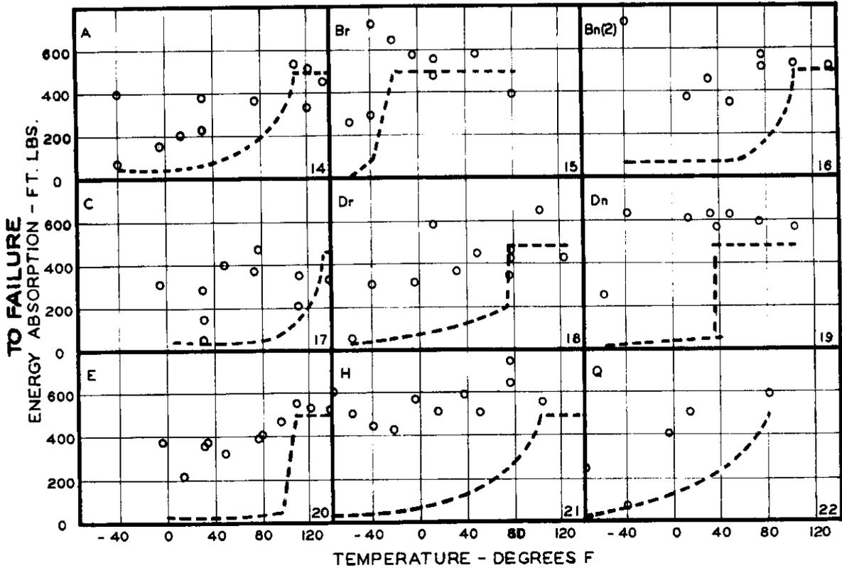
FIGURES 14-22 - ENERGY ABSORPTION VS TEMPERATURE
