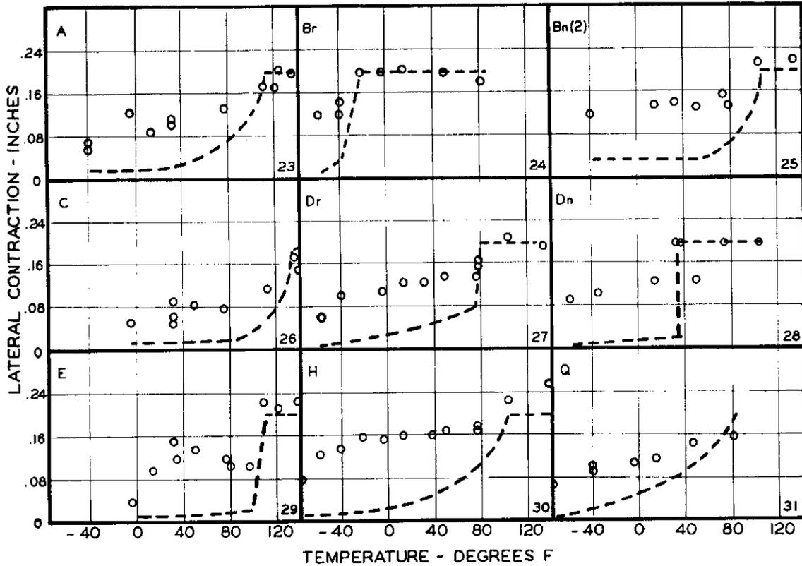
FIGURES 23-31 - LATERAL CONTRACTION VS TEMPERATURE
