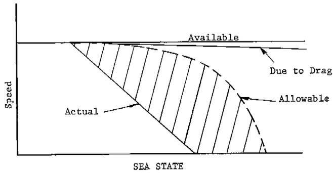
Fig. VII-3. Speed vs Sea State
