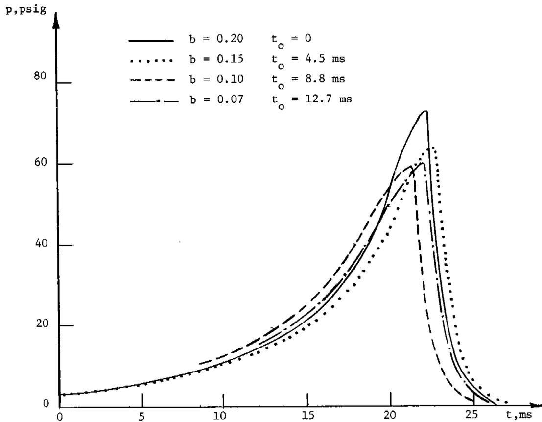
Fig. III-3. Pressure Versus Time at the Centerline of the Model<sup>9</sup>
