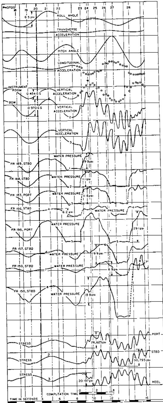
Fig. II-1. Experimental Data Acquired From Seakeeping Trials of Three Dutch Destroyers<sup>1</sup>
