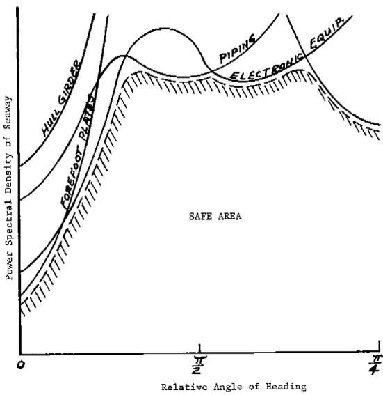
Fig. VII-5. Failure Envelope at Constant Speed
