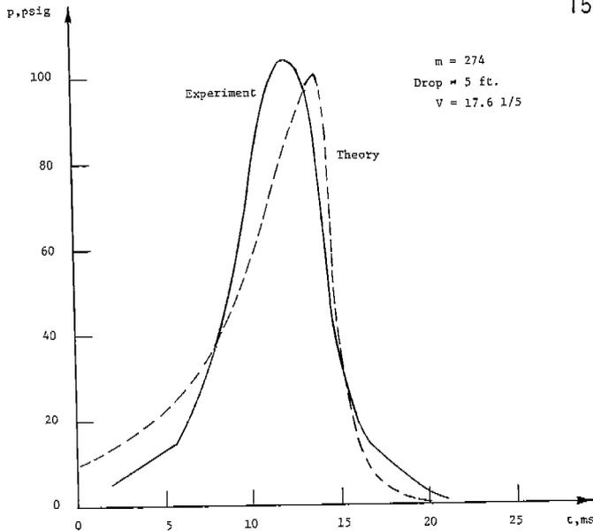
Fig. IV-3. Pressure-Time Curves by Two-Dimensional Theory<sup>9</sup>
