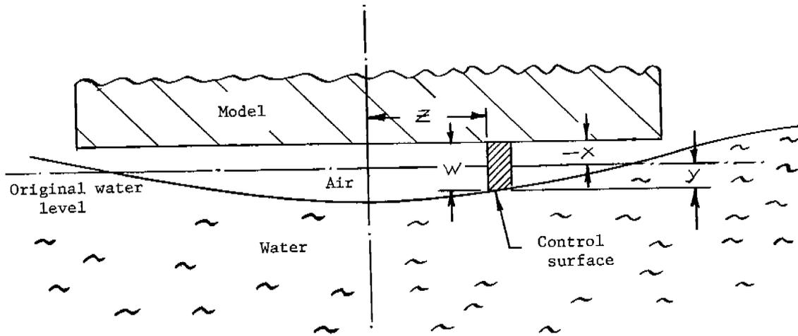
Fig. III-2. Impact Model and Control Surface<sup>9</sup>
