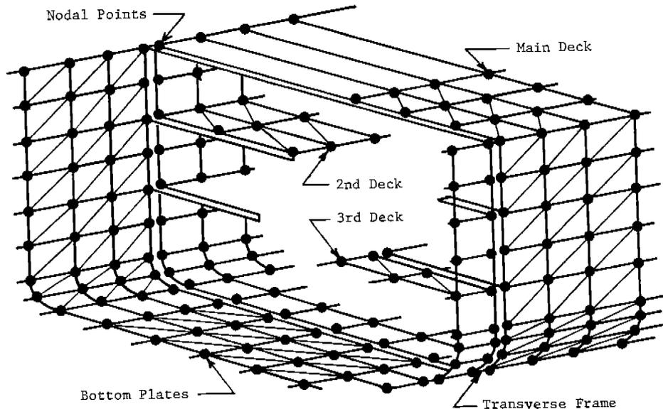
Fig. VII-1. Finite Element Break Down of Typical Ship Segment
