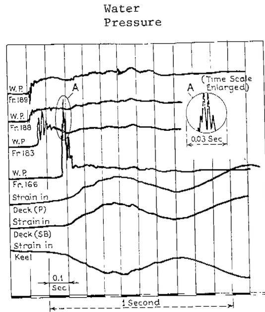
Fig. II-2. Sample of High Speed Slam<sup>2</sup>
