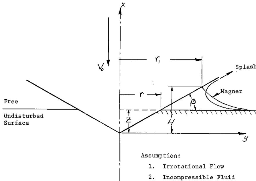
Fig. III-1. Wedge Entry Into Fluid Medium
