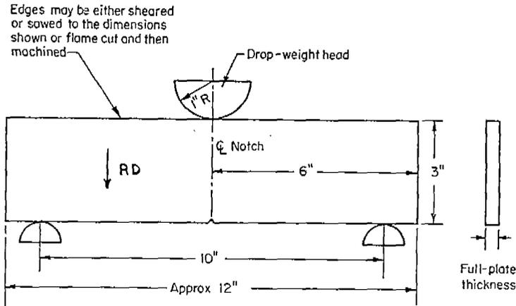
Fig. 7. Drop-Weight Tear-Test Specimen Employed at Battelle Memorial Institute<sup>4</sup>
