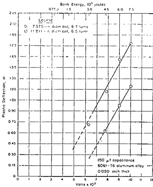
C. —Plastic deflection at the center of free-formed aluminum sheets for various energy levels discharged through coils of different diameters (ref. 5).
