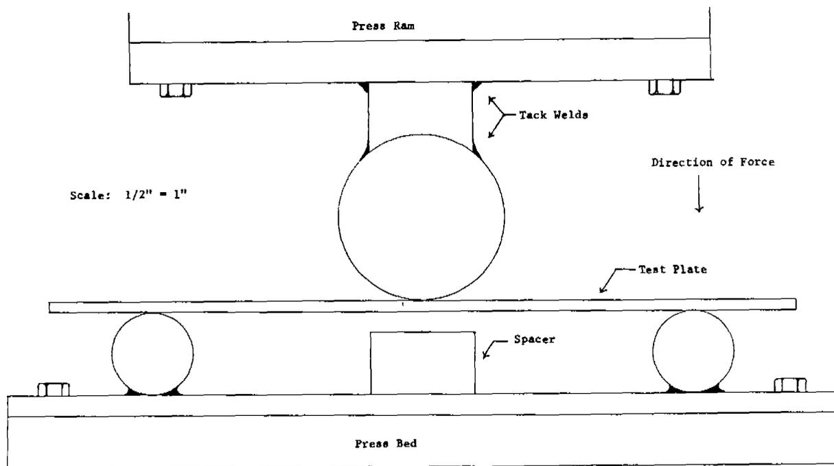
Fig. 3. Jigging for Mechanical Bending
