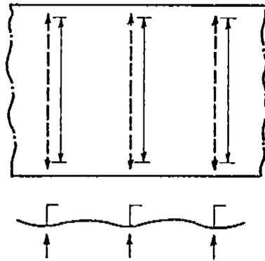
c. Line Heating Back of Welds
