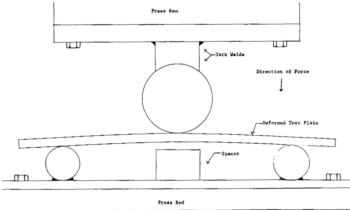
Fig. 6. Jigging for Mechanical Straightening
