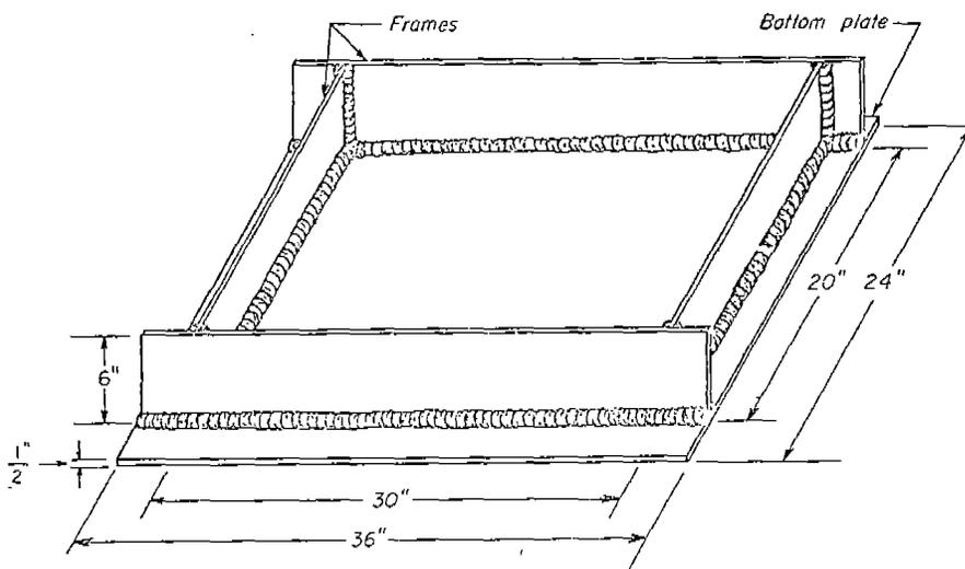
Fig. 8. Structural Weldment
