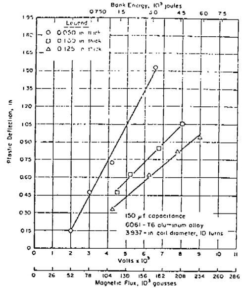
B. —Effect of discharge energy on the plastic deformation produced by electromagnetic hammers on free-formed aluminum sheets of three different thicknesses (ref. 5).
