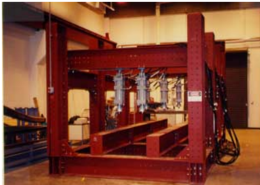
Figure 2. Structural Test System.
