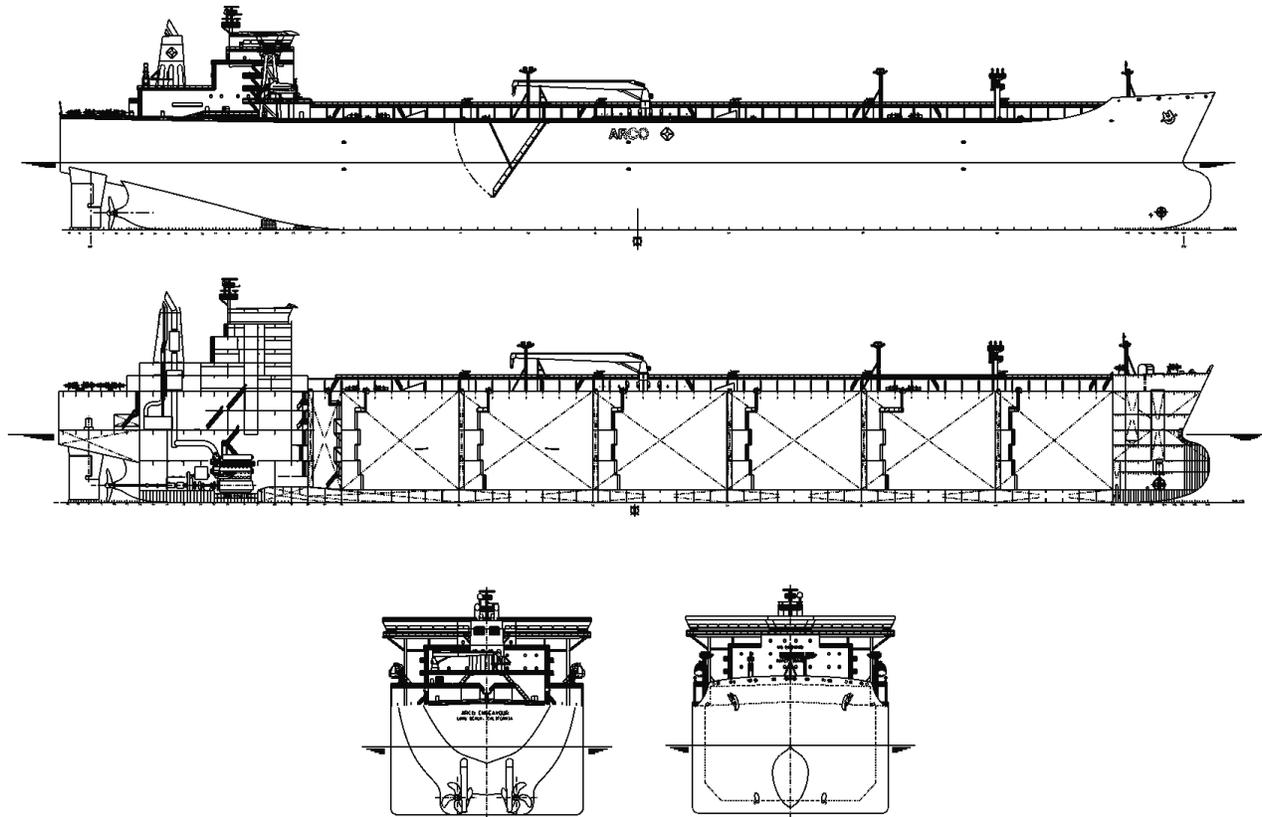
**Fig. 1** Inboard Profile, Outboard Profile, Bow and Stern Views
