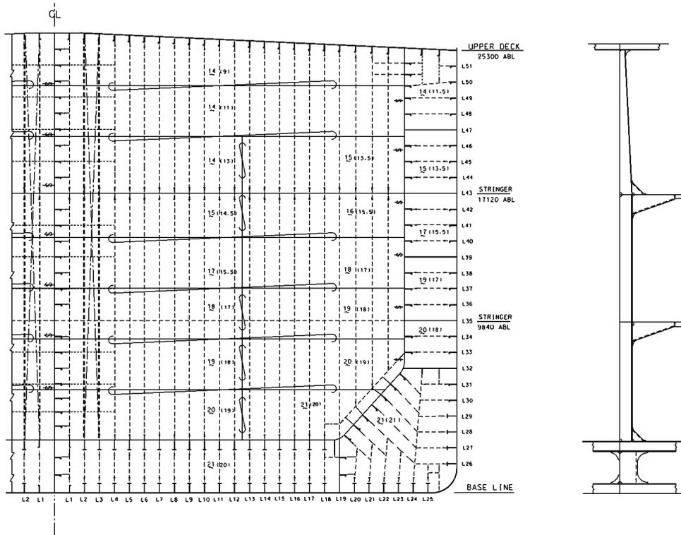
**Fig. 6** Transverse Bulkhead Arrangement Showing Scantlings (l), Typical Bulkhead Stiffener (r)
