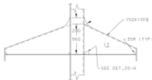
**Fig. D1** “Soft Heel” Tripping Brackets on Centerline Vertical Web Frames
