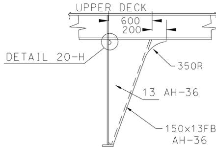
**Fig. D3** Tripping Bracket on Upper Deck Web Frame
