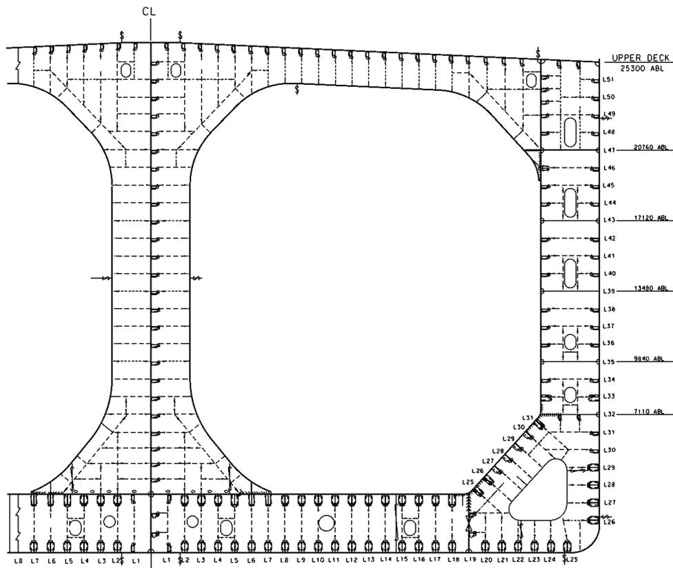
**Fig. 3** Typical Midship Section
