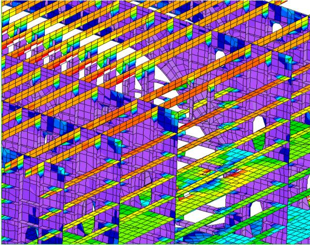
**Fig. 9** Upper Shear Strake (Plating and Bulkhead Removed)
