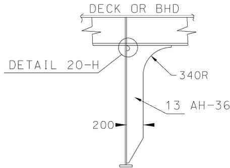
**Fig. D2** “Soft Heel” Web Stiffener on Upper Deck Transverse Web Frames or Centerline Vertical Web Frames
