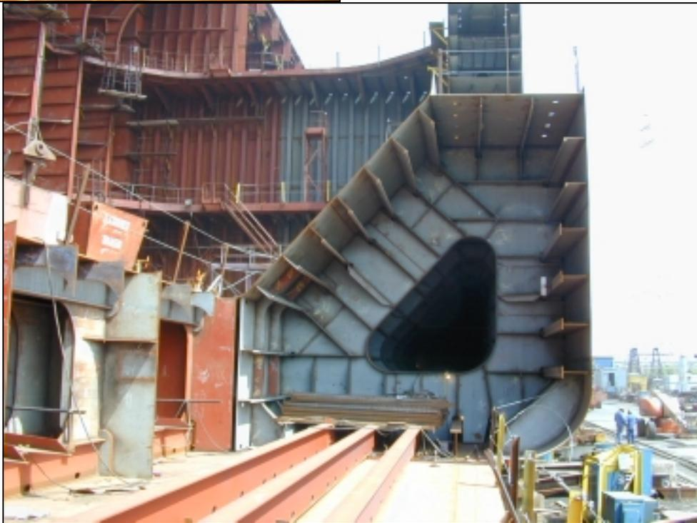
**Fig. A5** View of Hopper After Erection, Looking Aft
