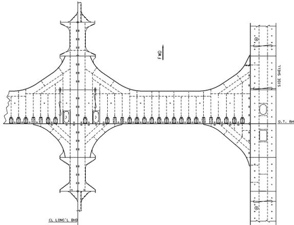
**Fig. 4** Transverse Bulkhead Stringer at Midship
