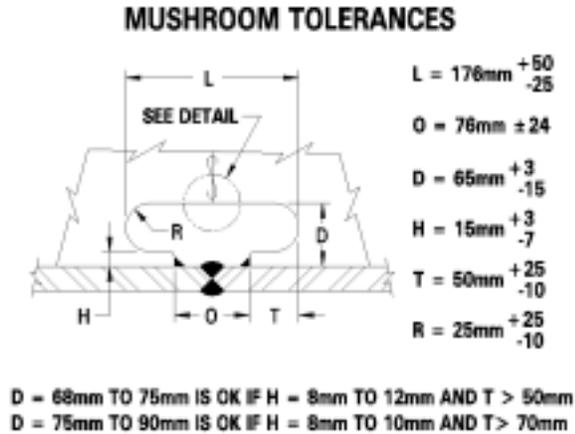
**Fig. 17** Construction Tolerance for “Mushroom” Cutouts
