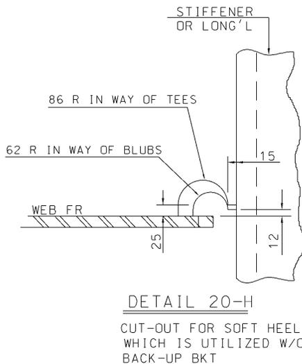
**Fig. D4** Detail of “Soft Heel” Cutouts for Bulb Plate and Tee Stiffeners
