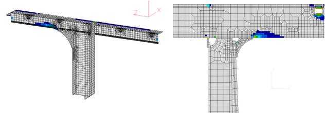
**Fig. 15** Initial and Final Bulkhead Stiffener to Deck Longitudinal Connection
