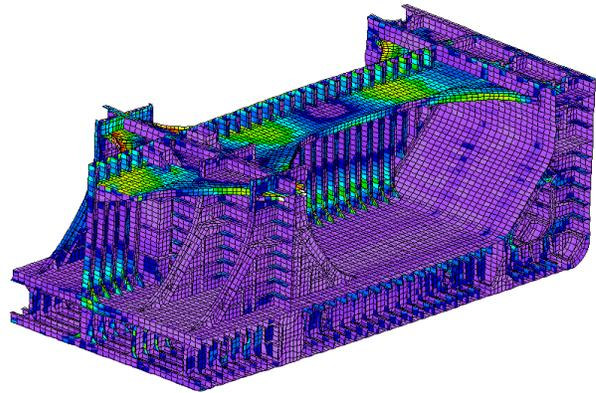
**Fig. 8** General Local Model at Transverse Bulkhead
