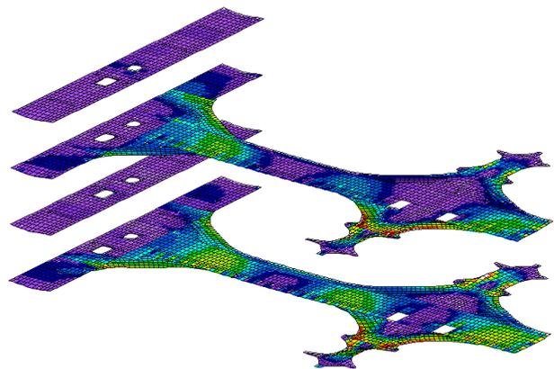
**Fig. 11** Horizontal Stringers, Checkerboard Loading, Bulkheads Removed
