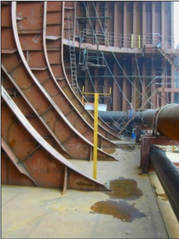
**Fig. A1** View Looking Aft Along Transverse Web Frames in Cargo Tank
