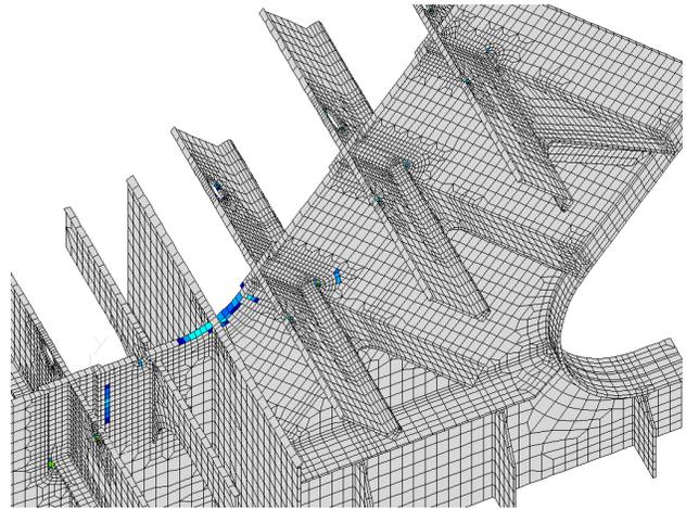
**Fig. 13** Lower Hopper, Tanktop Plating Removed
