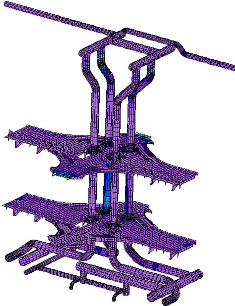
**Fig. 16** Cargo Riser and Drop Pipe Model (Upper Deck Removed)
