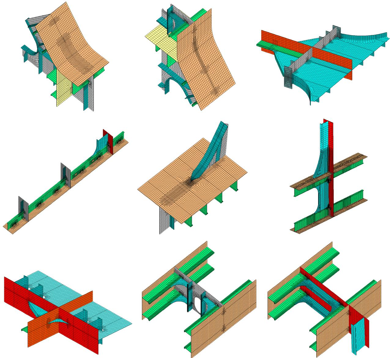
**Fig. 5** Nine Local Details in Preliminary Analysis (Top row, 1 to r: Lower Hopper, Upper Hopper, Stringer at Centerline Bulkhead; Middle Row, 1 to r: Bottom Longitudinal, Transverse Web Frame at Tank Top, Double Bottom at Transverse Bulkhead; Bottom Row, 1 to r: Horizontal Stringer at Transverse Bulkhead, Inner and Outer Shell at Transverse Bulkhead, Inner and Outer Shell at Web Frame)
