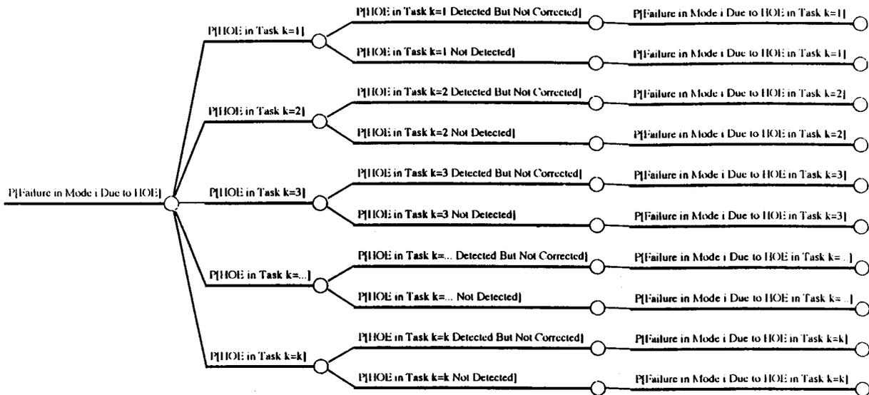
The likelihood of failure in a given mode  $i$  due to human and organizational error is the sum over all tasks ( $k$ ) of the likelihood's of undetected or uncorrected HOE in a given task  $k$  times the likelihood of failure in mode  $i$  given HOE in task  $k$ .
