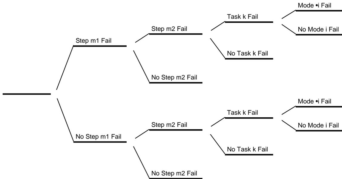
Failure analysis tree for a given step m1 which has a redundant step (m2), but which has no error detection or correction possibilities.
