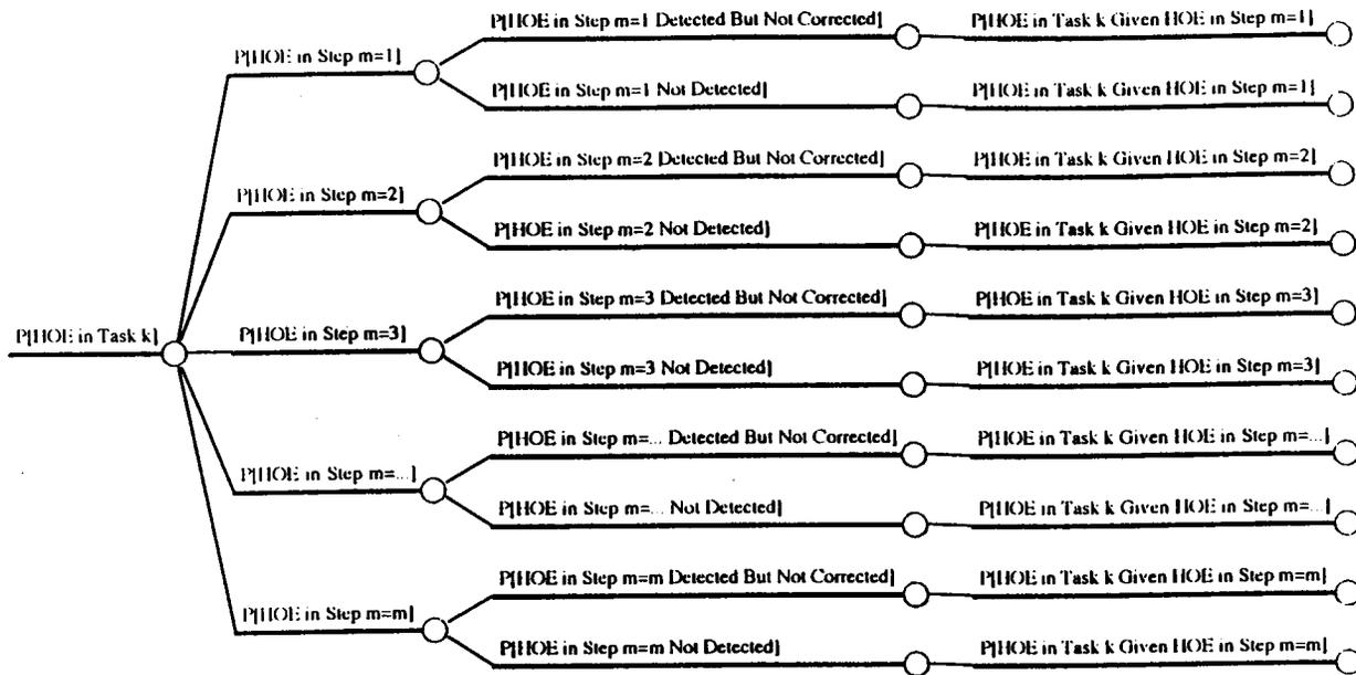
The likelihood of HOE in a given task (k) of failure mode (m) is obtained by taking the product of the likelihood of an undetected or uncorrected error in a given step (m) times the likelihood of HOE in task (k) given HOE in step i.
