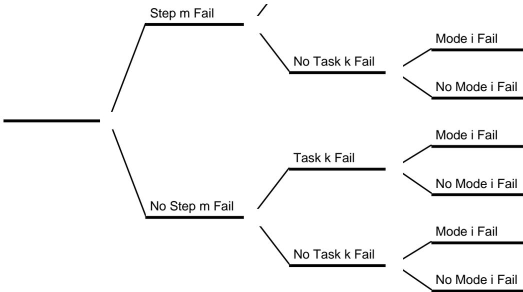
Failure analysis tree for a given step m which has no redundant steps, error detection or correction possibilities.
