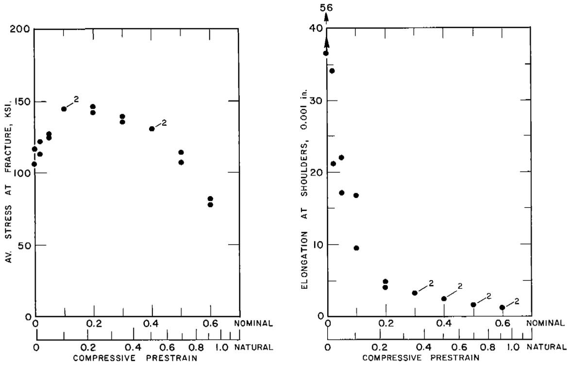
Fig. 13. Tension Tests of Notched ABS-B Steel Bars at  $-16^{\circ}\text{F}$  Notch Radius  $\rho = 0.030$  in.
