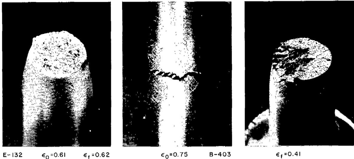
Fig. 4. Ductile Fractures of Highly Prestrained Bars.
