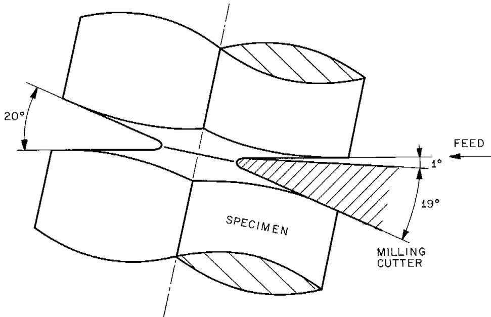
Fig. 7. Detail of Notch During Machining
