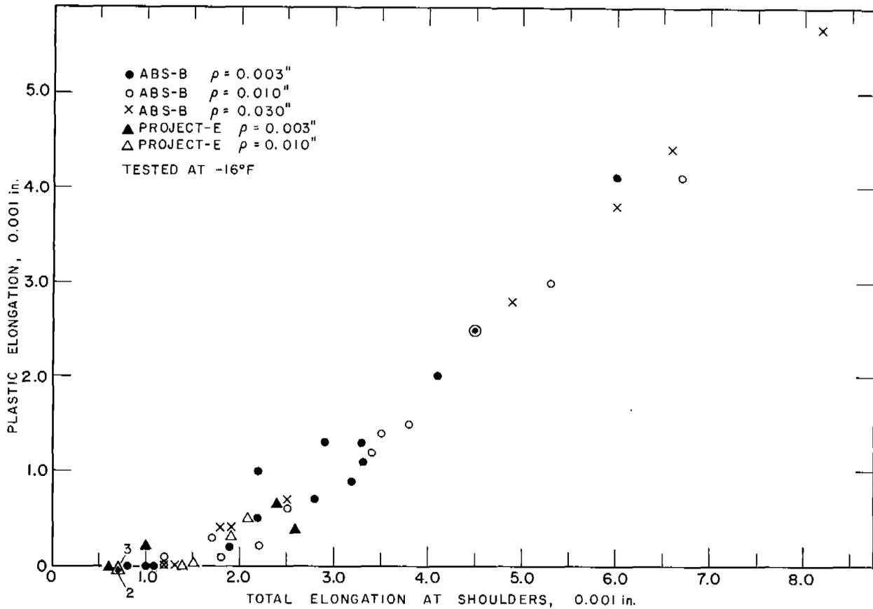
Fig. 10. Plastic vs Total Elongation at the Shoulders of All Notched Bars at  $-16^{\circ}\text{F}$
