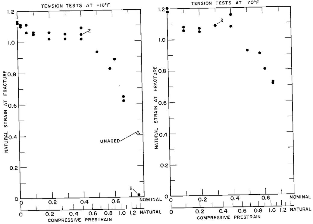
Fig. 2. Bars of ABS-B Steel Compressed at 70°F and Aged.
