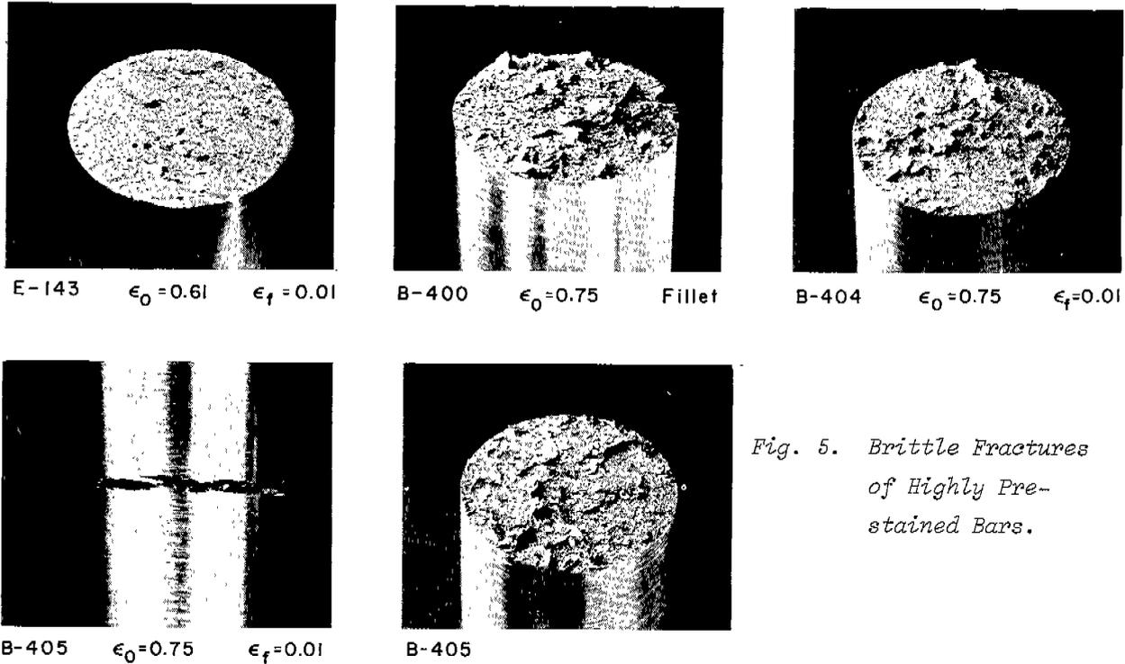
Fig. 5. Brittle Fractures of Highly Pre-stained Bars.
