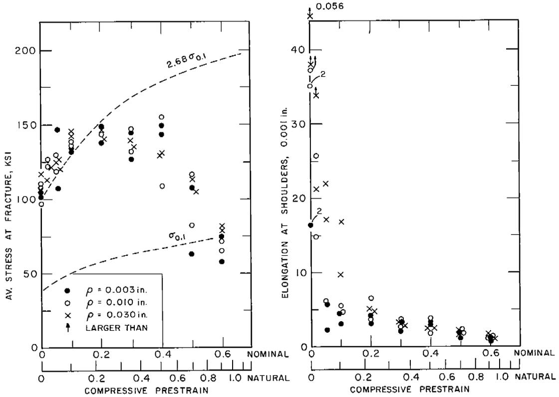
Fig. 14. Collected Results of Notched Bar Tests of ABS-B Steel Aged and Tested at  $-16^{\circ}\text{F}$
