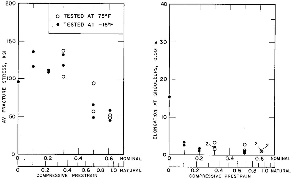
Fig. 15. Tension Tests of Notched E-Steel Bars at 75° and -16° F Notch Radius  $\rho = 0.003$  in.
