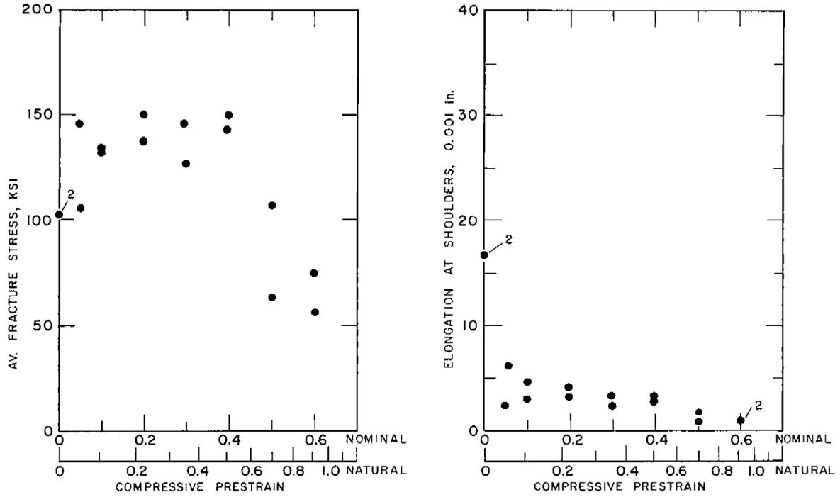
Fig. 11. Tension Tests of Notched ABS-B Steel Bars at  $-16^{\circ}\text{F}$  Notch Radius  $\rho = 0.003$  in.
