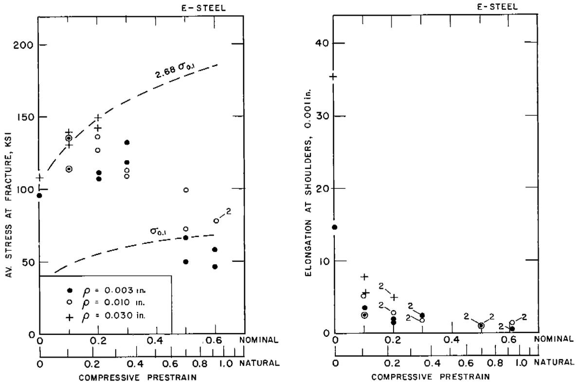
Fig. 17. Collected Results of Notched Bar Tests of Project E-Steel Aged and Tested at -16° F
