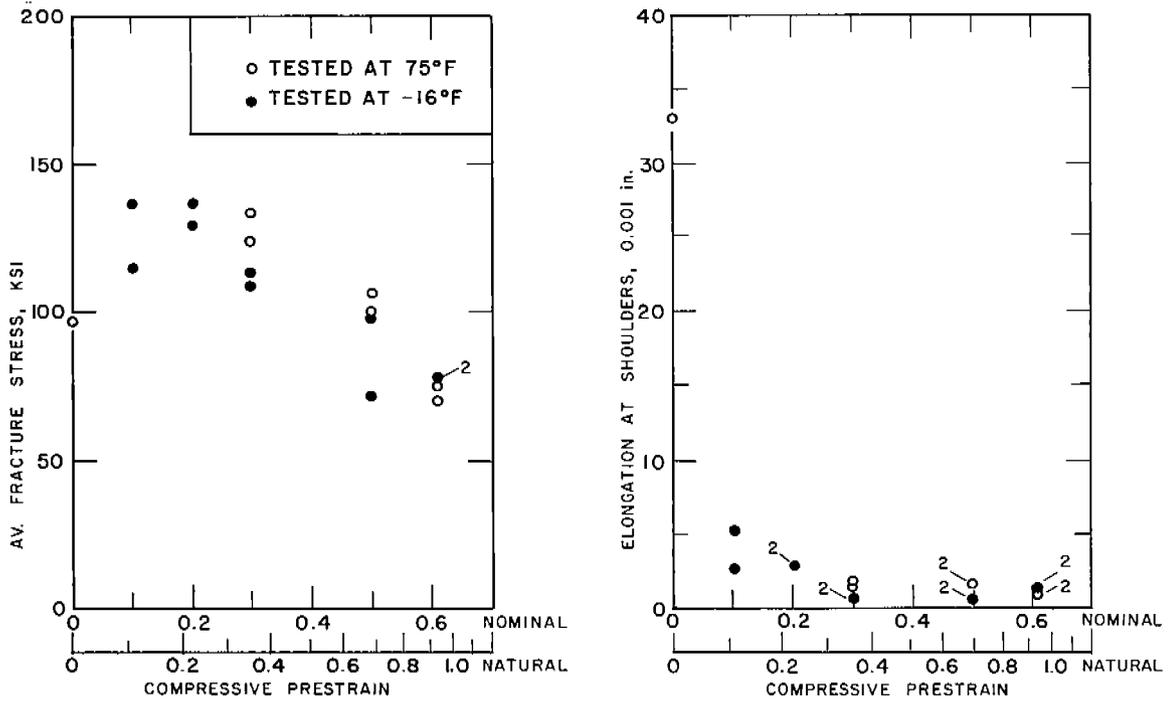
Fig. 16. Tension Tests of Notched E-Steel Bars at 75° and -16° F Notch Radius  $\rho = 0.010$  in.
