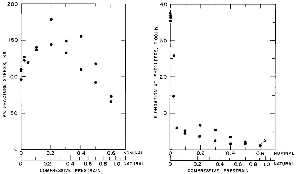
Fig. 12. Tension Tests of Notched ABS-B Steel Bars at  $-16^{\circ}\text{F}$  Notch Radius  $\rho = 0.010$  in.
