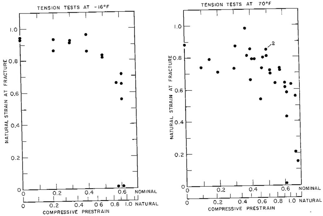
Fig. 3. Bars of Project E-Steel Compressed at 70°F and Aged.
