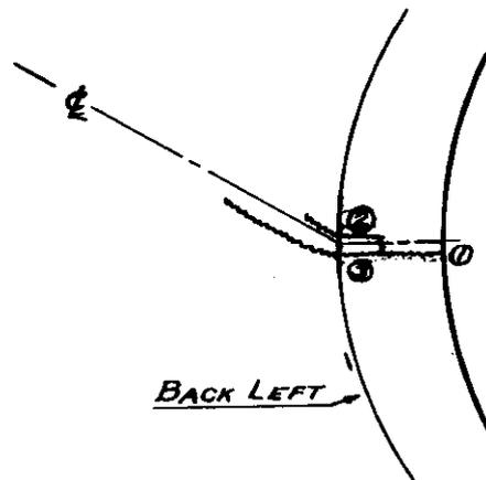
①, ②, ③ DENOTES ORDER IN WHICH CRACKS DEVELOPED ON INSIDE SURFACE OF HOLE - CRACK SPREAD ALONG ① - JUMPED TO ②. ORIGINAL CRACK THEN PROPAGATED ALONG ③ AND FINALLY ② BECAME ARRESTED.
