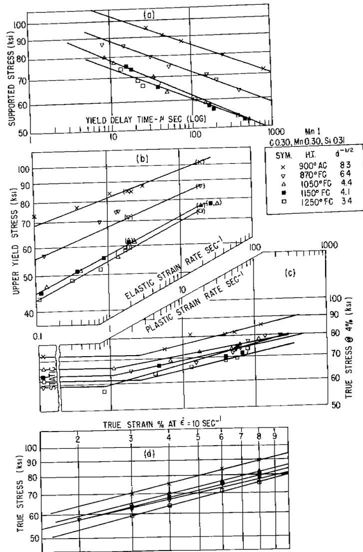
Fig. 9. Summary of dynamic yield and flow data for high carbon, low manganese steel, Mn-1.
