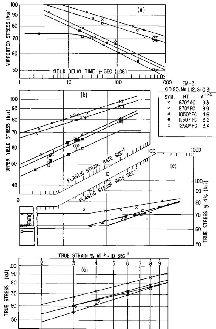
Fig. 8. Summary of dynamic yield and flow data for medium carbon, high manganese steel, EM-3.
