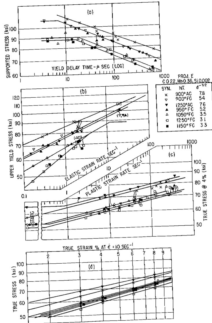
Fig. 6. Summary of dynamic yield and flow data for medium carbon, low manganese steel, Proj. E.
