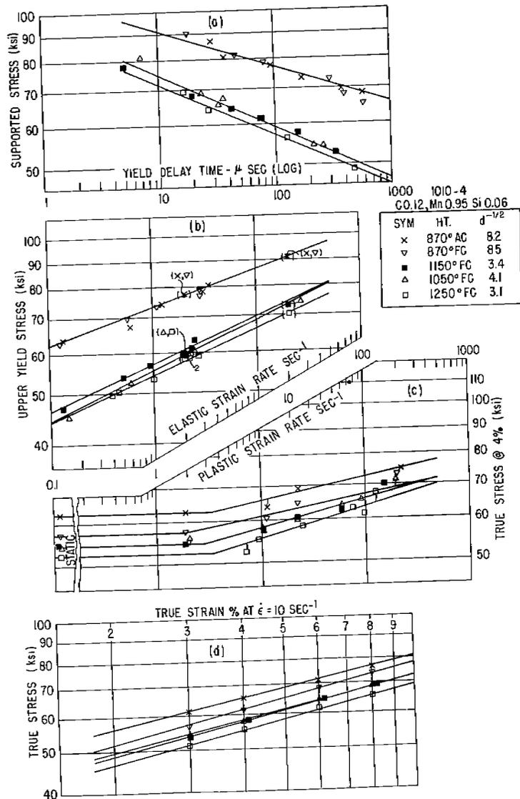
Fig. 5. Summary of dynamic yield and flow data for low carbon, high manganese steel, 1010-4.
