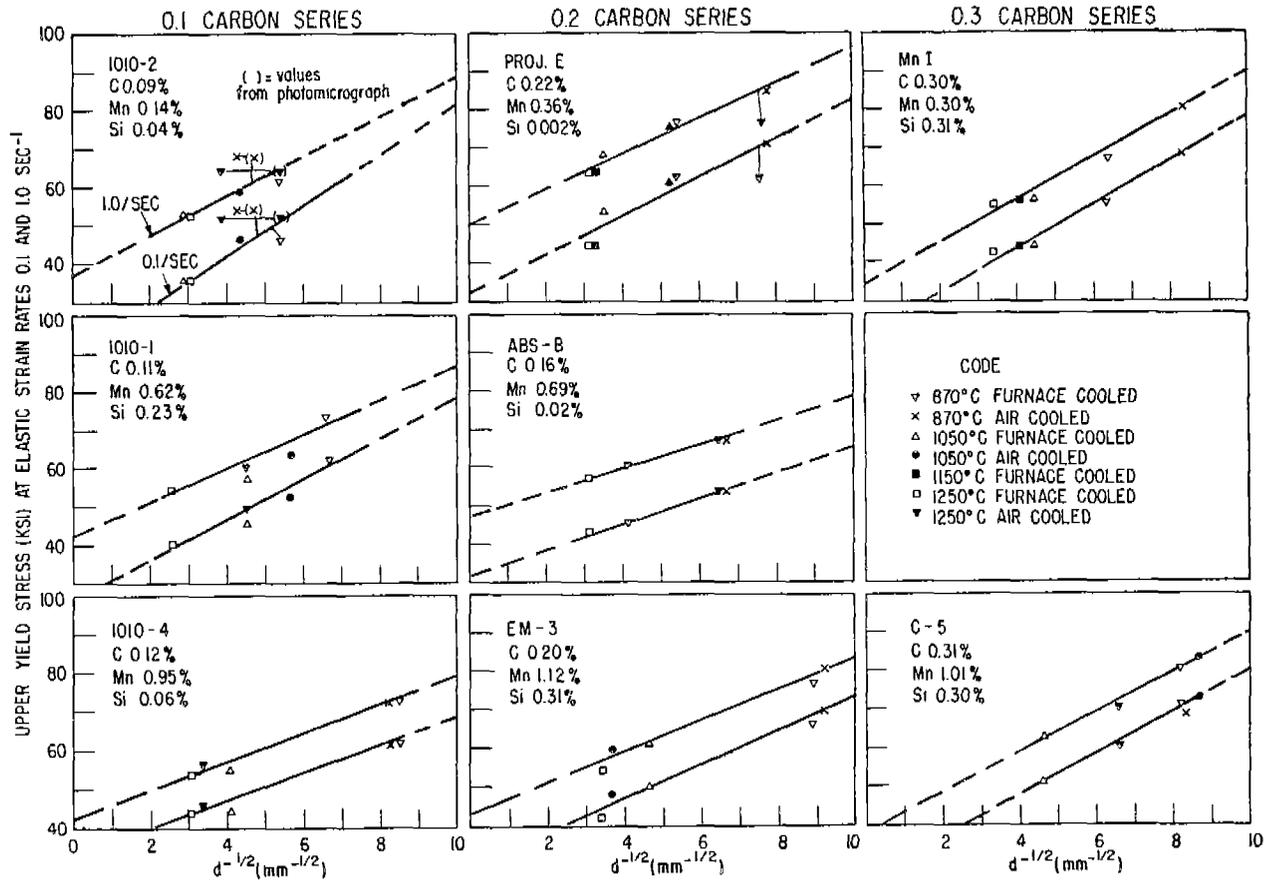
Fig. 11 - Upper yield stress at selected elastic (loading) strain rates of 0.1 and 1.0 per sec against ferrite grain size parameter,  $d^{-1/2}$ .
