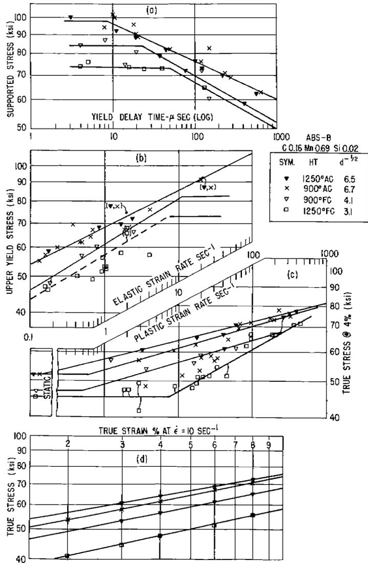
Fig. 7. Summary of dynamic yield and flow data for medium carbon, medium manganese steel, ABS-B.
