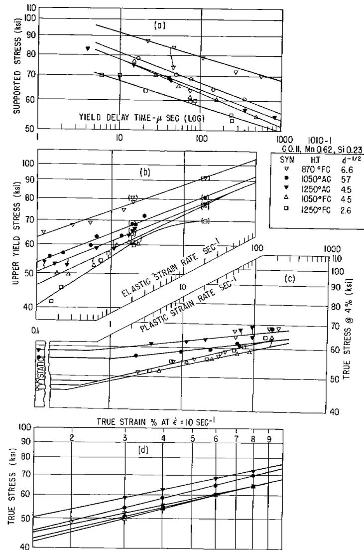
Fig. 3. Summary of dynamic yield and flow data for low carbon, low manganese steel, 1010-2.
