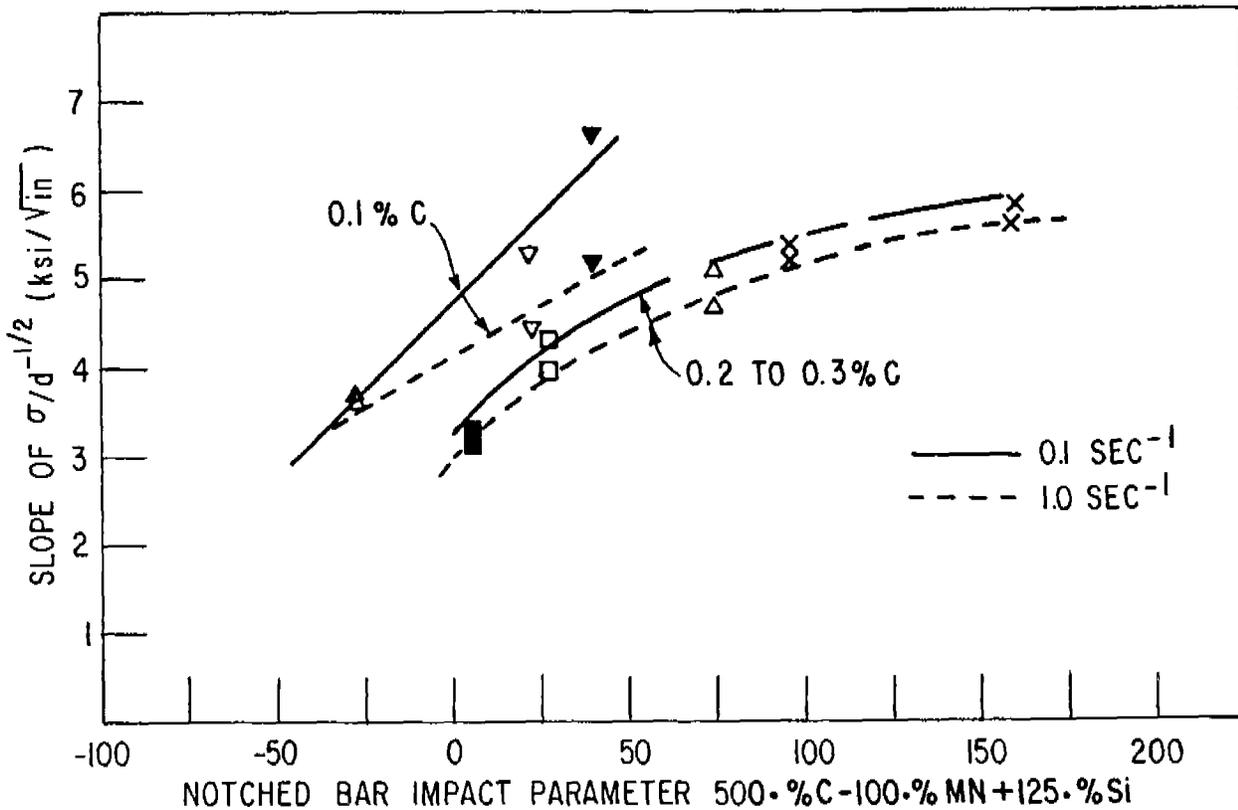
Fig. 13 - Comparison of sensitivity of yield stress to grain size to a notched bar transition temperature parameter based on effects of composition.
