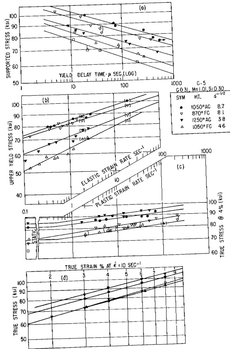
Fig. 10. Summary of dynamic yield and flow data for high carbon, high manganese steel, C-5.
