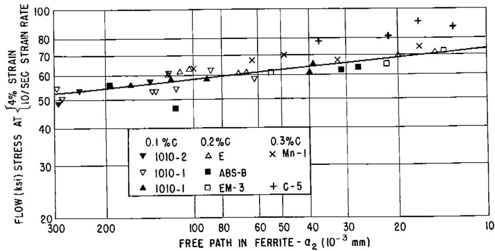
Fig. 12 - Flow stress at selected strain (4%) and strain rate (10/sec) as a function of free ferrite path parameter  $\alpha_2$ .
