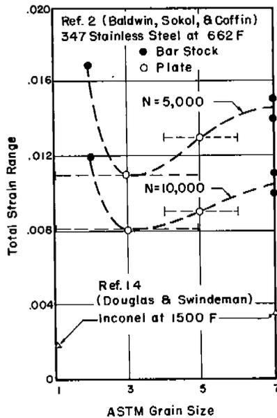
FIG. 7 EFFECT OF GRAIN SIZE
