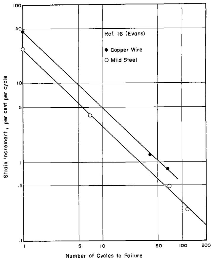
FIG. 3 CONSTANT STRAIN-INCREMENT TEST DATA
