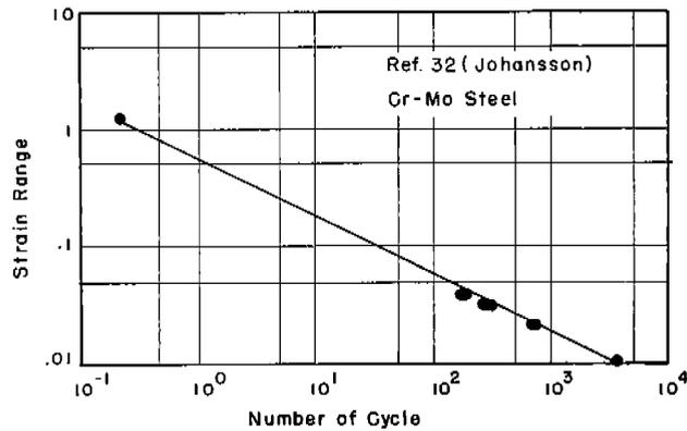
FIG. 4 STRAIN RANGE VS. LIFE ON LOG-LOG PLOT
