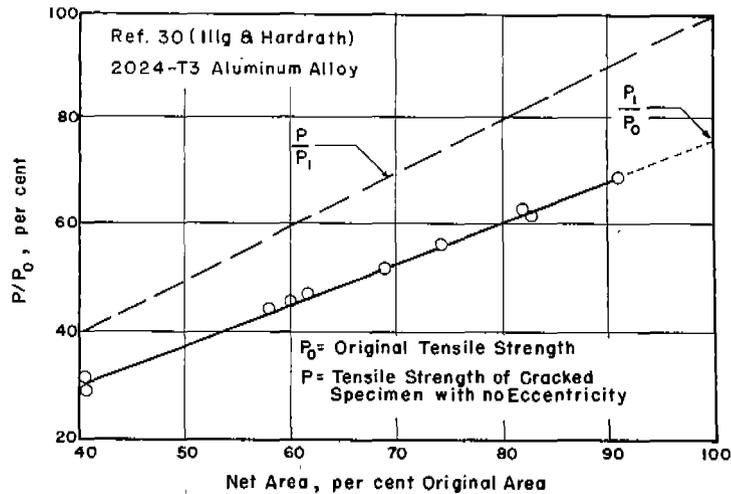
FIG. 5 STRENGTH OF SPECIMENS WITH FATIGUE CRACKS
