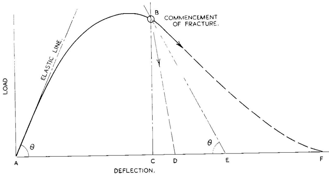
Fig. 4. A Schematic Load-Deflection Curve Indicating the Distinction between Stable and Unstable Fracturing. If the Curve Continues to the Right of the Reflected Elastic Line, BE, such as along BF, the Fracture will be of a Stable Kind, but if the Curve Continues to the Left of BE, the Fracture will be Unstable.
