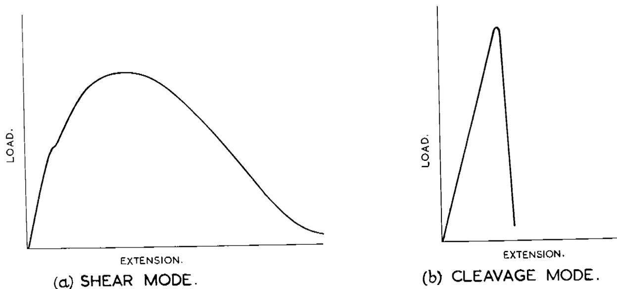
Fig. 3. Load-Extension Curves Illustrating Relevant Distinction between Shear and Cleavage Fracture Behavior.
