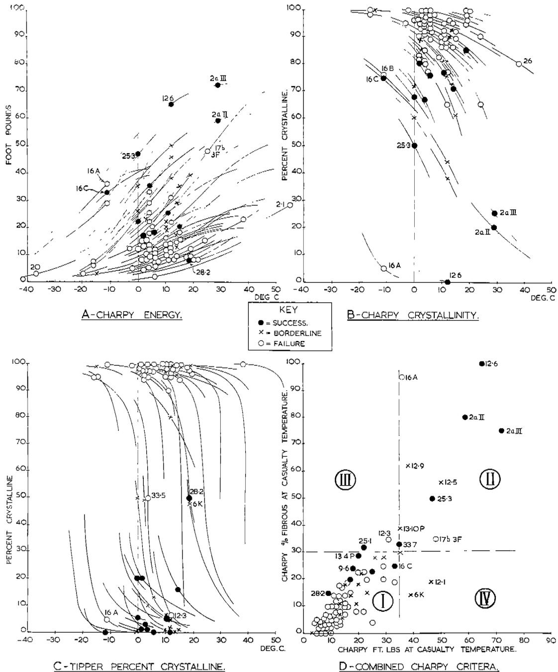
Fig. 8. Data from Various Tests on Ship Casualty Material.
