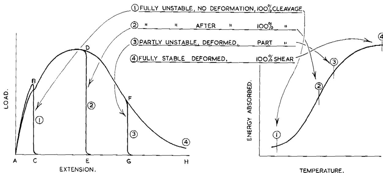
Fig. 6. Schematic Diagrams Representing Successive Charpy Tests on the Same Material at Different Temperatures.
