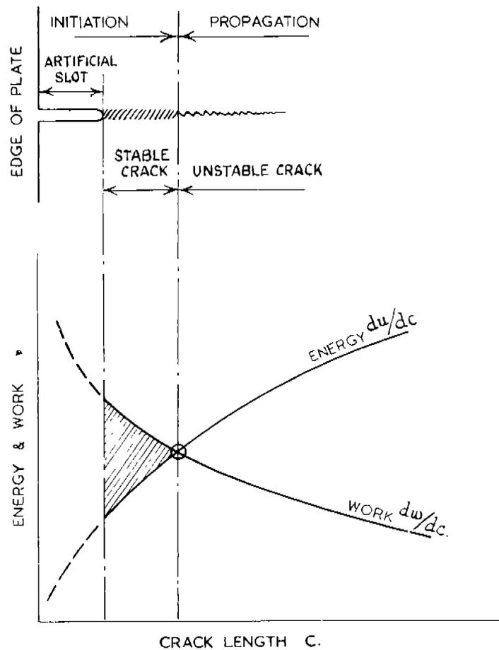
Fig. 5. Schematic Diagrams to Determine the Initiation and Propagation Stages of Fracture.
